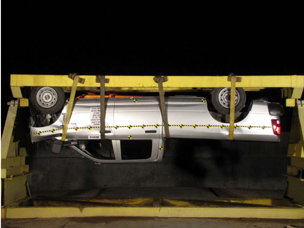
FIGURE 68. Vehicle at 180°on Static Rollover Device
