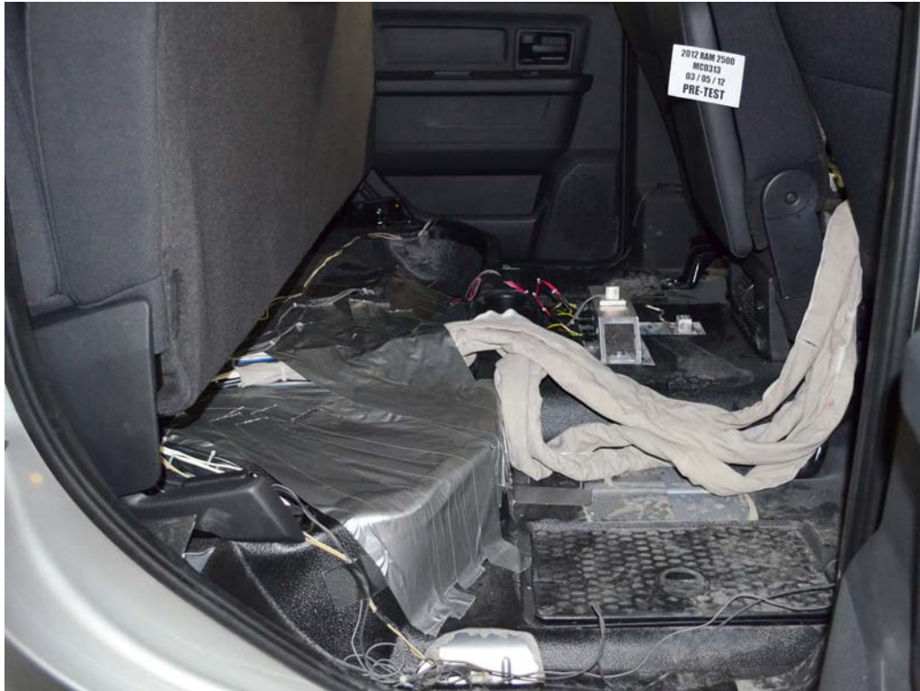
FIGURE 27. Pre-Test Dummy Cable Routing
