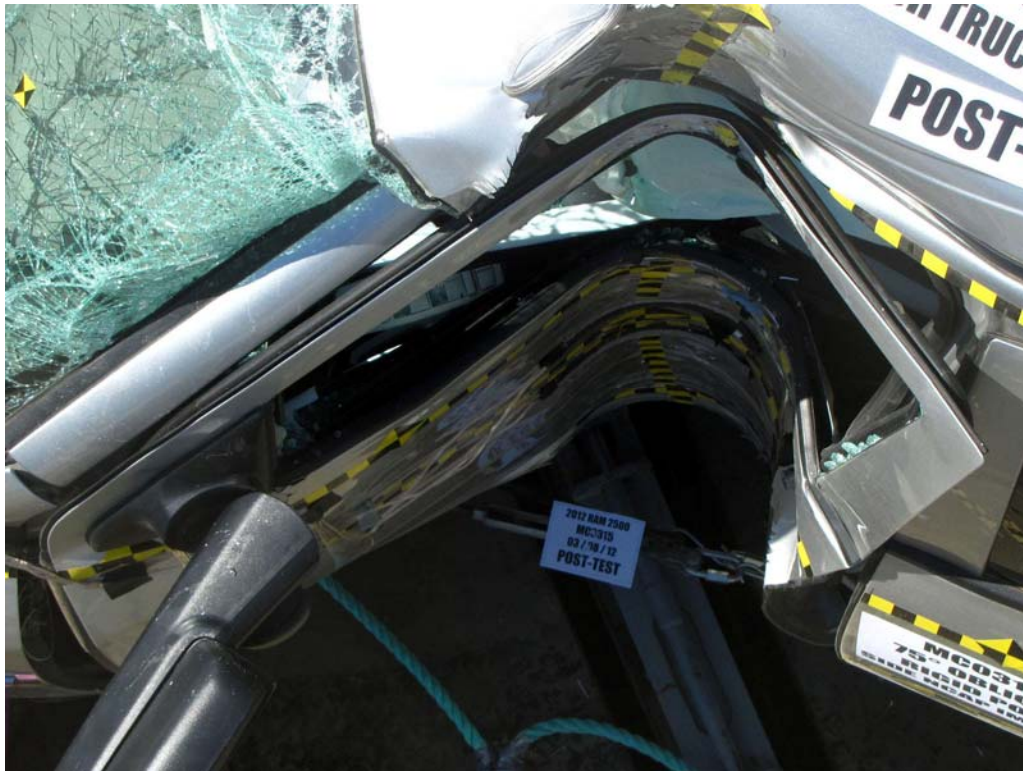
FIGURE 41. Post-Test Driver Dummy and Door Clearance
