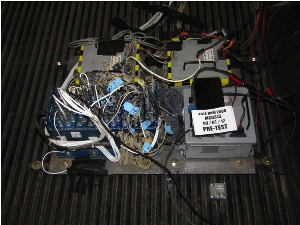
FIGURE 60. Pre-Test Ballast View
