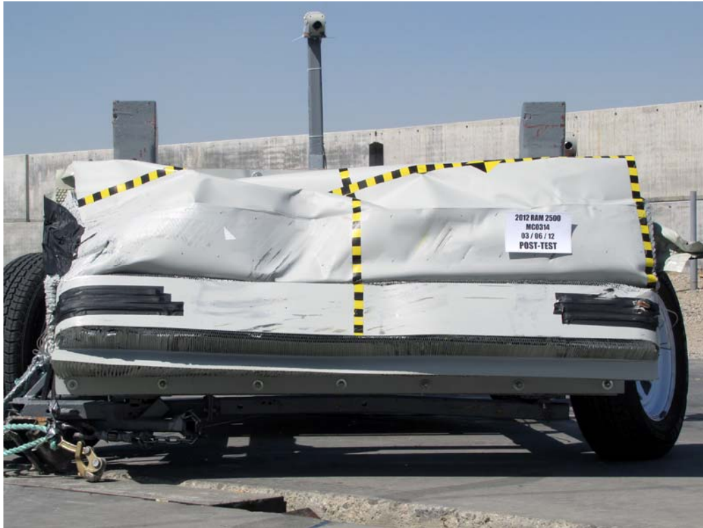
FIGURE 83. Post-Test Front View of MDB Impactor Face
