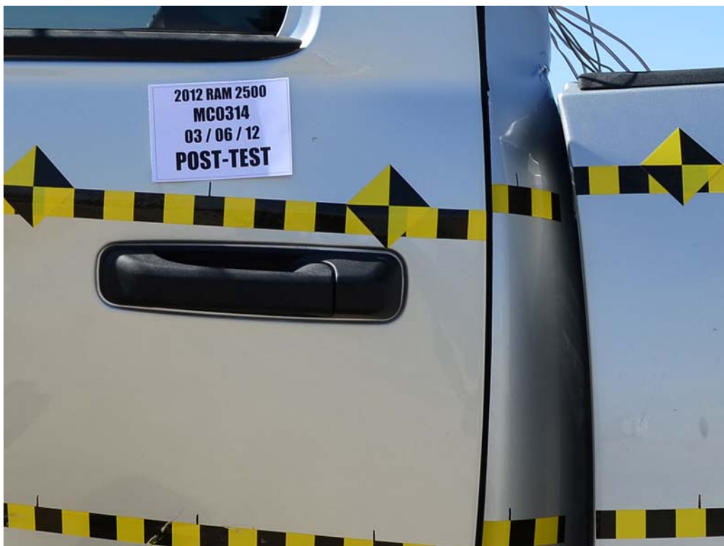
FIGURE 24. Post-Test Left Rear Door Latch Close-Up
