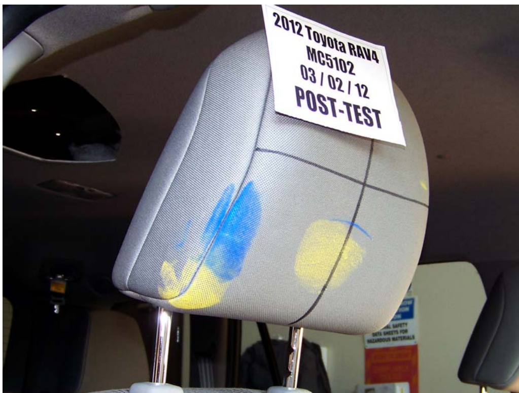
FIGURE 62a. Post-Test Passenger Dummy Contact With Headrest
