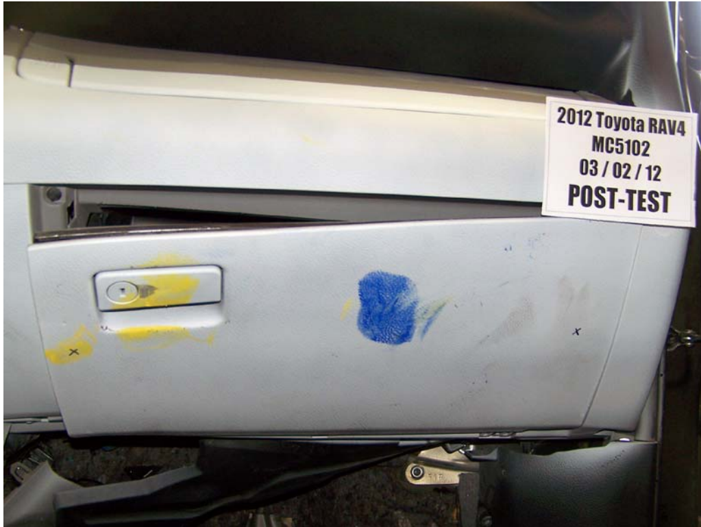
FIGURE 62b. Post-Test Passenger Dummy Contact With Glovebox
