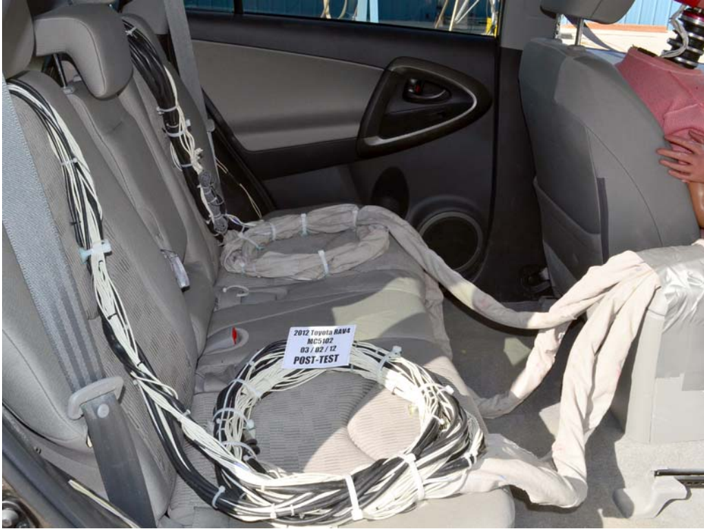
FIGURE 28. Post-Test Dummy Cable Routing
