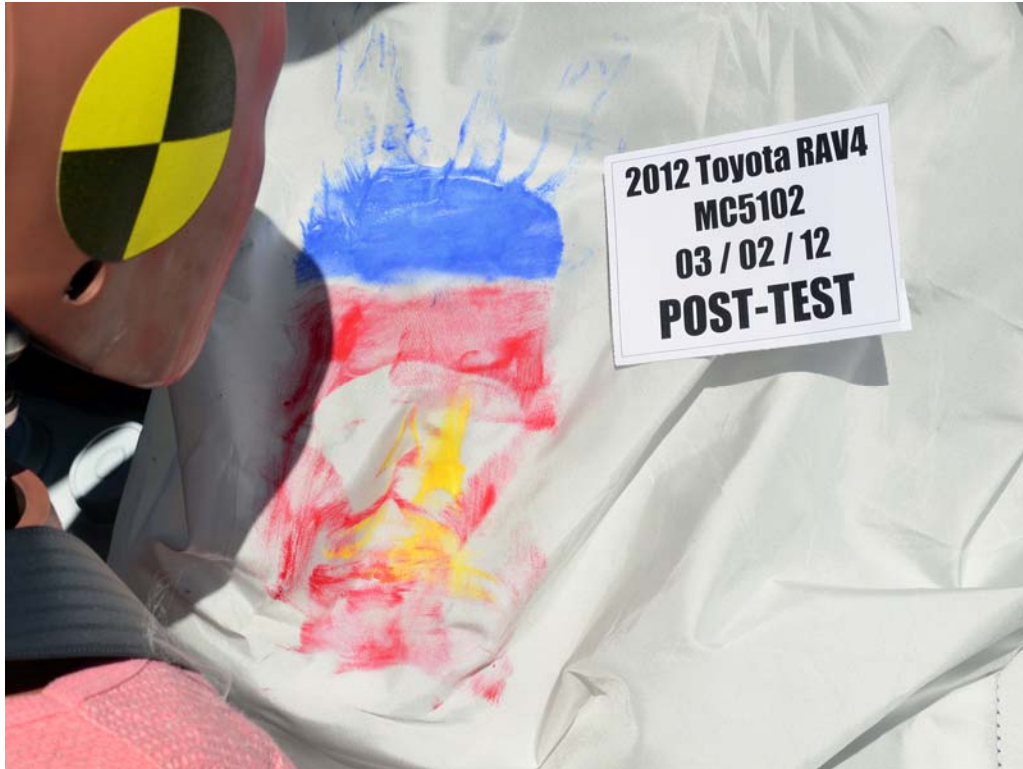
FIGURE 62. Post-Test Passenger Dummy Contact With Airbag
