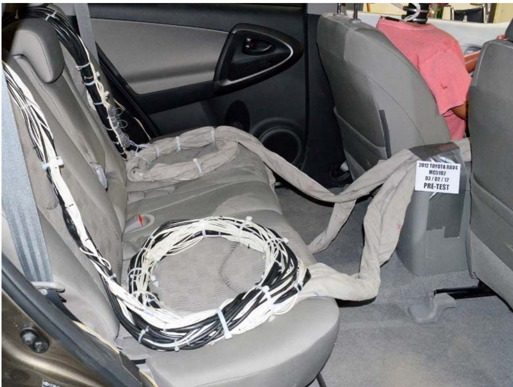
FIGURE 27. Pre-Test Dummy Cable Routing
