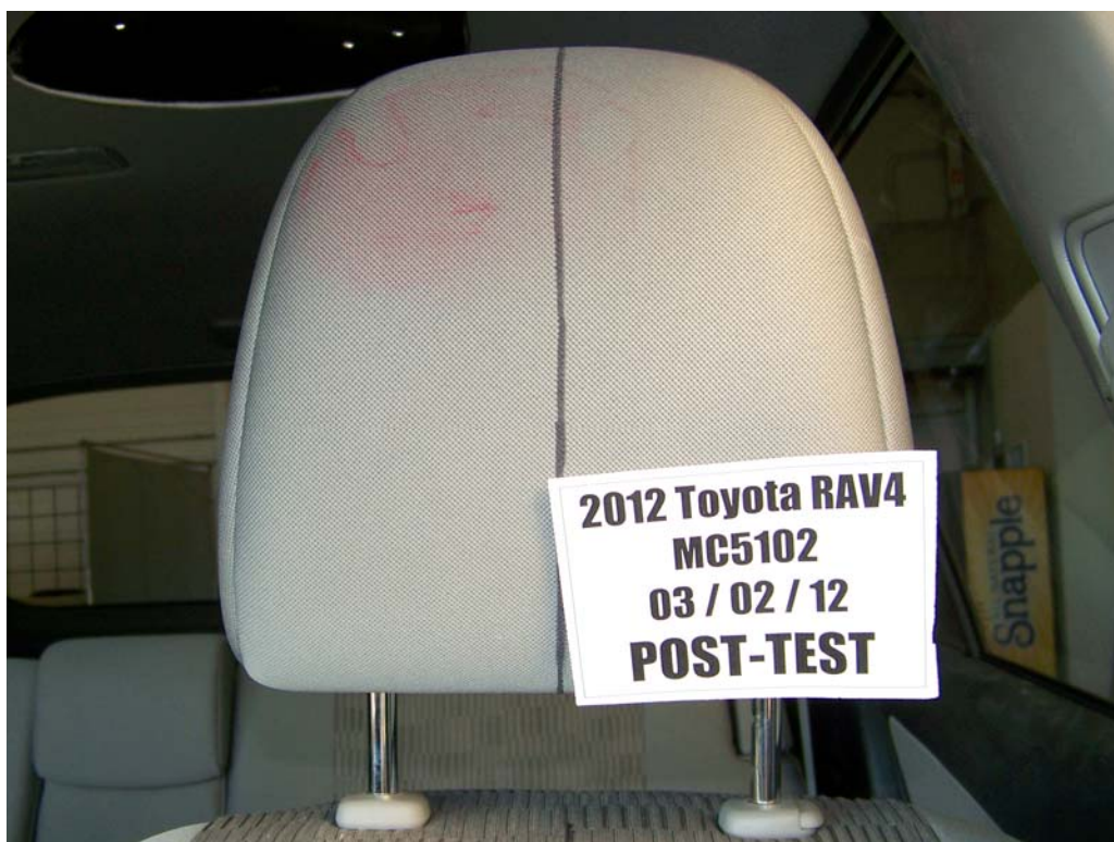
FIGURE 45. Post-Test Driver Dummy Contact With Headrest
