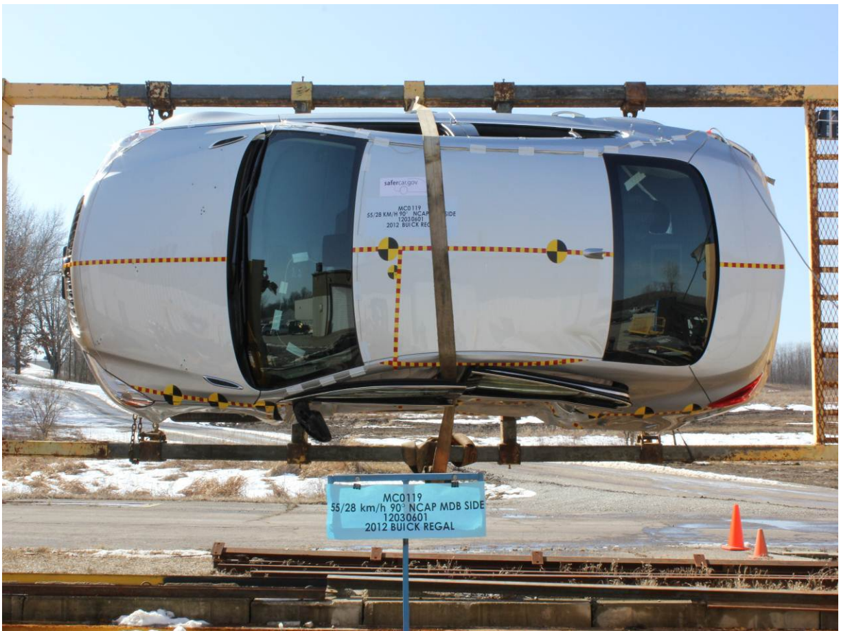
FMVSS No. 301 Static Rollover 270 Degrees
