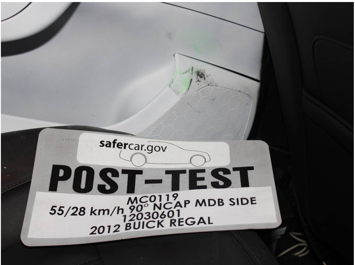
Post-Test Rear Passenger Dummy Knee Contact with Vehicle Interior View
