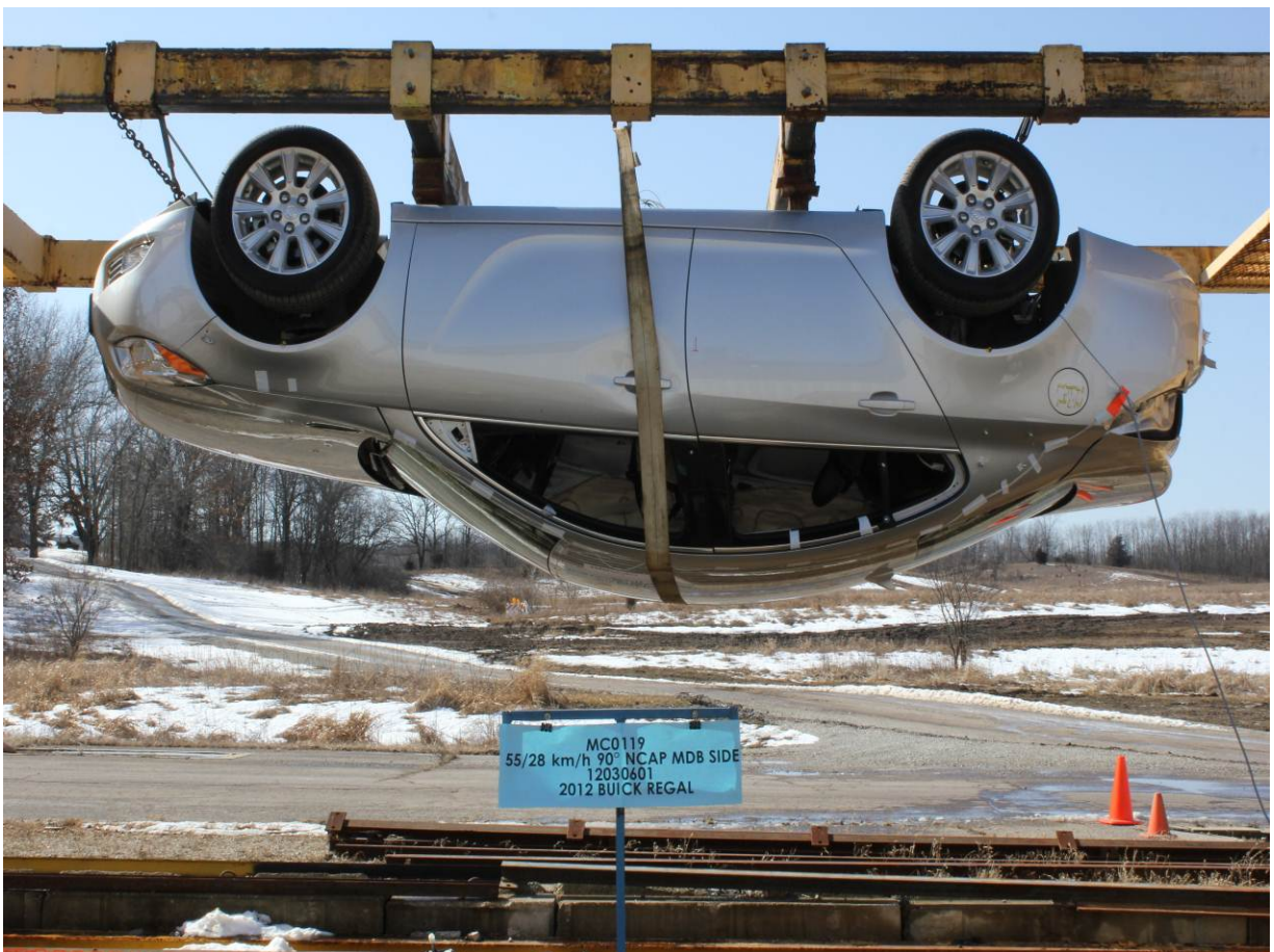
FMVSS No. 301 Static Rollover 180 Degrees
