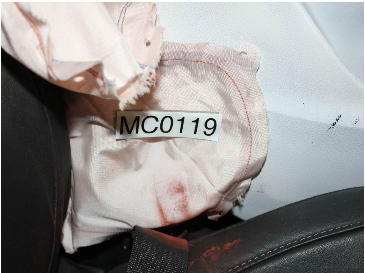
Post-Test Driver Dummy Close-up Pelvis Contact with Side Airbag View
