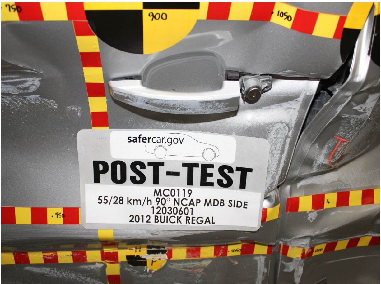
Post-Test Left Front Door Latch Close-Up
