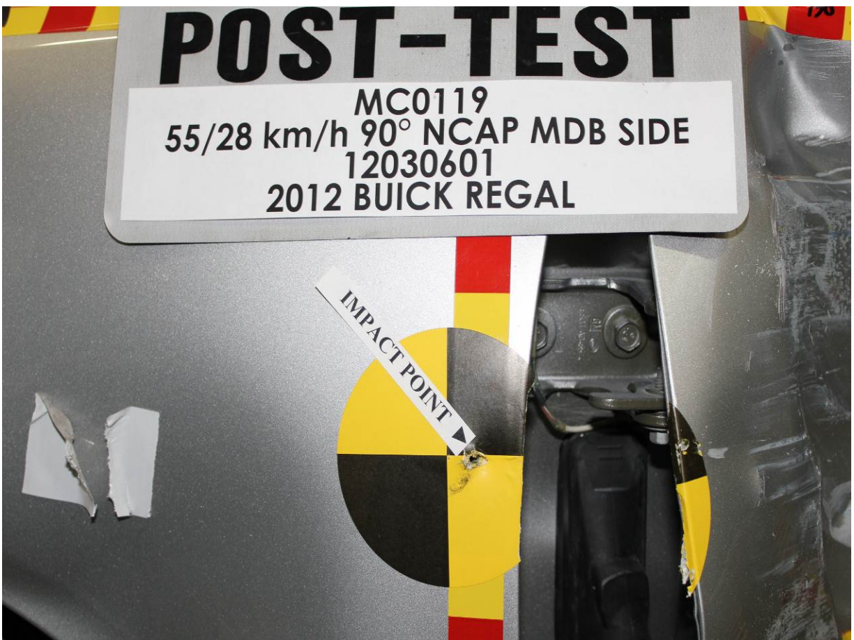
Post-Test Close-Up View of Impact Point Target
