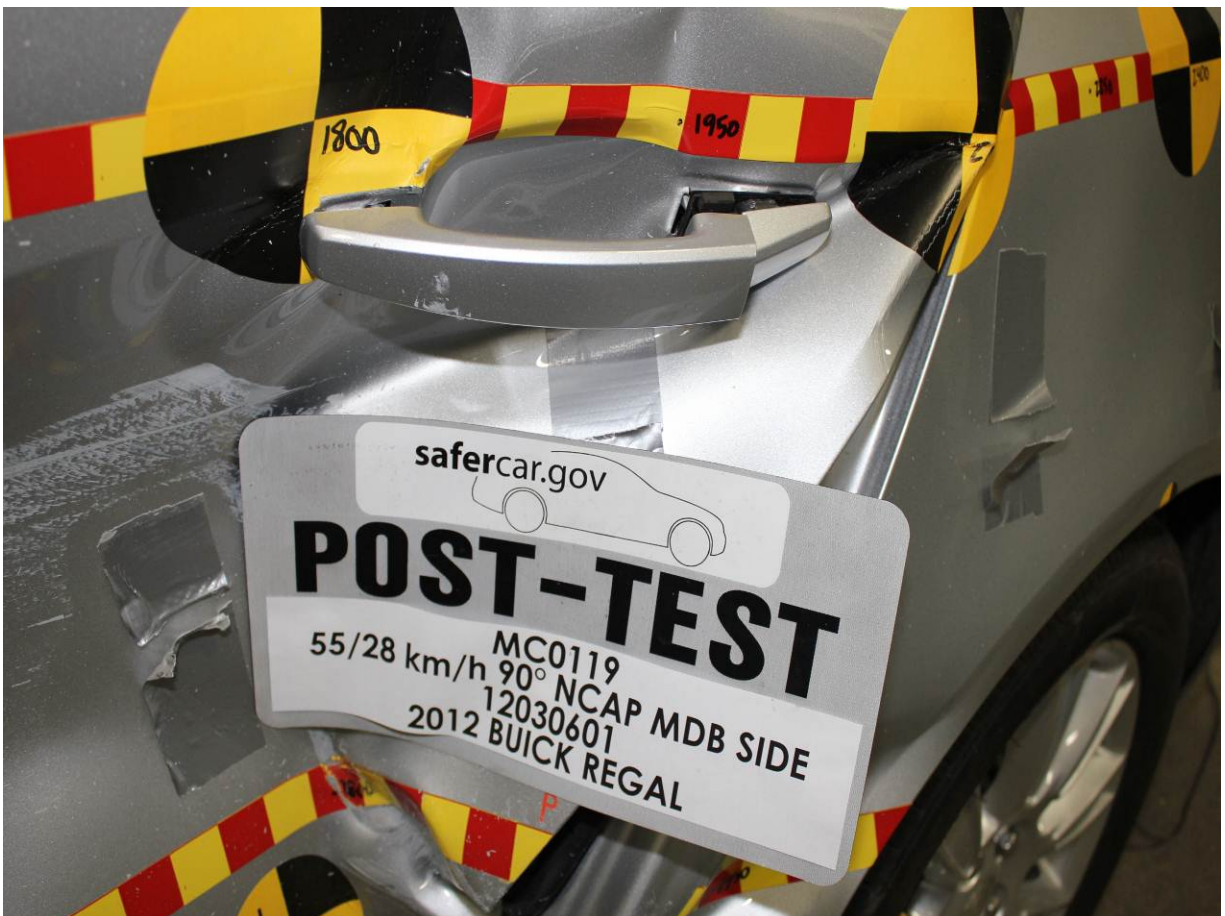
Post-Test Left Rear Door Latch Close-Up
