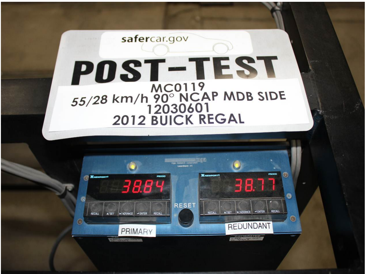
Post-Test Primary and Redundant Speed Trap Read-Out
