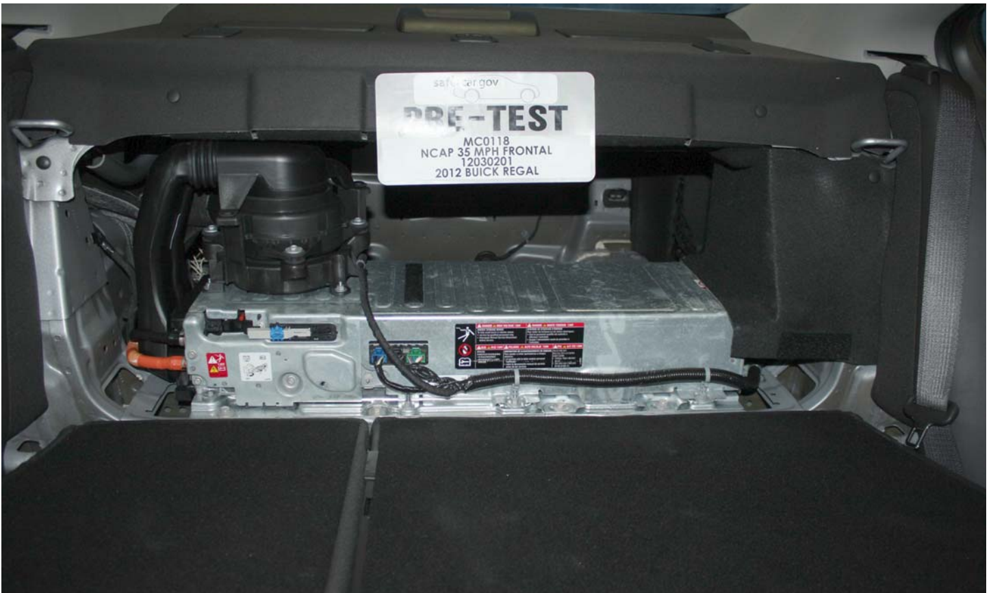
No. 020 Pre-Impact View Propulsion Battery Venting System(S)
