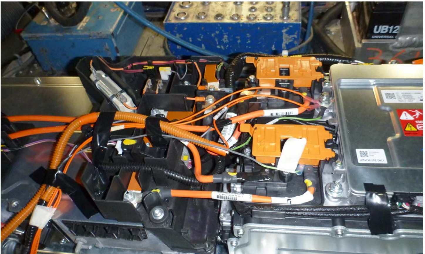
No. 014 Pre-Impact View Of Propulsion Battery Module(S)
