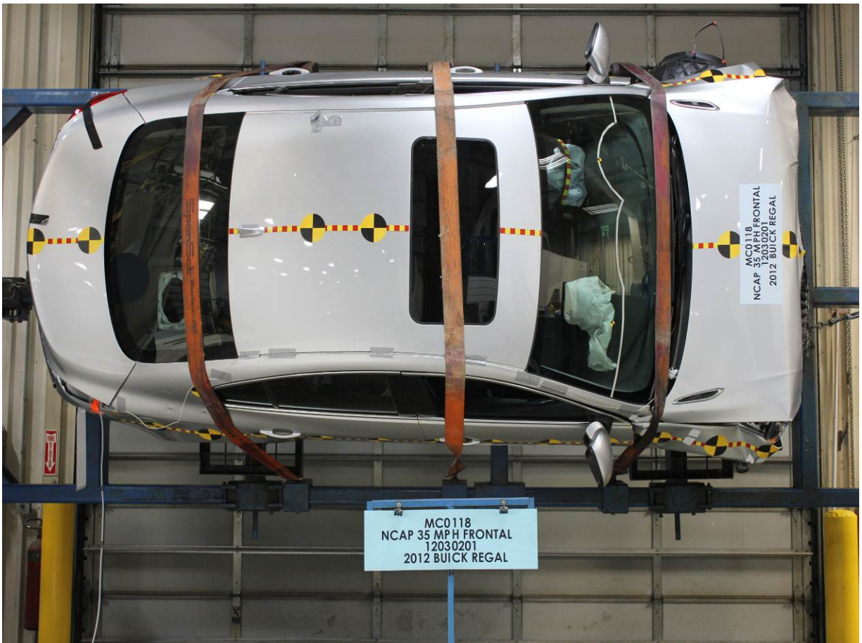
Vehicle at 90 Degrees on Static Rollover Device
