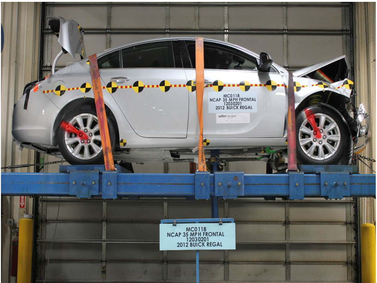
Vehicle at 360 Degrees on Static Rollover Device
