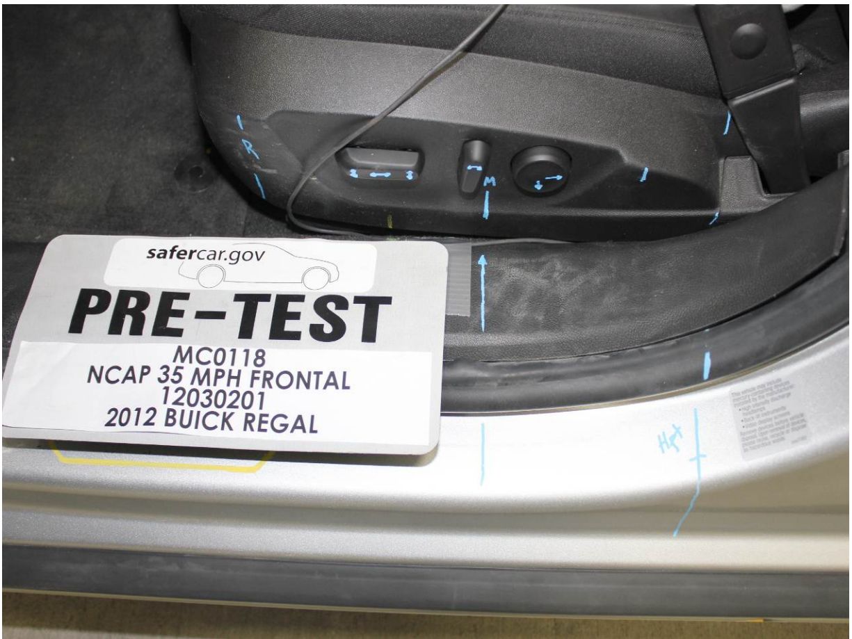
Pre-Test Driver's Seat Fore-Aft Markings
