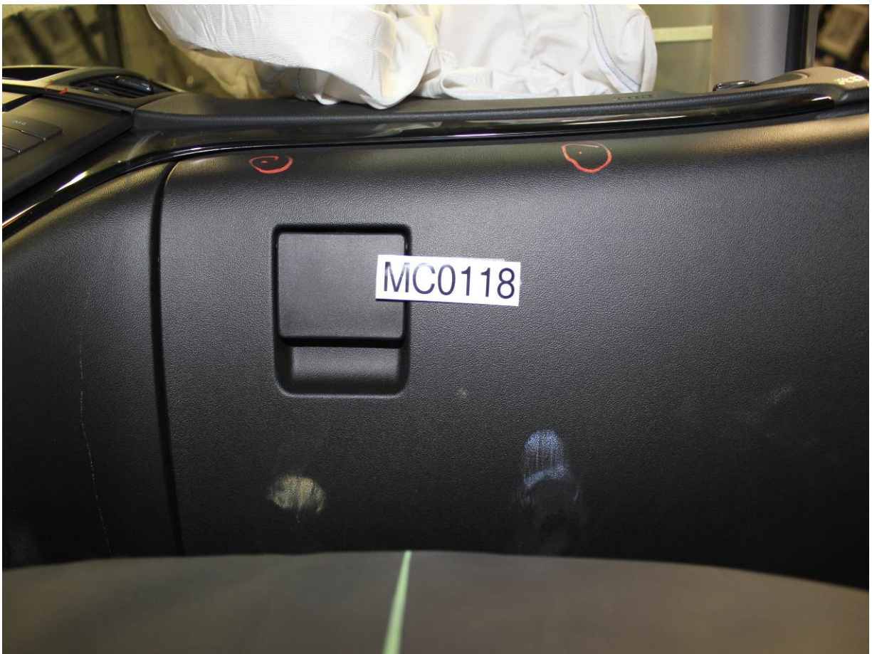
Post-Test Passenger Dummy Contact with Knee Bolster
