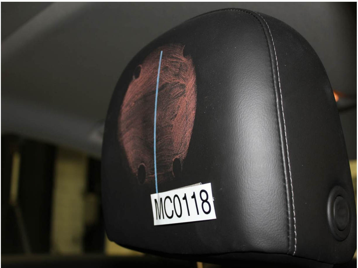
Post-Test Driver Dummy Contact with Headrest
