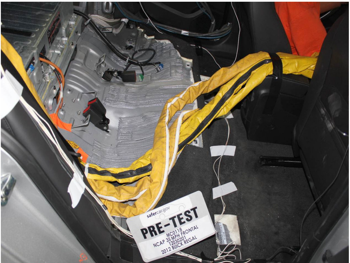
Pre-Test Dummy Cable Routing
