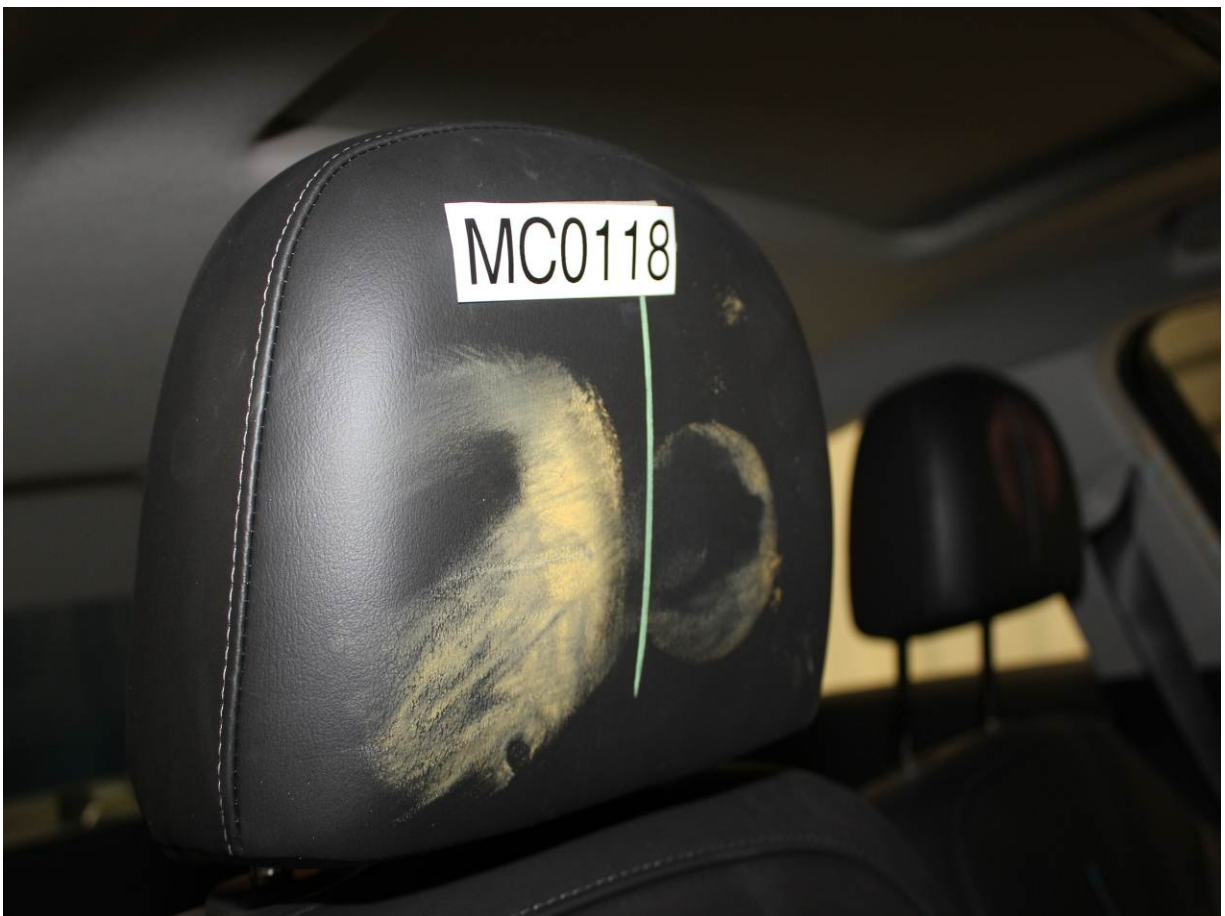
Post-Test Passenger Dummy Contact with Headrest
