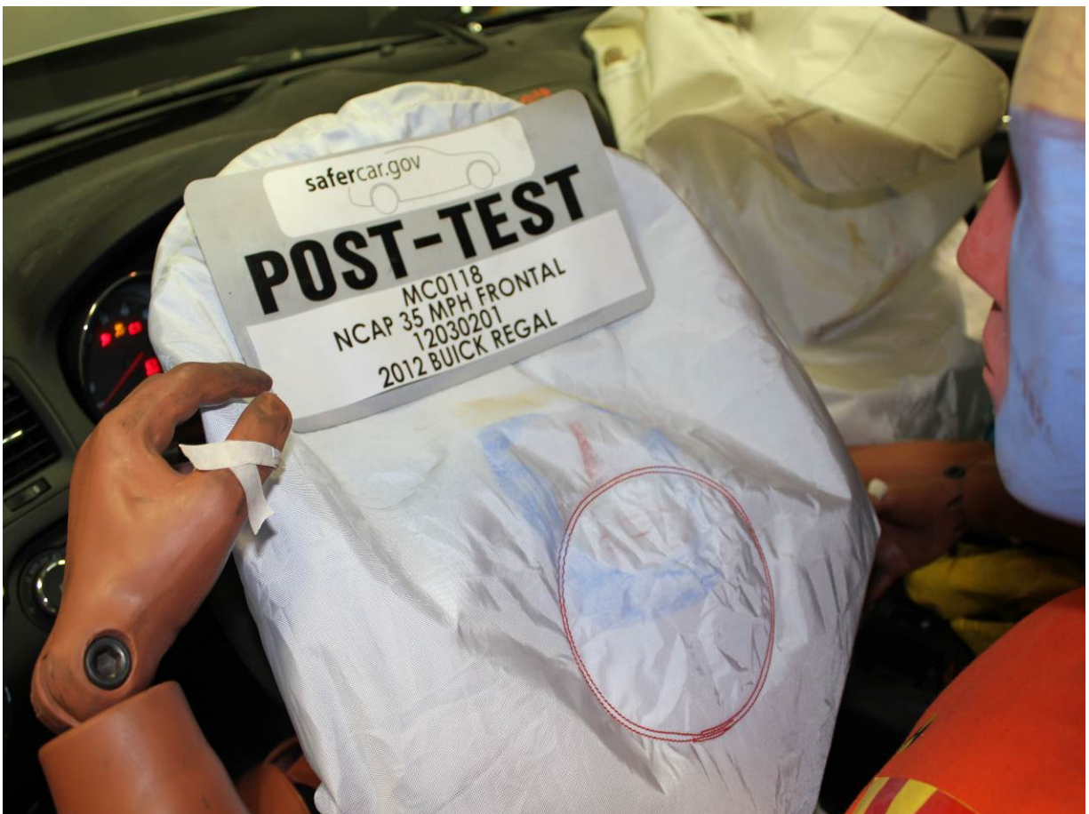
Post-Test Driver Dummy Contact with Airbag
