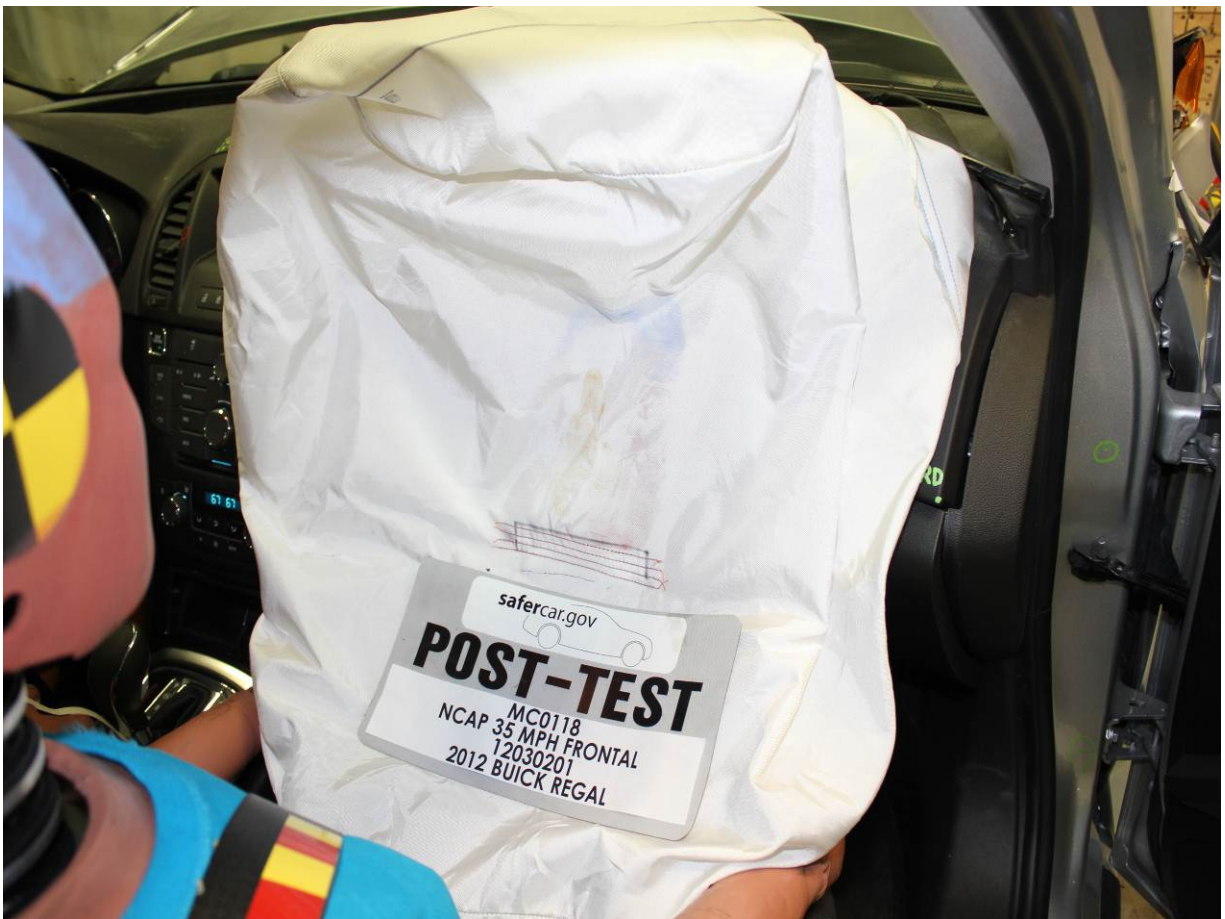
Post-Test Passenger Dummy Contact with Airbag
