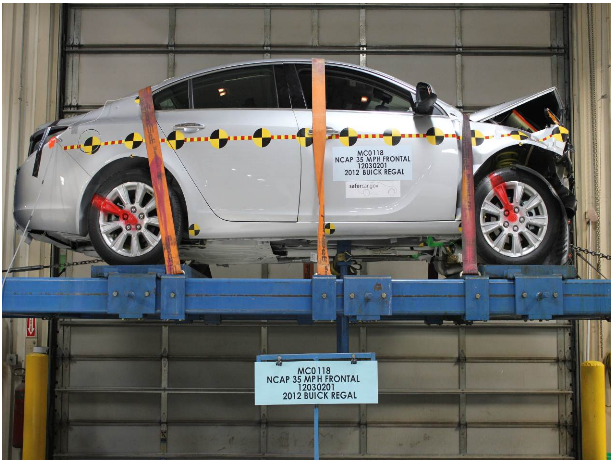
Vehicle at 0 Degrees on Static Rollover Device
