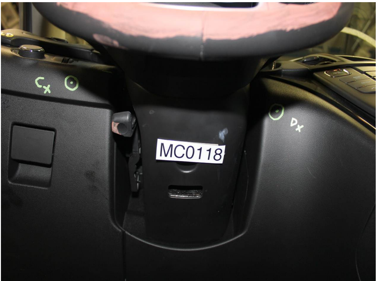
Post-Test Driver Dummy Contact with Knee Bolster
