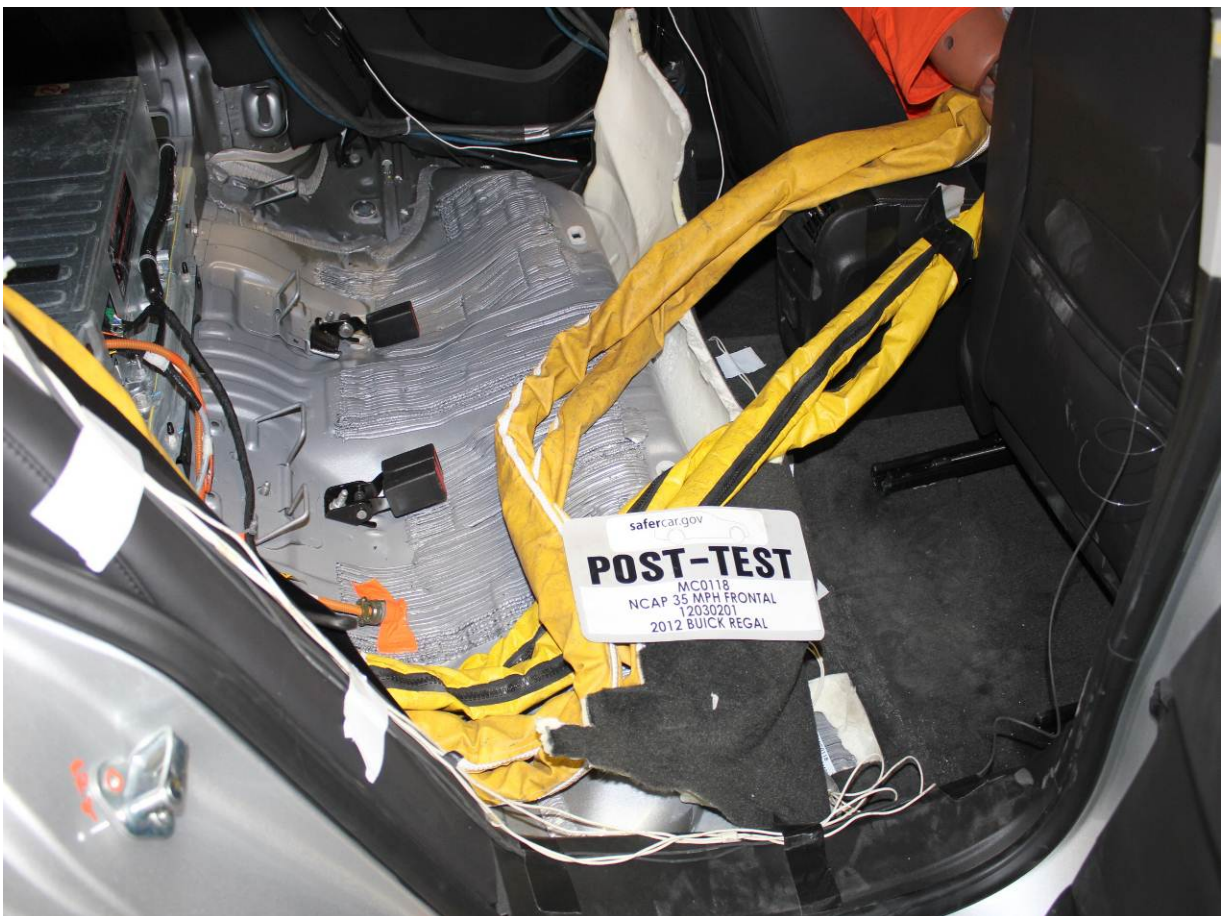
Post-Test Dummy Cable Routing
