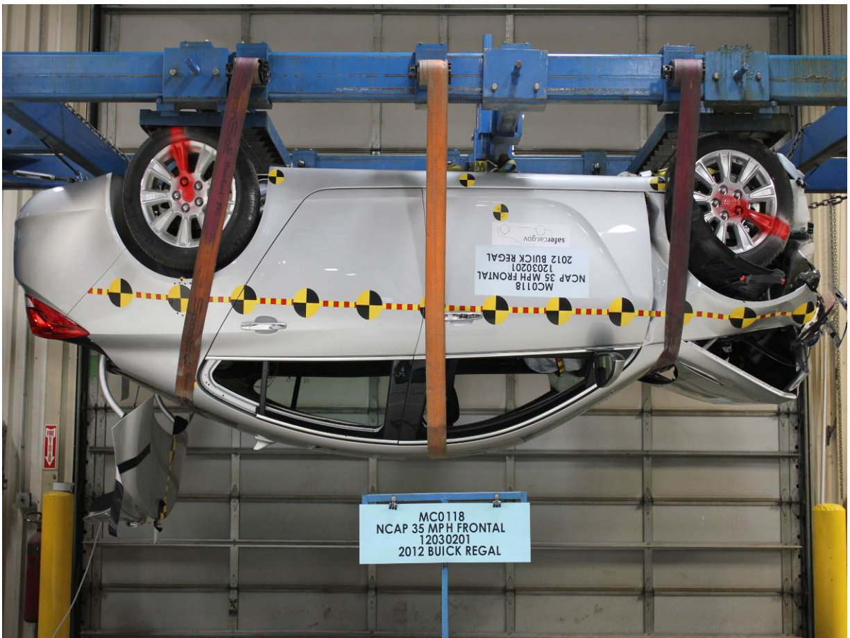
Vehicle at 180 Degrees on Static Rollover Device
