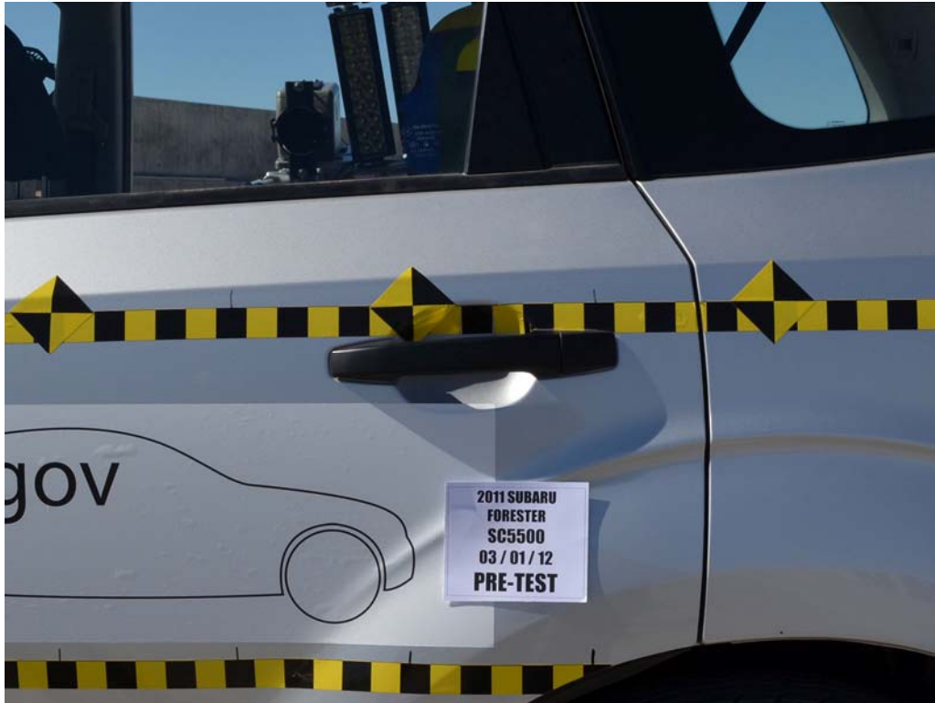
FIGURE 23. Pre-Test Left Rear Door Latch Close-Up
