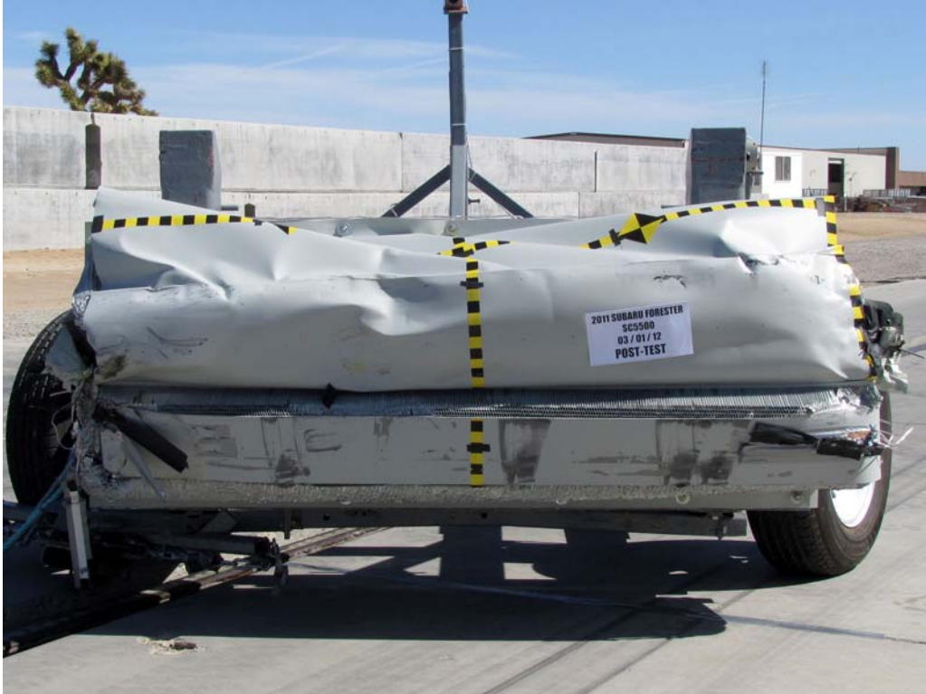
FIGURE 83. Post-Test Front View of MDB Impactor Face
