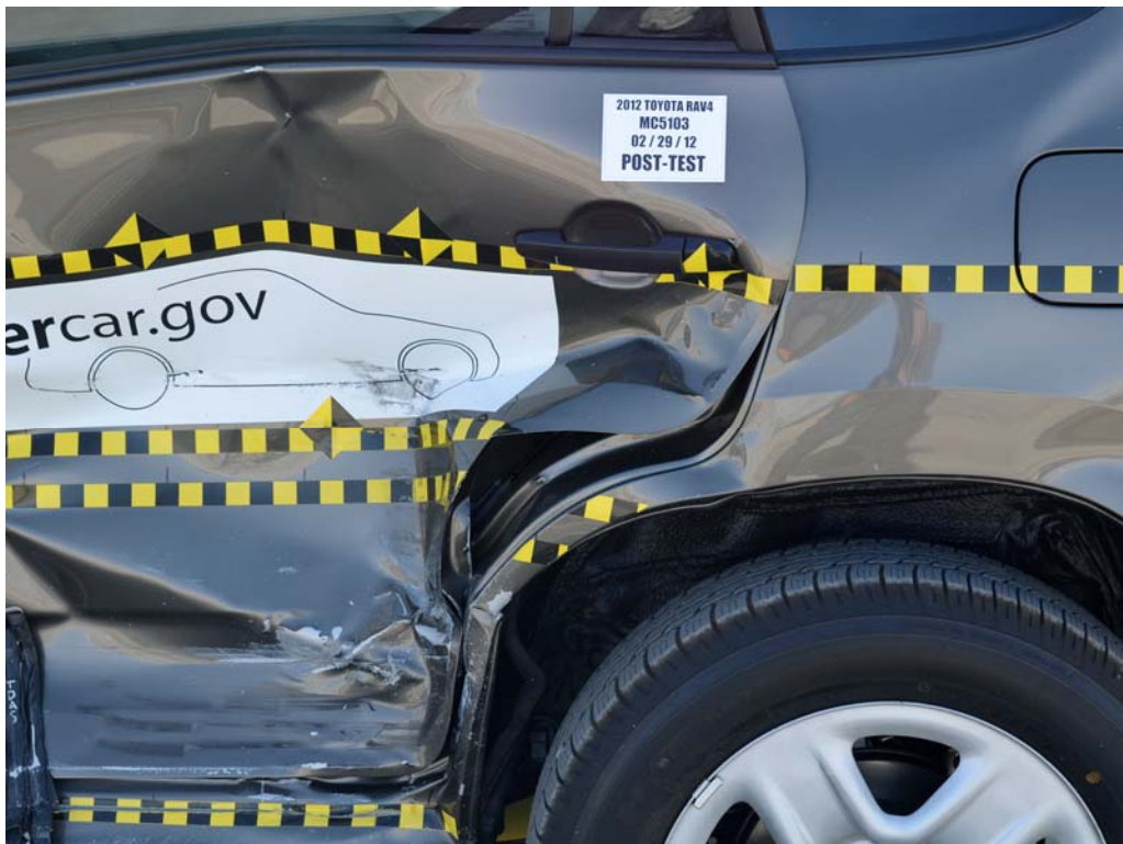
FIGURE 24. Post-Test Left Rear Door Latch Close-Up
