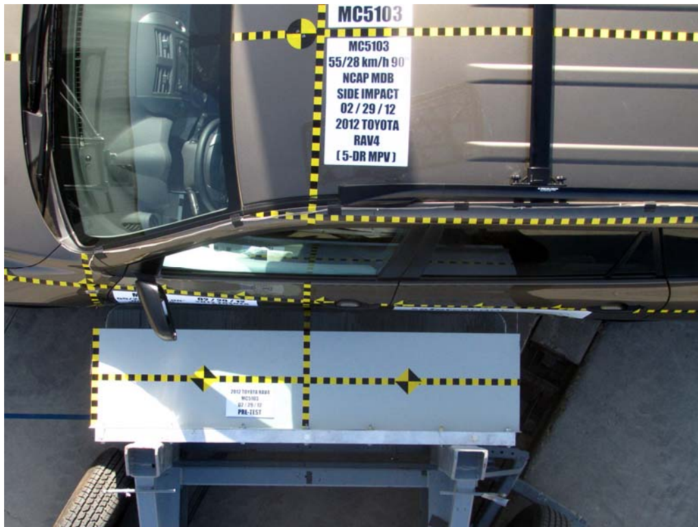
FIGURE 15. Pre-Test Overhead View of Test Area
