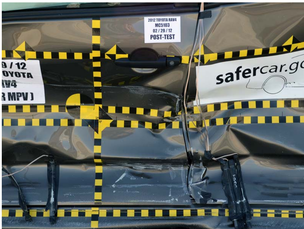
FIGURE 22. Post-Test Left Front Door Latch Close-Up
