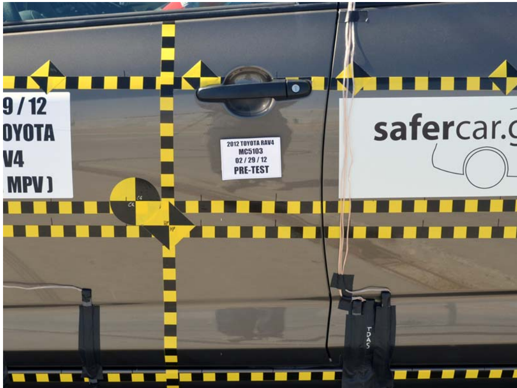
FIGURE 21. Pre-Test Left Front Door Latch Close-Up
