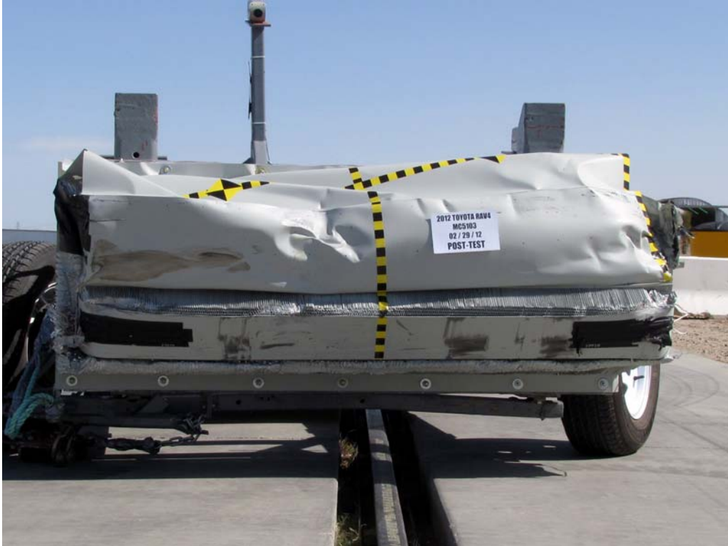
FIGURE 83. Post-Test Front View of MDB Impactor Face
