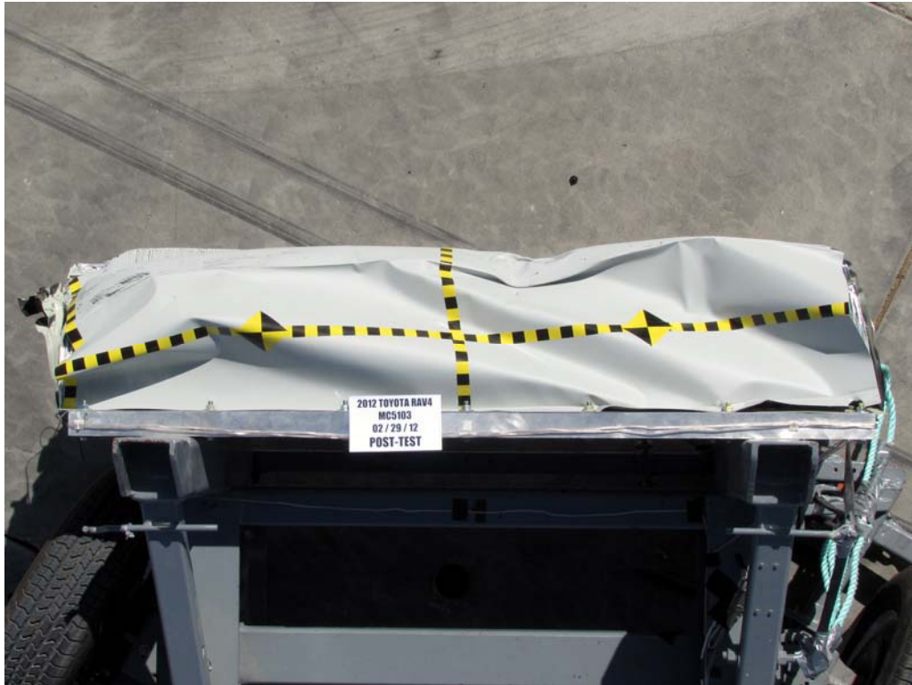
FIGURE 85. Post-Test Top View of MDB Impactor Face
