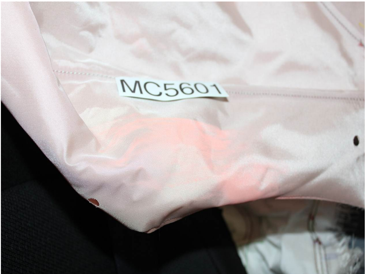
Post-Test Driver Dummy Close-up Torso Contact with Side Curtain Airbag View
