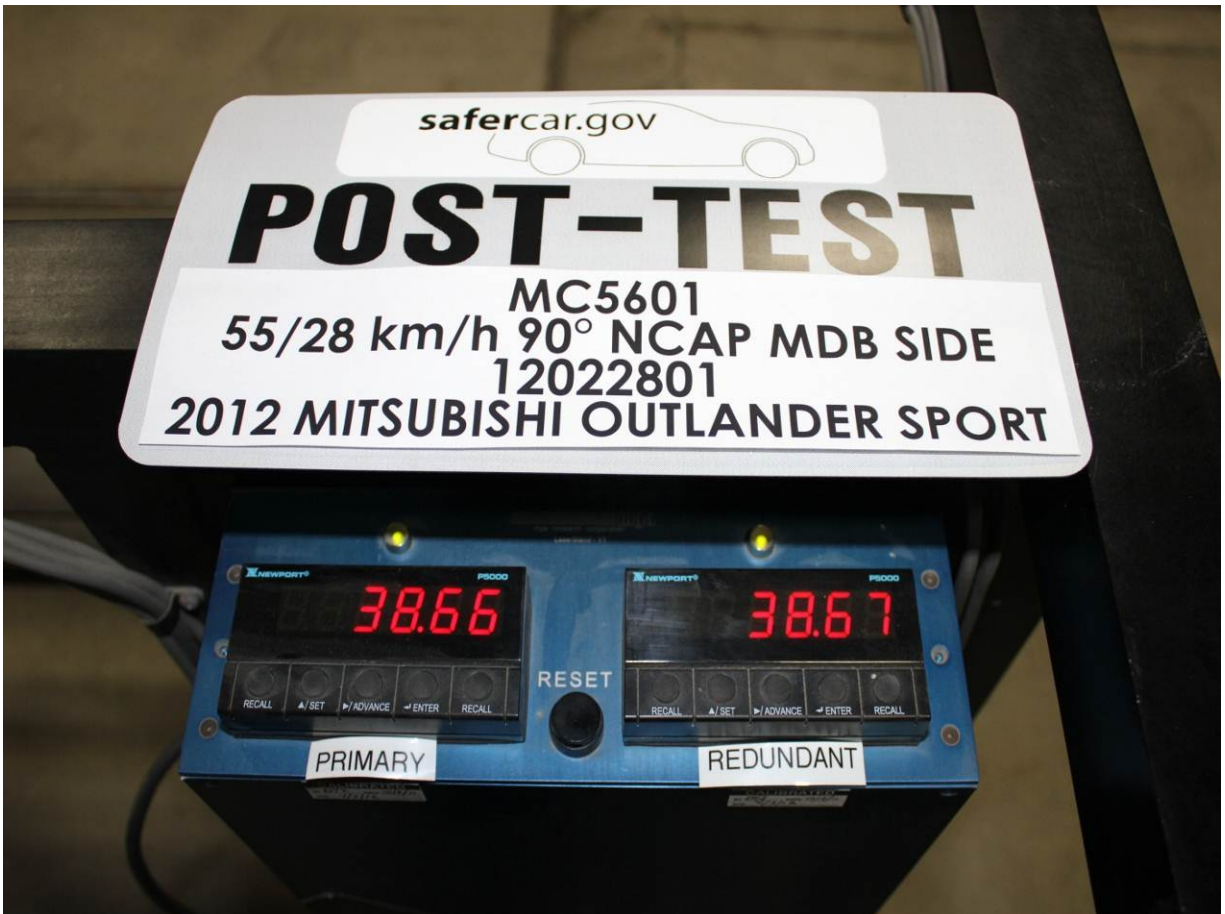
Post-Test Primary and Redundant Speed Trap Read-Out
