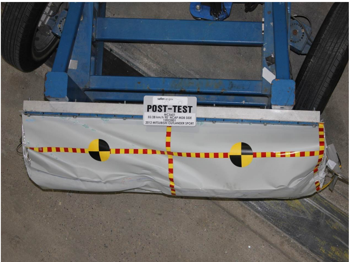
Post-Test Top View of MDB Impactor Face
