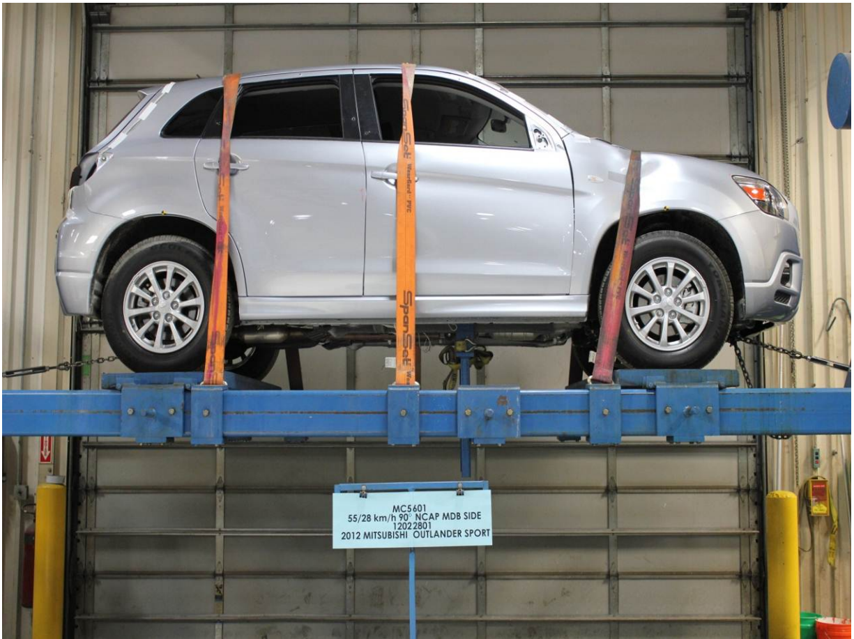
FMVSS No. 301 Static Rollover 360 Degrees
