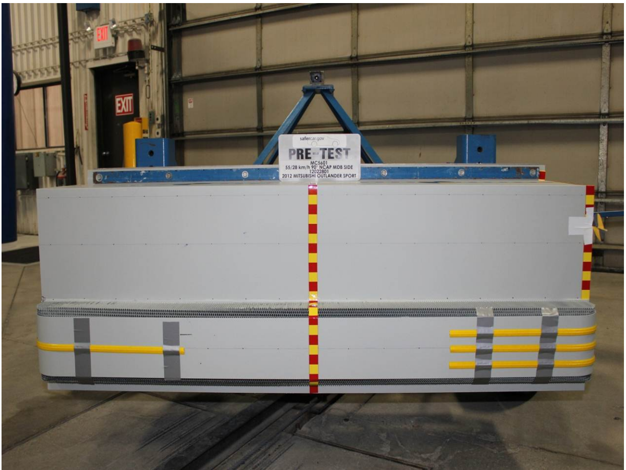
Pre-Test Front View of MDB Impactor Face
