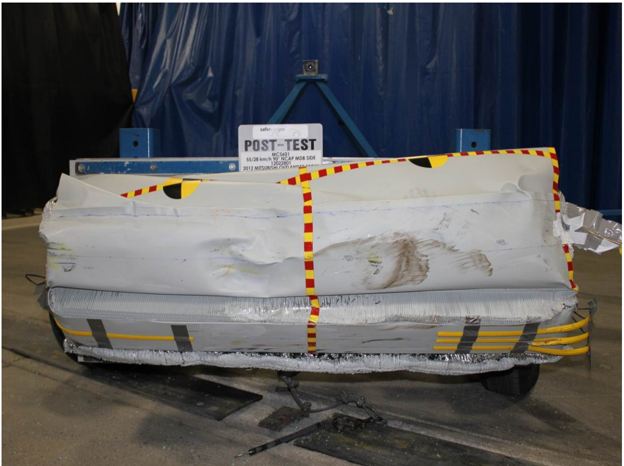
Post-Test Front View of MDB Impactor Face
