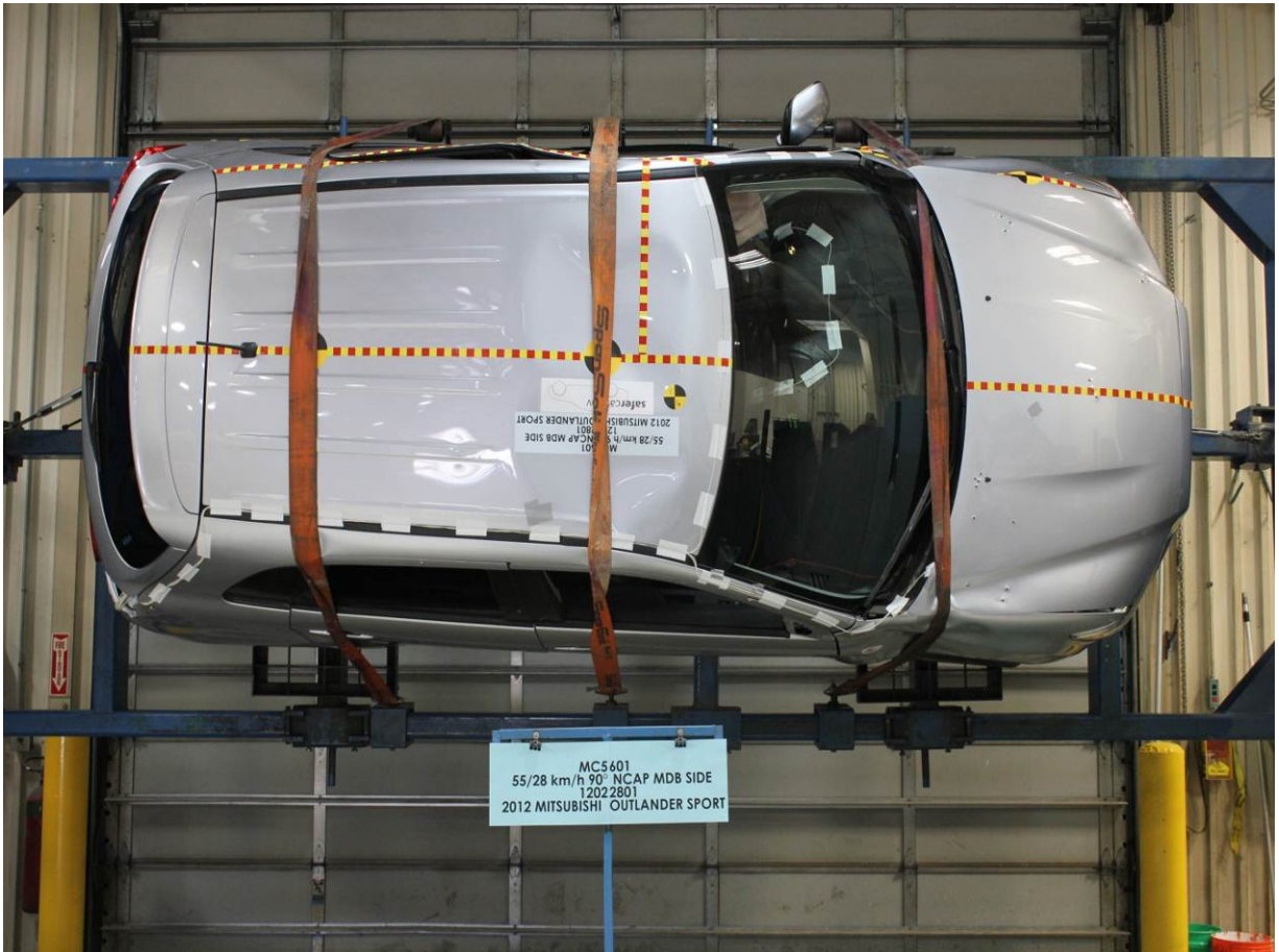
FMVSS No. 301 Static Rollover 270 Degrees
