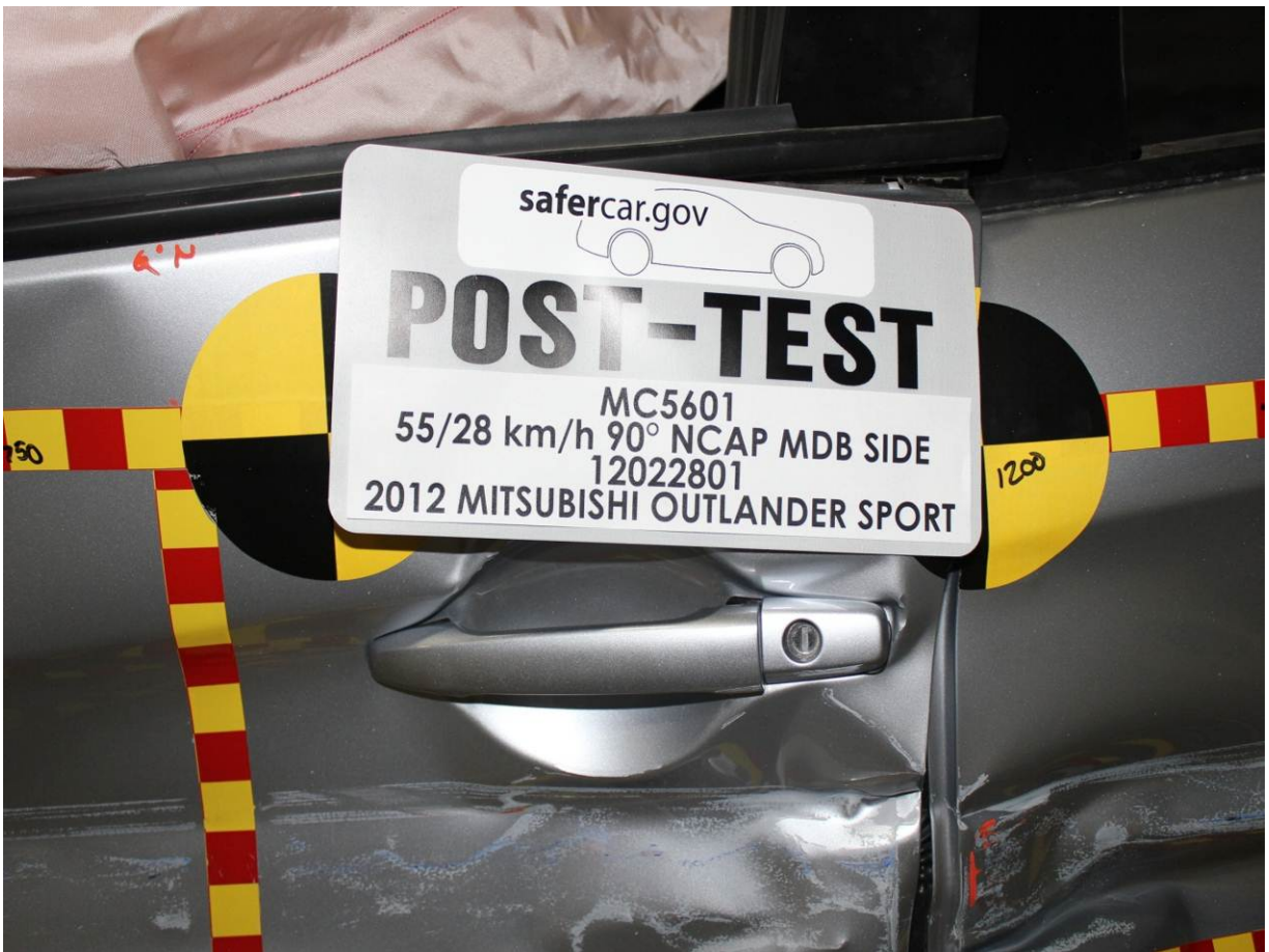
Post-Test Left Front Door Latch Close-Up
