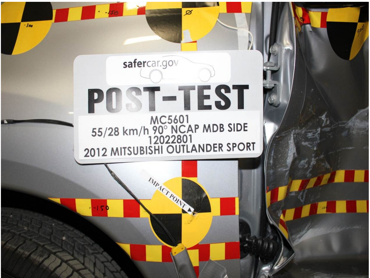
Post-Test Close-Up View of Impact Point Target
