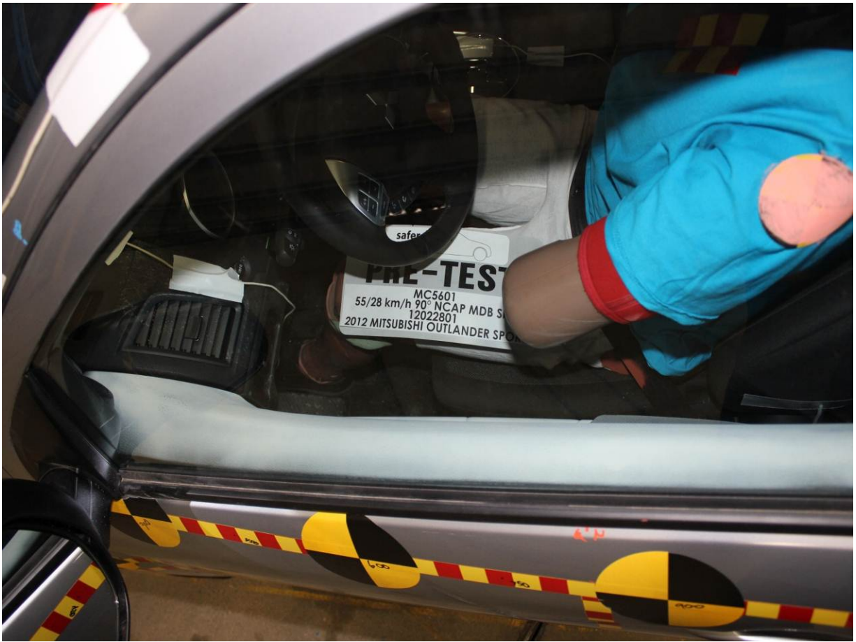
Pre-Test Driver Dummy and Door Clearance View
