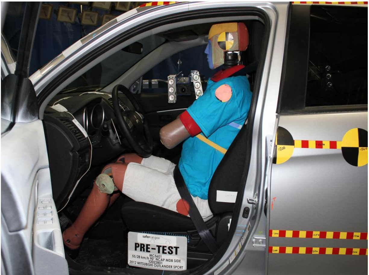
Pre-Test Left Side View of Driver Dummy Showing Belt and Chalking
