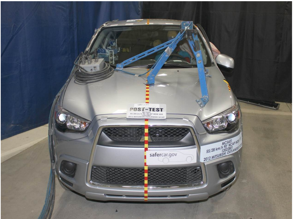
Post-Test Frontal View of Test Vehicle
