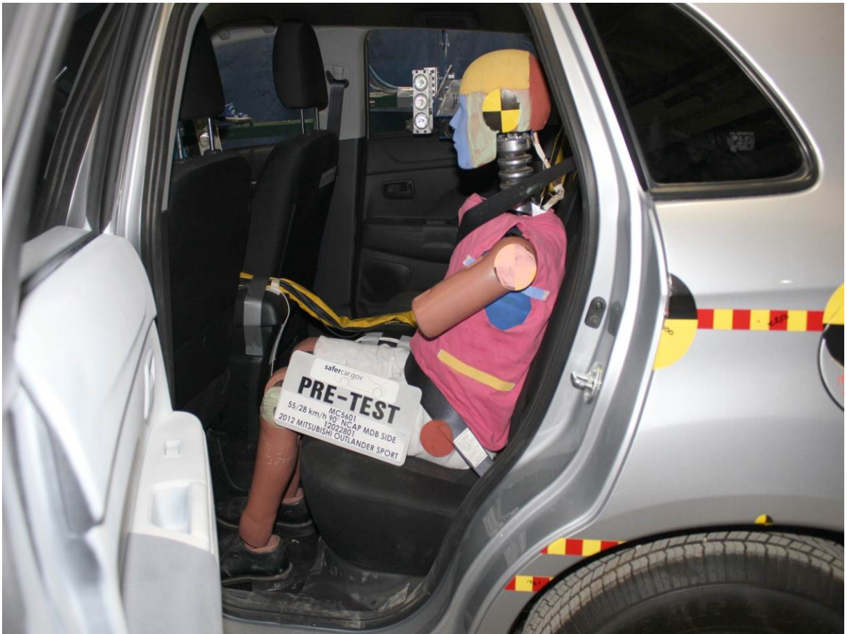
Pre-Test Left Side View of Rear Passenger Dummy Showing Belt and Chalking
