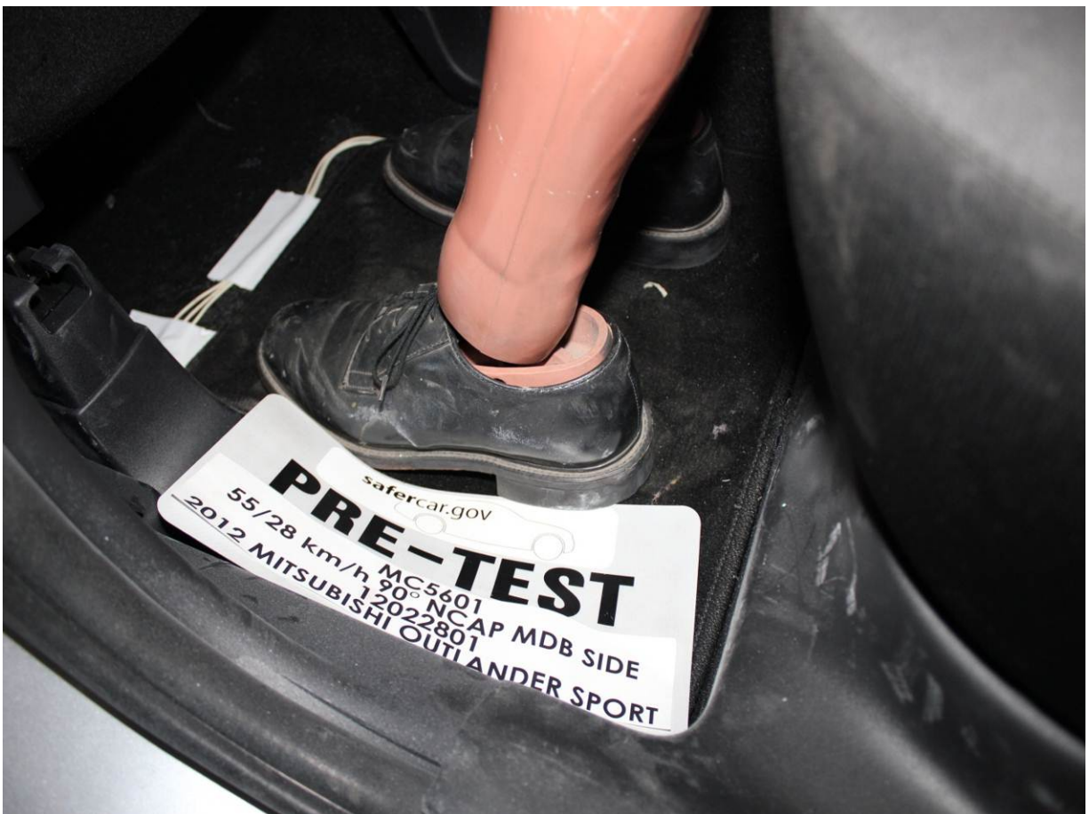
Pre-Test Placement of Rear Passenger Dummy's Feet
