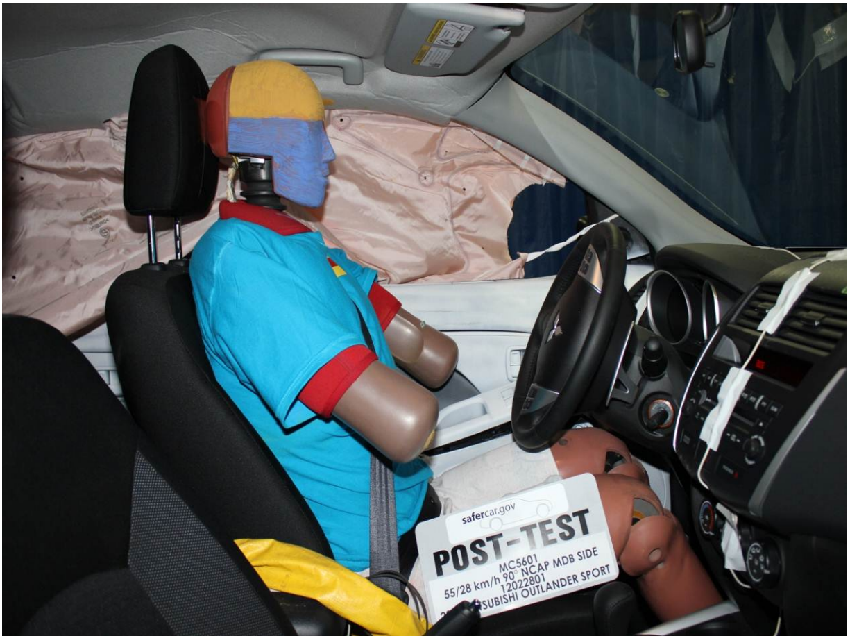
Post-Test Right Side View of Driver Dummy and Front Seat of Occupant Compartment
