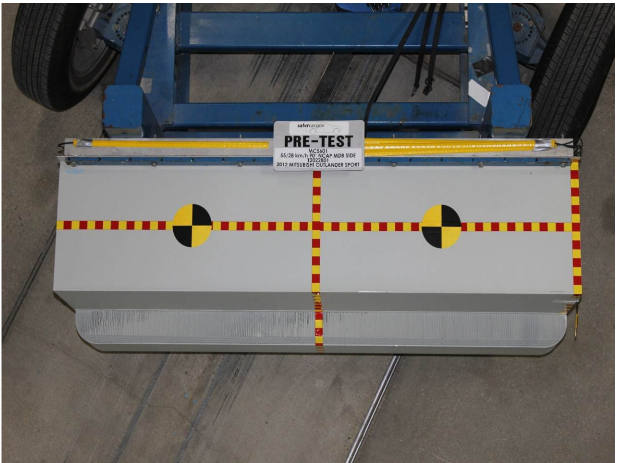
Pre-Test Top View of MDB Impactor Face
