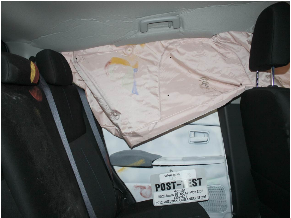
Post-Test Rear Passenger Inner Door Panel View
