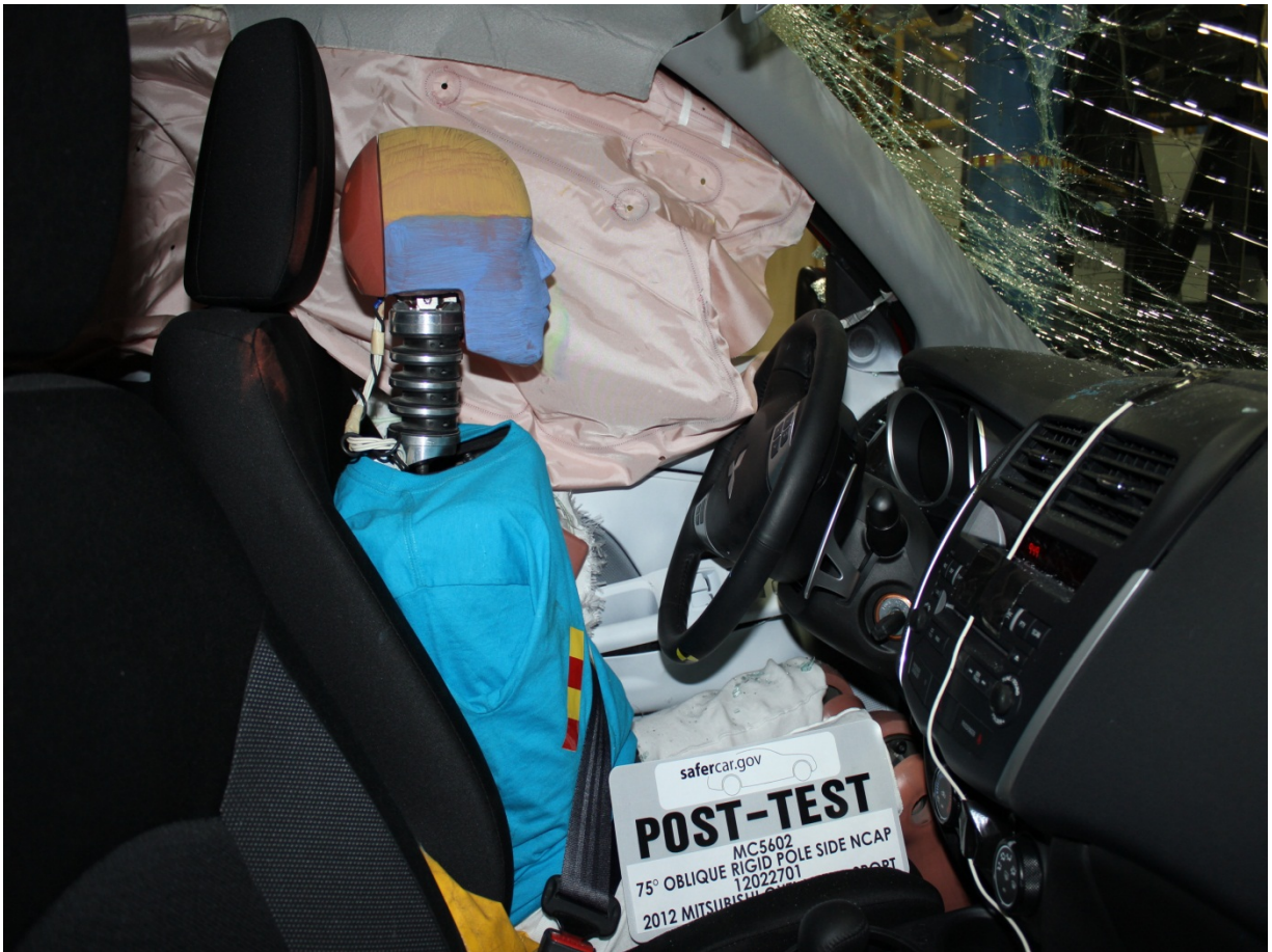
Post-Test Right Side View of Dummy and Front Seat of Occupant Compartment
