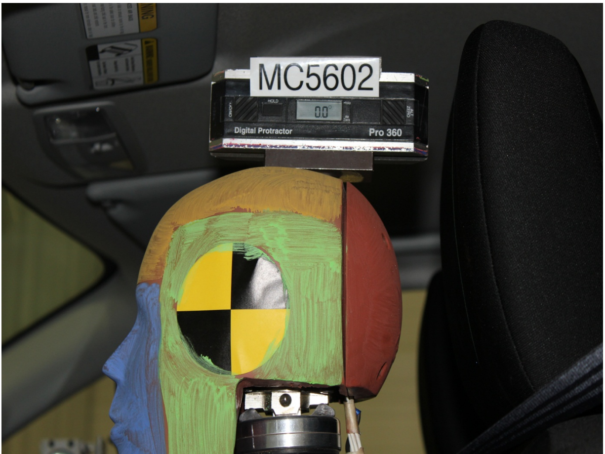
Pre-Test Left Side View of Dummy's Head Showing Dummy's Head is Level
