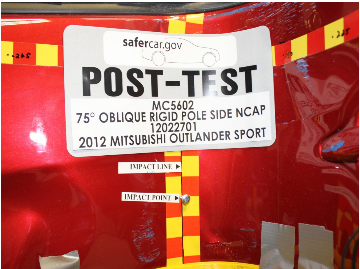
Post-Test Close-Up View of Impact Point Target Showing Impact Location
