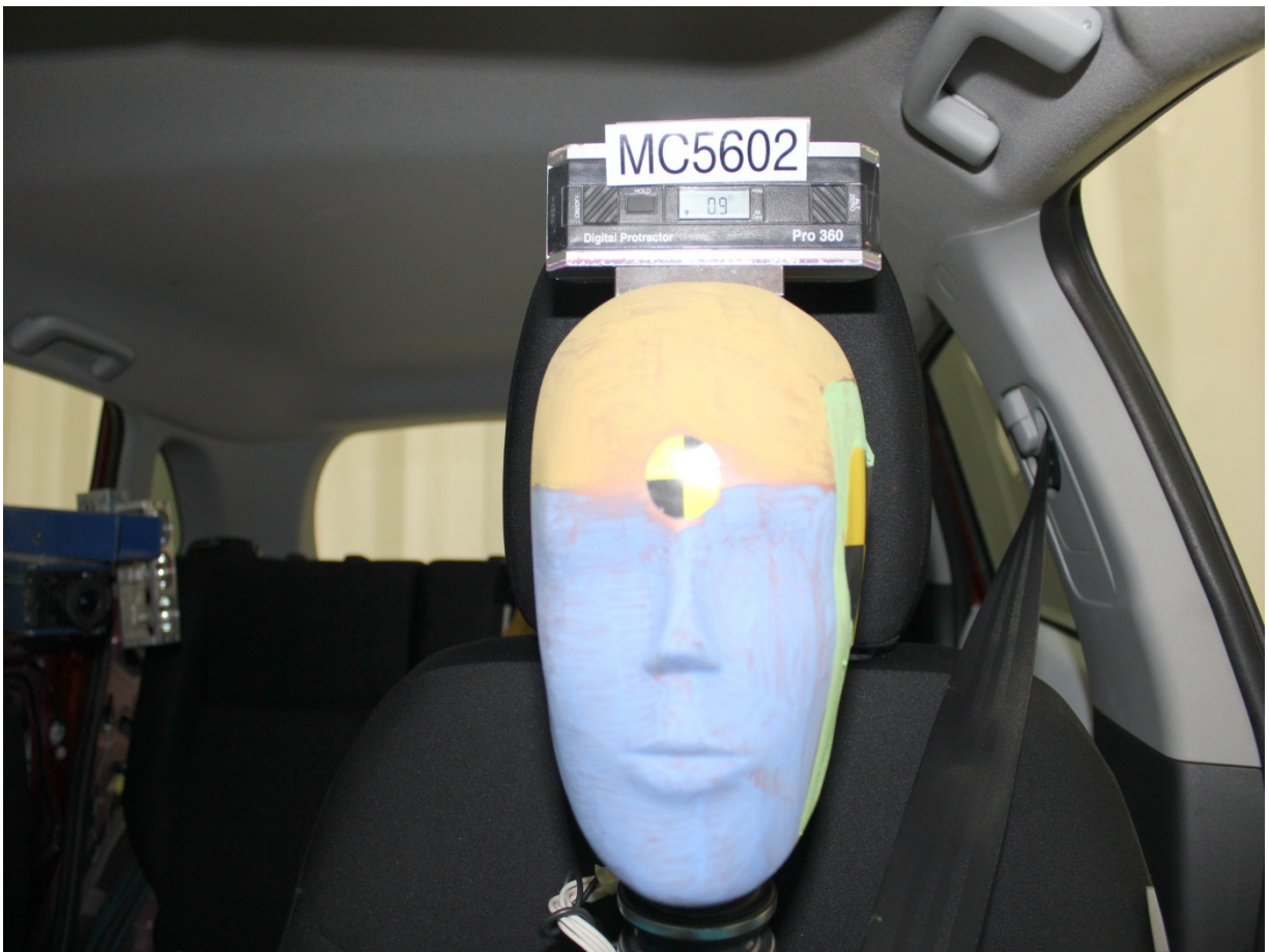
Pre-Test Front Close-Up View of Dummy Head and Shoulders in Relation to Head Restraint
