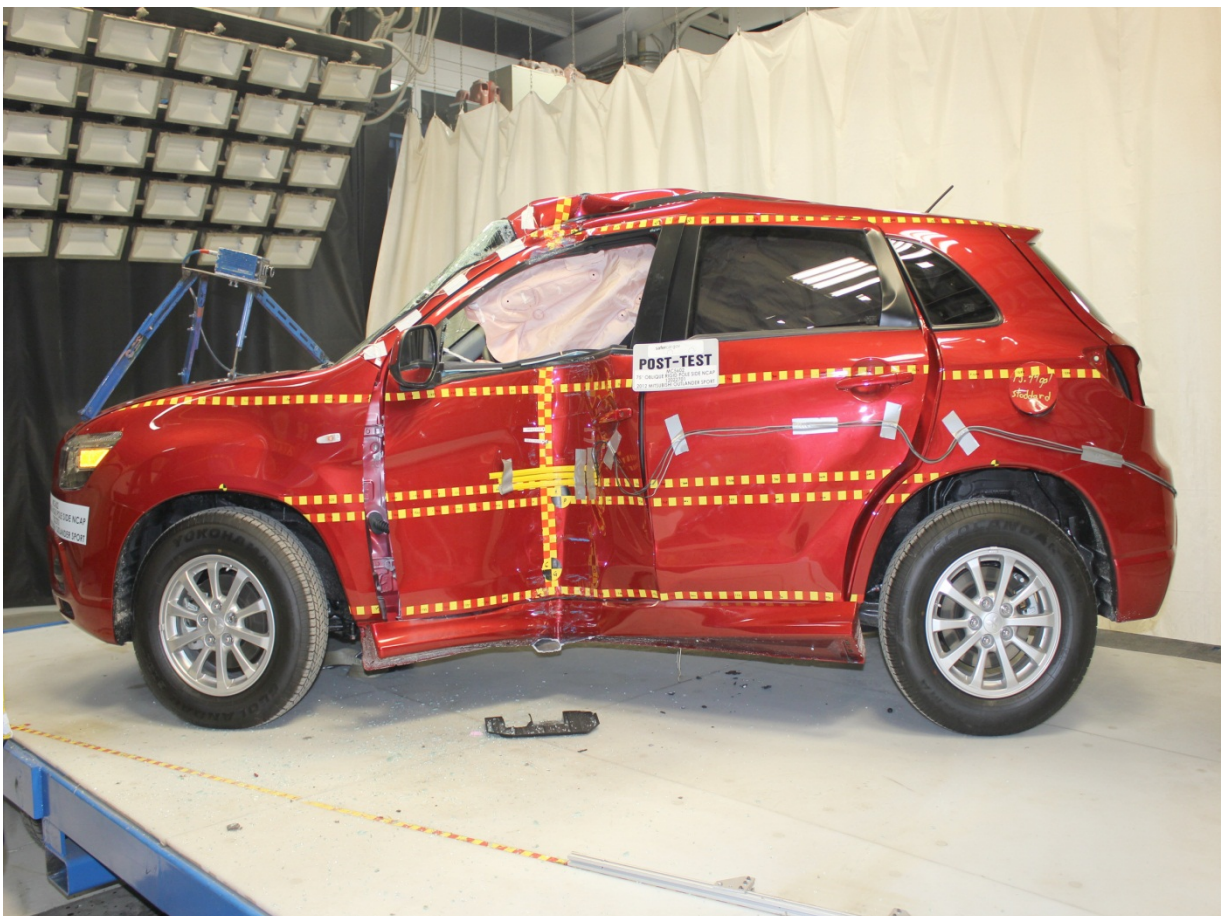
Post-Test Left Side View of Test Vehicle
