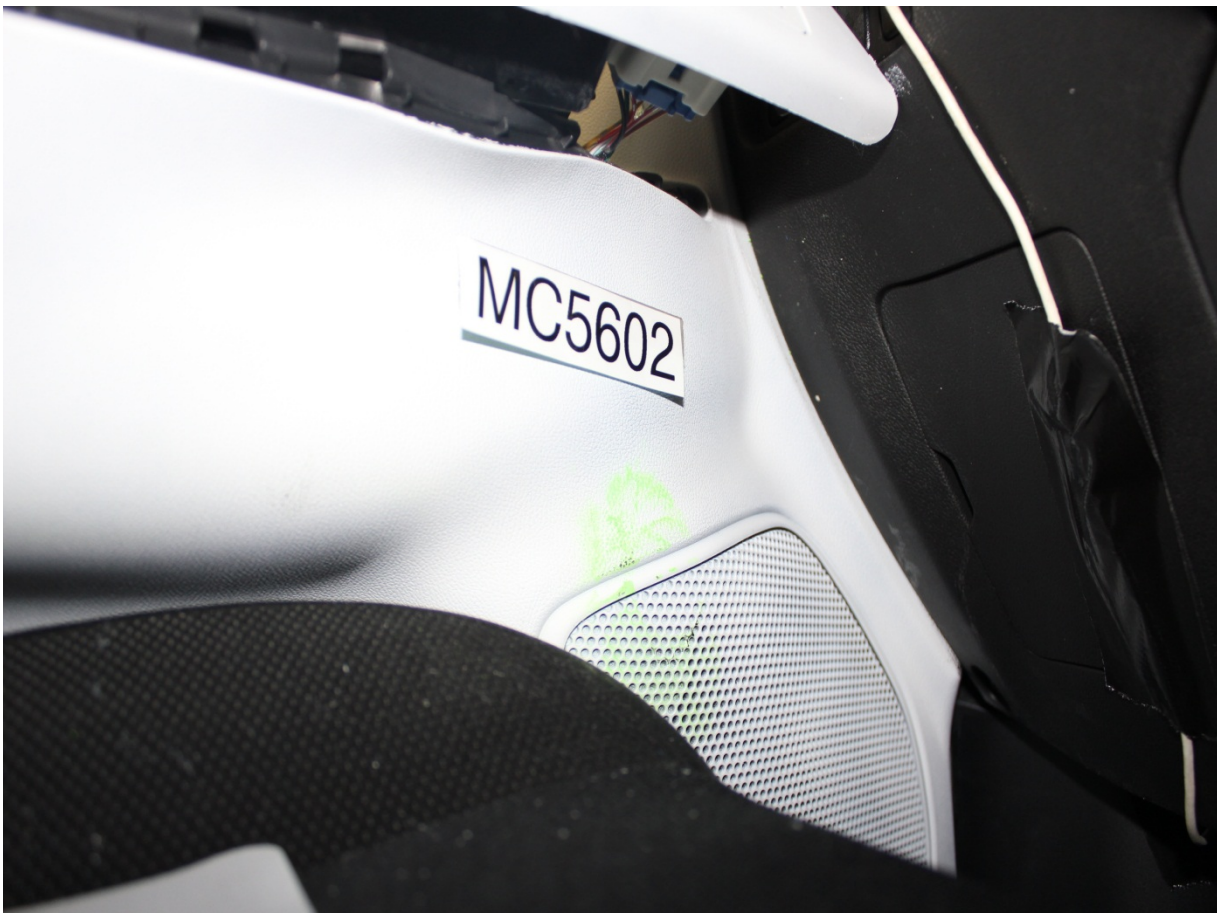
Post-Test Dummy Knee Contact with Vehicle Interior View
