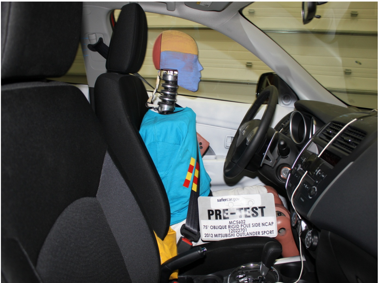
Pre-Test Right Side View of Dummy and Front Seat of Occupant Compartment
