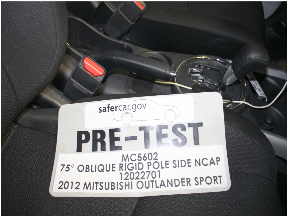
Pre-Test View of Disengaged Parking Brake
