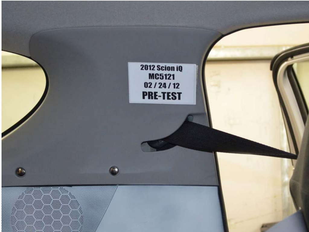
FIGURE 33. Pre-Test View of Belt Anchorage for Dummy
