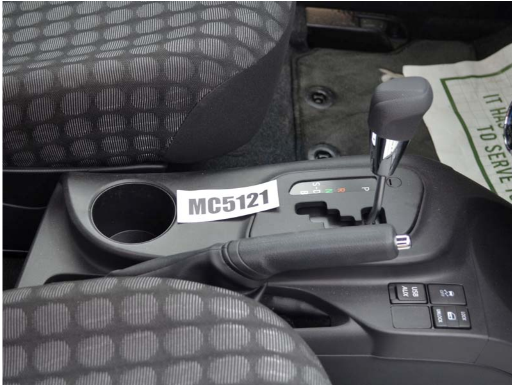
FIGURE 35. View of Disengaged Parking Brake
