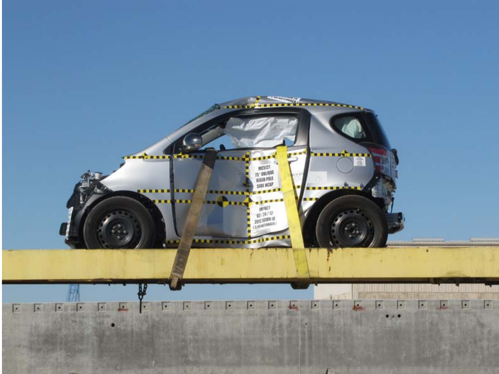
FIGURE 62. FMVSS No. 301-305 Rollover 0 Degrees
