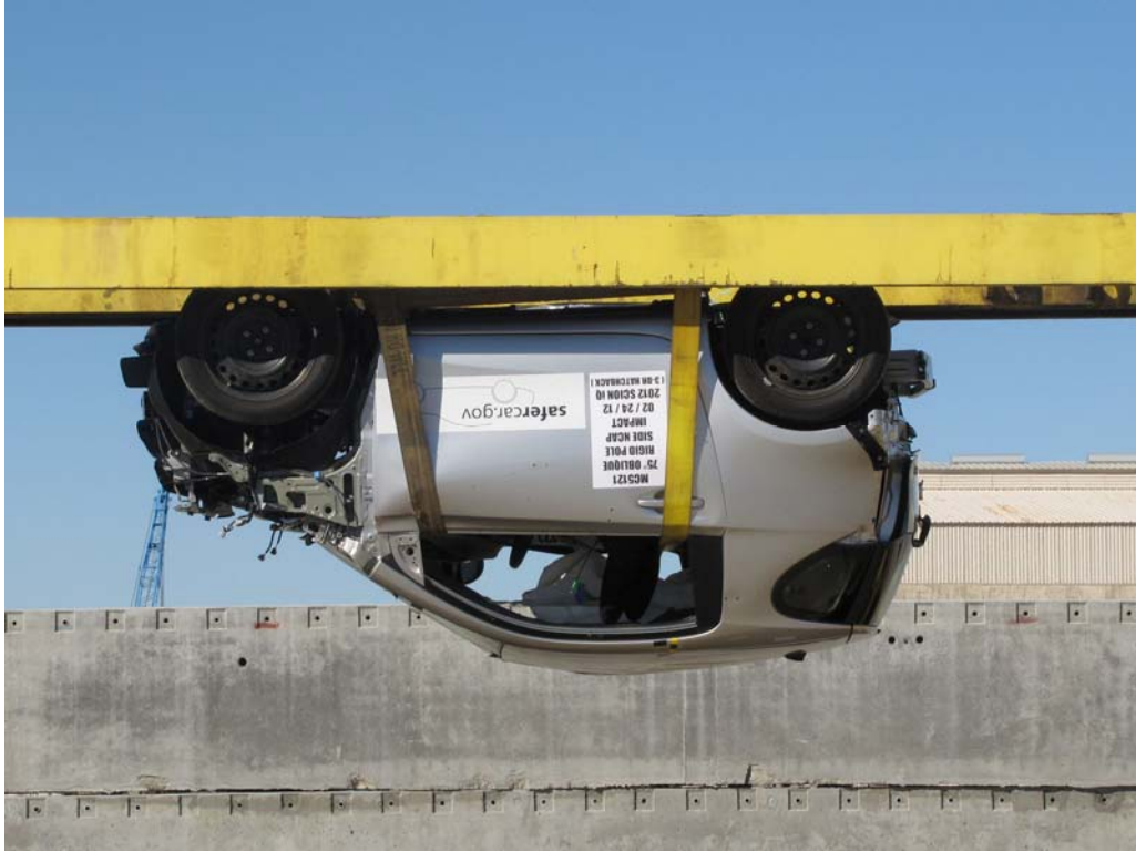
FIGURE 64. FMVSS No. 301-305 Rollover 180 Degrees
