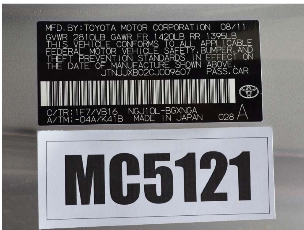
FIGURE 54. Close-Up View of Vehicle's Certification Label
