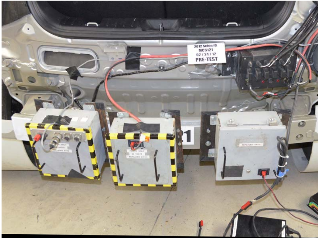
FIGURE 60. Pre-Test Ballast View
