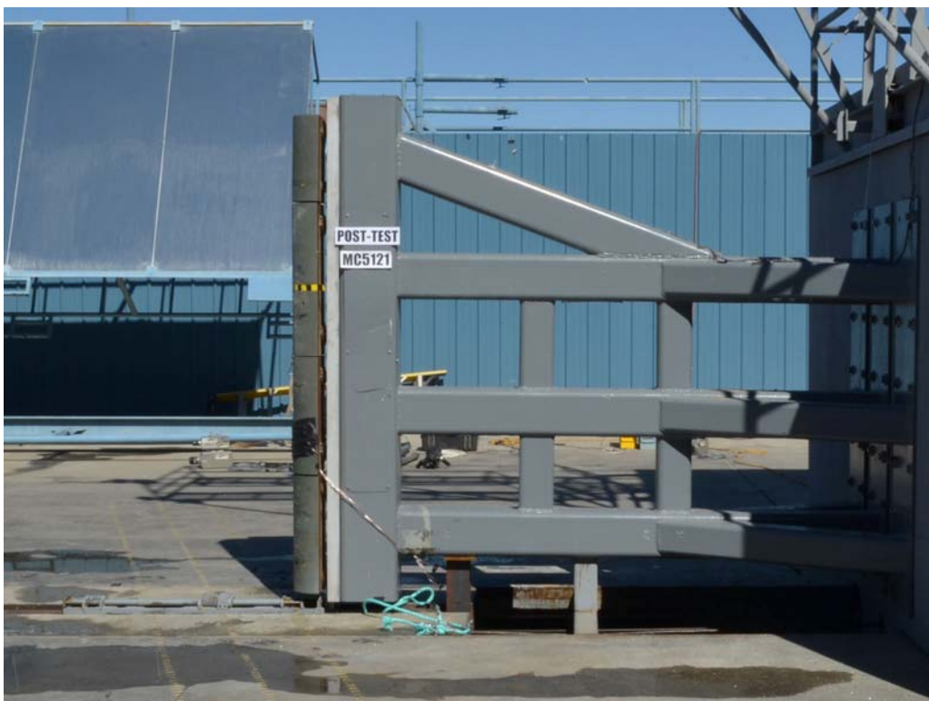
FIGURE 59. Post-Test Pole Barrier Side View
