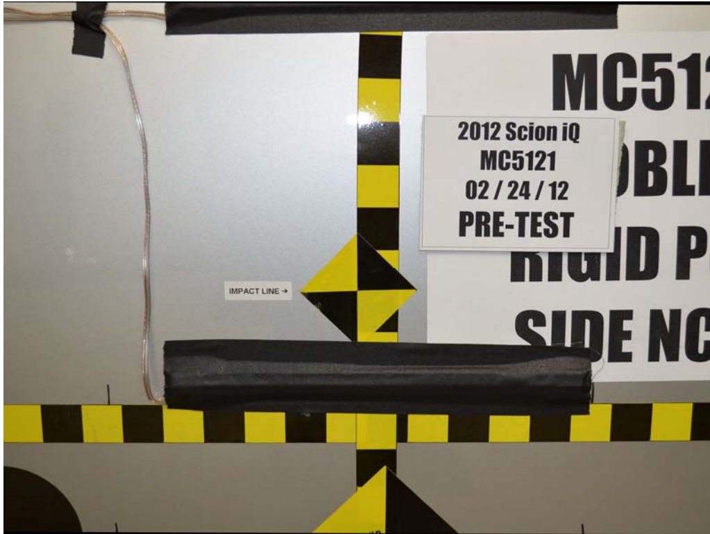
FIGURE 19. Pre-Test Close-Up View of Impact Point Target
