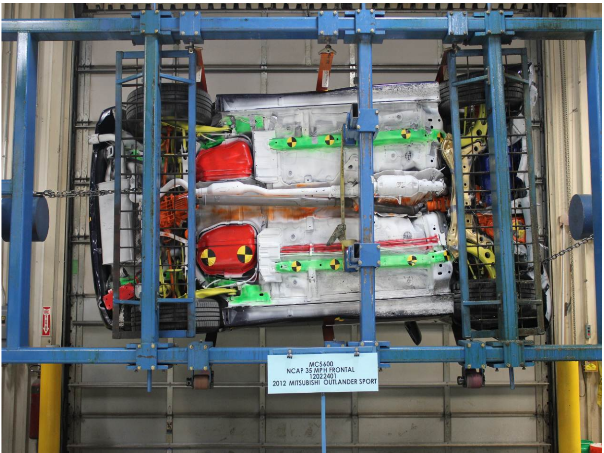
Vehicle at 90 Degrees on Static Rollover Device
