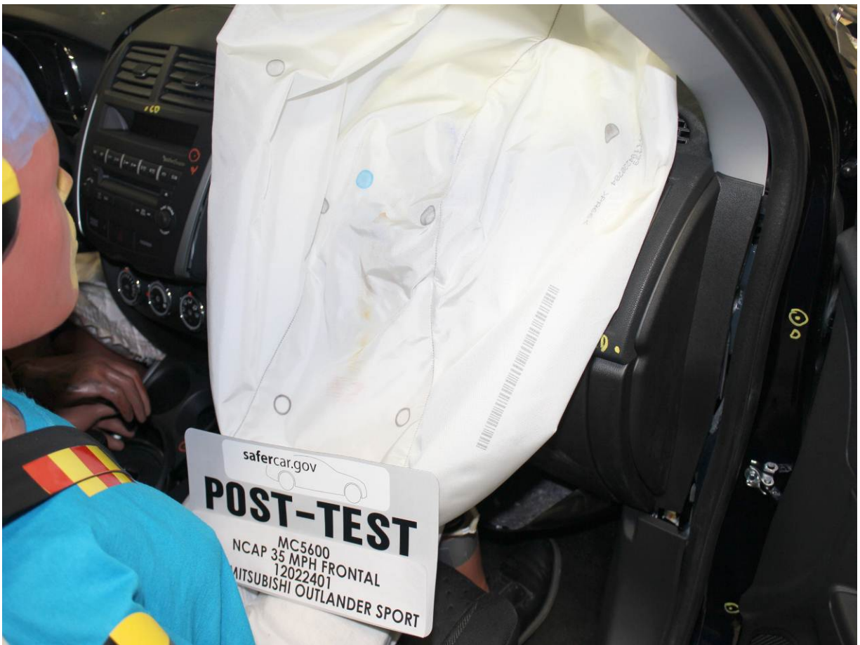
Post-Test Passenger Dummy Contact with Airbag
