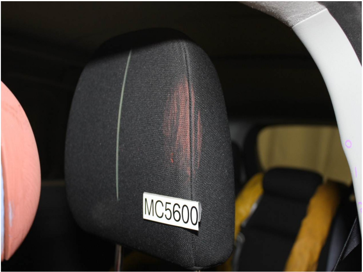
Post-Test Driver Dummy Contact with Headrest
