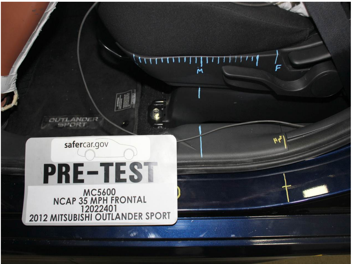
Pre-Test Driver's Seat Fore-Aft Markings
