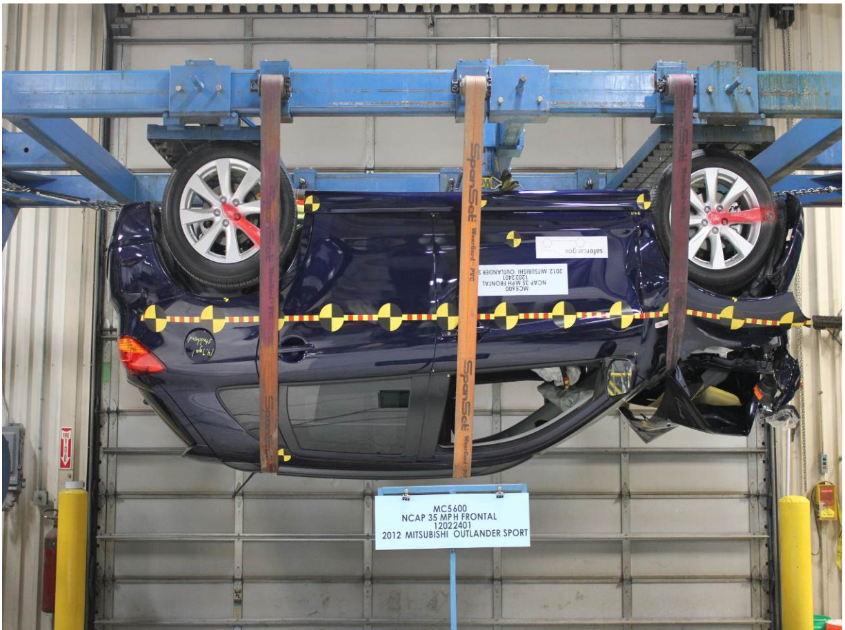
Vehicle at 180 Degrees on Static Rollover Device
