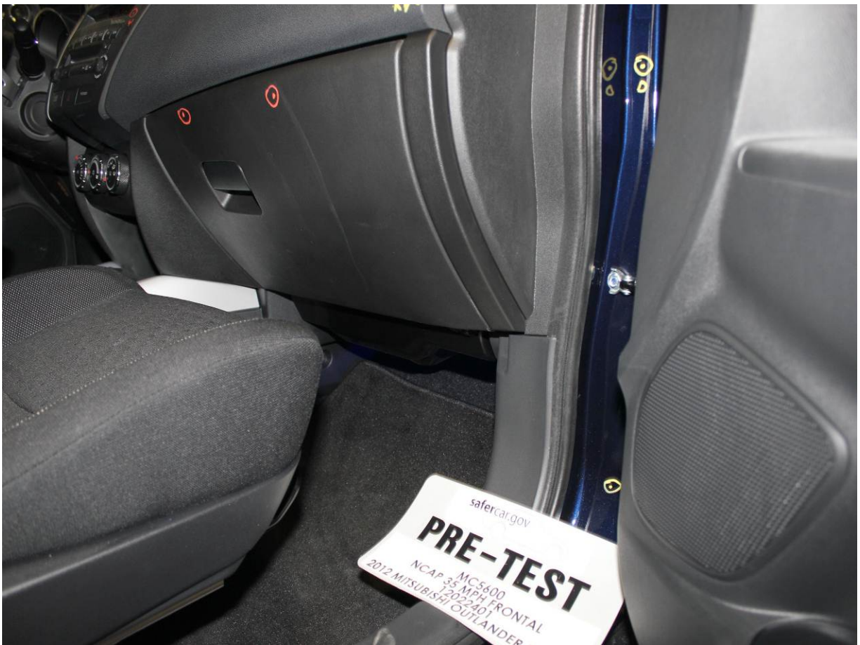
Pre-Test Passenger's Side Knee Bolster (without dummy)
