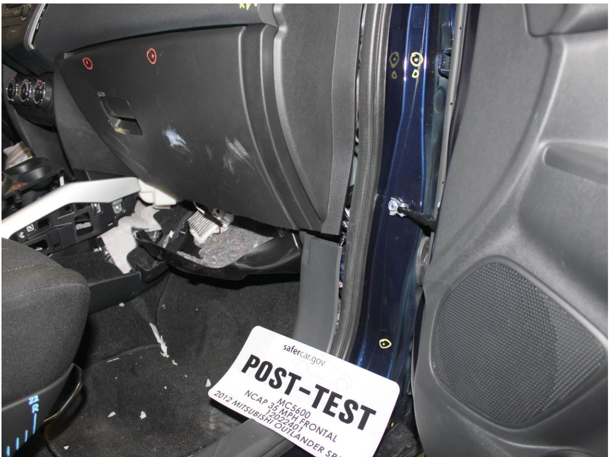
Post-Test Passenger's Side Knee Bolster (without dummy)
