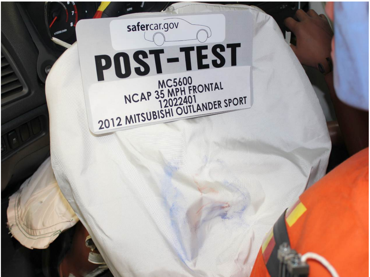
Post-Test Driver Dummy Contact with Airbag
