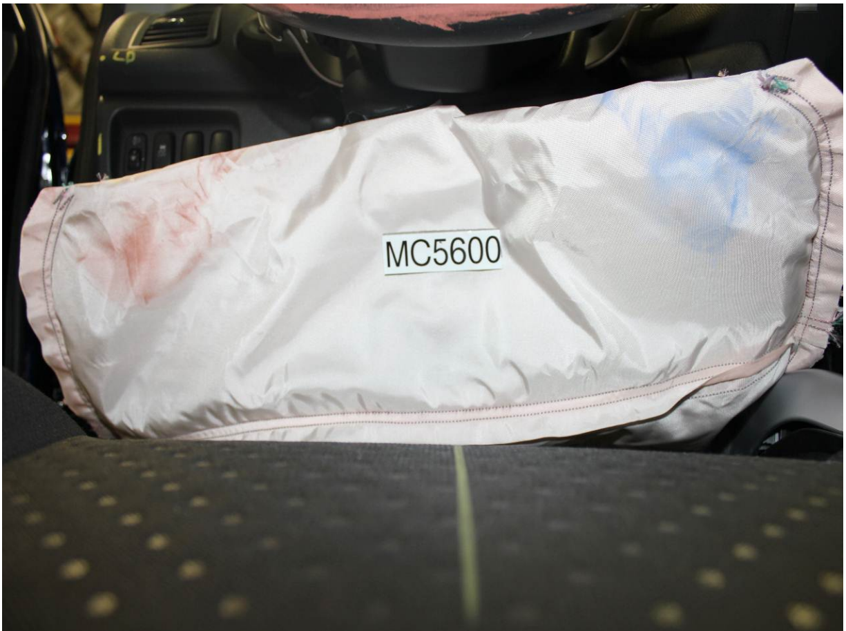
Post-Test Driver Dummy Contact with Knee Airbag
