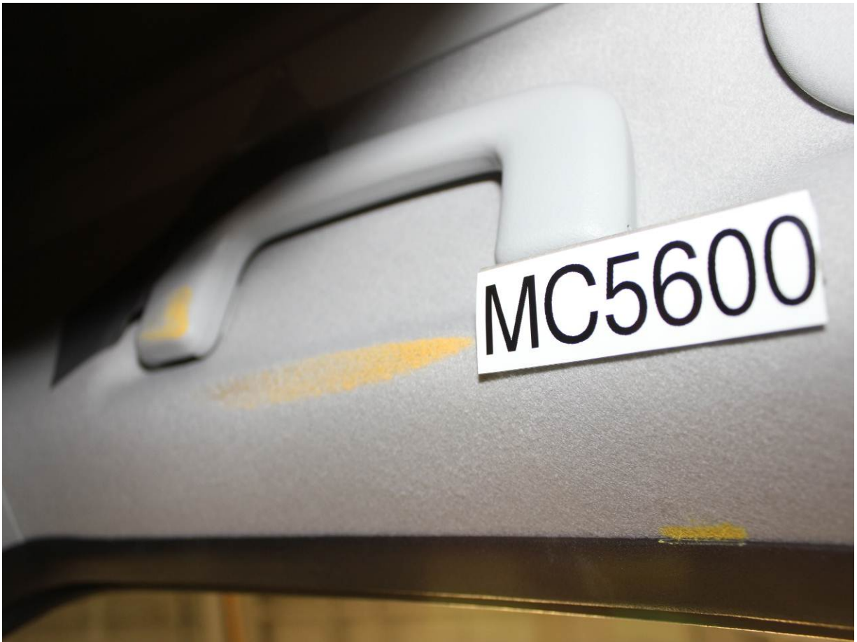
Post-Test Passenger Dummy Contact with Side Header
