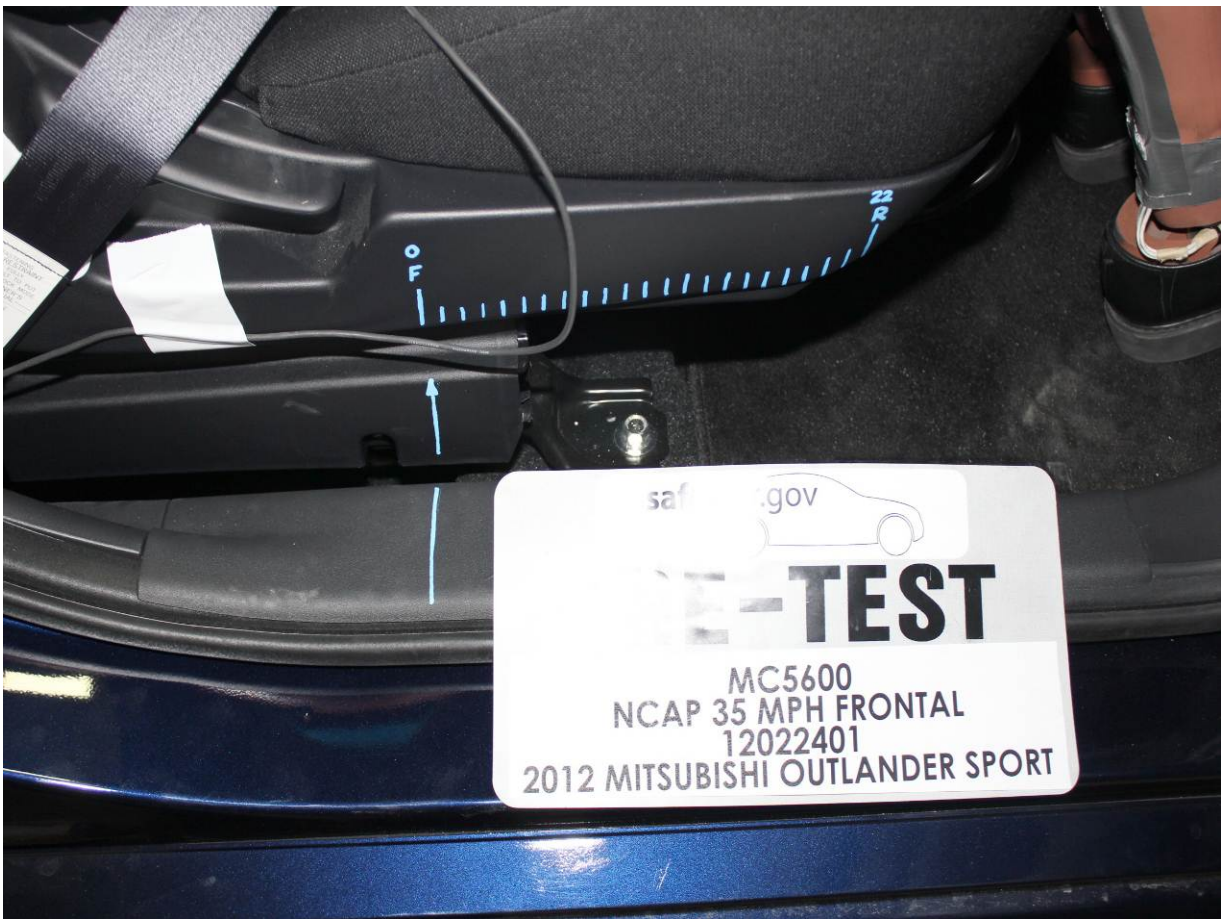
Pre-Test Passenger's Seat Fore-Aft Markings
