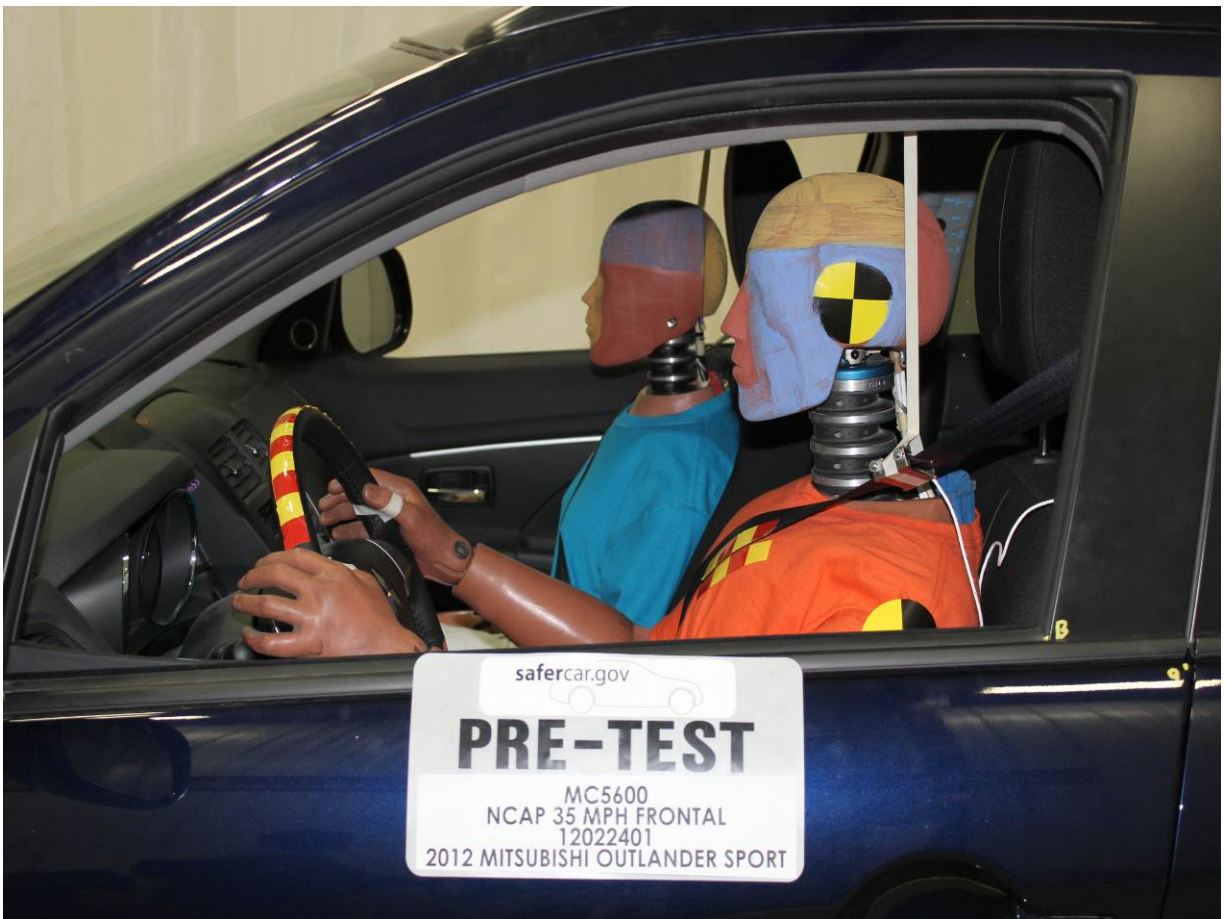
Pre-Test Driver Dummy Window View
