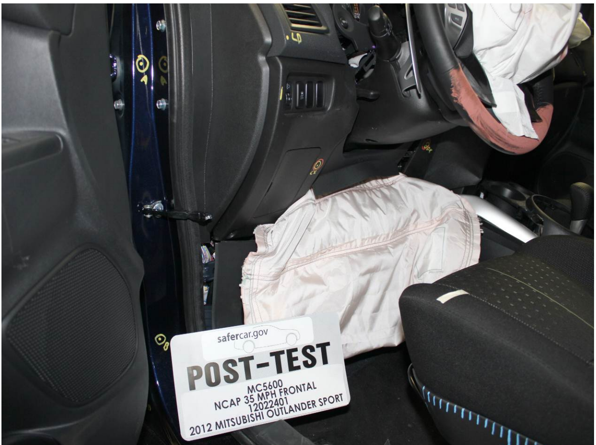
Post-Test Driver's Side Knee Bolster (without dummy)
