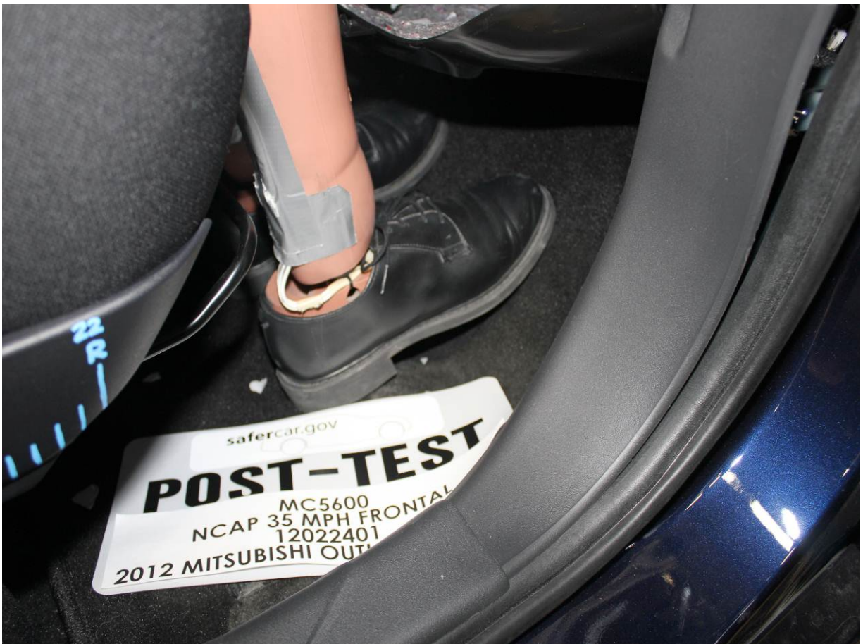
Post-Test Passenger Dummy Feet
