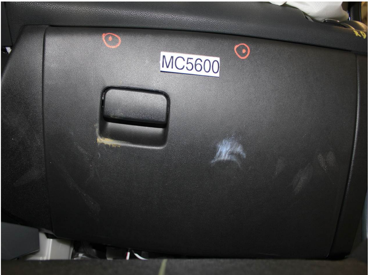
Post-Test Passenger Dummy Contact with Knee Bolster
