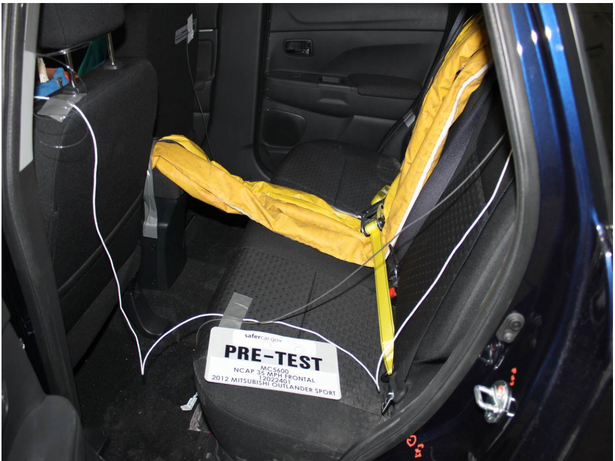
Pre-Test Dummy Cable Routing
