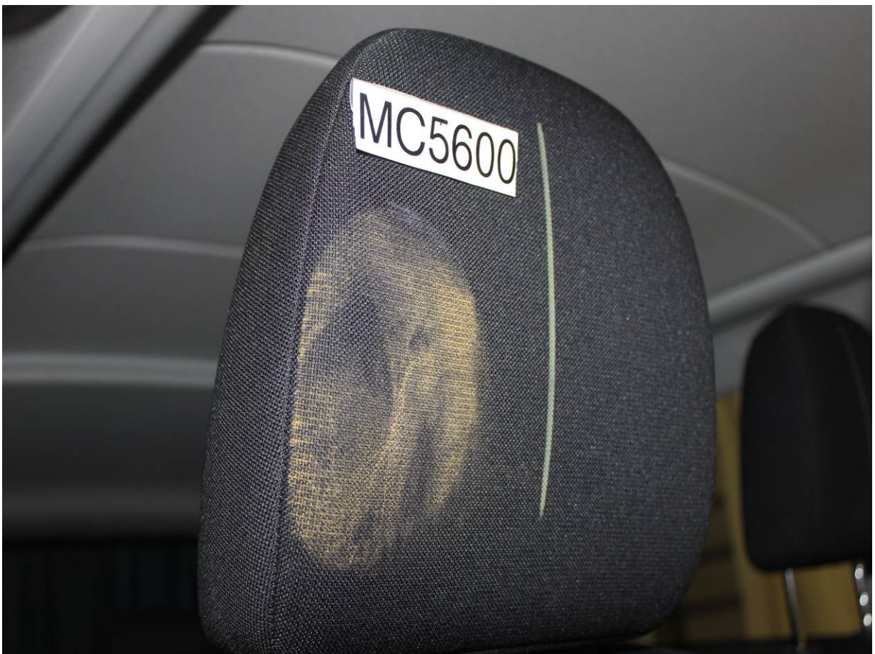
Post-Test Passenger Dummy Contact with Headrest
