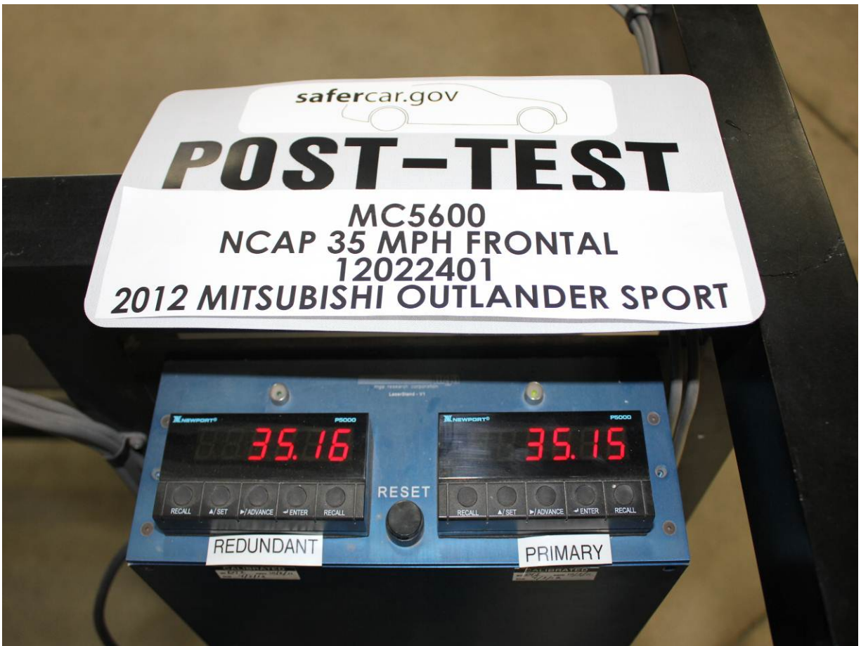
Post-Test Speed Trap Read-Out
