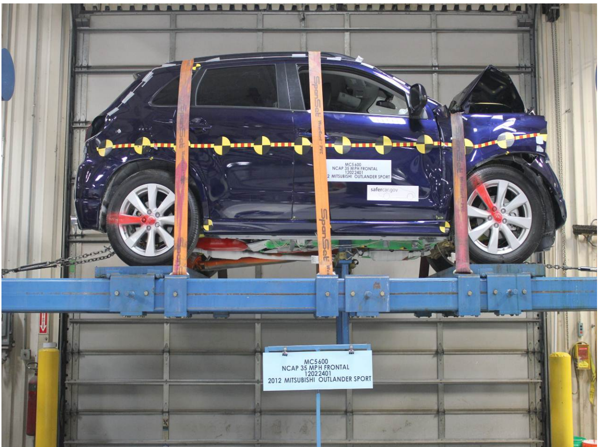
Vehicle at 360 Degrees on Static Rollover Device
