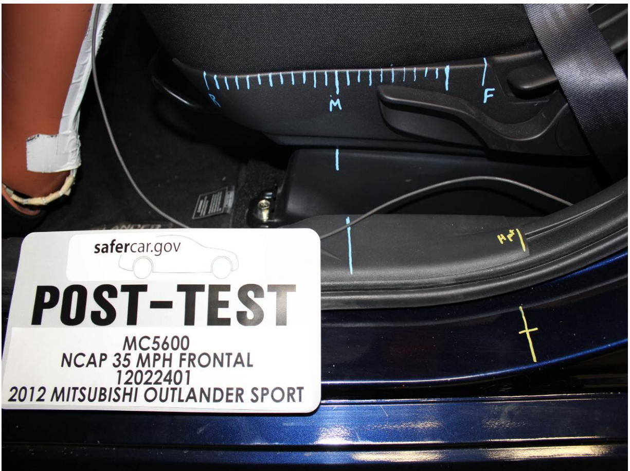
Post-Test Driver's Seat Fore-Aft Markings
