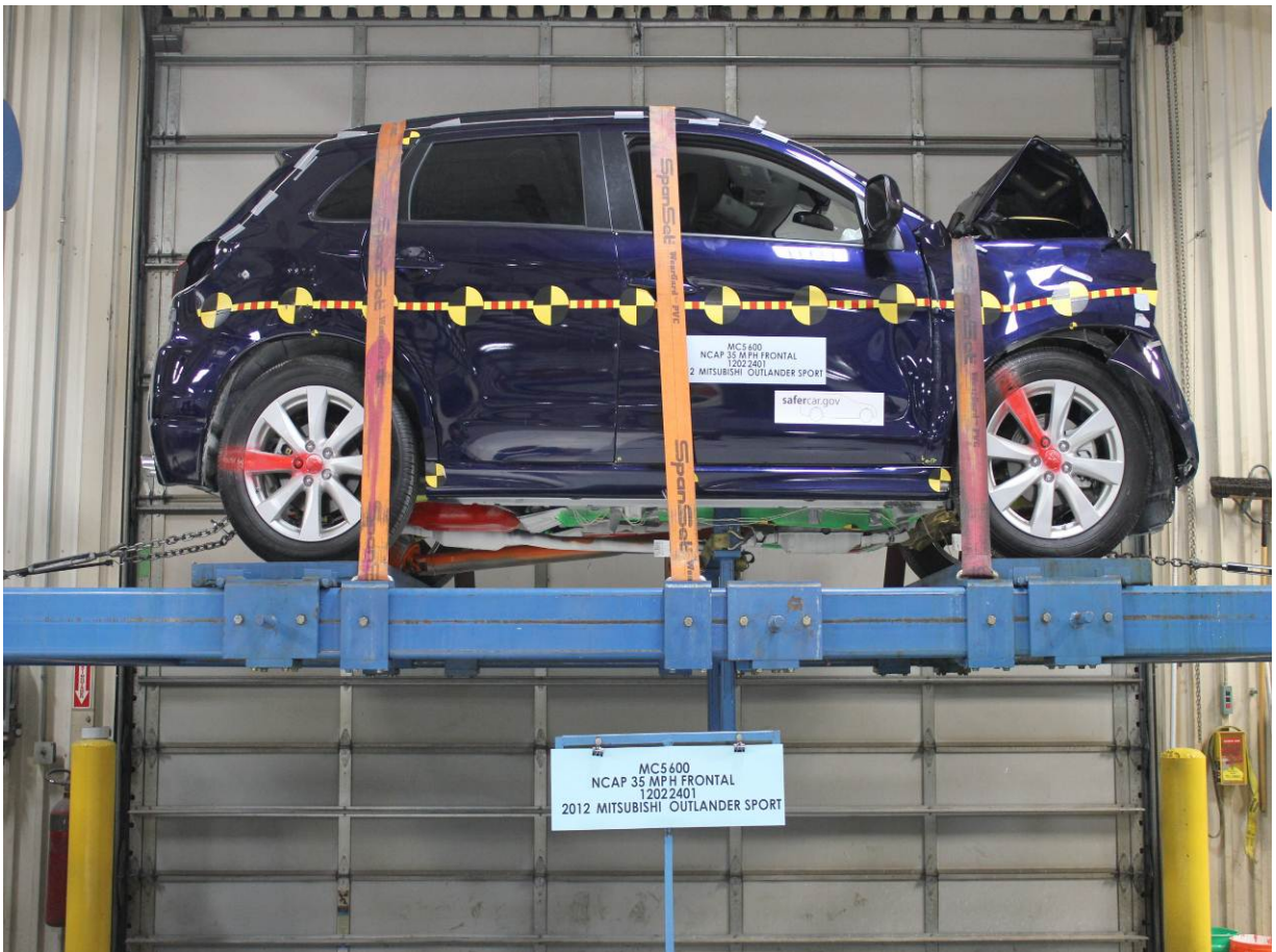
Vehicle at 0 Degrees on Static Rollover Device
