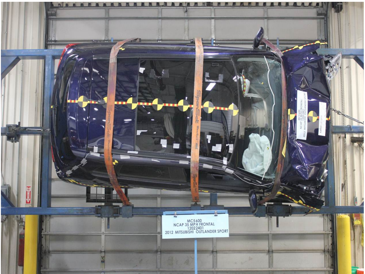
Vehicle at 270 Degrees on Static Rollover Device
