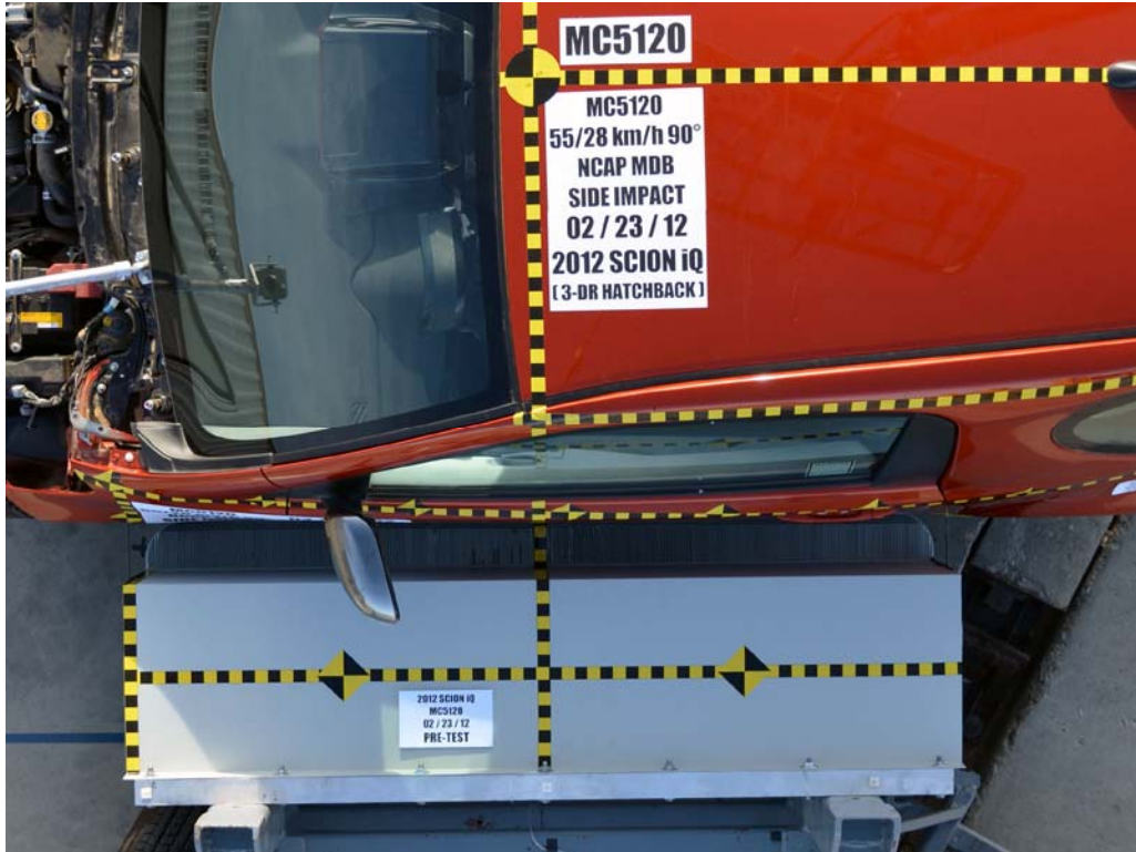
FIGURE 15. Pre-Test Overhead View of Test Area
