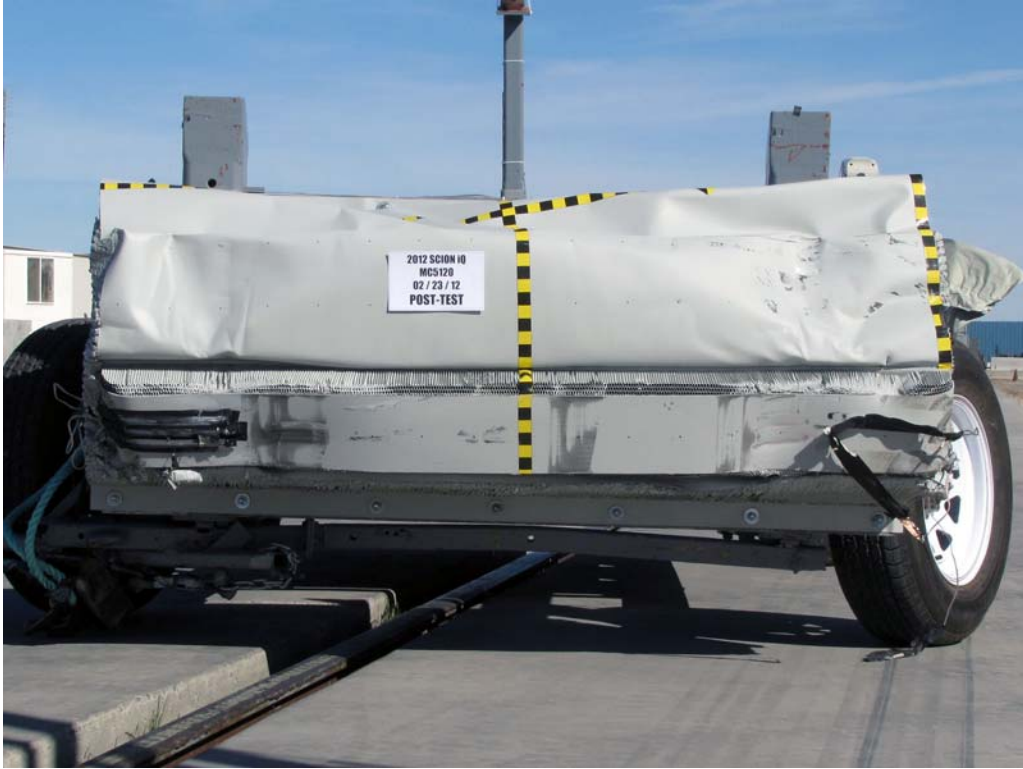
FIGURE 83. Post-Test Front View of MDB Impactor Face
