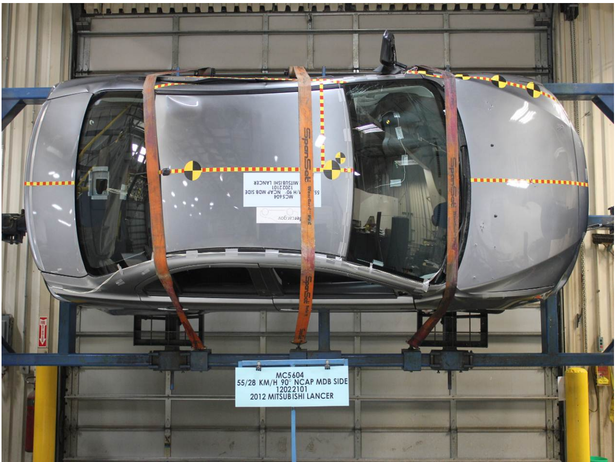
FMVSS No. 301 Static Rollover 270 Degrees
