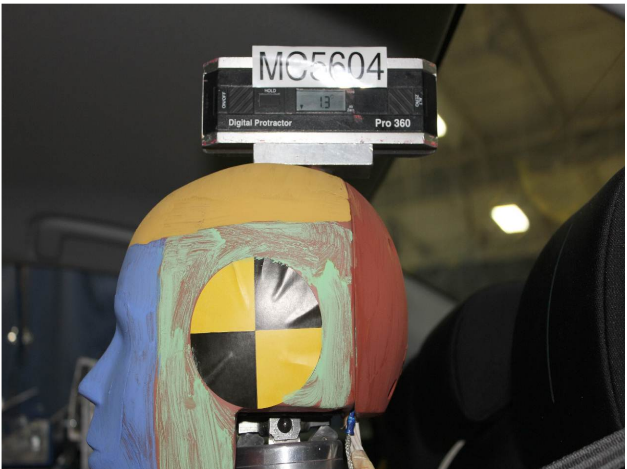
Pre-Test View of Rear Passenger Dummy's Head Showing Dummy's Head is Level
