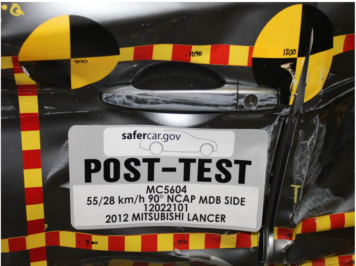
Post-Test Left Front Door Latch Close-Up
