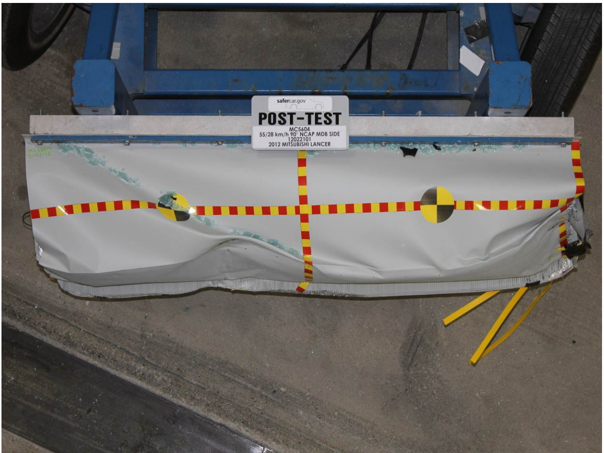
Post-Test Top View of MDB Impactor Face
