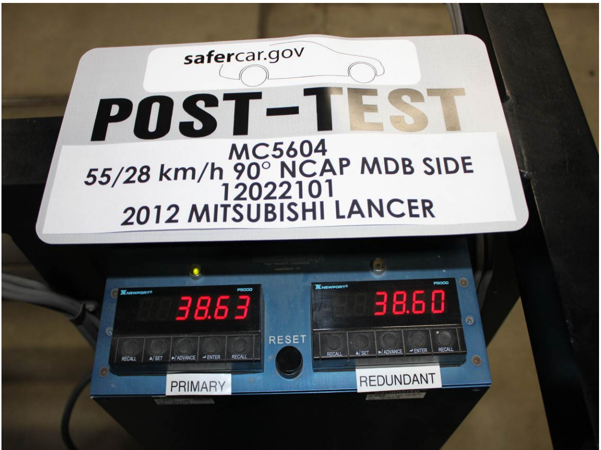
Post-Test Primary and Redundant Speed Trap Read-Out
