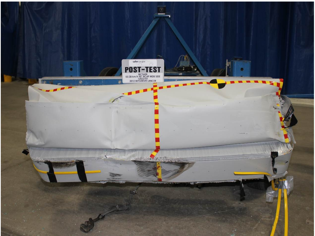
Post-Test Front View of MDB Impactor Face
