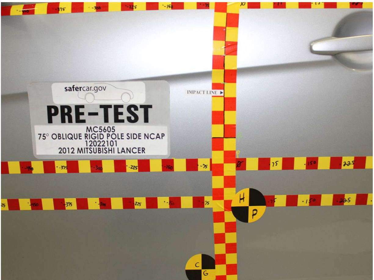
Pre-Test Close-Up View of Impact Point Target
