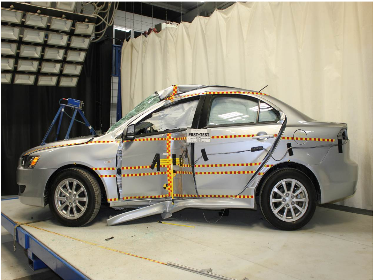
Post-Test Left Side View of Test Vehicle
