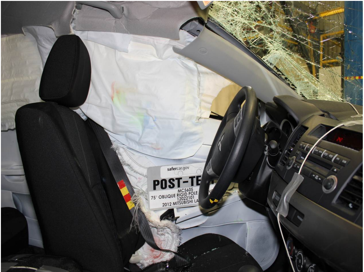
Post-Test Inner Door Panel View Showing Dummy Contact Location
