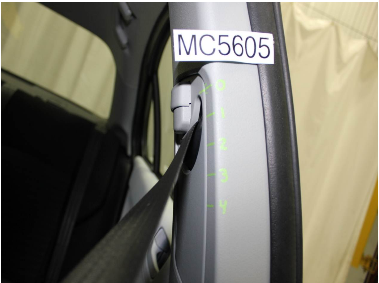
Pre-Test View of Belt Anchorage for Dummy
