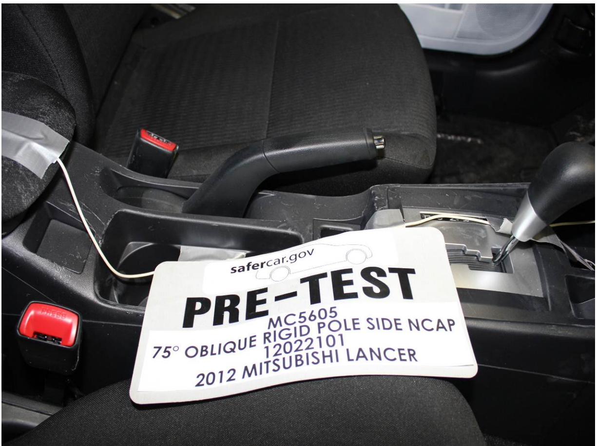
Pre-Test View of Disengaged Parking Brake
