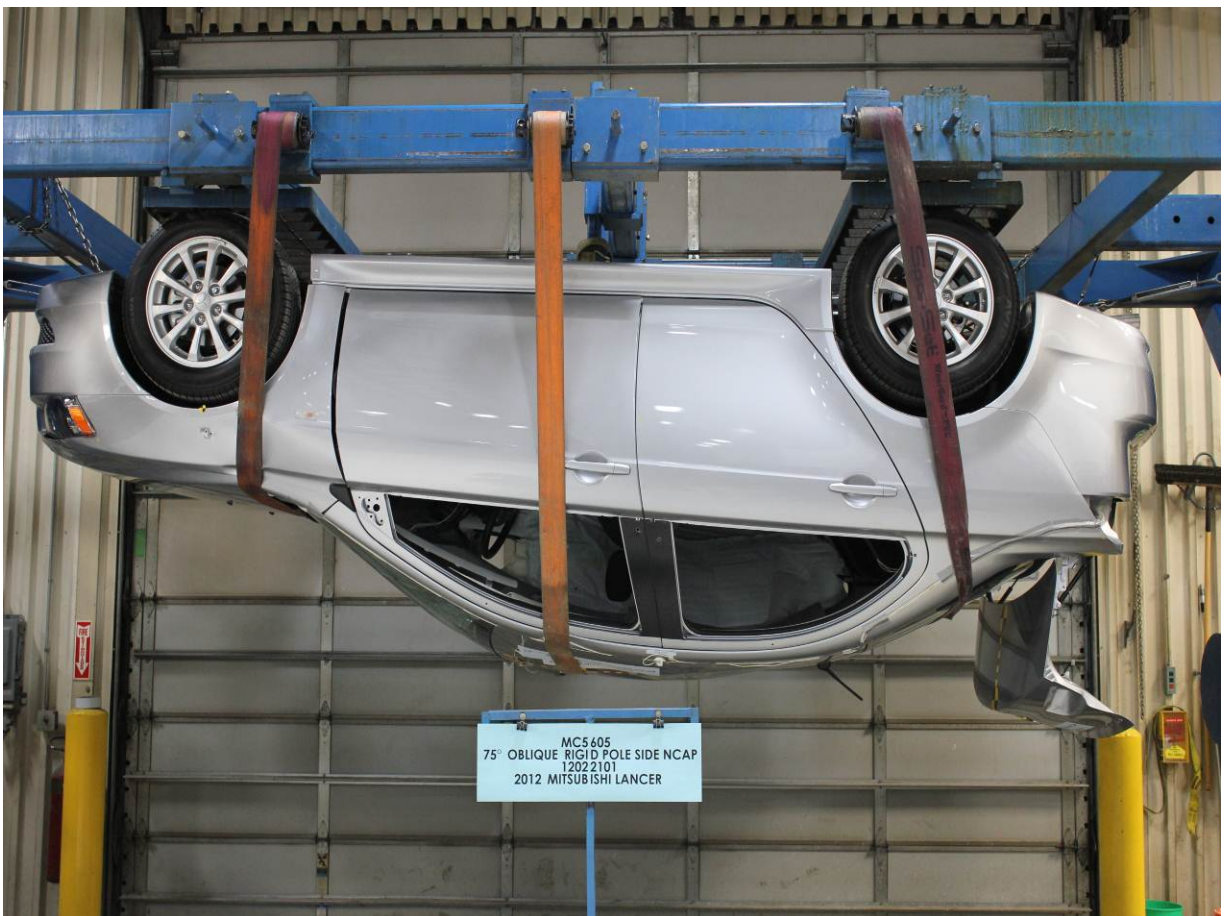
FMVSS No. 301 Static Rollover 180 Degrees
