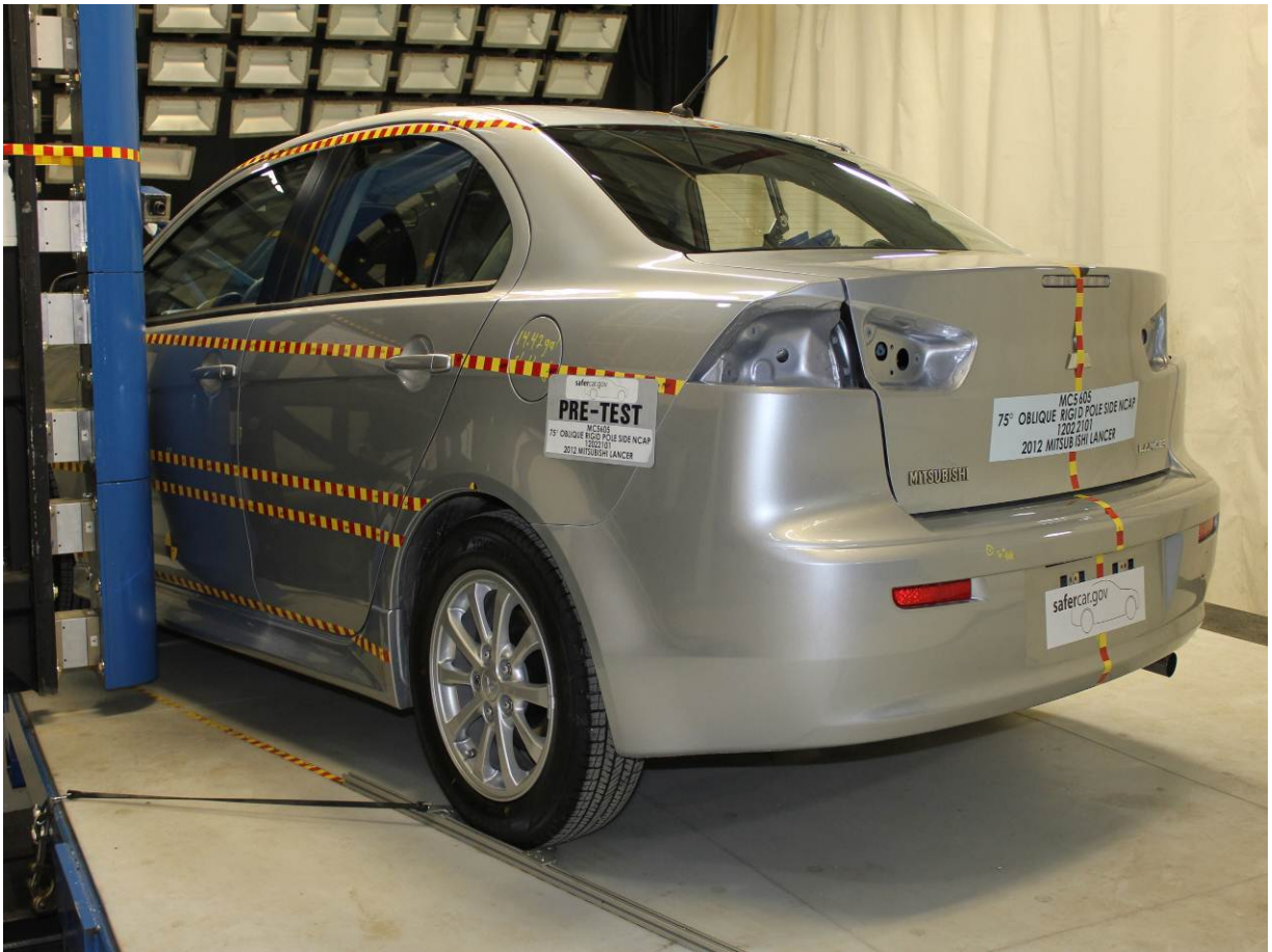
Pre-Test Right Side View of Pole Positioned Against Side of Vehicle
