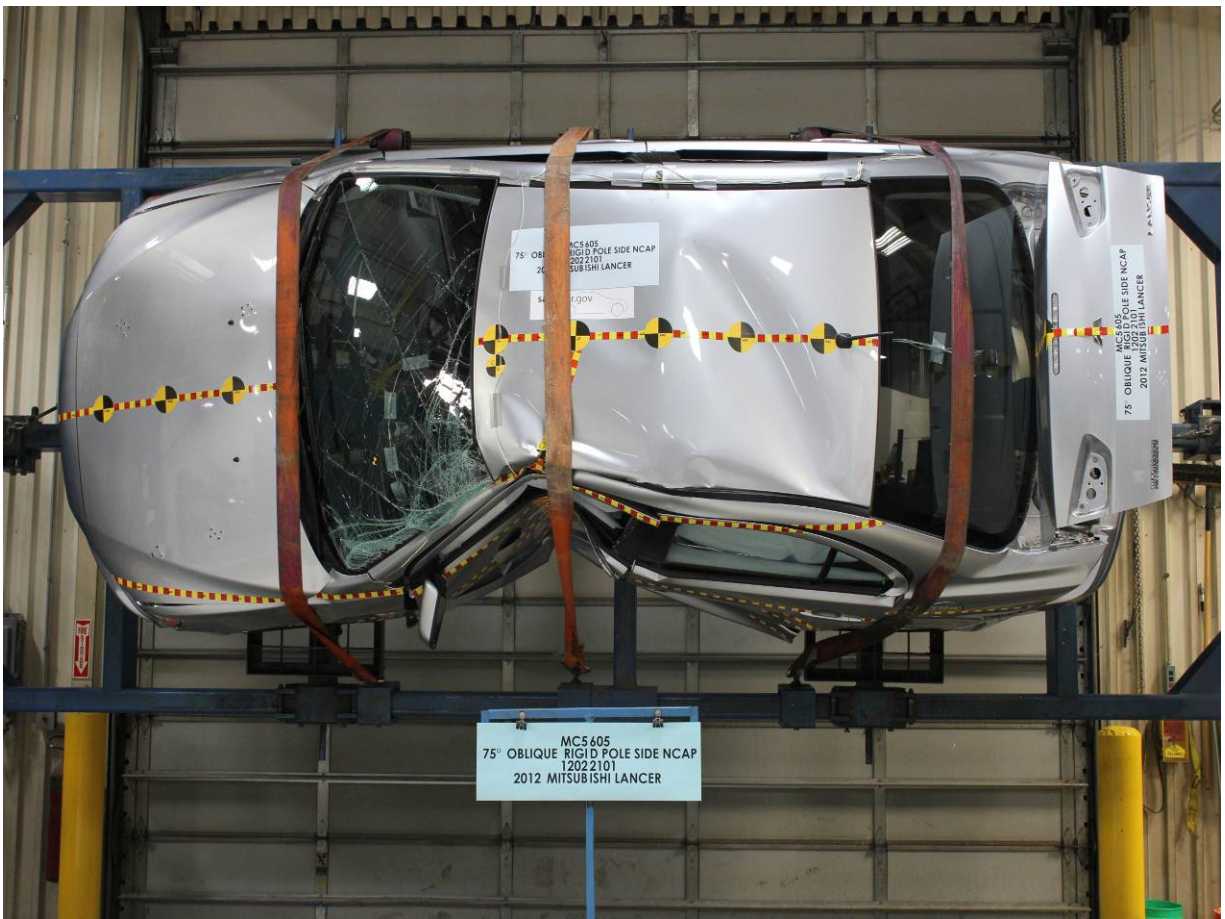
FMVSS No. 301 Static Rollover 90 Degrees
