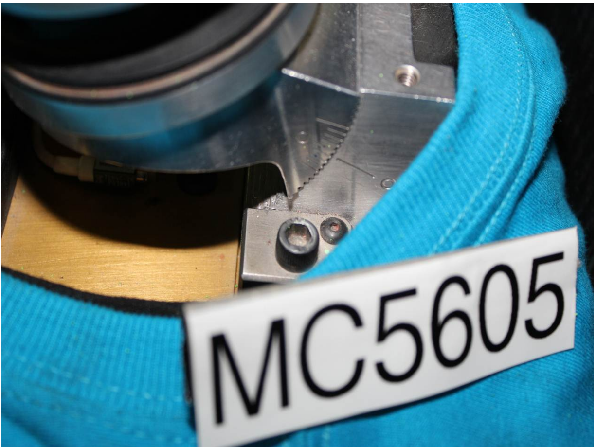
Pre-Test Left Side View of Dummy's Neck Showing Position of Adjustable Neck Bracket
