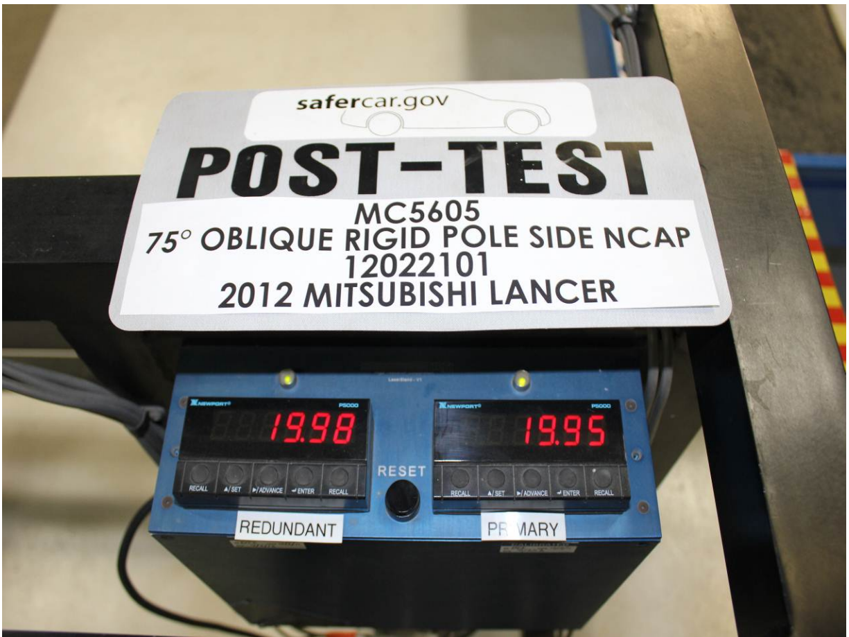
Post-Test Primary and Redundant Speed Trap Read-Out
