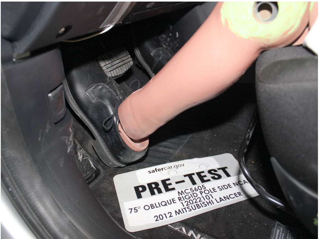
Pre-Test Placement of Dummy's Feet
