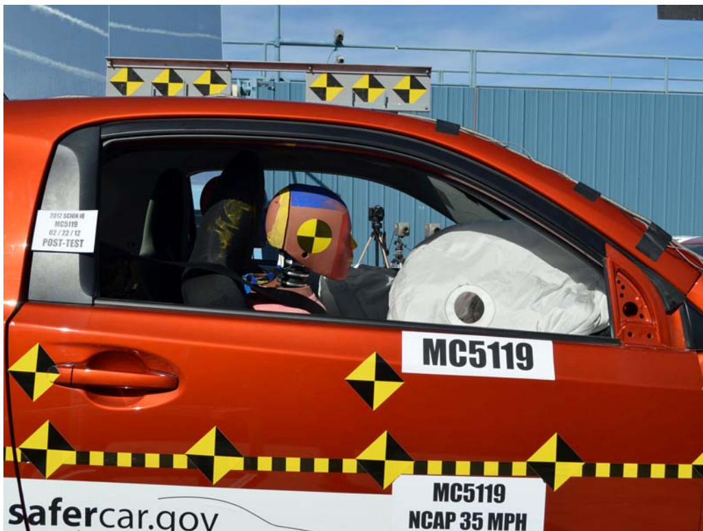
FIGURE 51. Post-Test Passenger Dummy Window View
