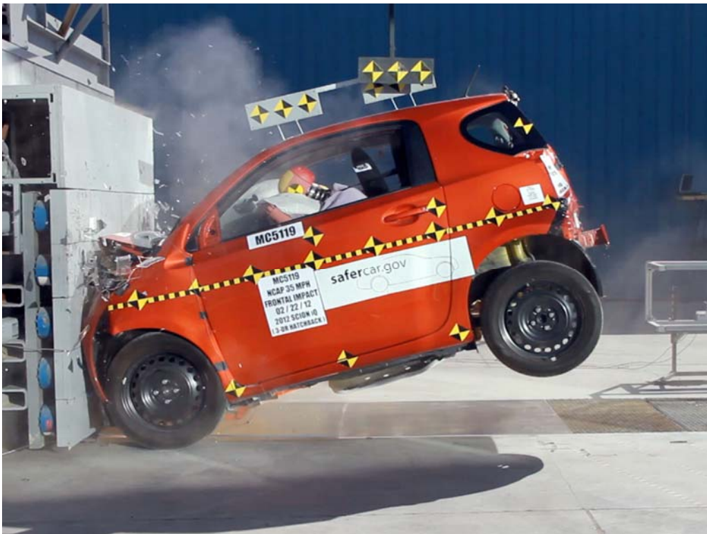
FIGURE 71. 2012 Scion iQ Frontal Impact Event
