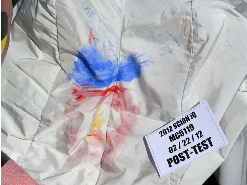
FIGURE 62. Post-Test Passenger Dummy Contact With Airbag
