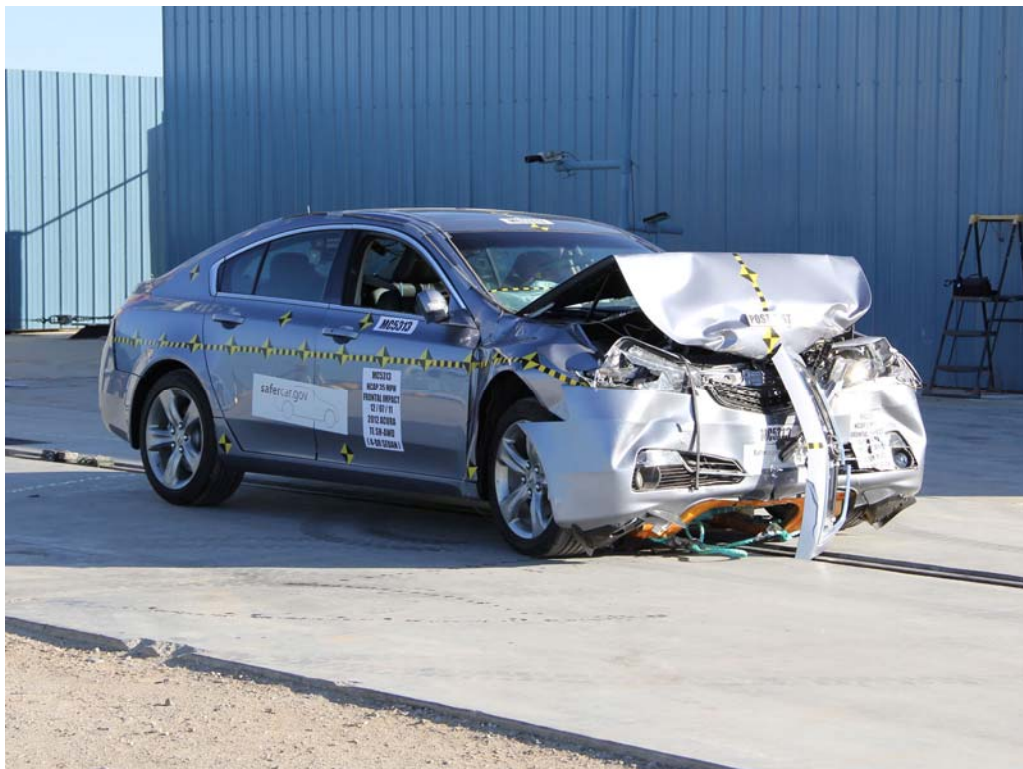
FIGURE 4. Post-Test Left Front 3/4 View of NCAP Frontal Impact Test
