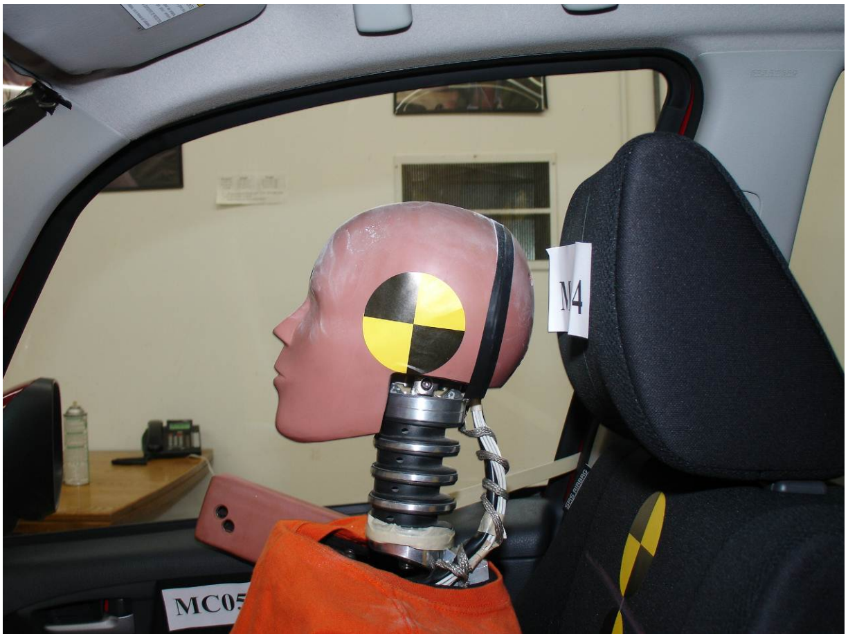
Pre-Test SID-IIs Dummy Left Side Closeup View
