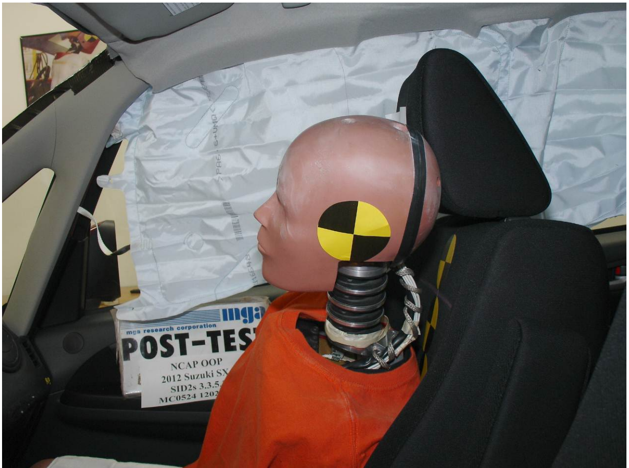
Post-Test SID-IIs Dummy Left Side Closeup View
