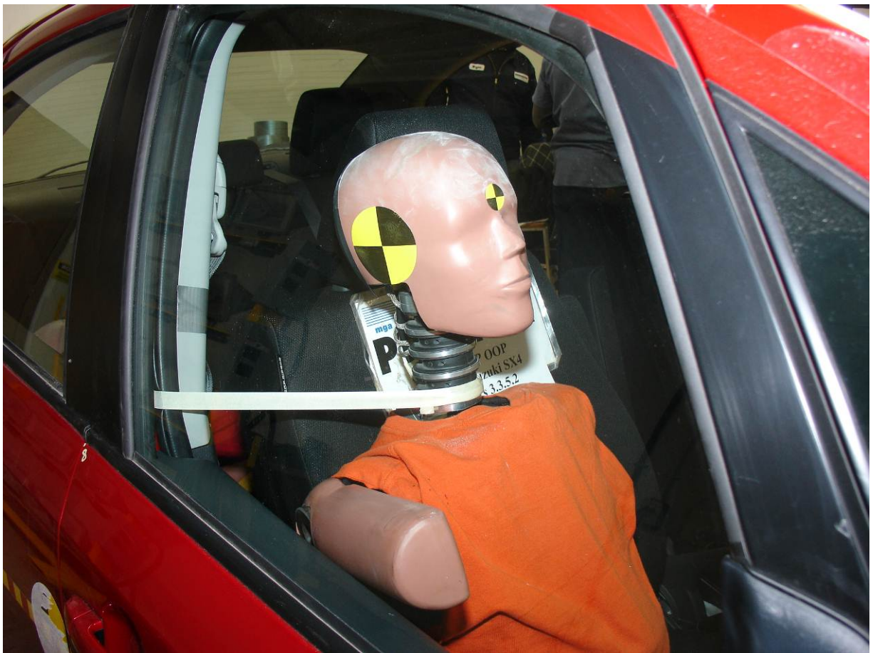
Pre-Test SID-IIs Dummy Right ¾ Front View
