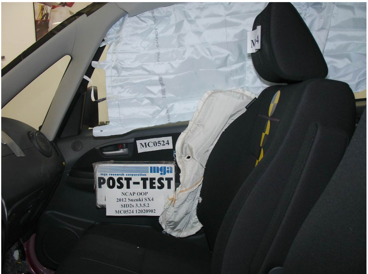
Post-Test Curtain Airbag Left View
