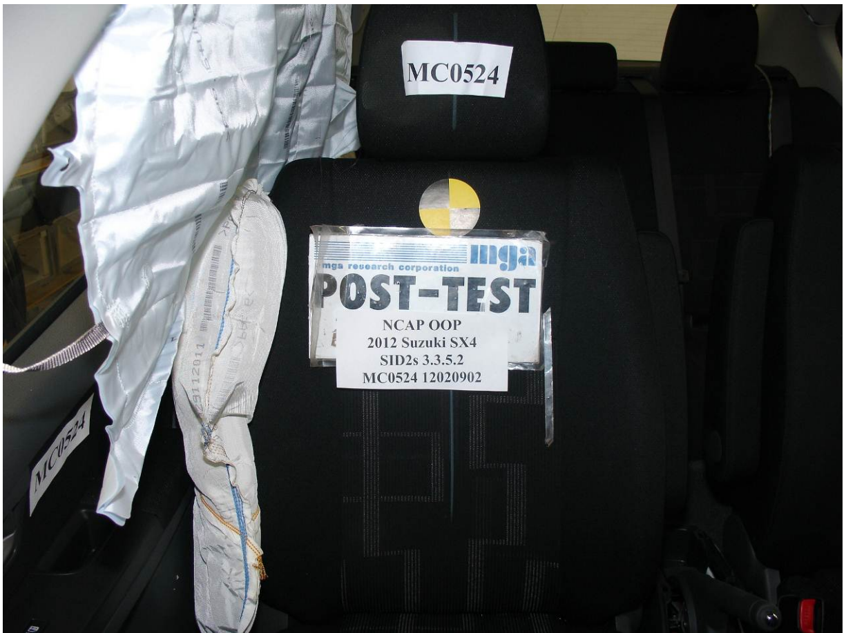
Post-Test Curtain Airbag Front View
