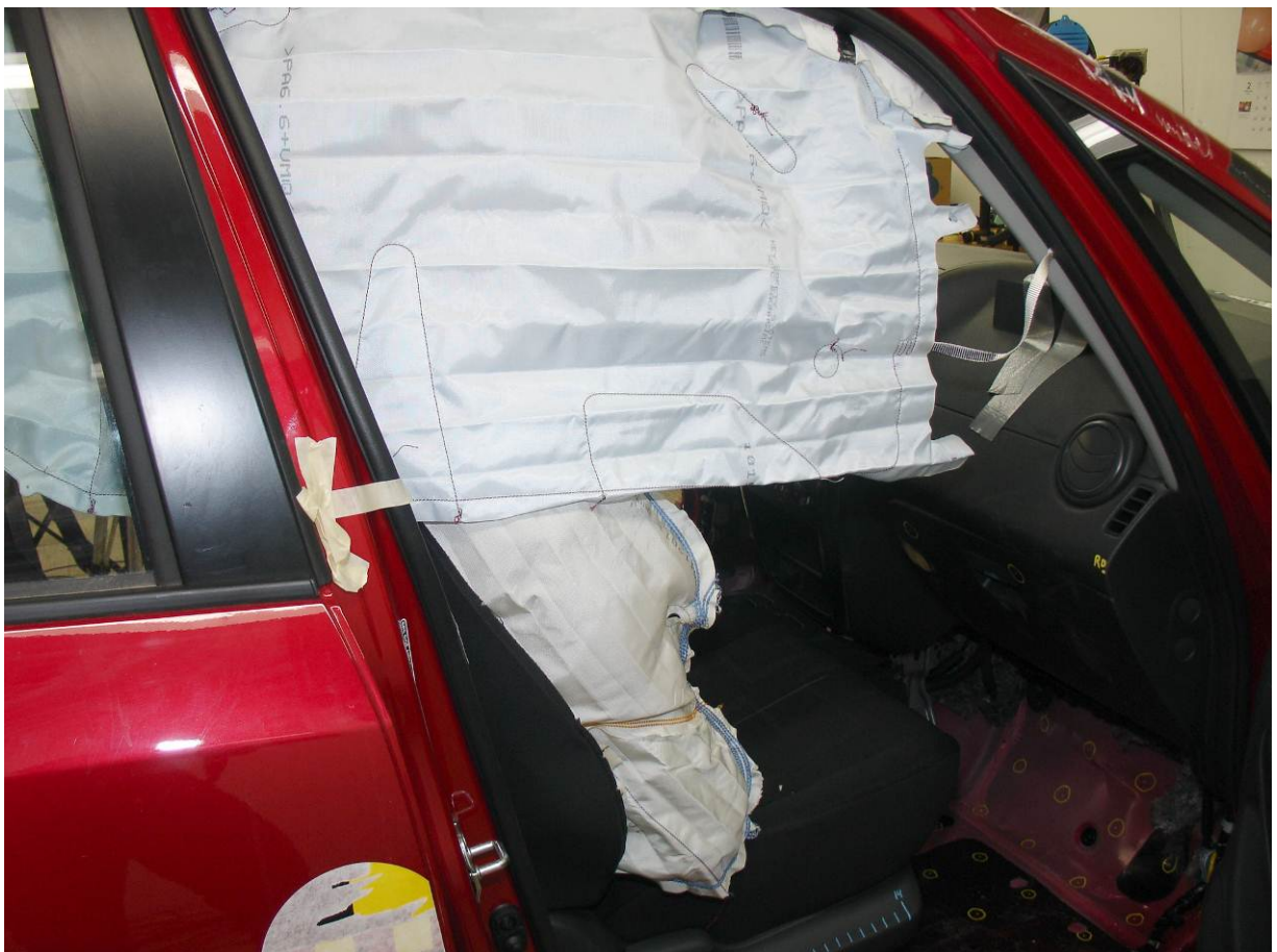
Post-Test Curtain Airbag Right View (Door Open)
