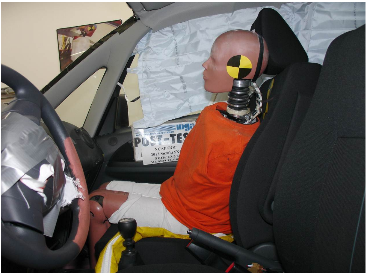
Post-Test SID-IIs Dummy Left Side View
