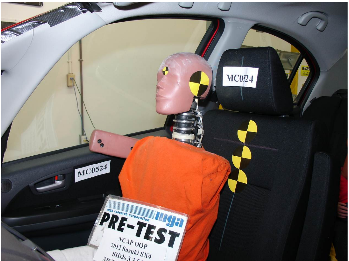
Pre-Test SID-IIs Dummy Left ¾ Front View
