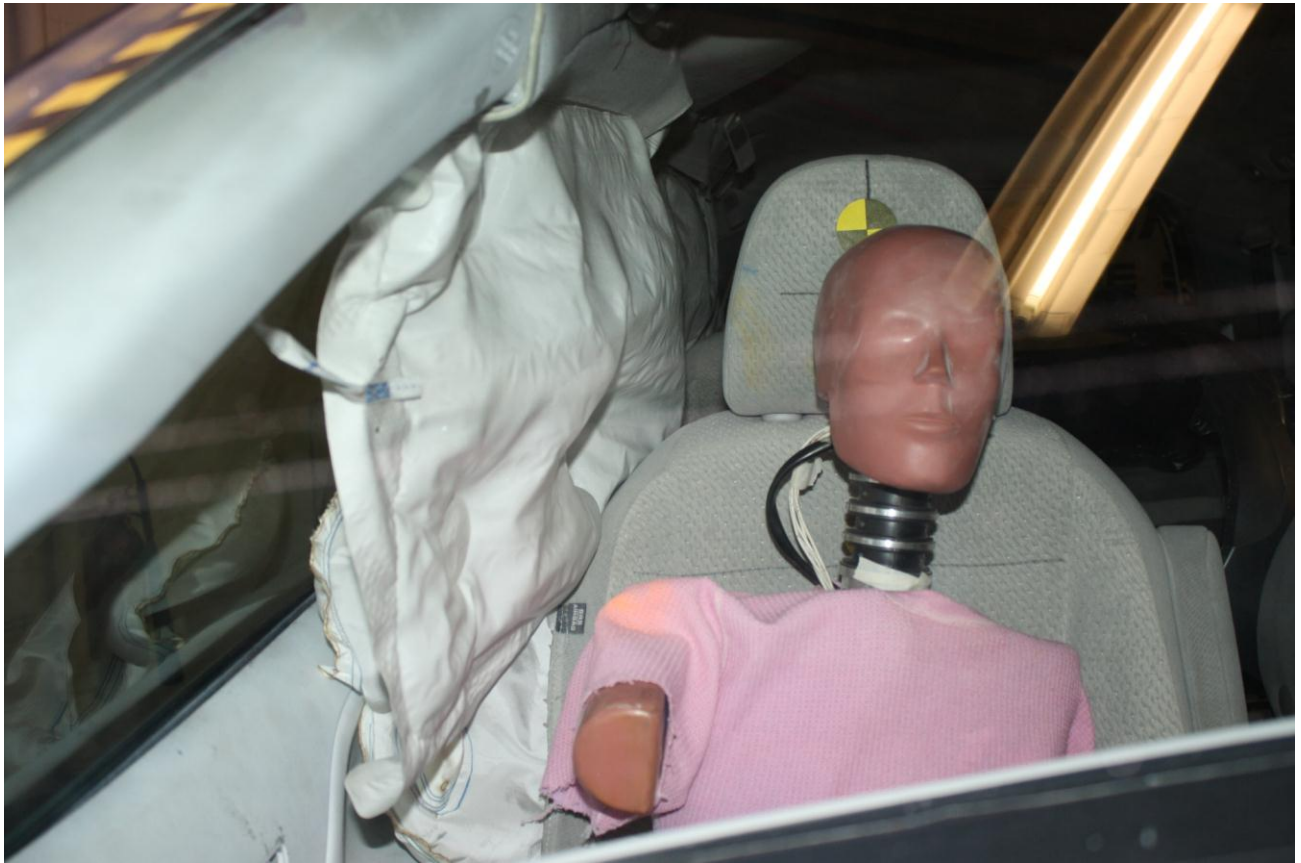
Figure A-19: Post-Test Curtain Airbag Front View
