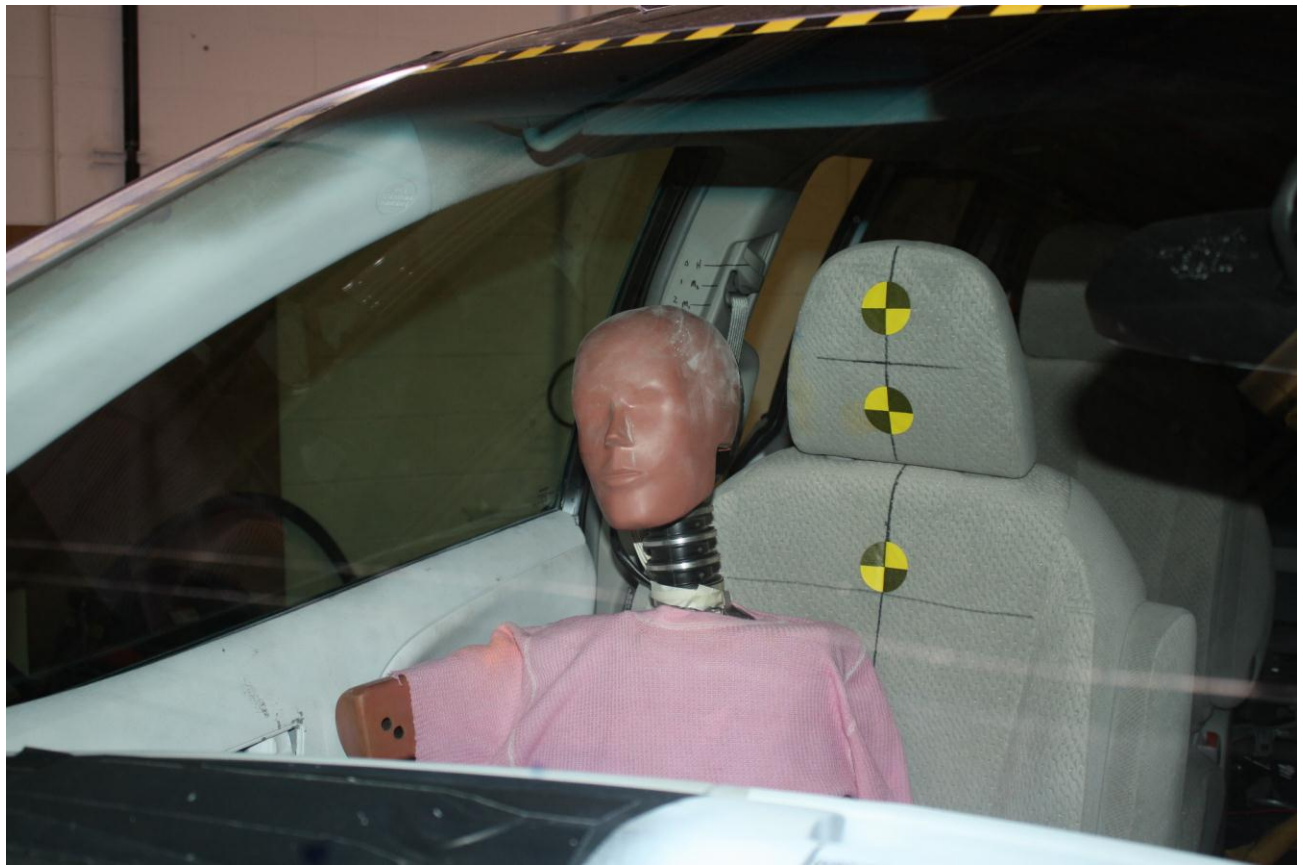
Figure A-9: Pre-Test 5th female SID-IIIs Dummy Left \frac{3}{4} Front View
