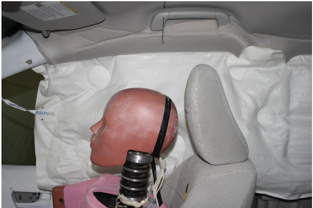
Figure A-17: Post-Test Curtain Airbag Left Side View
