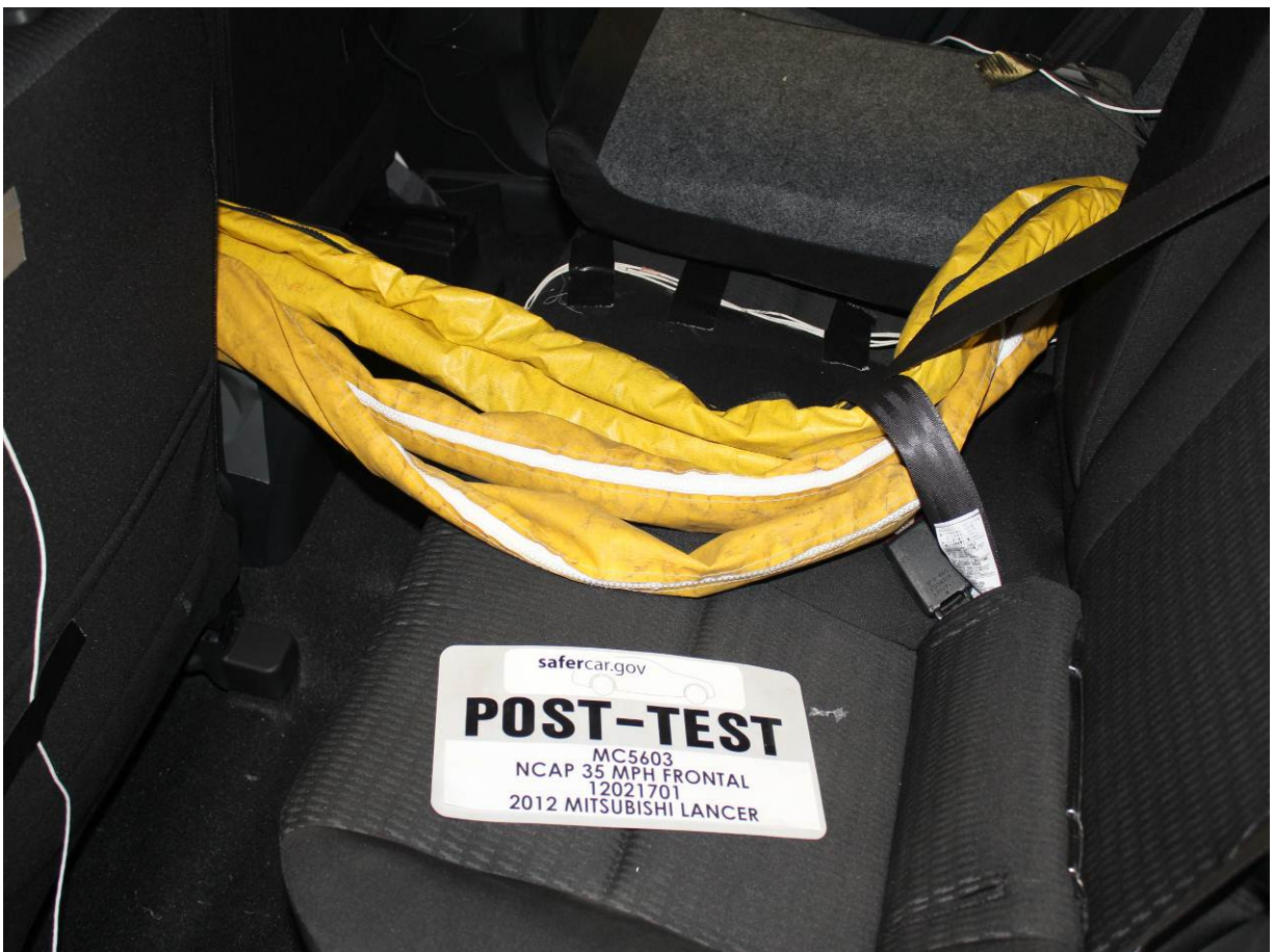
Post-Test Dummy Cable Routing
