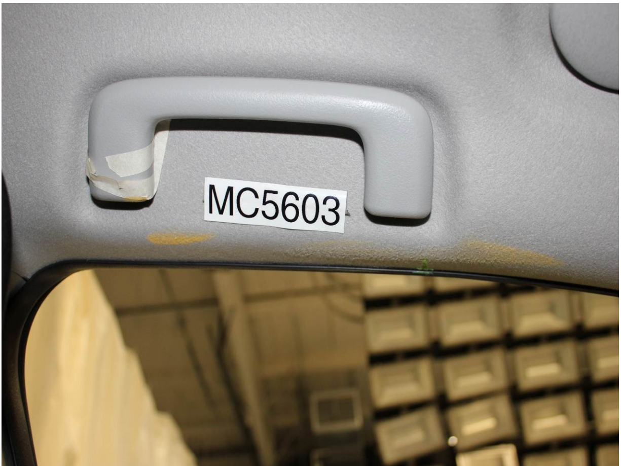
Post-Test Driver Dummy Contact with Side Header
