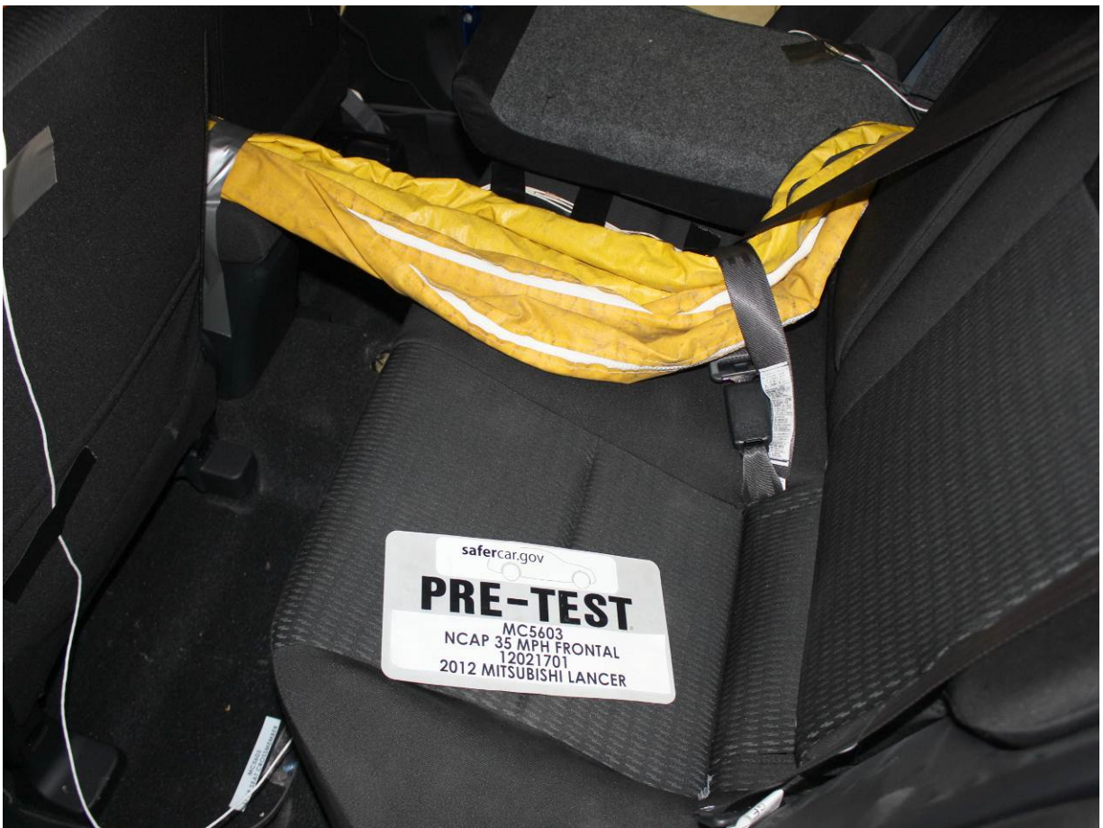
Pre-Test Dummy Cable Routing
