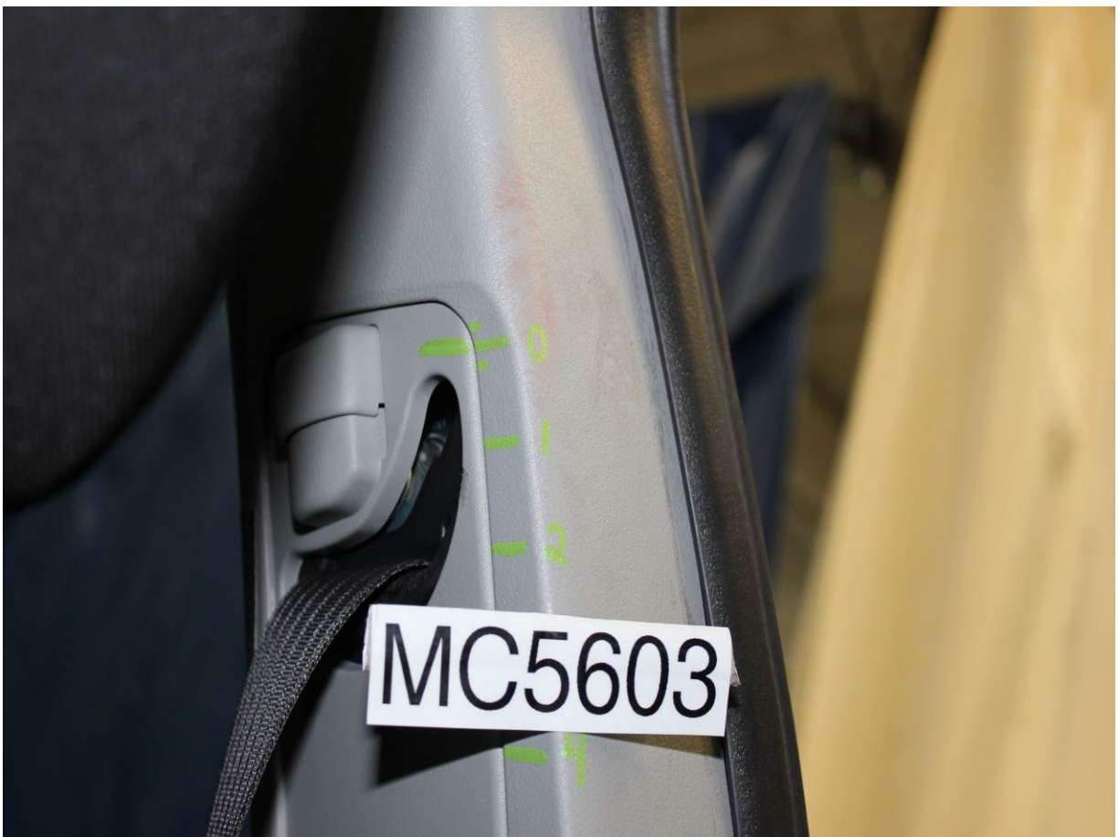
Post-Test Driver Dummy Contact with B-Pillar
