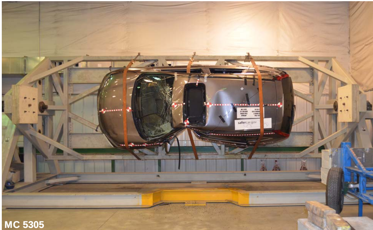
Figure 063: FMVSS No. 301 Static Rollover 90 Degrees
