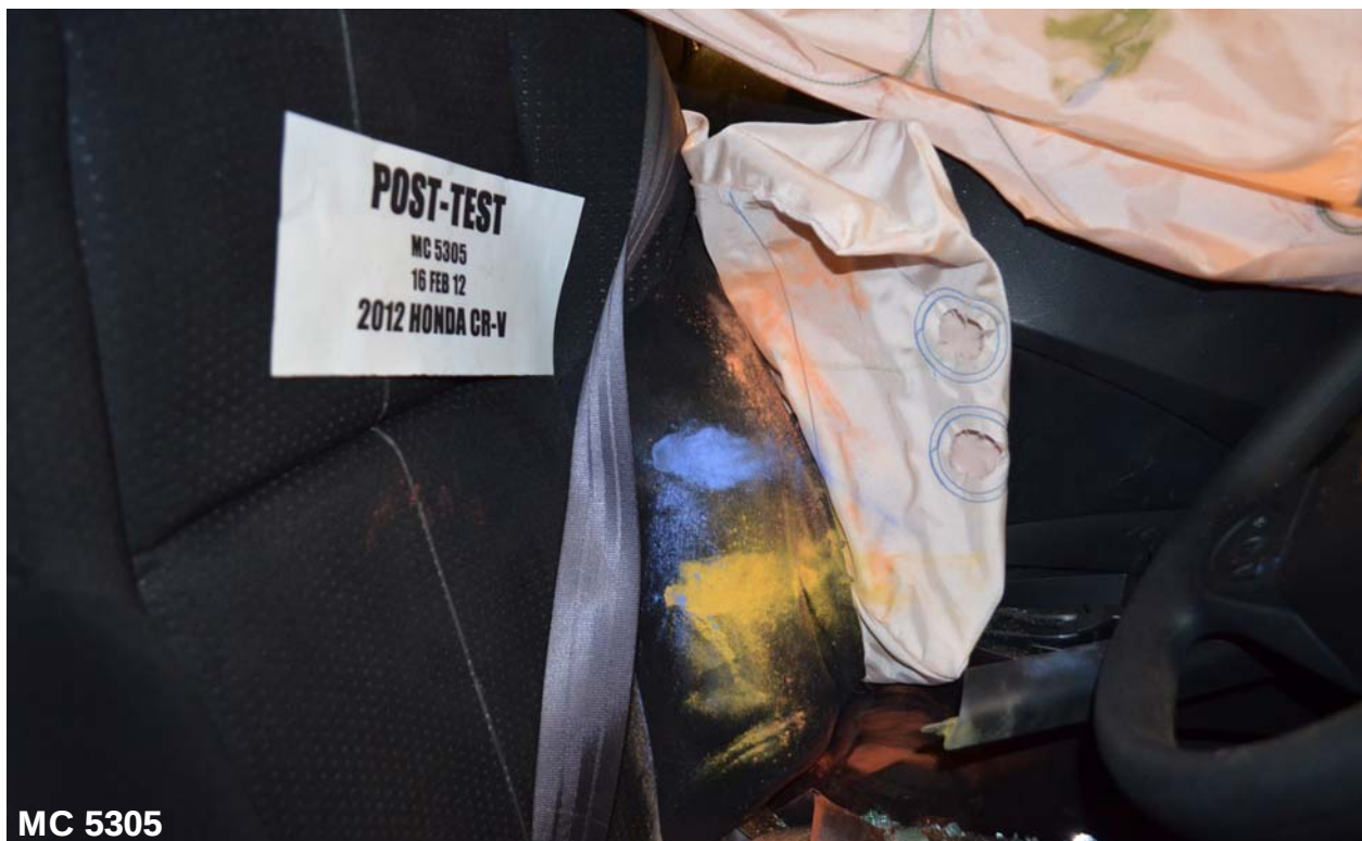
Figure 048: Post-Test Dummy Close-Up Torso Contact with Vehicle Interior View
