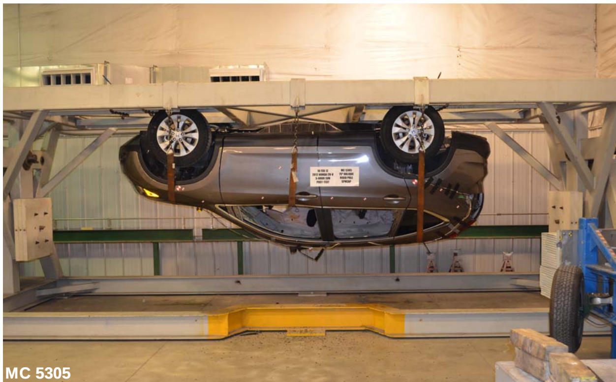
Figure 064: FMVSS No. 301 Static Rollover 180 Degrees
