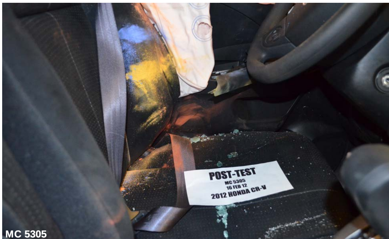
Figure 050: Post-Test Dummy Close-Up Pelvis Contact with Vehicle Interior View
