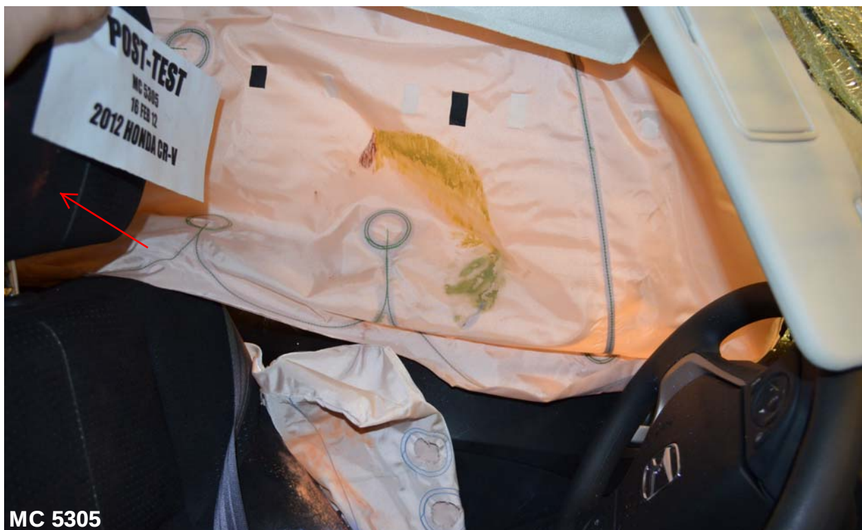
Figure 046 Post-Test Dummy Close-Up Head Contact with Vehicle Interior View
