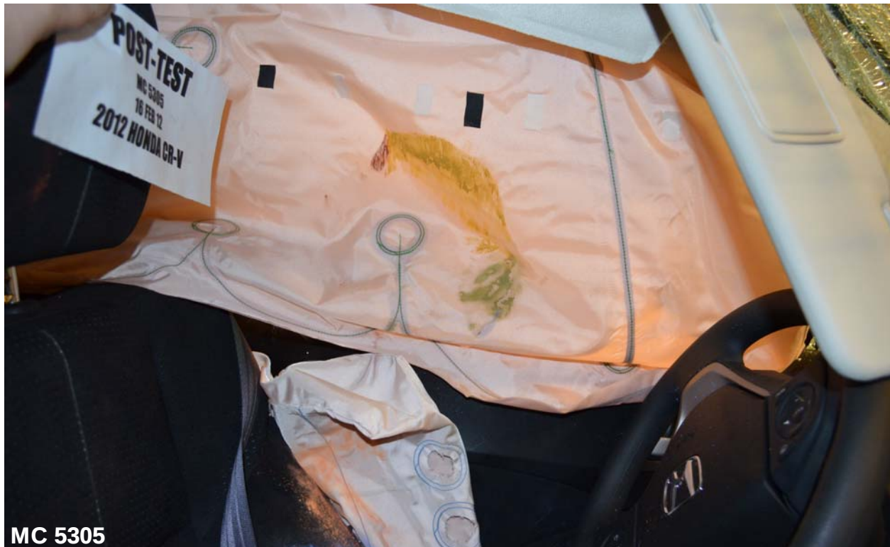
Figure 047: Post-Test Dummy Close-Up Head Contact with Side Air bag View
