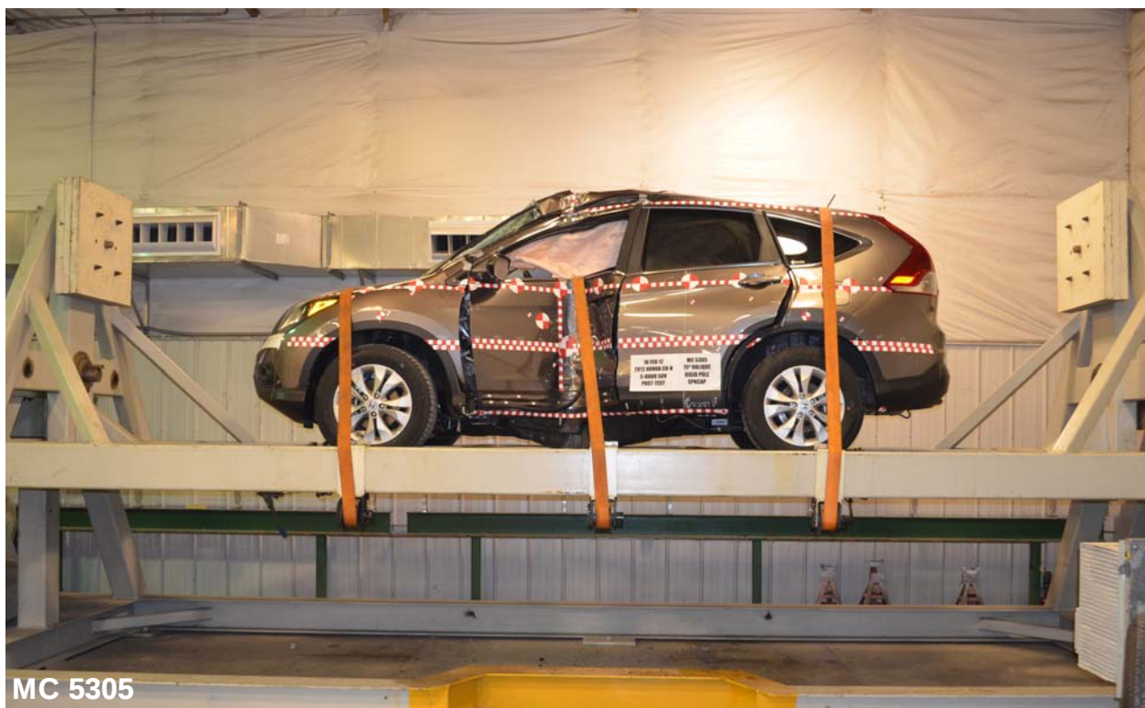
Figure 066: No. 066 FMVSS No. 301 Static Rollover 360 Degrees
