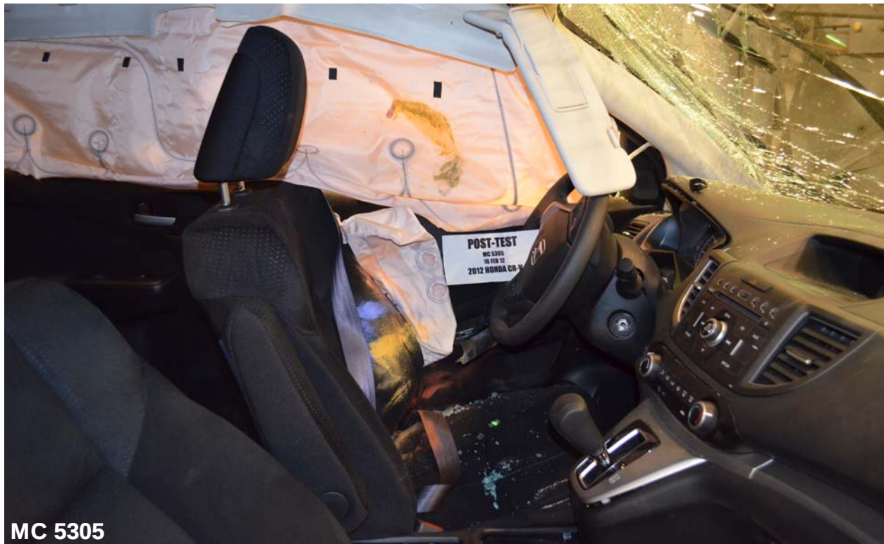
Figure 045: Post-Test Inner Door Panel View Showing Dummy Contact Locations
