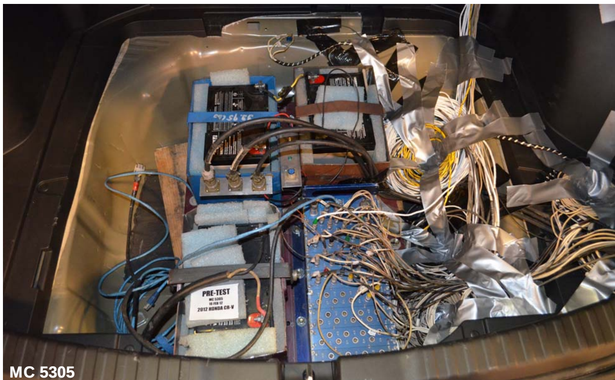
Figure 060: Pre-Test Ballast View
