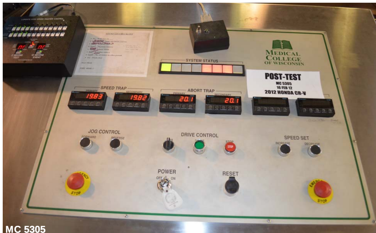
Figure 061: Post-Test Primary and Redundant Speed Trap Read-Out
