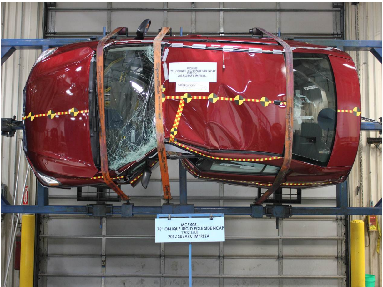
FMVSS No. 301 Static Rollover 270 Degrees
