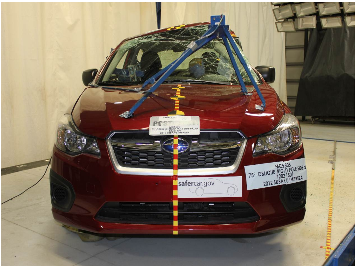
Post-Test Frontal View of Test Vehicle
