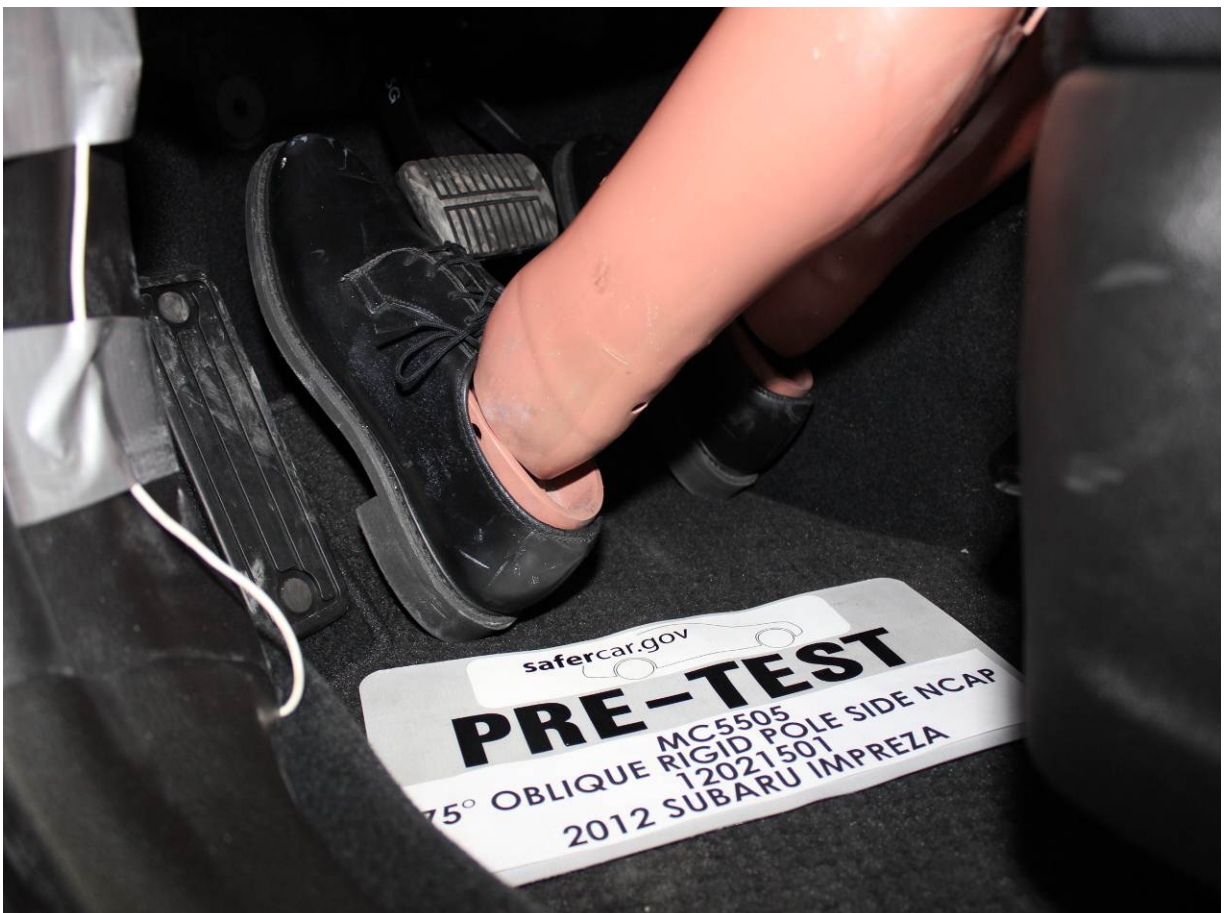
Pre-Test Placement of Dummy's Feet
