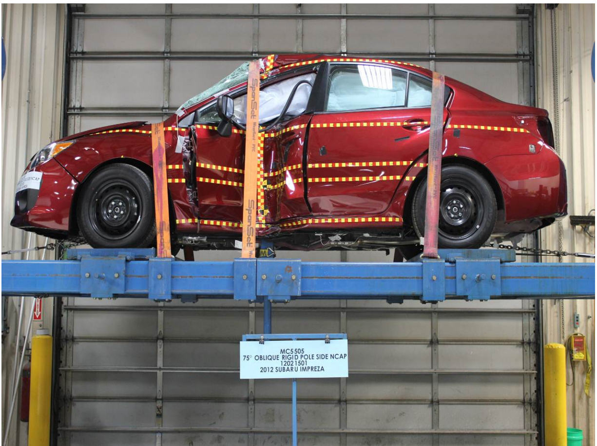
FMVSS No. 301 Static Rollover 360 Degrees
