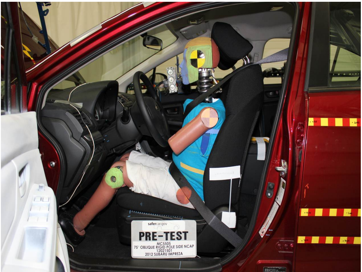
Pre-Test Left Side View of Dummy Showing Belt and Chalking
