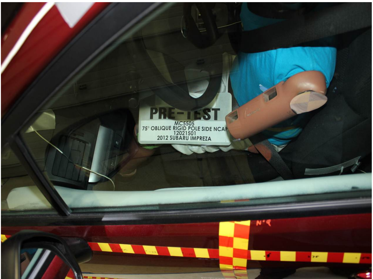
Pre-Test Dummy and Door Clearance View
