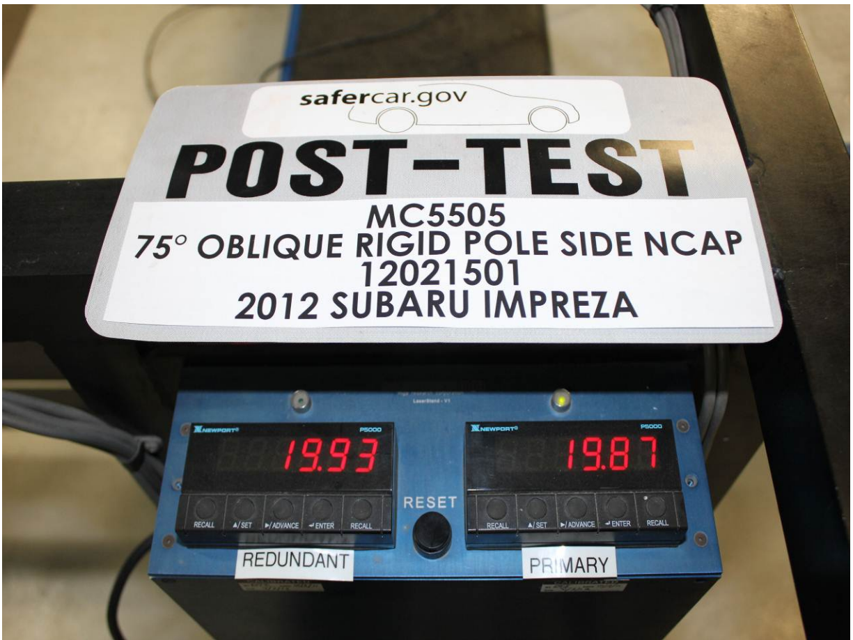
Post-Test Primary and Redundant Speed Trap Read-Out
