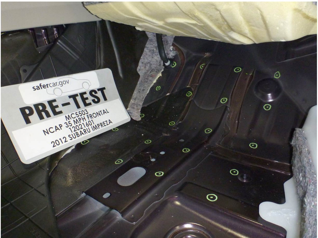
Pre-Test Passenger's Side Floorpan
