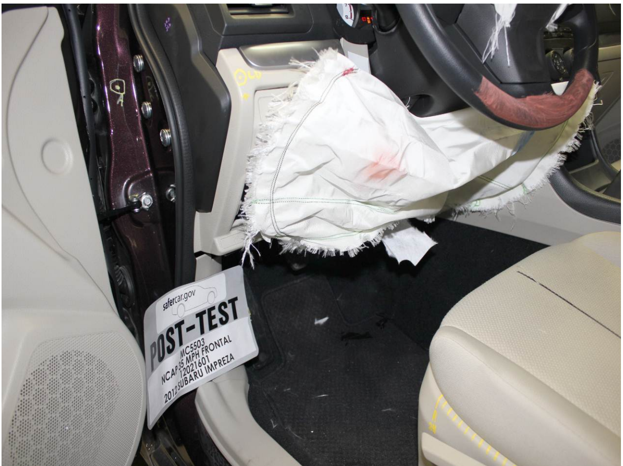
Post-Test Driver's Side Knee Bolster (without dummy)
