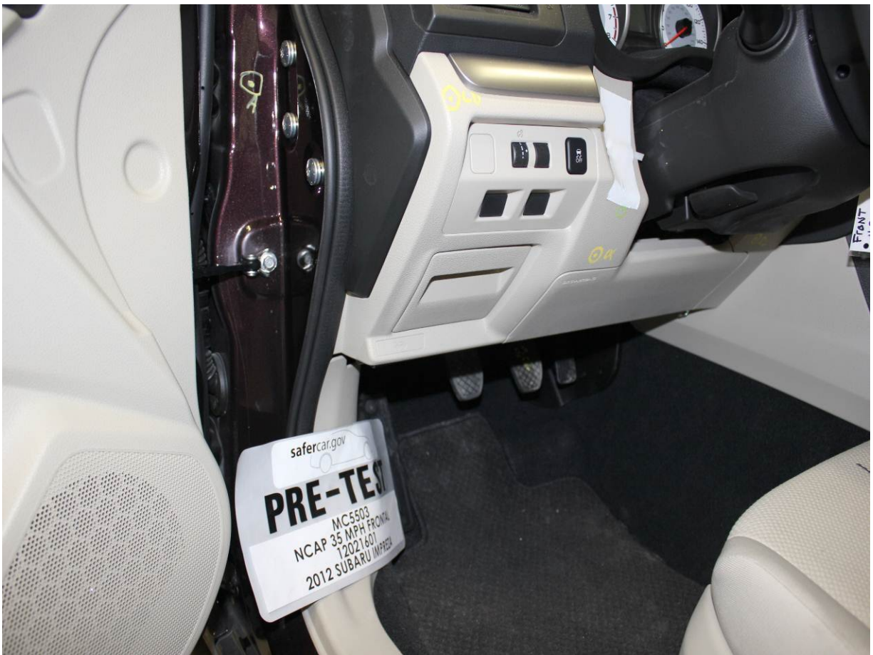
Pre-Test Driver's Side Knee Bolster (without dummy)
