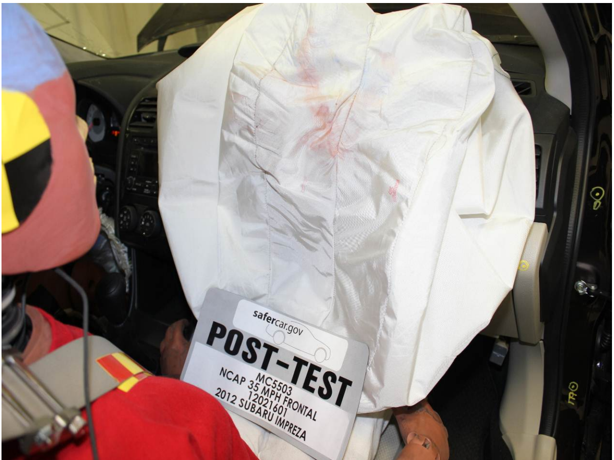
Post-Test Passenger Dummy Contact with Airbag
