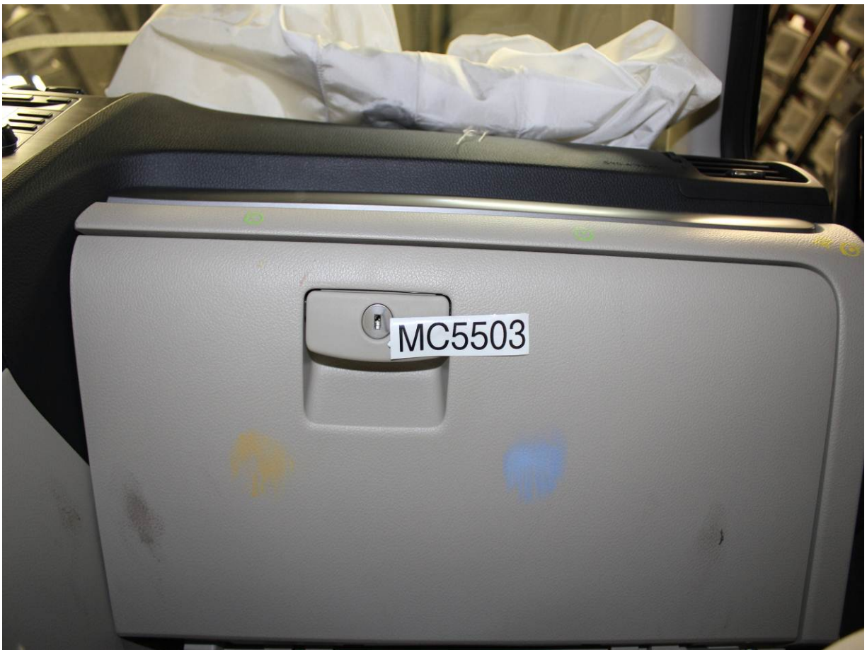
Post-Test Passenger Dummy Contact with Glovebox
