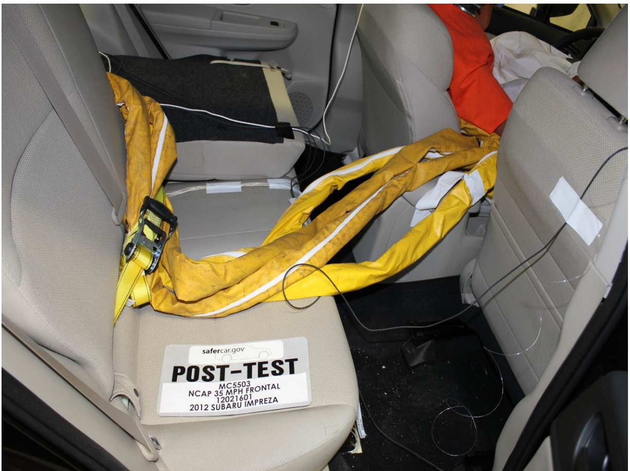
Post-Test Dummy Cable Routing
