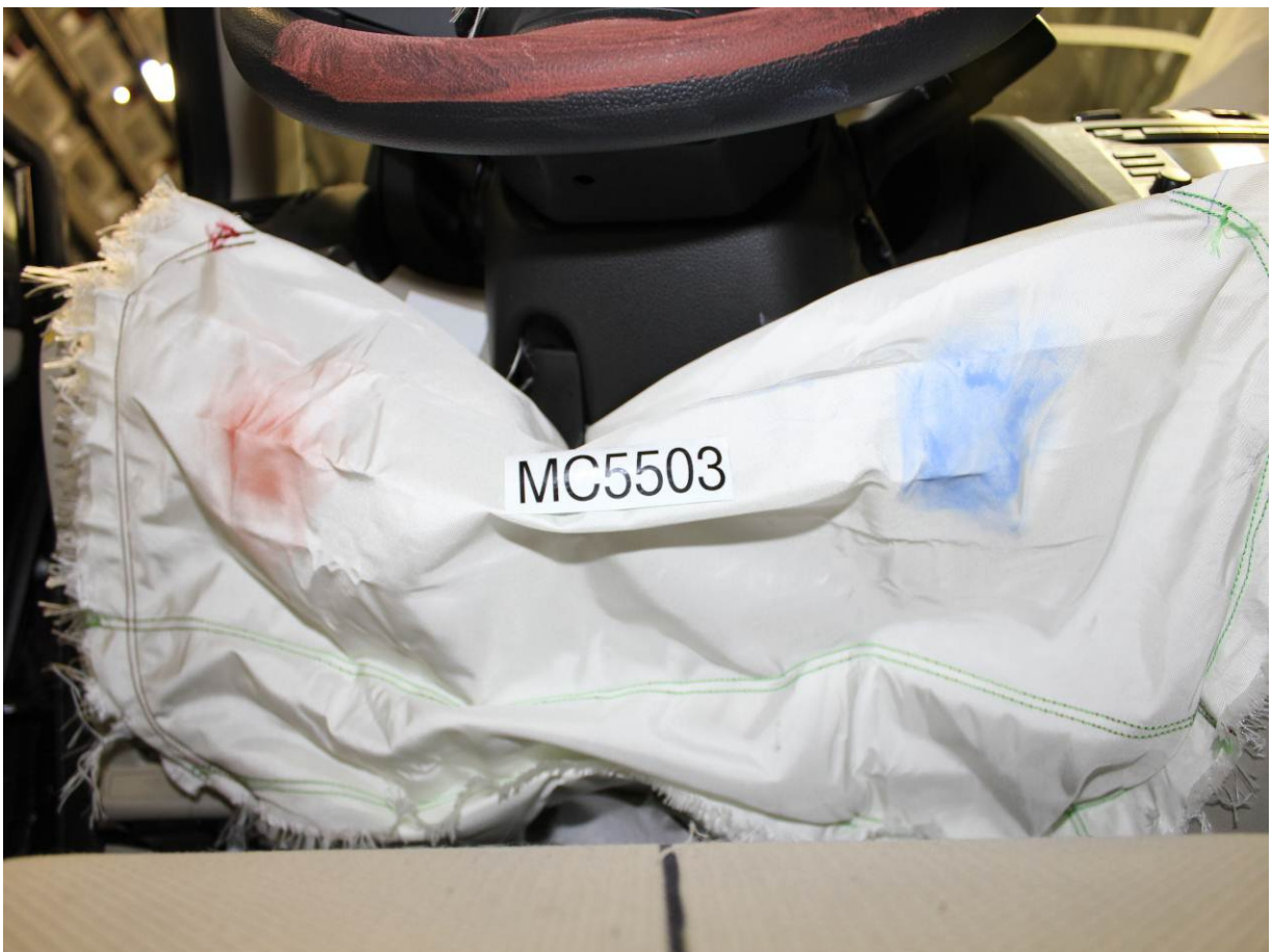
Post-Test Driver Dummy Contact with Knee Airbag
