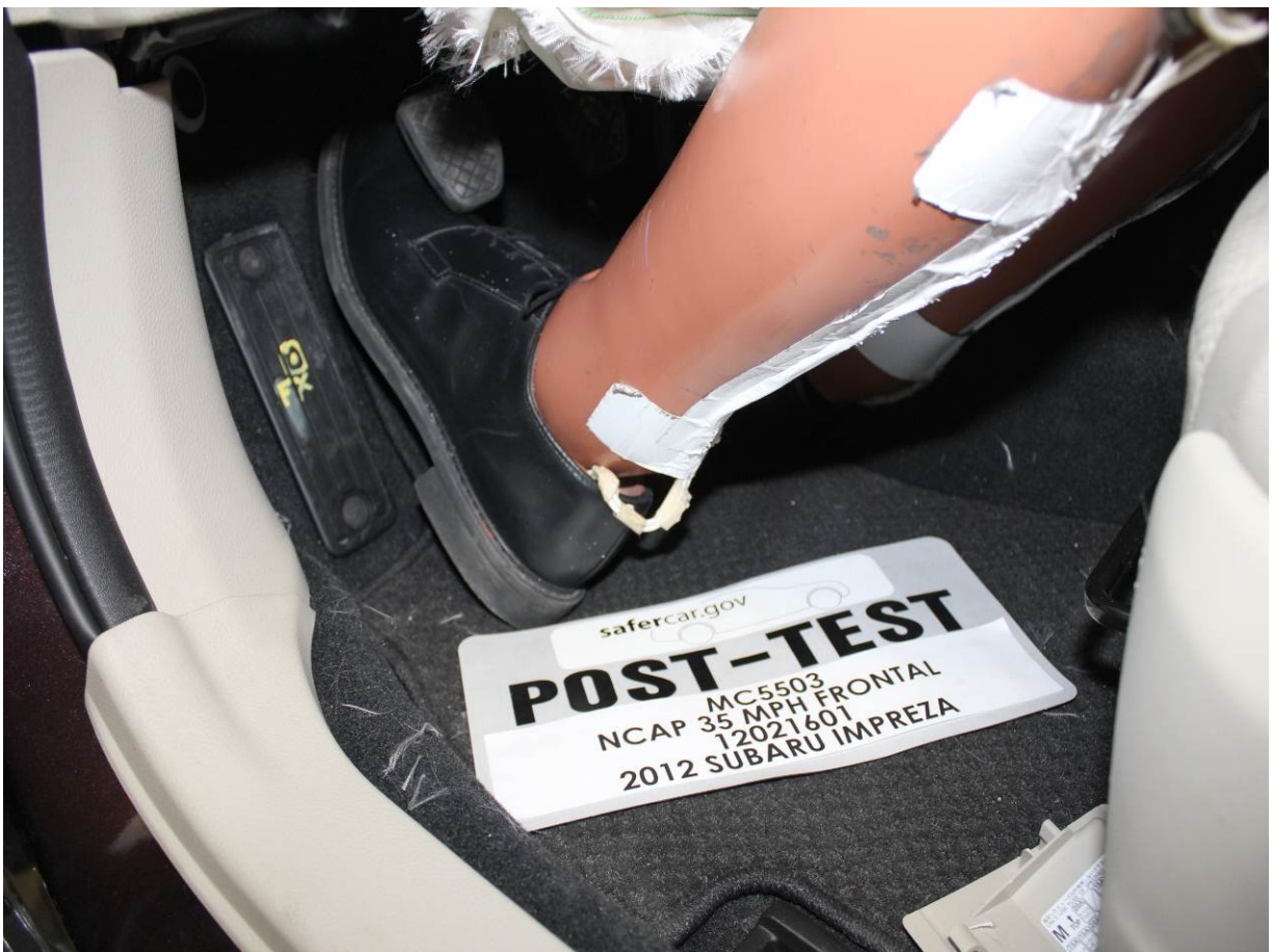
Post-Test Driver Dummy Feet
