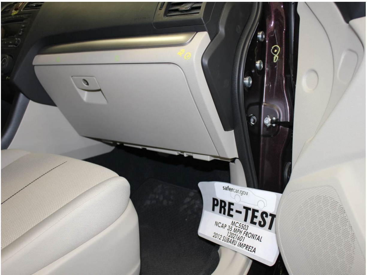
Pre-Test Passenger's Side Knee Bolster (without dummy)
