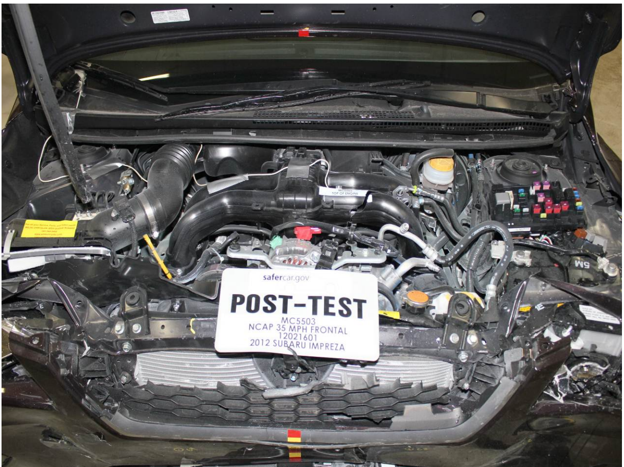
Post-Test Engine Compartment View
