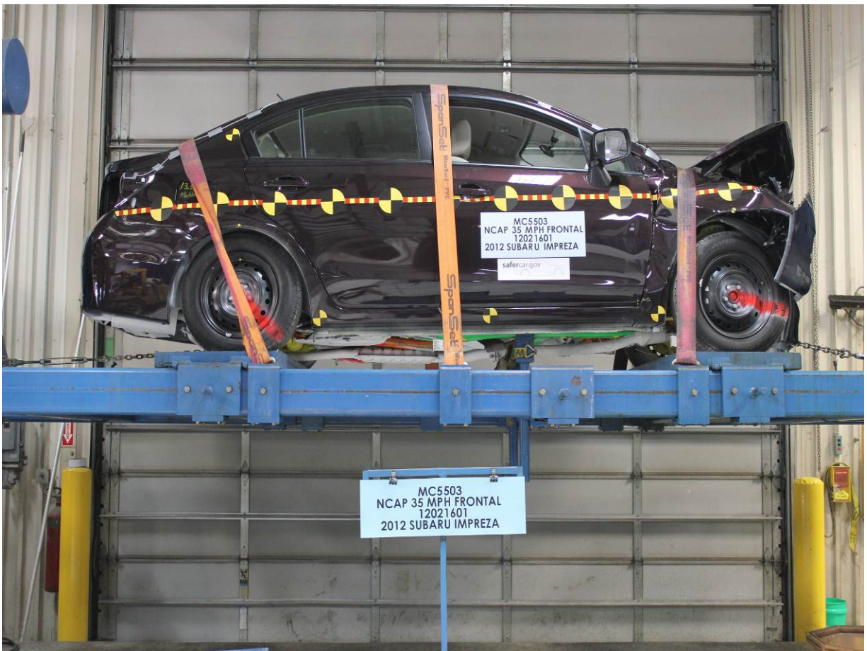
Vehicle at 0 Degrees on Static Rollover Device
