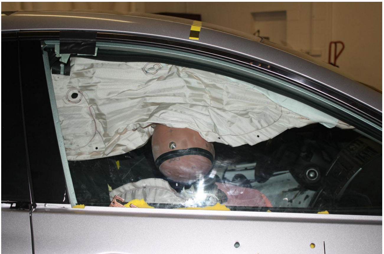
Figure A-20: Post-Test Curtain Airbag Right Side View
