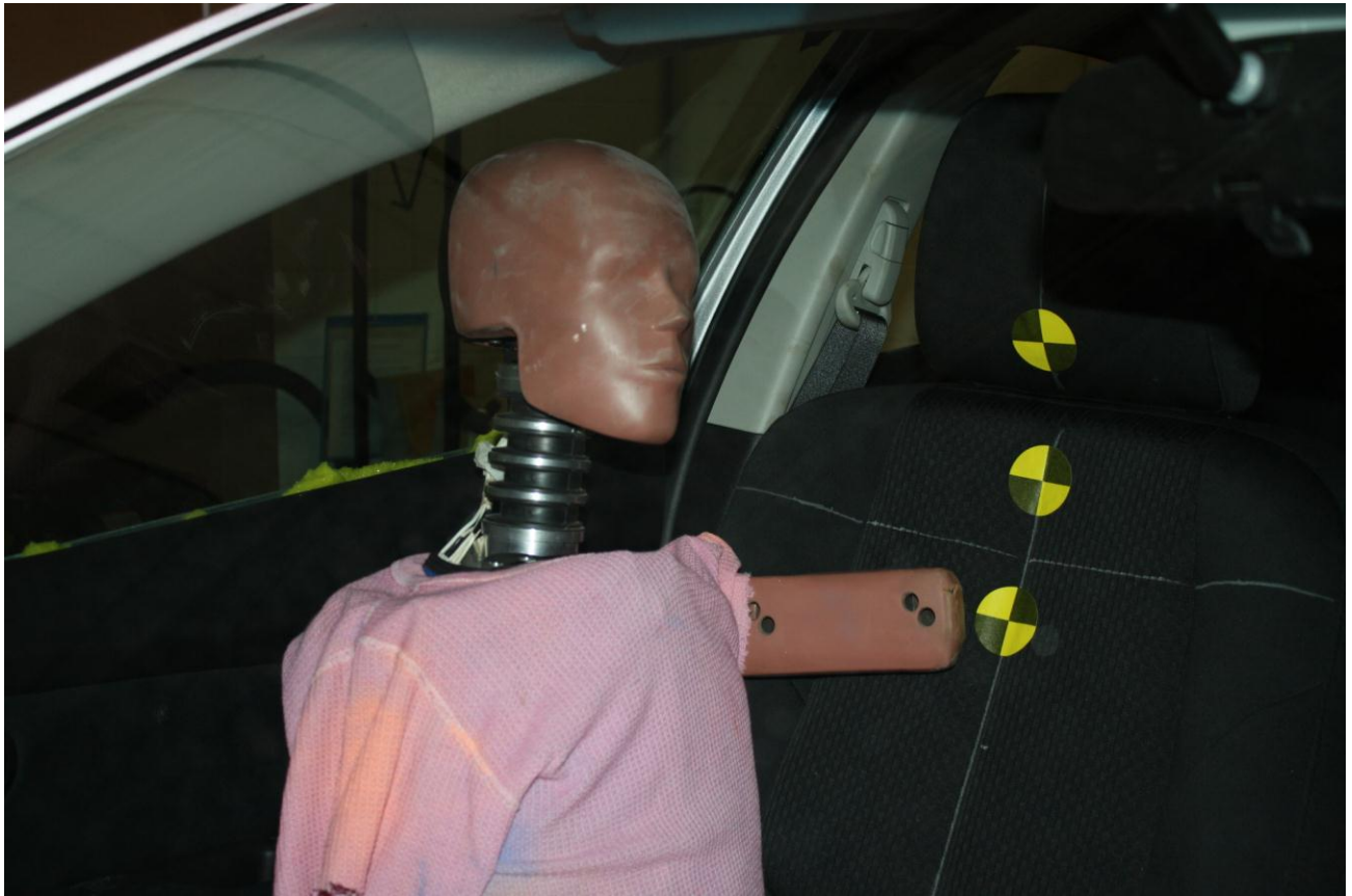
Figure A-11: Pre-Test 5th female SID-IIIs Dummy Left ¾ Front Closeup View
