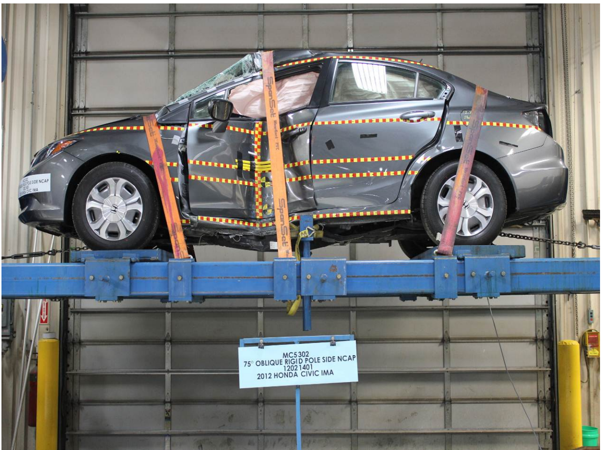
Vehicle at 360 Degrees on Static Rollover Device
