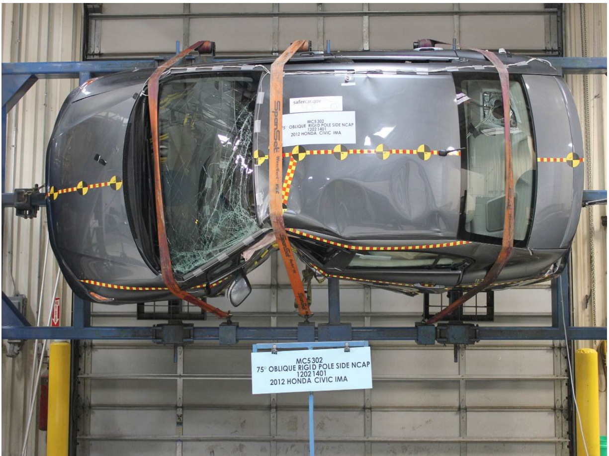
Vehicle at 90 Degrees on Static Rollover Device
