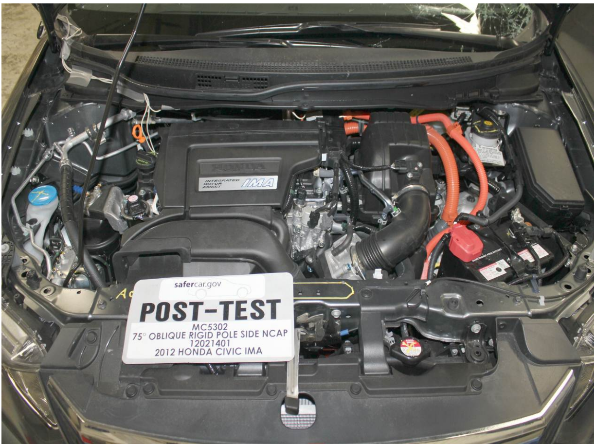
Post-Test View of Electric Propulsion Drive
