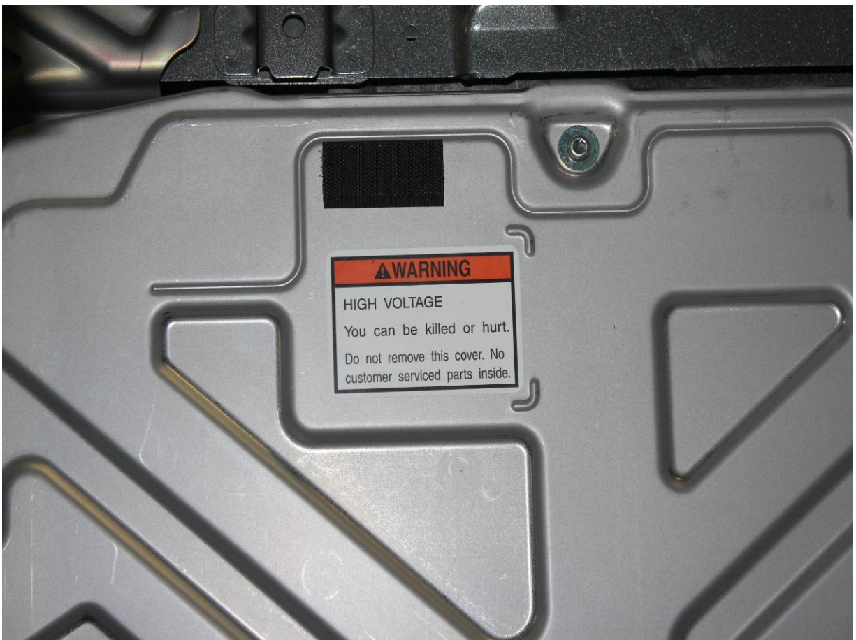
High Voltage Warning Label
