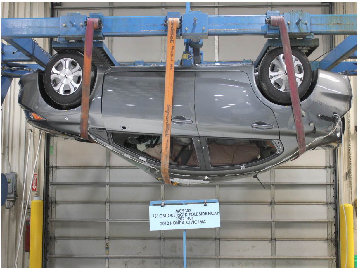
Vehicle at 180 Degrees on Static Rollover Device
