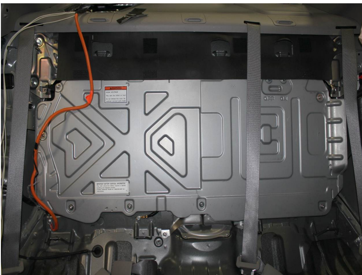
Post-Test View of Electric Energy Storage/Conversion System
