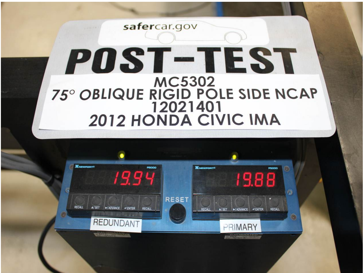
Post-Test Primary and Redundant Speed Trap Read-Out
