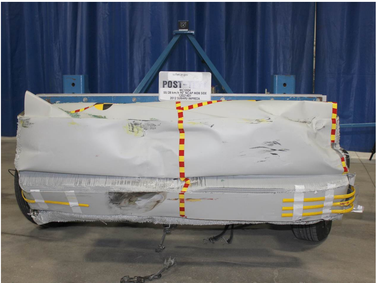
Post-Test Front View of MDB Impactor Face
