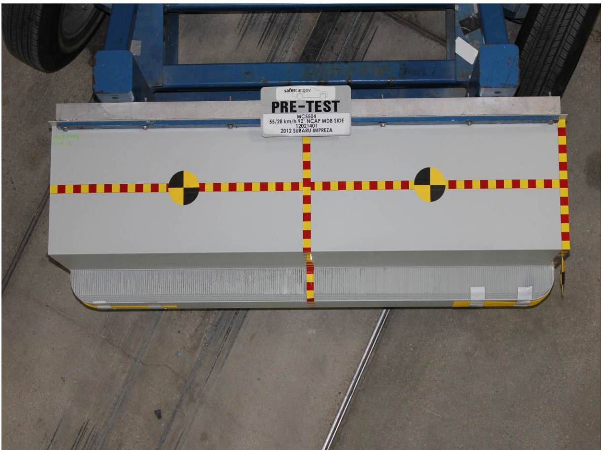
Pre-Test Top View of MDB Impactor Face
