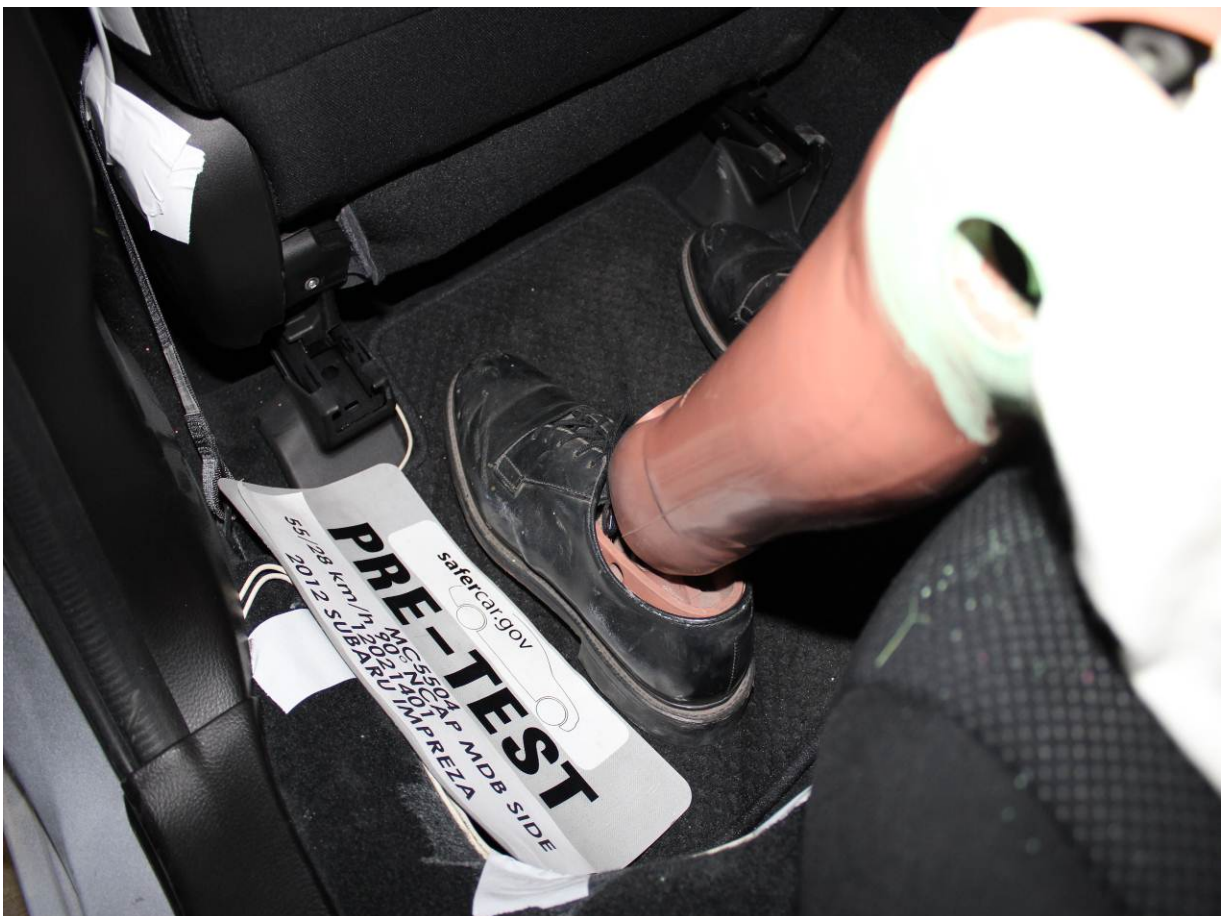
Pre-Test Placement of Rear Passenger Dummy's Feet
