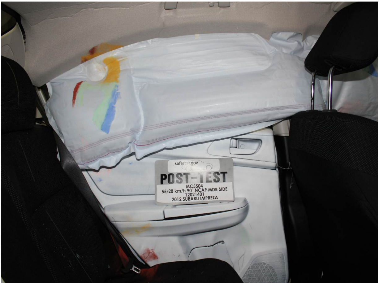
Post-Test Rear Passenger Inner Door Panel View
