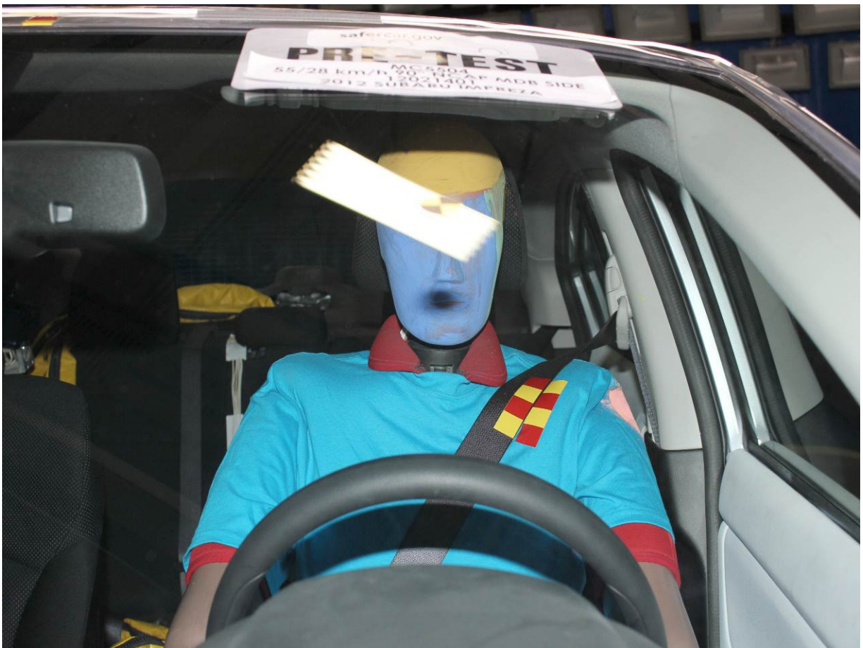
Pre-Test Front Close-Up View of Driver Dummy
