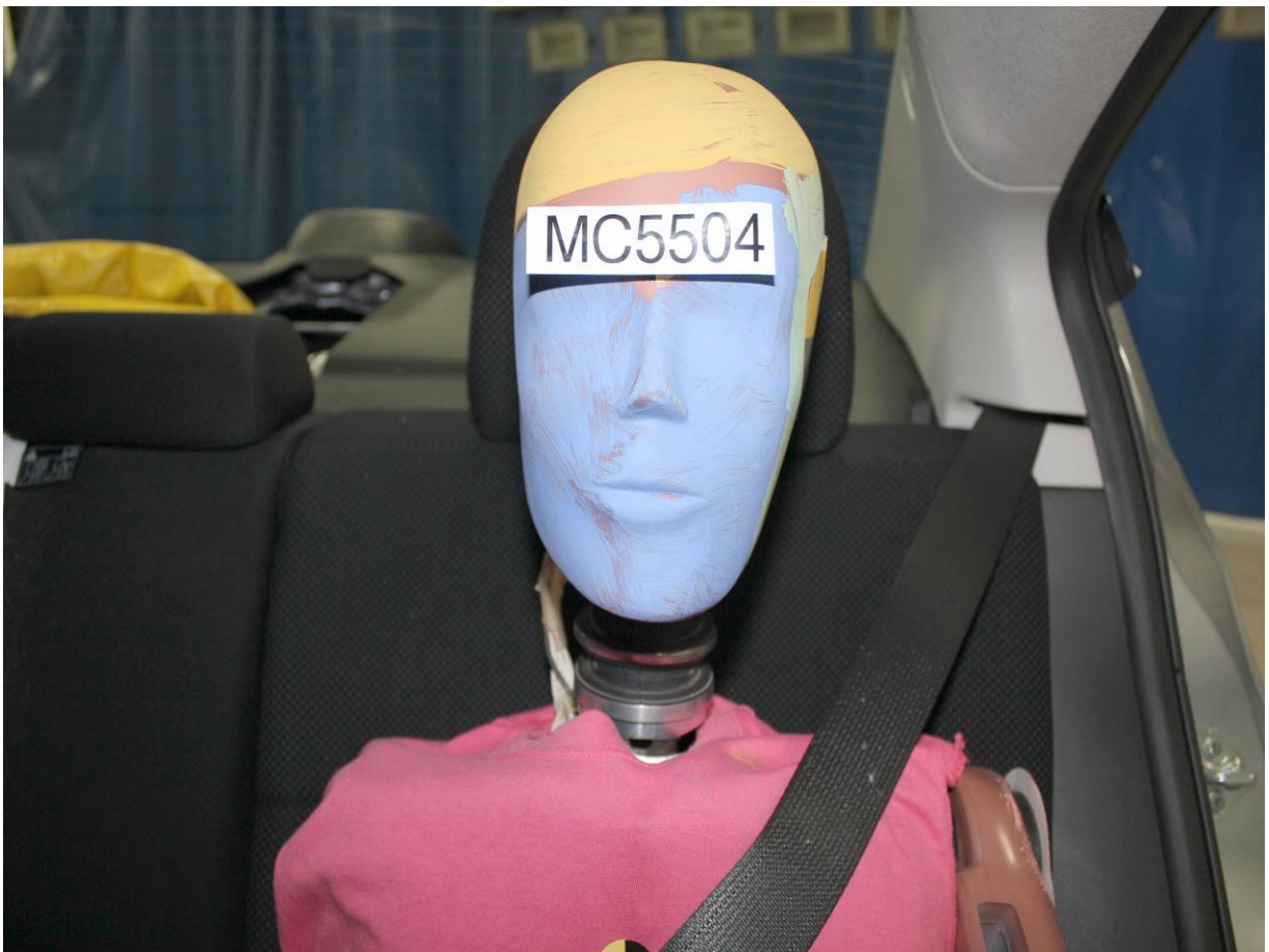
Pre-Test Frontal View of Rear Passenger Dummy Head and Shoulders in Relation to Head Restraint
