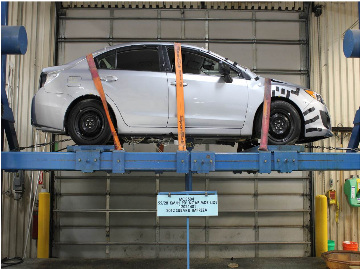
FMVSS No. 301 Static Rollover 0 Degrees
