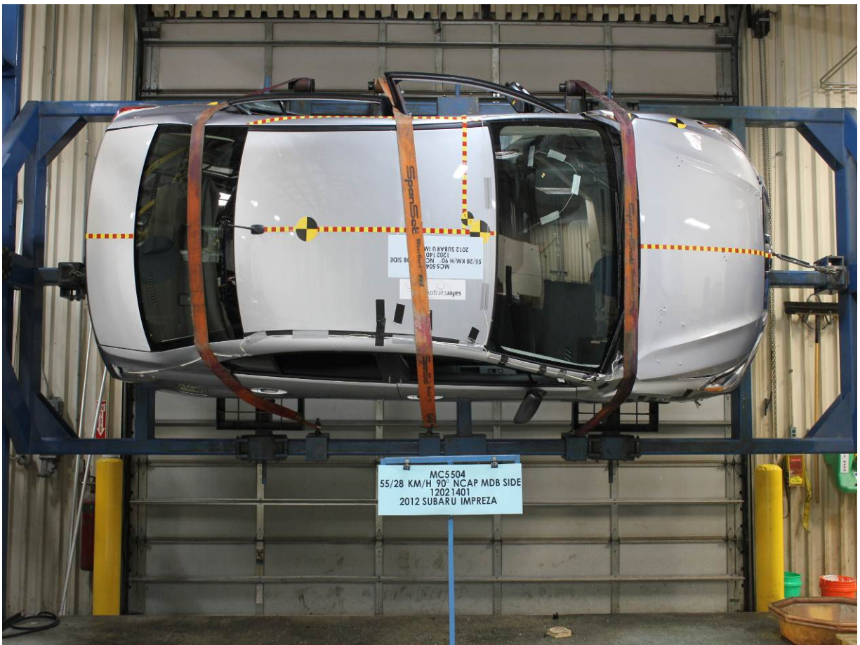
FMVSS No. 301 Static Rollover 90 Degrees
