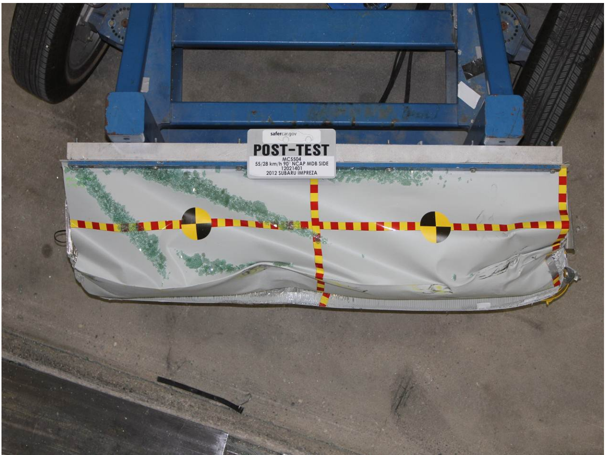
Post-Test Top View of MDB Impactor Face
