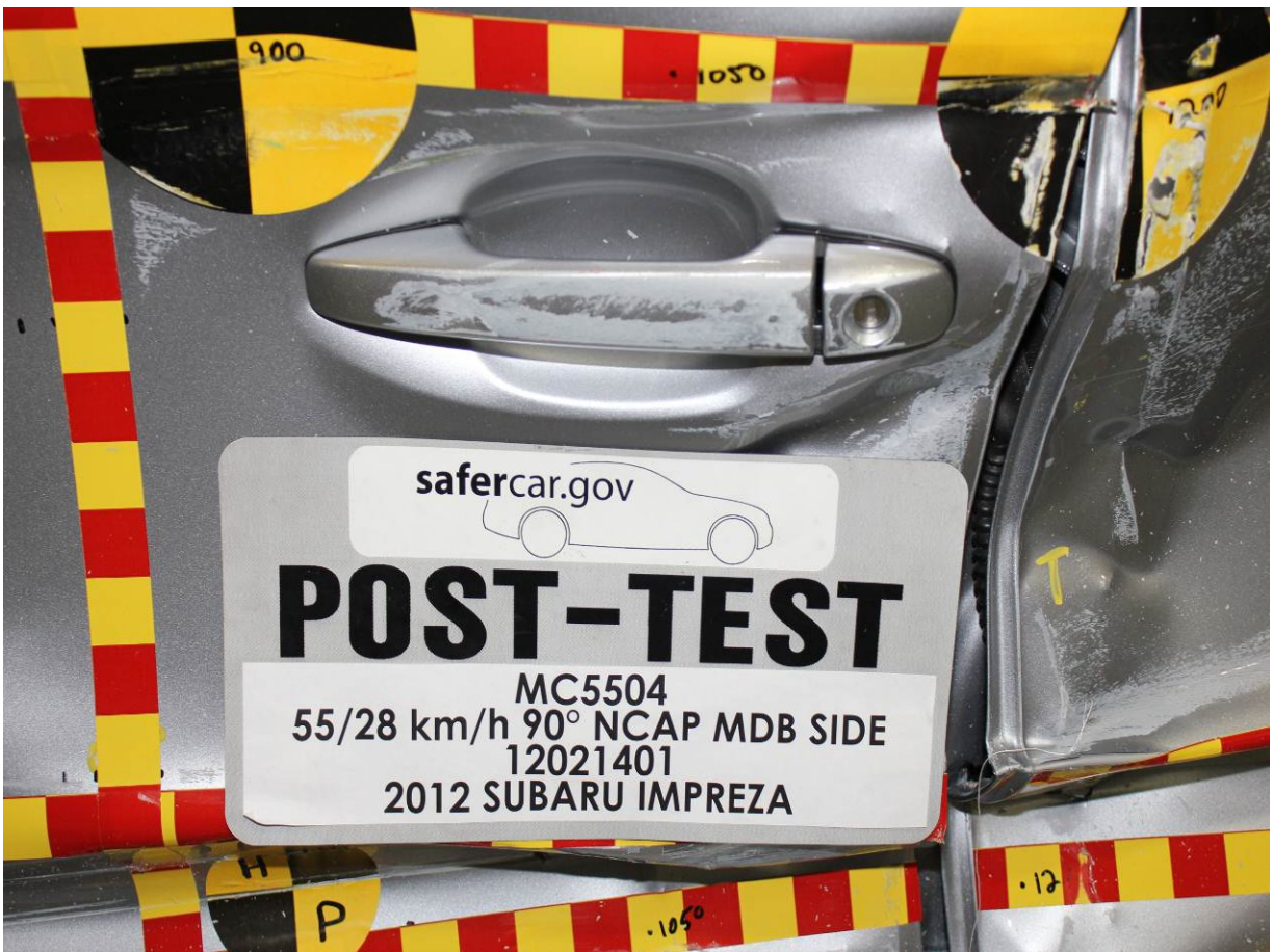
Post-Test Left Front Door Latch Close-Up
