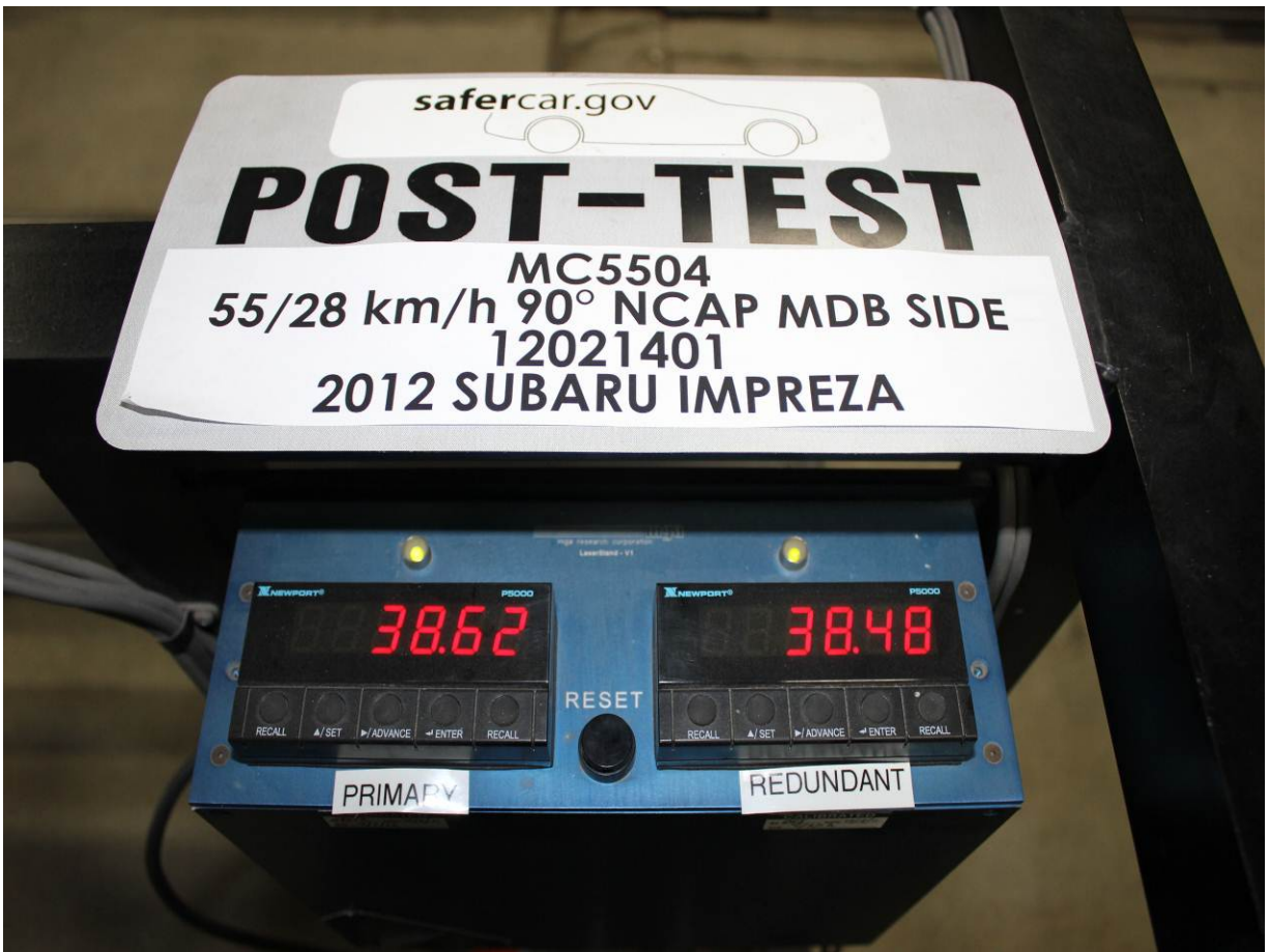
Post-Test Primary and Redundant Speed Trap Read-Out
