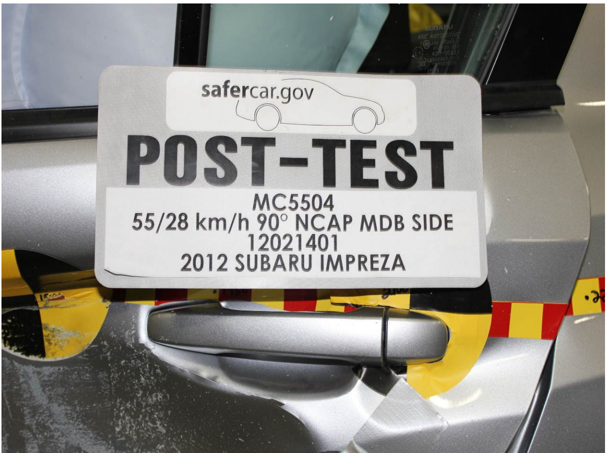
Post-Test Left Rear Door Latch Close-Up
