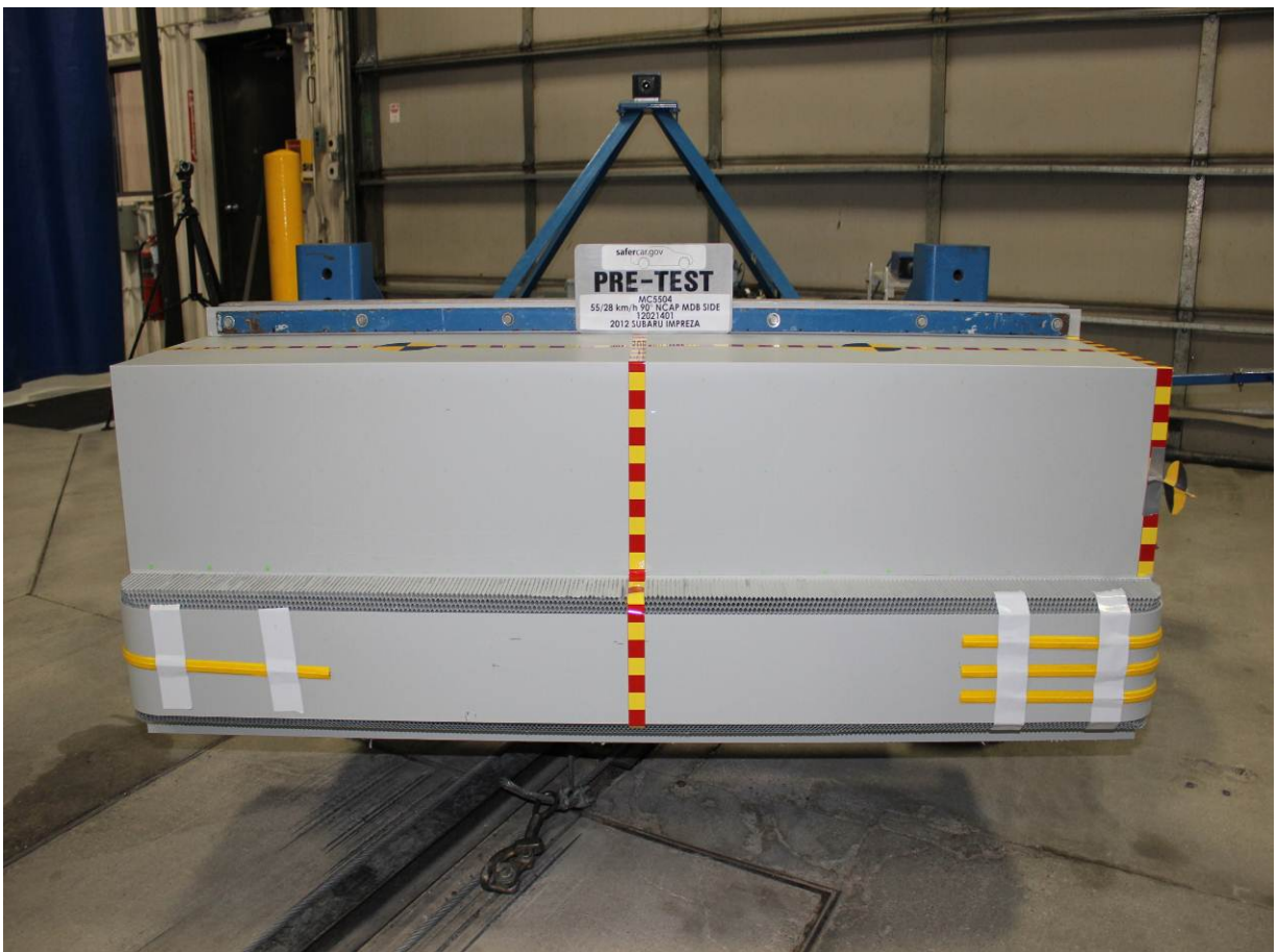
Pre-Test Front View of MDB Impactor Face
