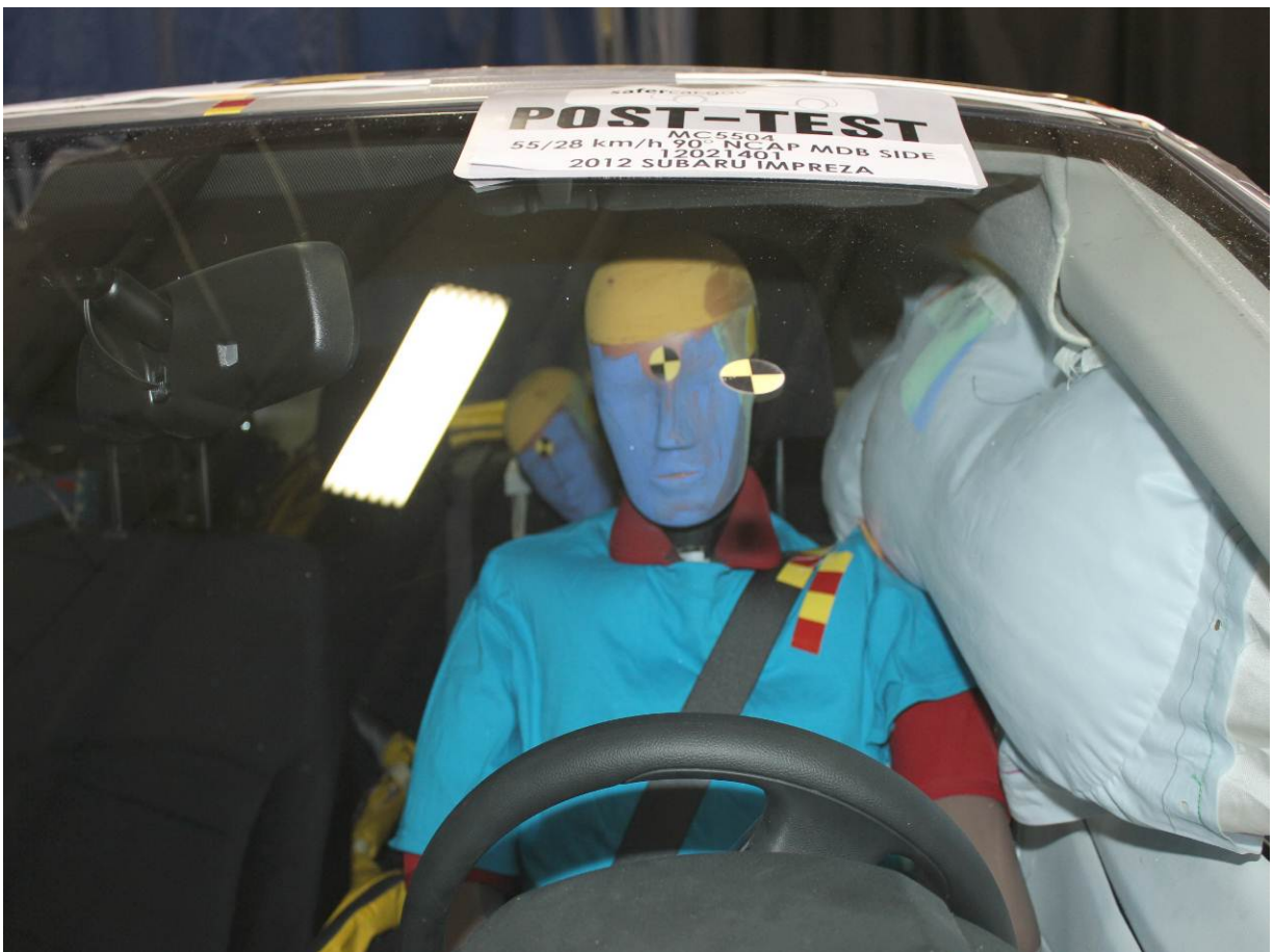
Post-Test Front Close-Up View of Driver Dummy
