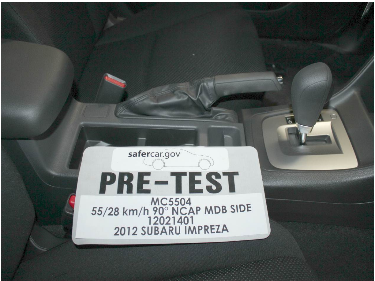
Pre-Test View of Disengaged Parking Brake
