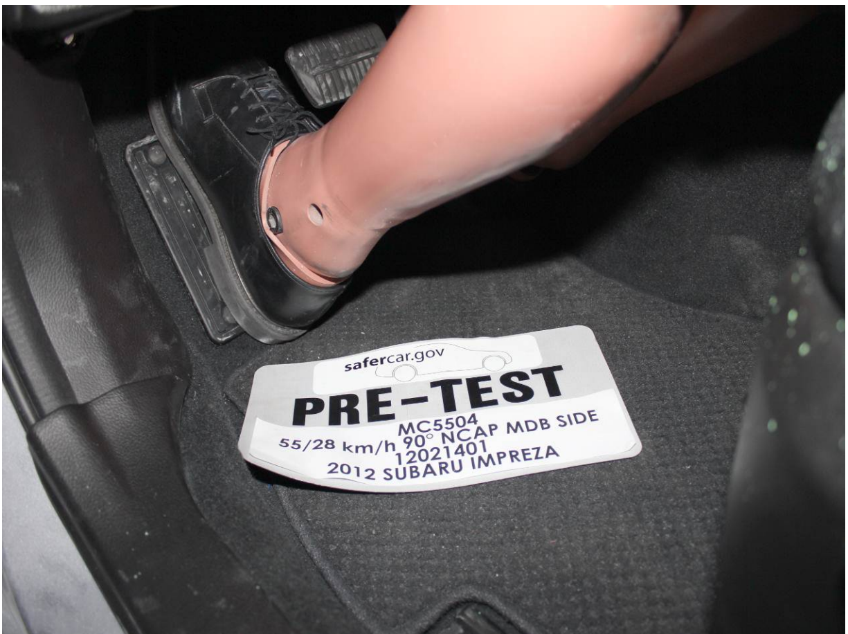
Pre-Test Placement of Driver Dummy's Feet
