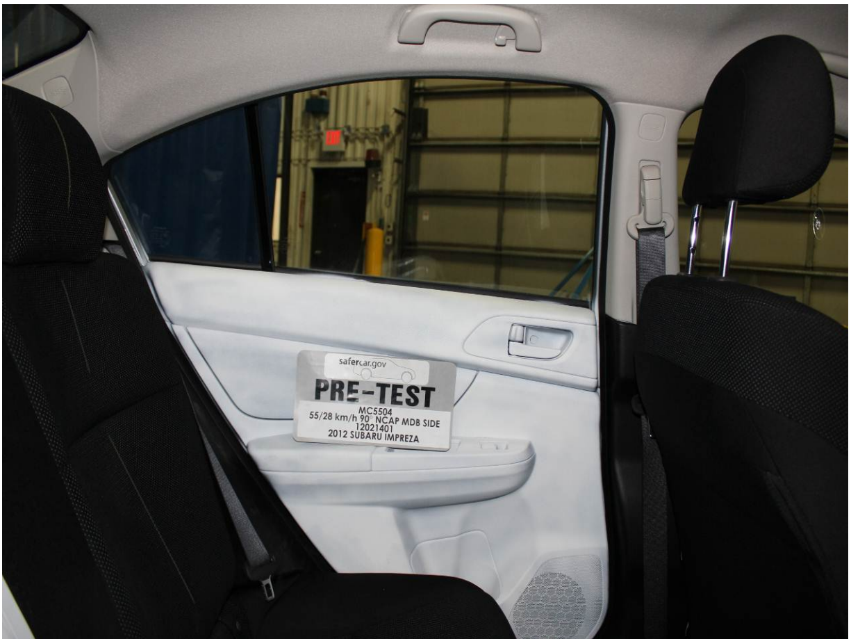
Pre-Test Rear Passenger Inner Door Panel View
