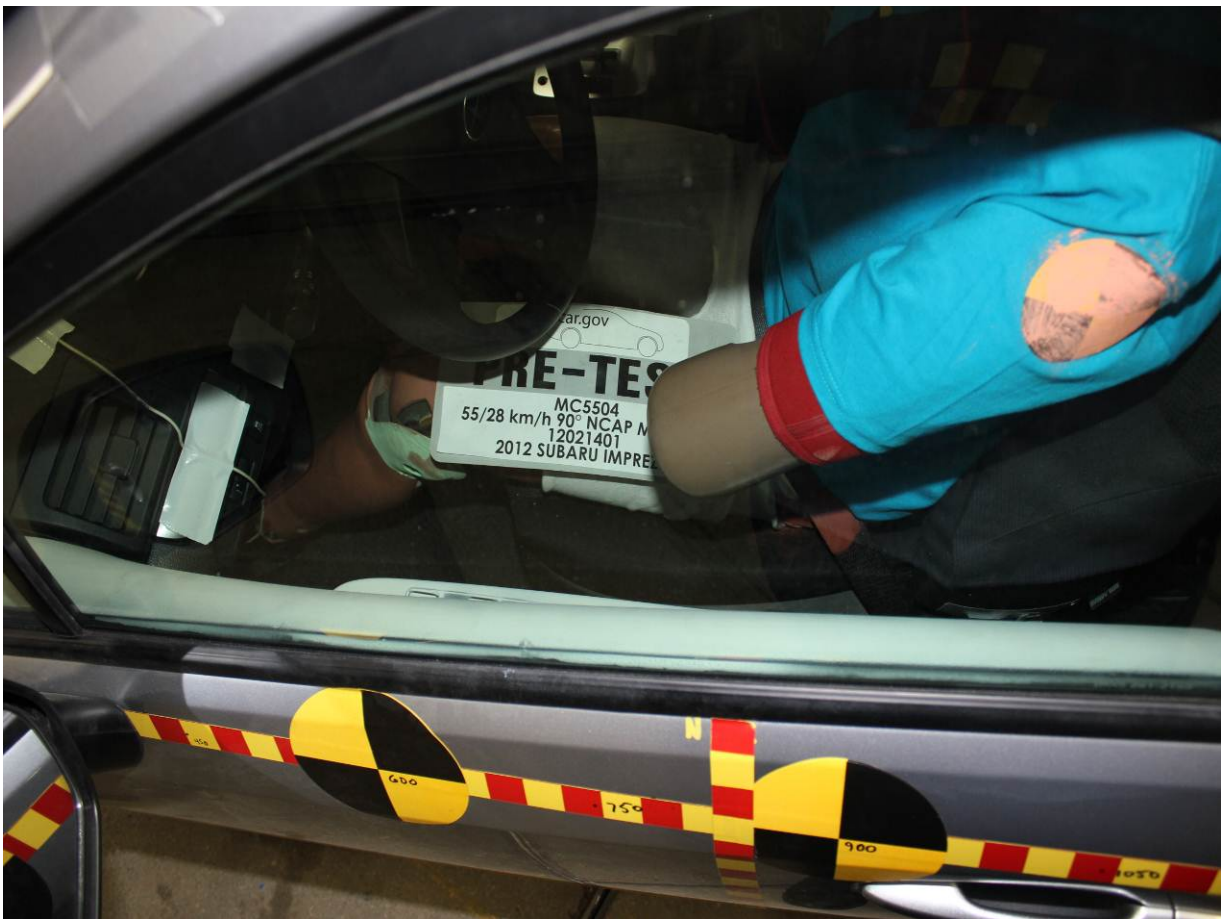
Pre-Test Driver Dummy and Door Clearance View
