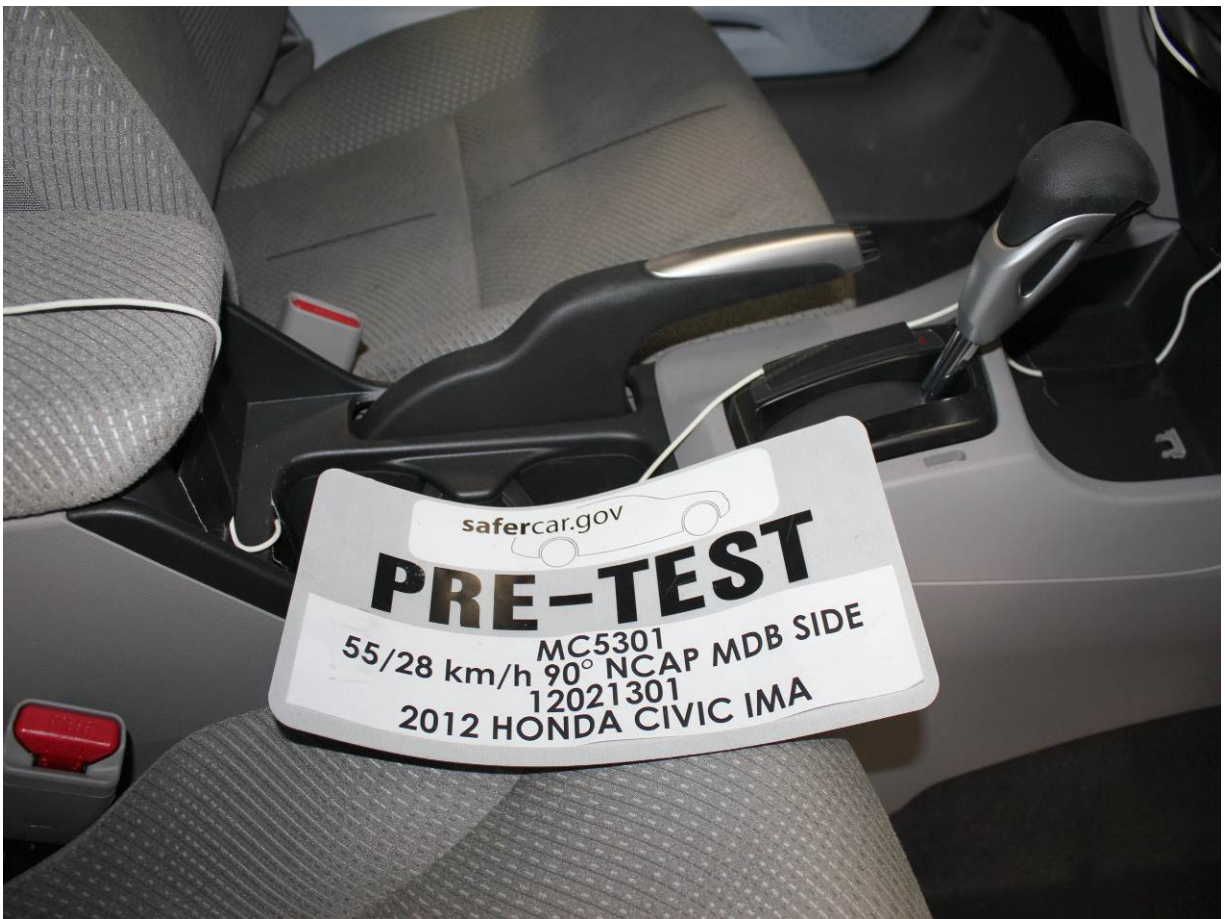
Pre-Test View of Disengaged Parking Brake
