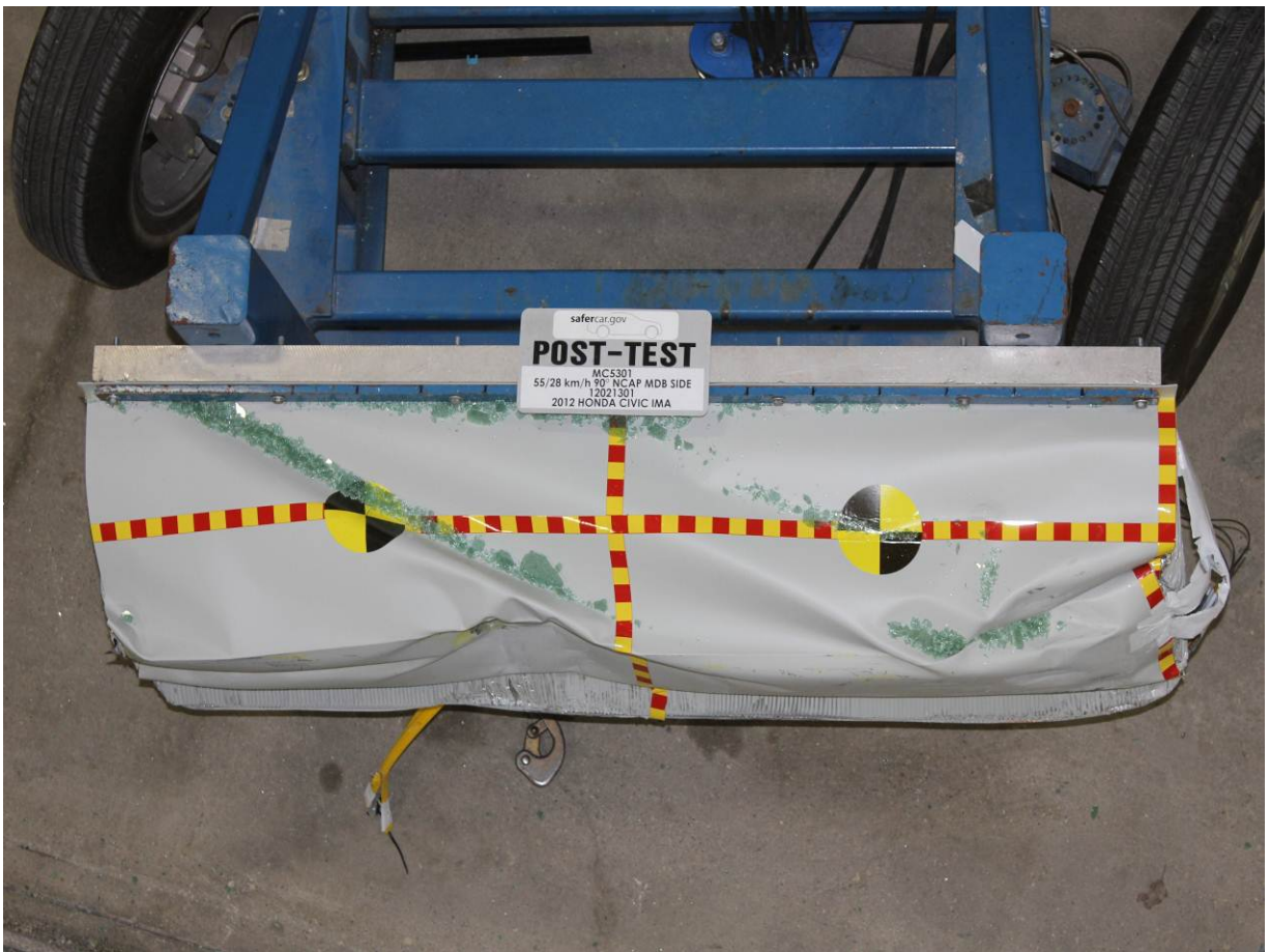
Post-Test Top View of MDB Impactor Face
