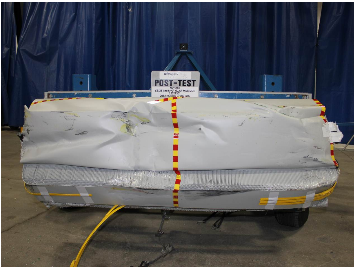
Post-Test Front View of MDB Impactor Face
