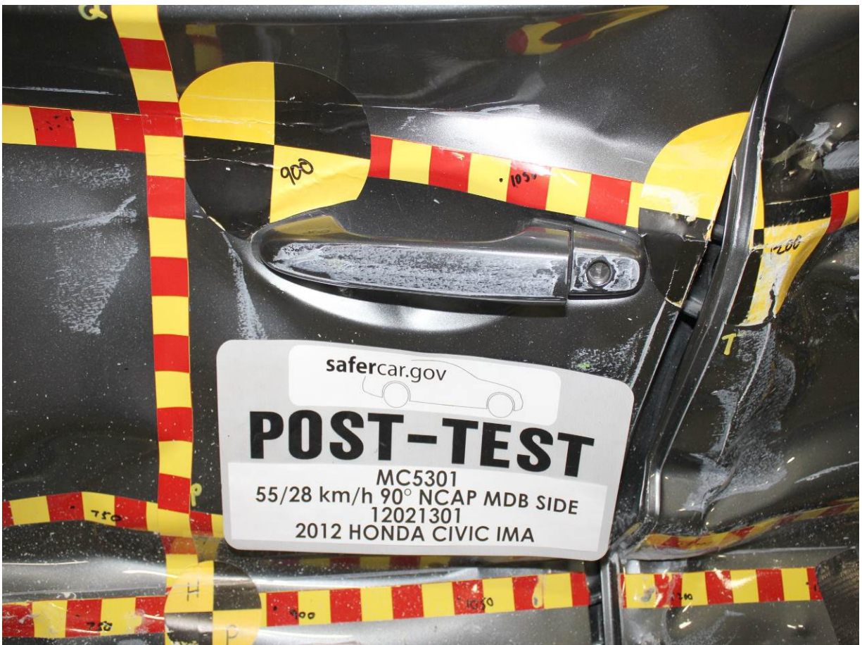
Post-Test Left Front Door Latch Close-Up
