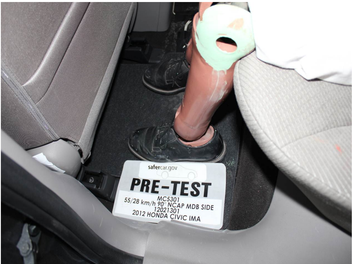
Pre-Test Placement of Rear Passenger Dummy's Feet
