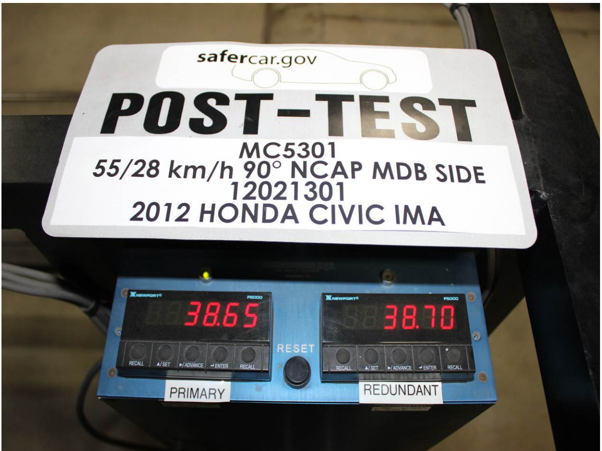
Post-Test Primary and Redundant Speed Trap Read-Out
