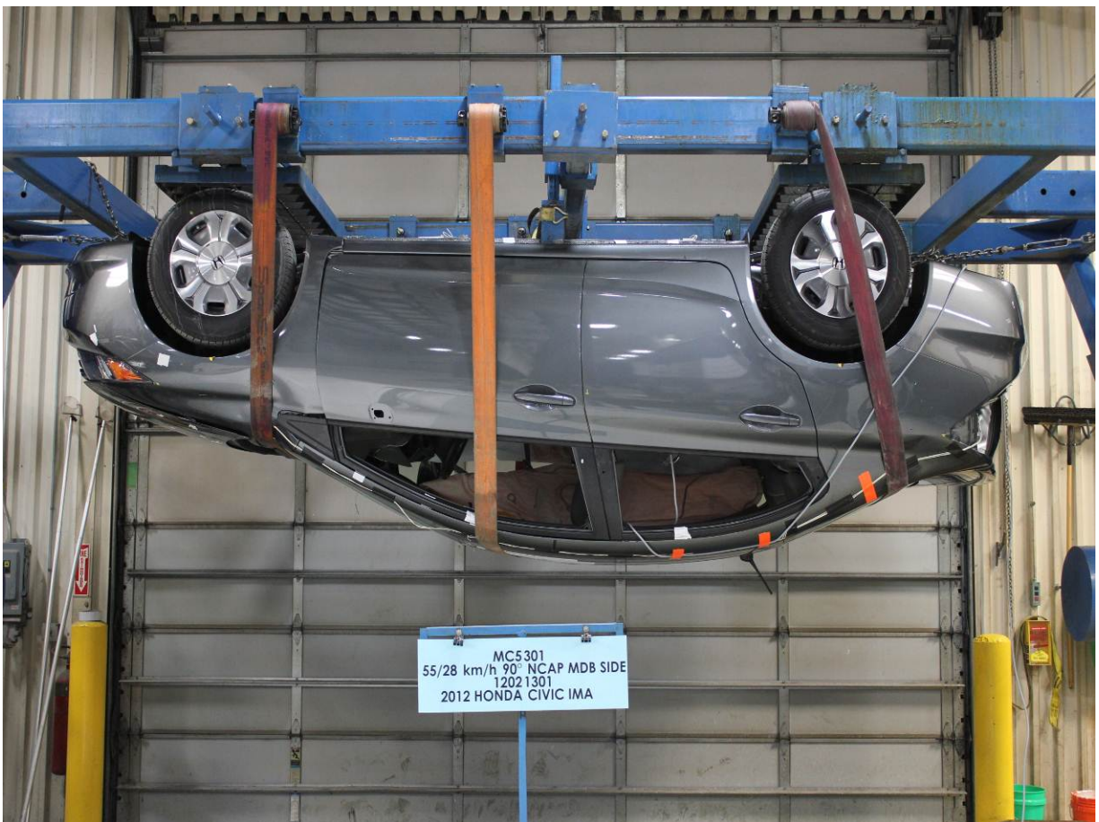
FMVSS No. 301 Static Rollover 180 Degrees
