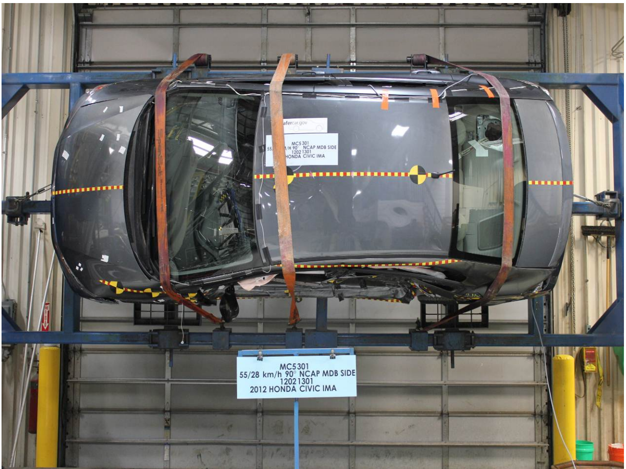
FMVSS No. 301 Static Rollover 90 Degrees
