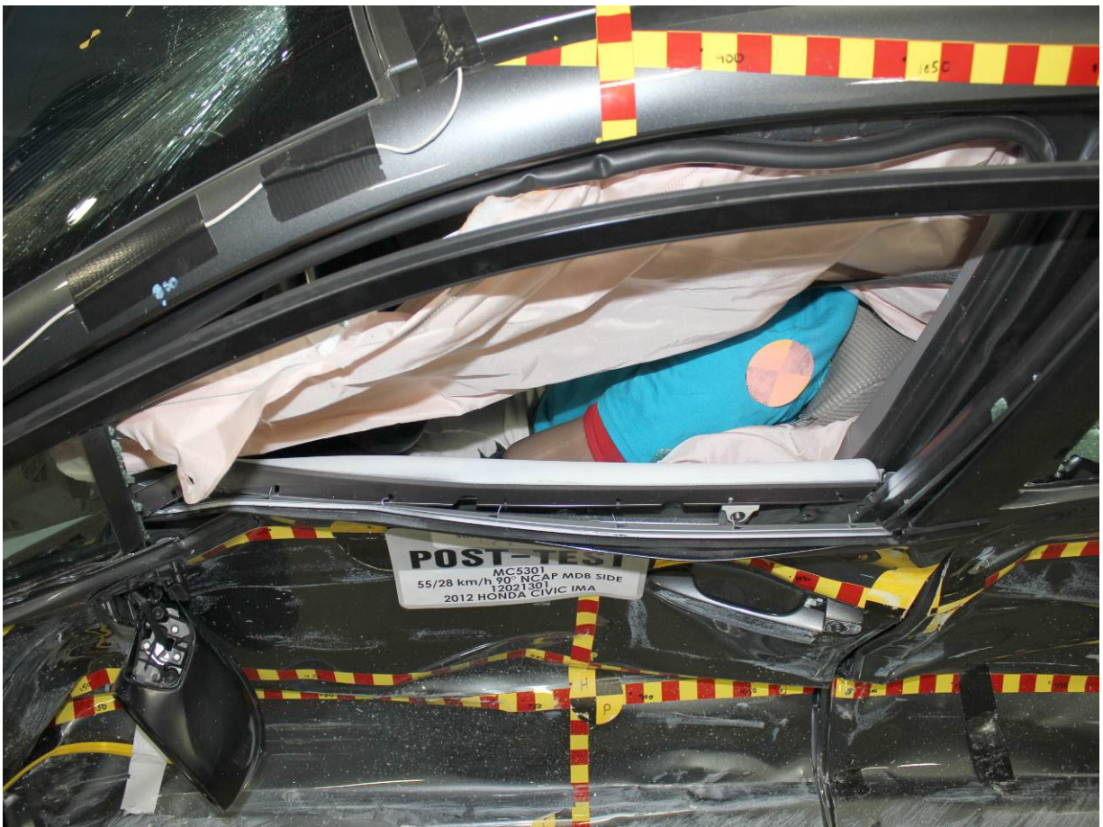
Post-Test Driver Dummy and Door Clearance View
