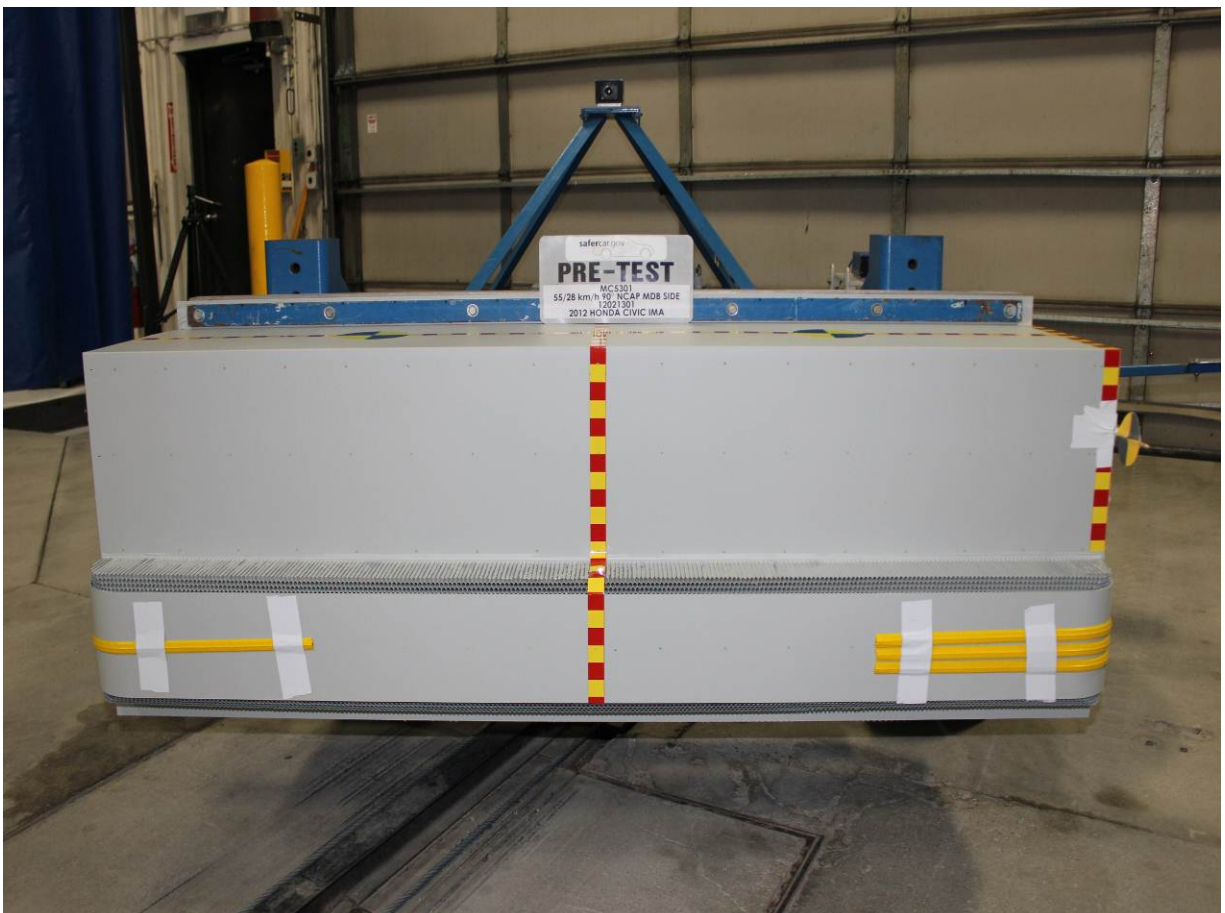
Pre-Test Front View of MDB Impactor Face
