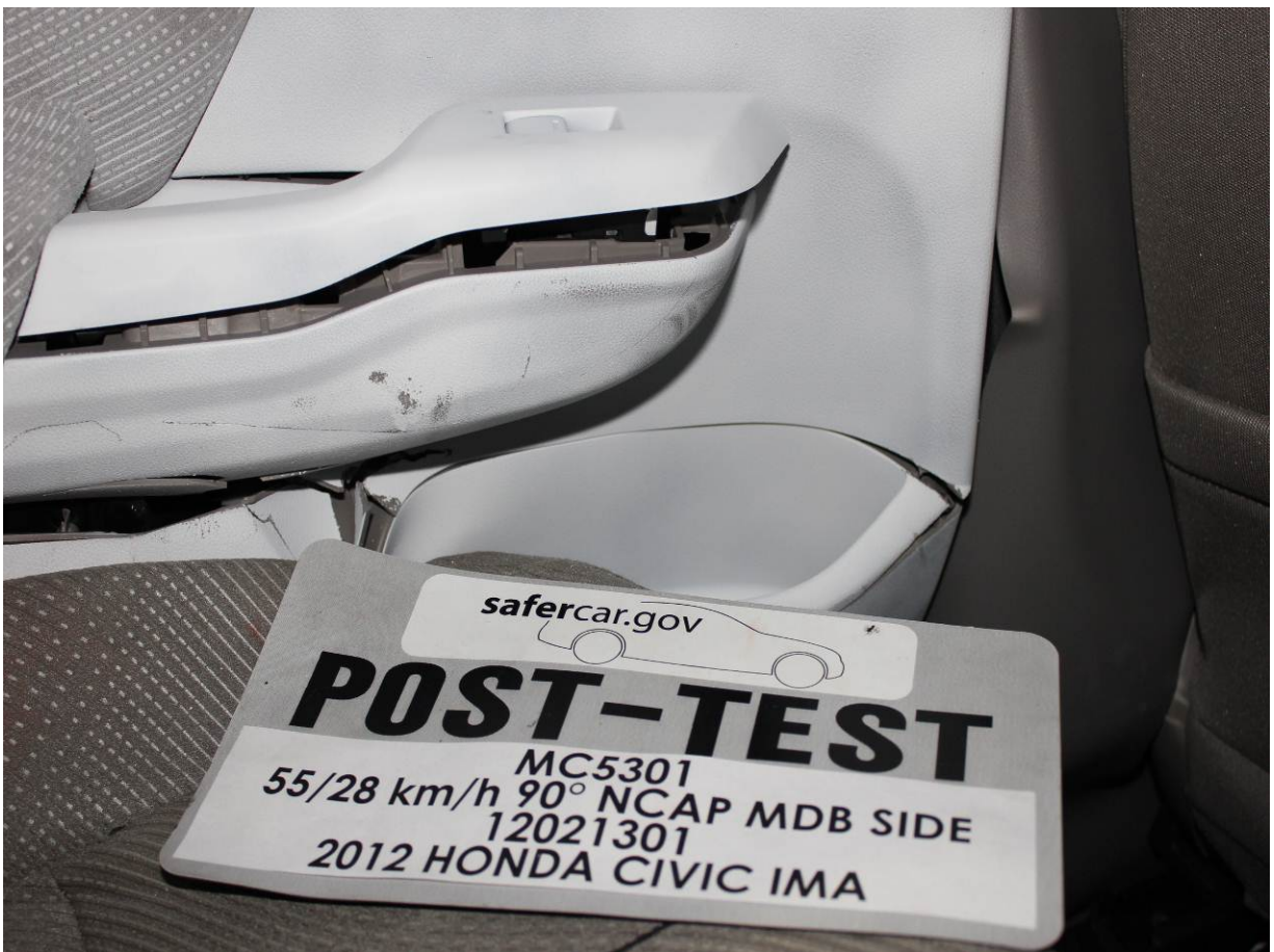
Post-Test Left Rear Passenger Dummy Knee Contact with Vehicle Interior View
