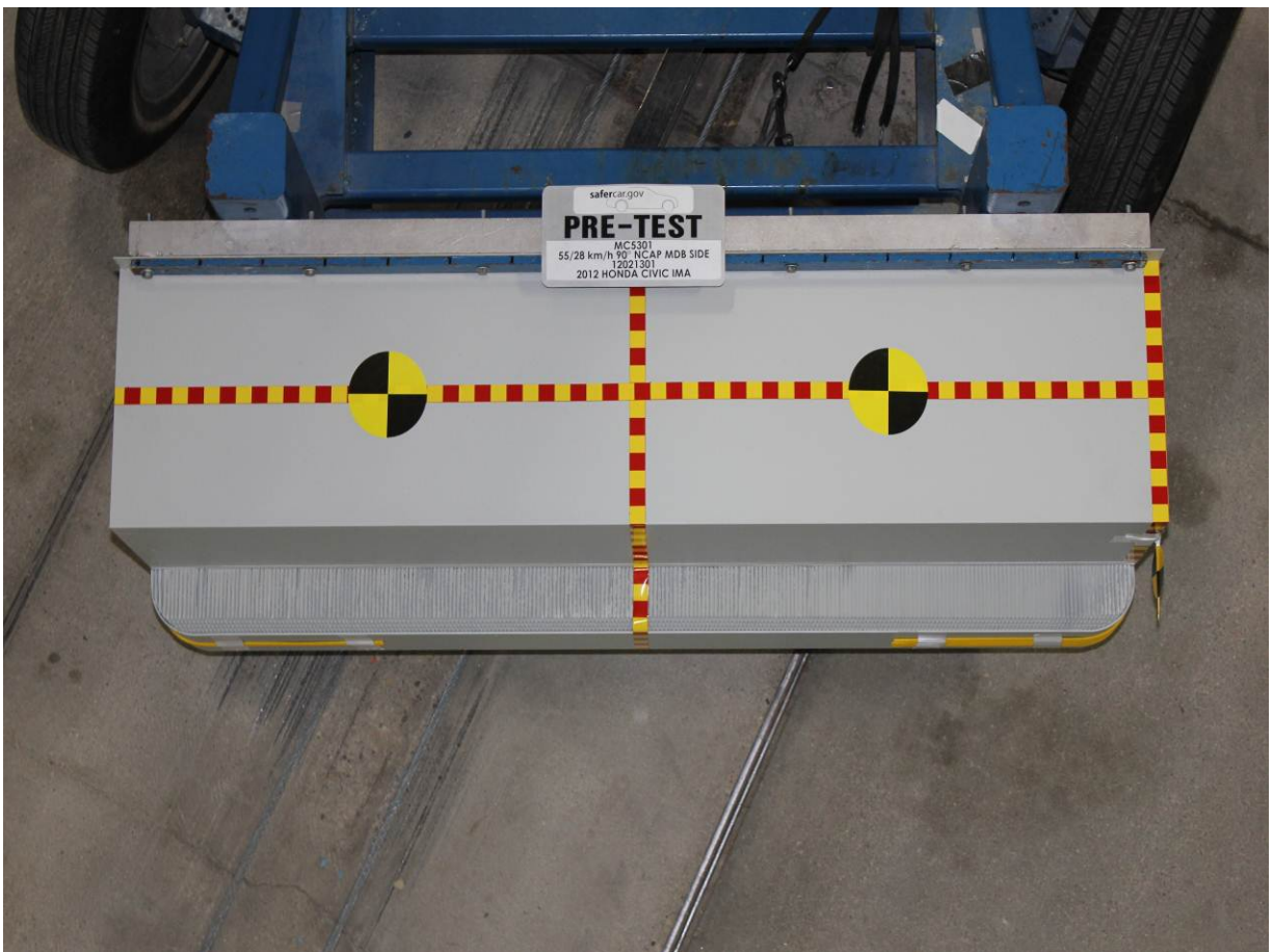
Pre-Test Top View of MDB Impactor Face
