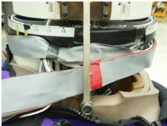
Figure 1. Front of dummy showing chest band location
