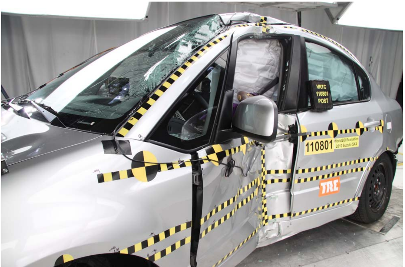
Figure A-6 Post-Test Left Front Tight View
