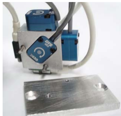
Figure 3. Aluminum block with 3 linear accelerometers and 3 angular rate sensors installed. Block was mounted to plate shown and secured to dummy front spine box at the top
