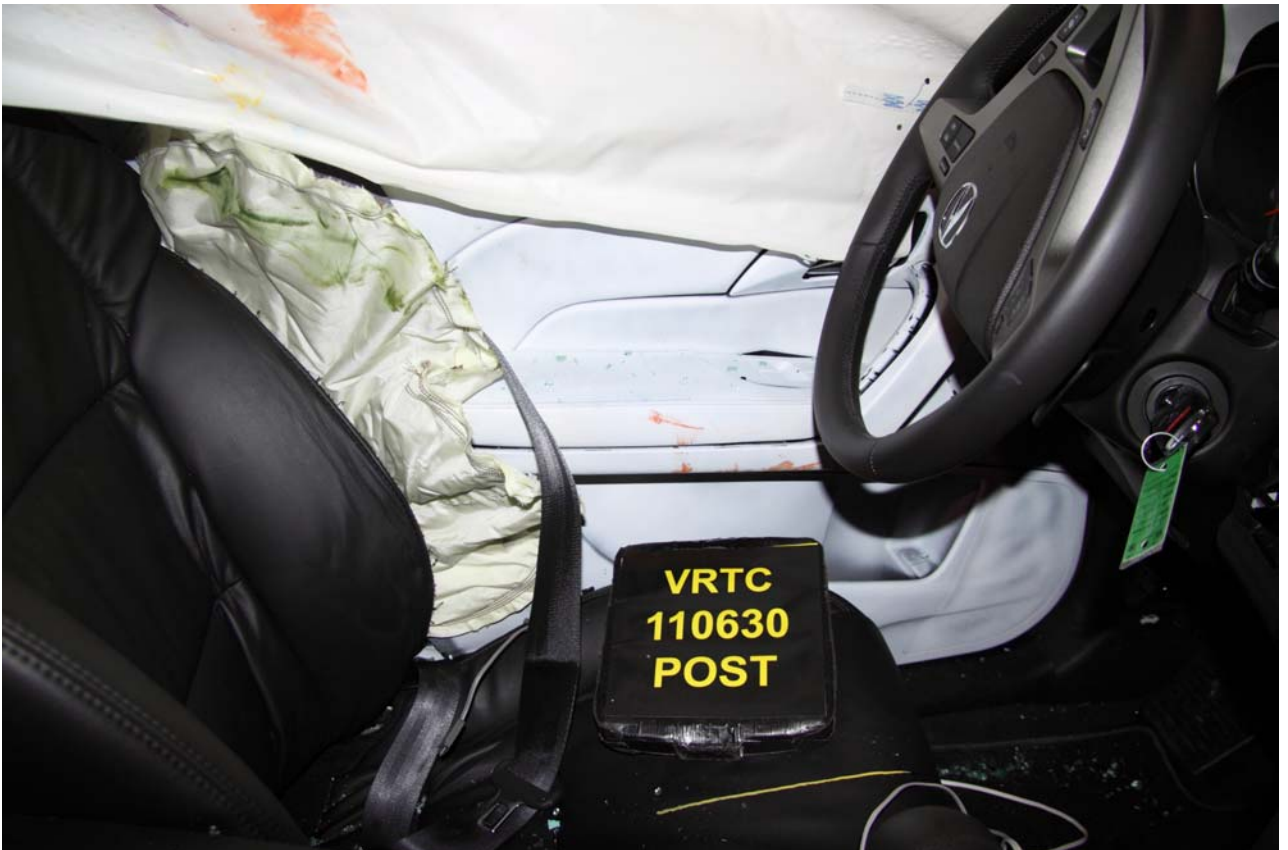
Figure A-42 Post-Test Driver Door Panel View
