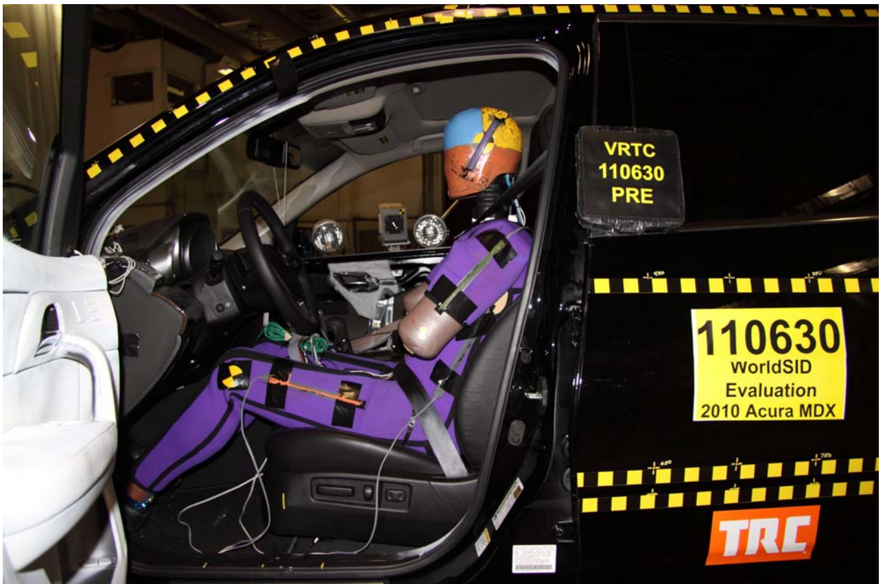
Figure A-34 Pre-Test Driver Dummy - View 3
