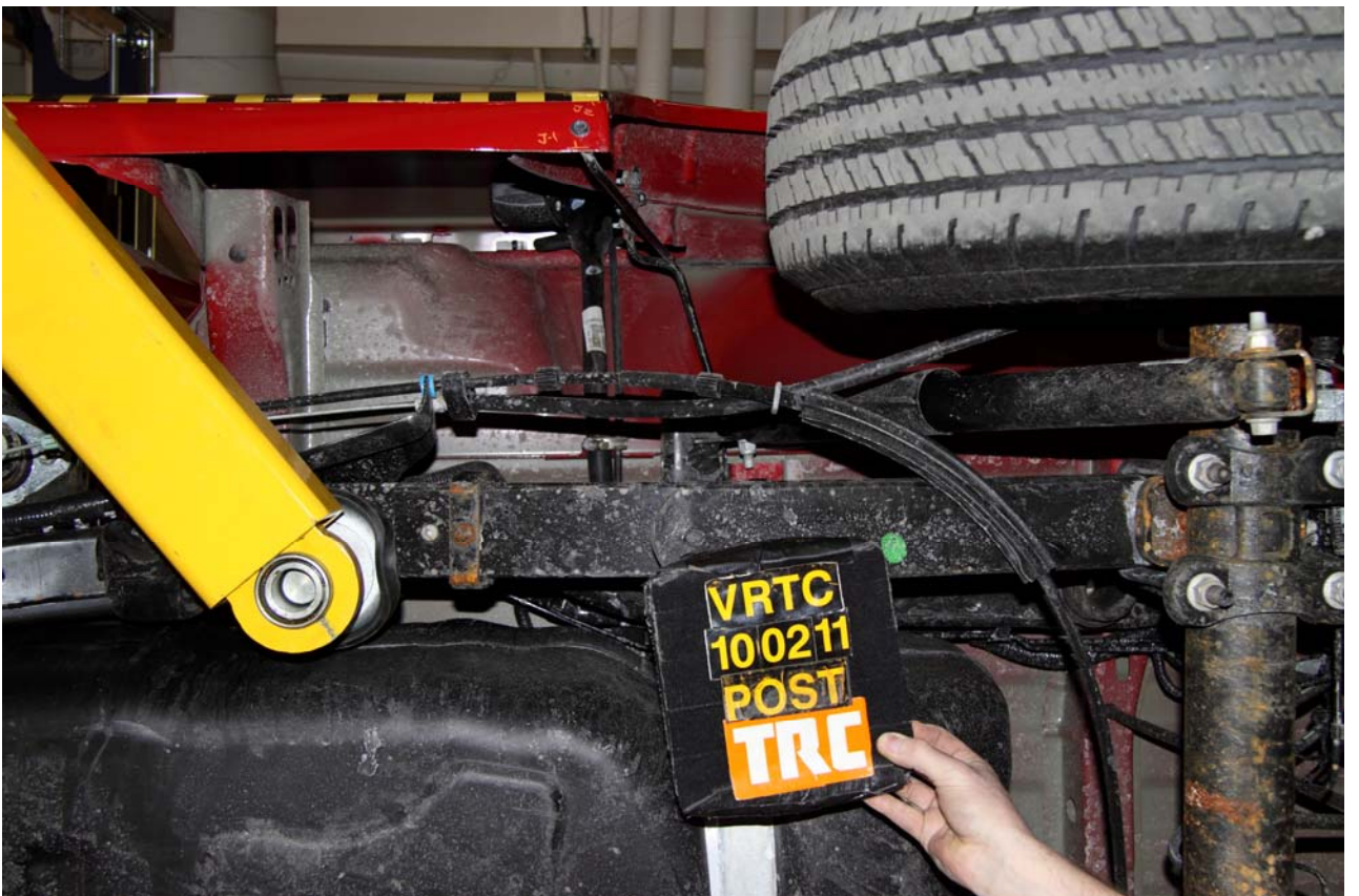
Figure A-36 Post-Test Fuel Filler Neck View
