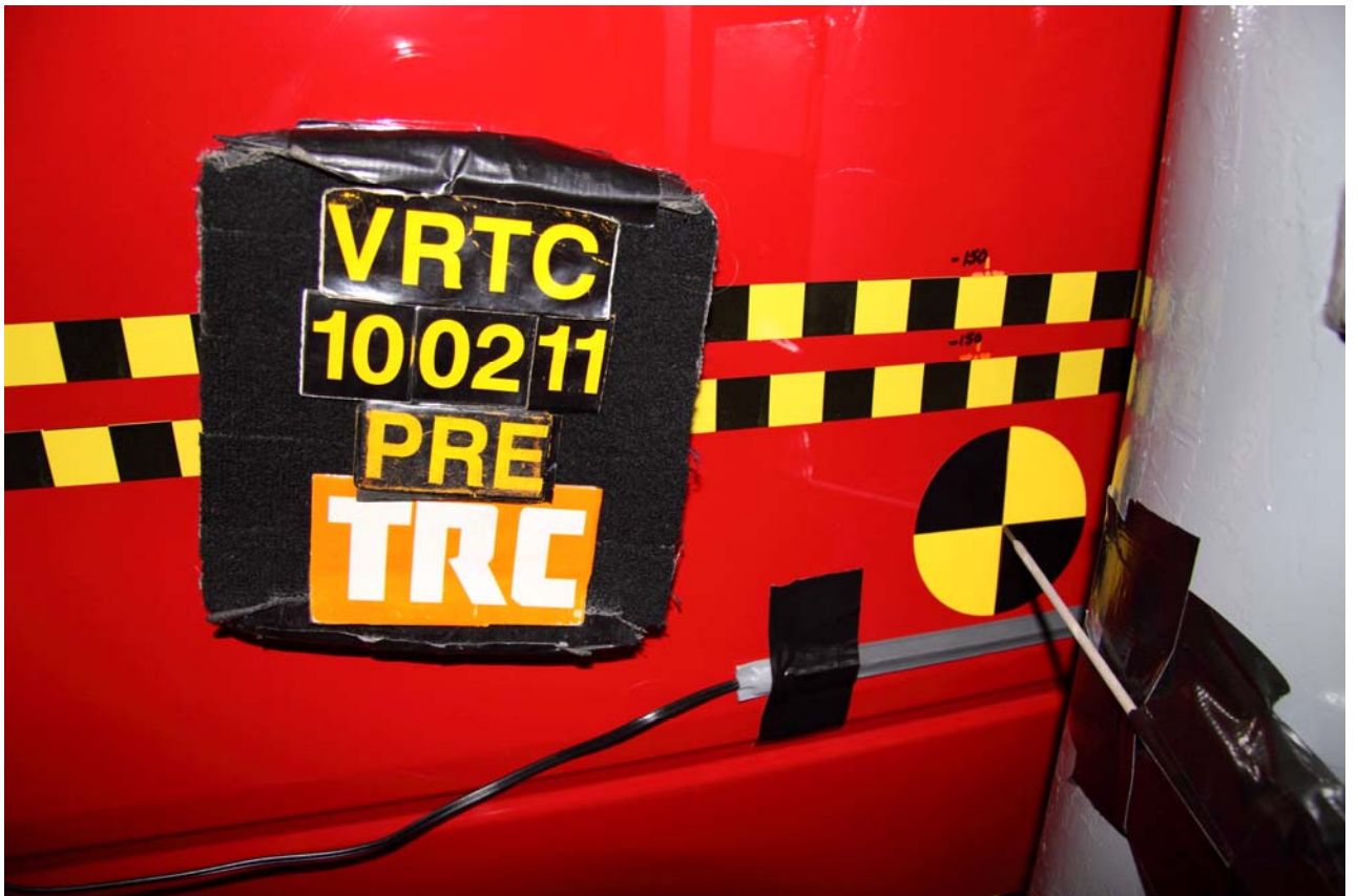
Figure A-19 Pre-Test Primary Impact Point View
