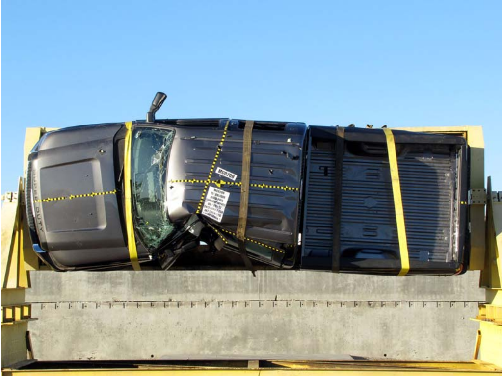
FIGURE 63. FMVSS No. 301-305 Rollover 90 Degrees
