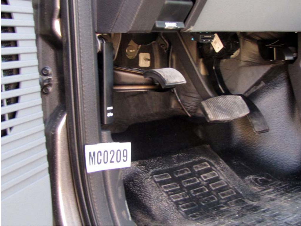
FIGURE 35. View of Disengaged Parking Brake
