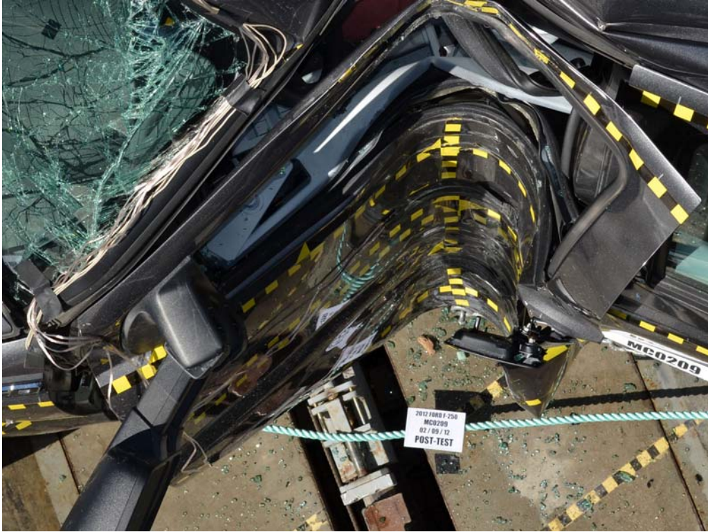
FIGURE 41. Post-Test Driver Dummy and Door Clearance
