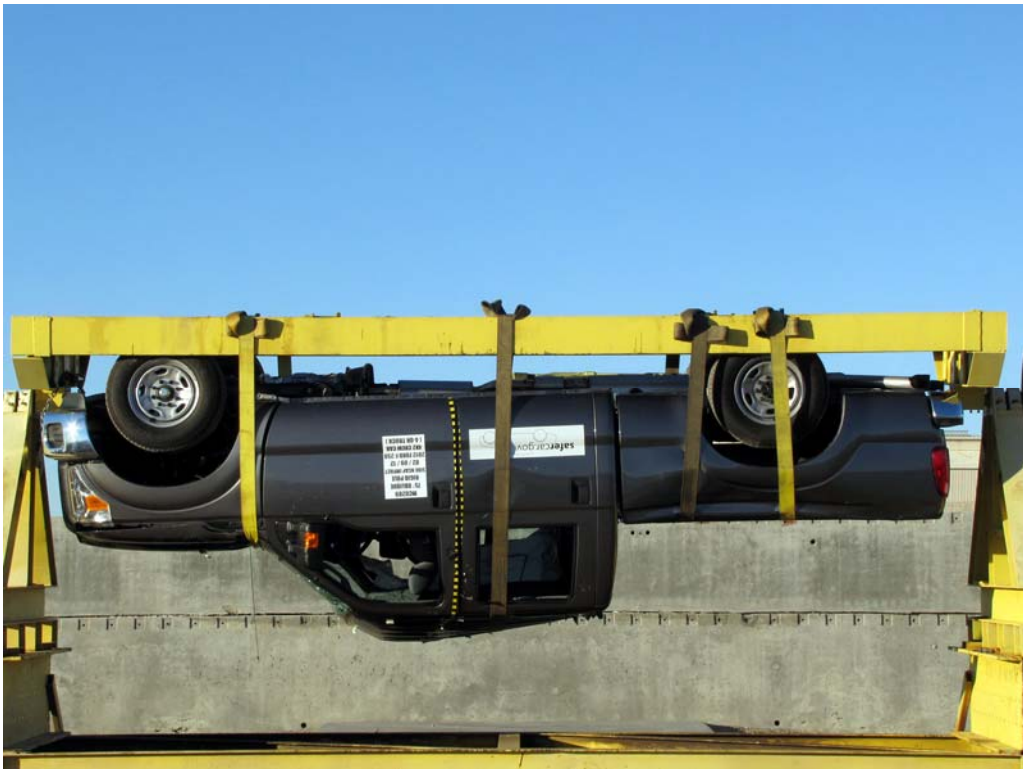
FIGURE 64. FMVSS No. 301-305 Rollover 180 Degrees
