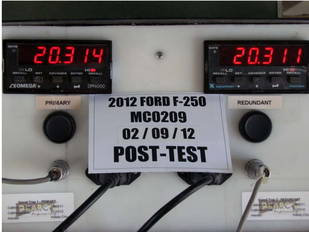
FIGURE 61. Post-Test Primary and Redundant Speed Trap Read-Out
