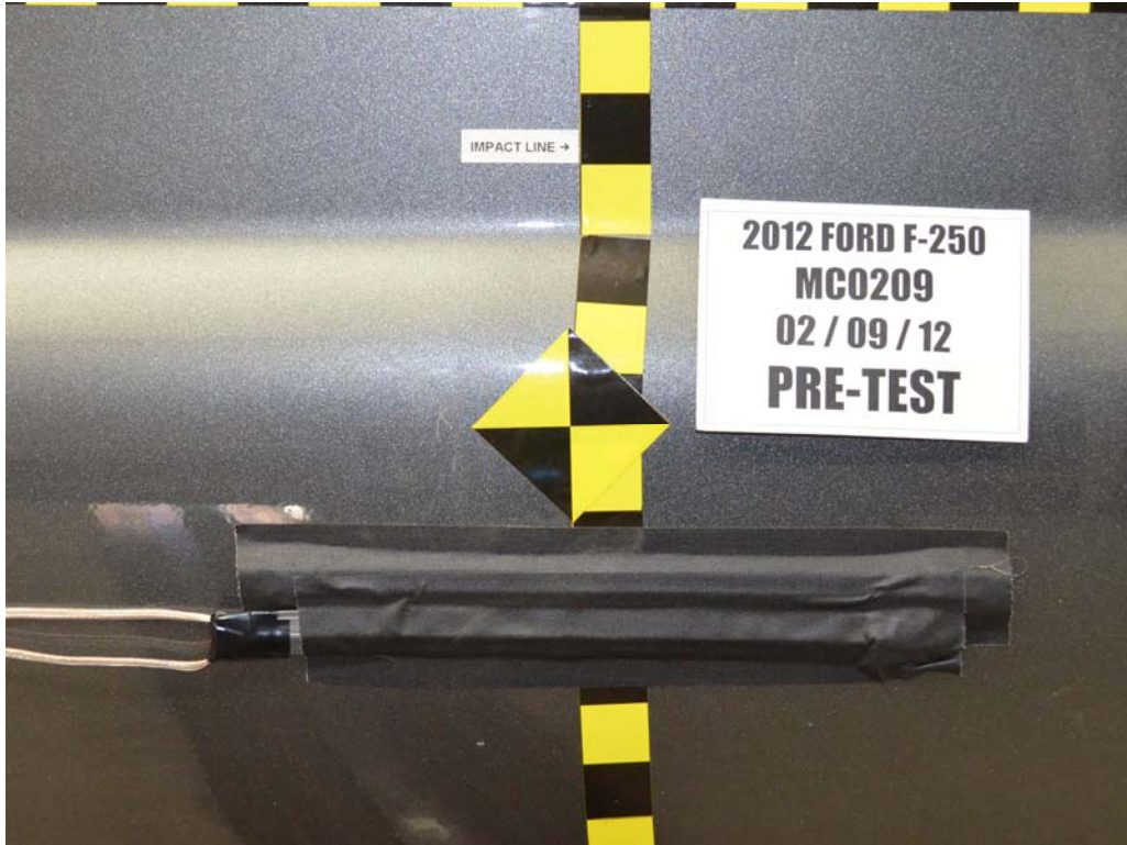
FIGURE 19. Pre-Test Close-Up View of Impact Point Target
