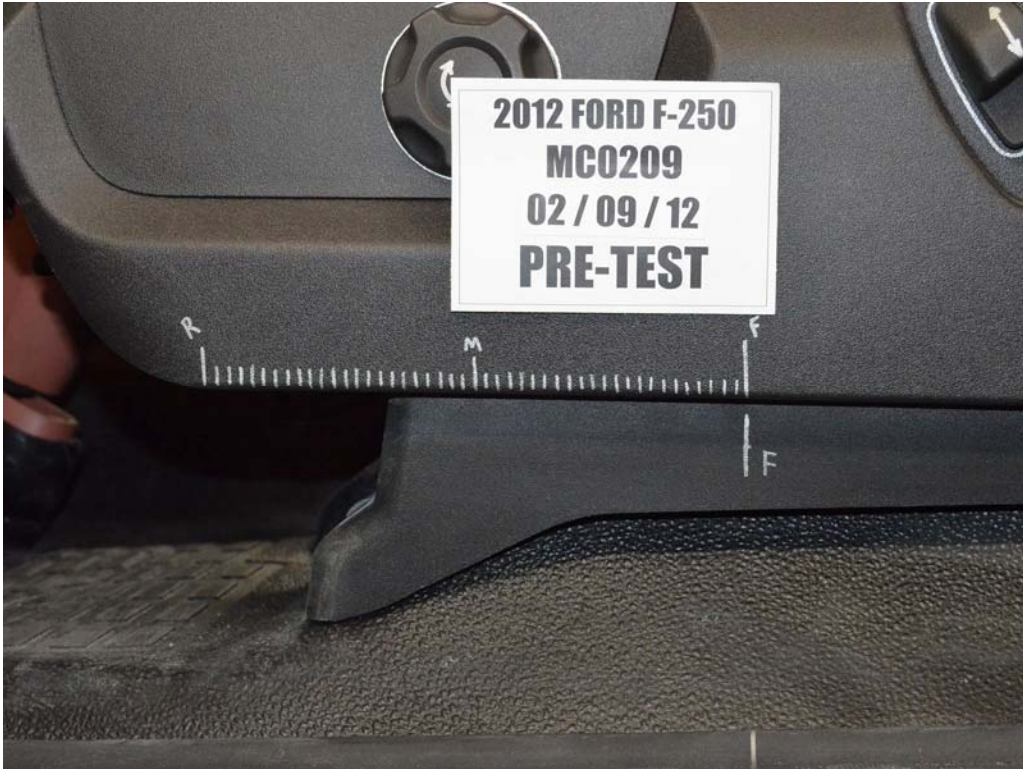
FIGURE 37. Pre-Test Close-Up Left Side View of Driver Seat Track
