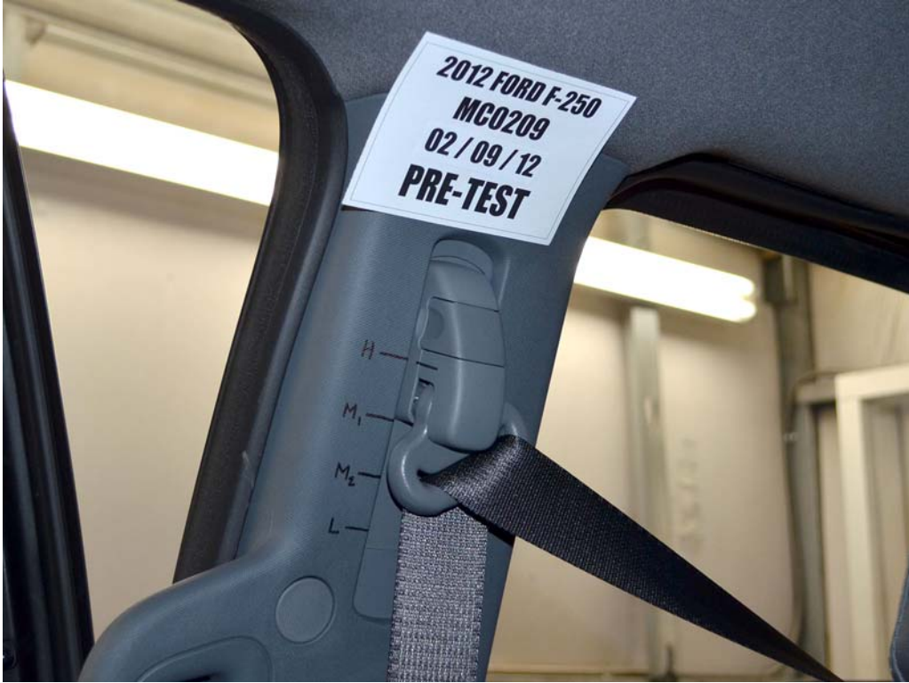
FIGURE 33. Pre-Test View of Belt Anchorage for Dummy
