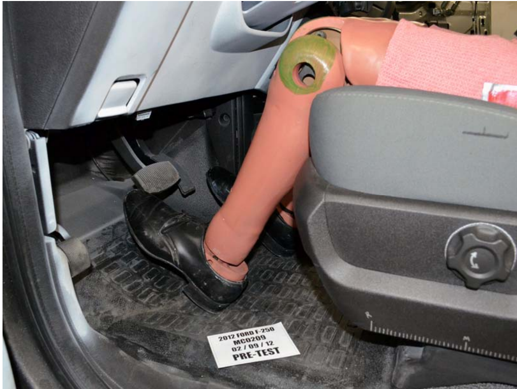
FIGURE 32. Pre-Test Placement of Dummy's Feet
