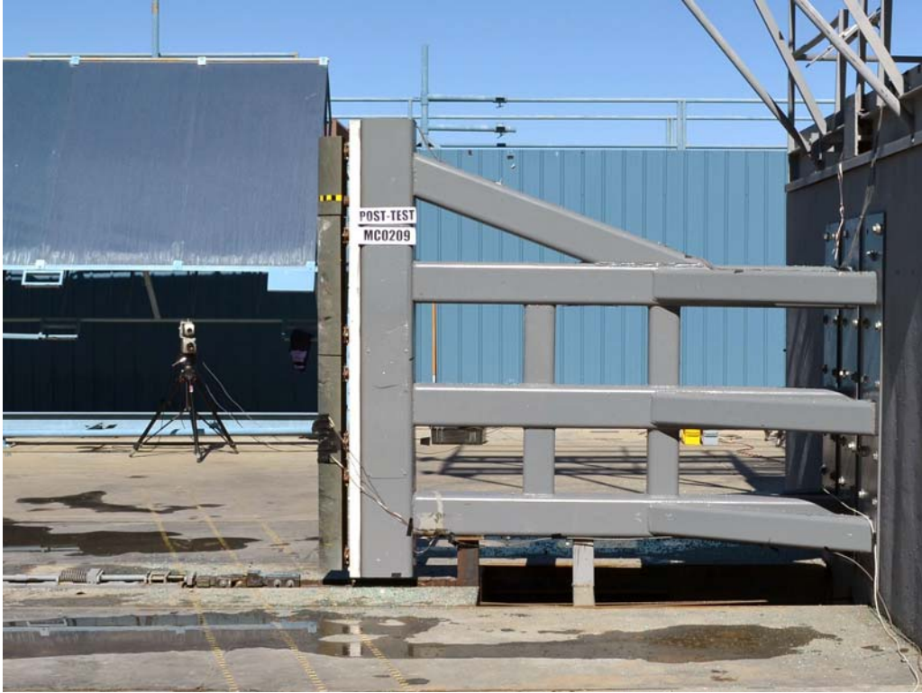
FIGURE 59. Post-Test Pole Barrier Side View
