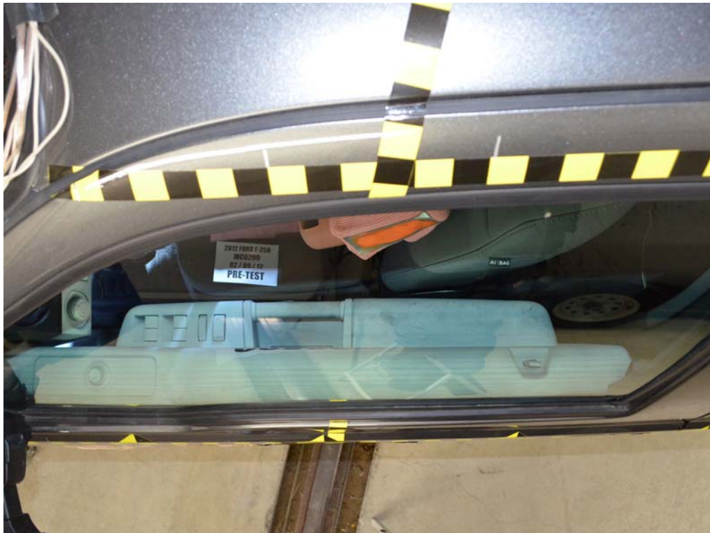
FIGURE 40. Pre-Test Driver Dummy and Door Clearance
