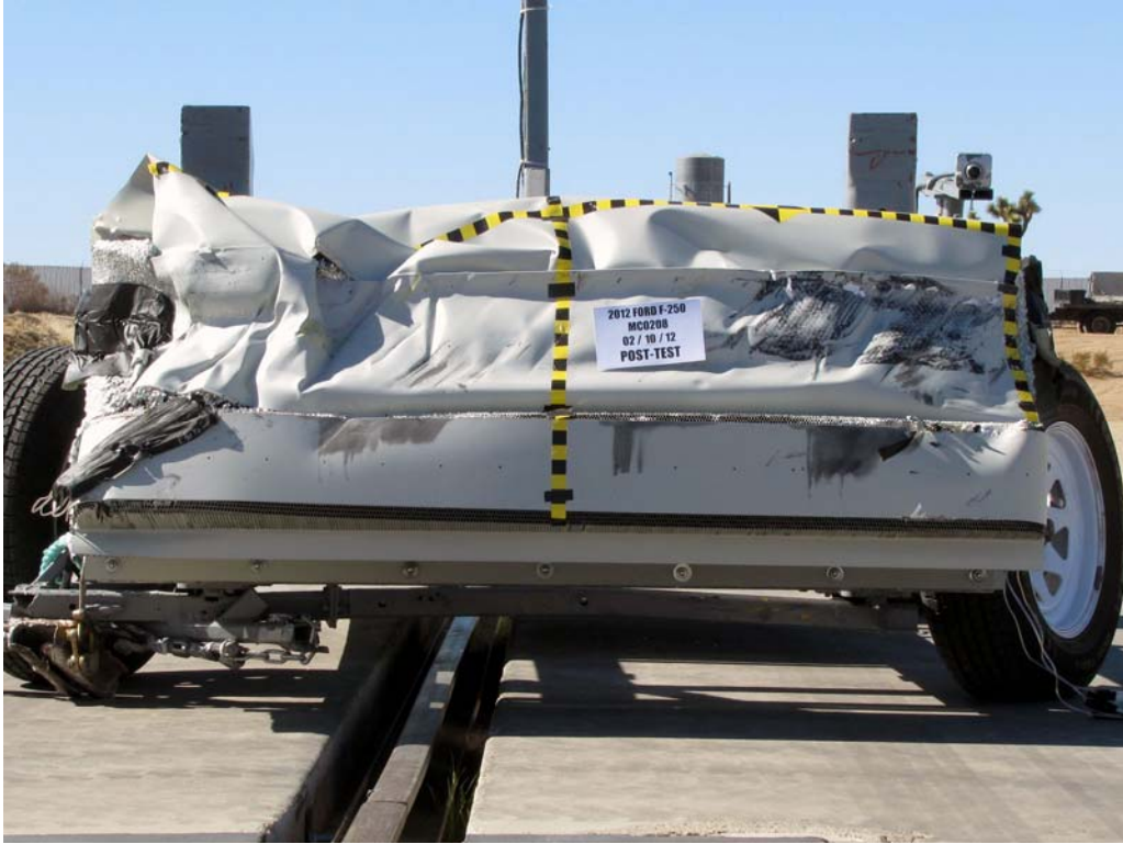
FIGURE 83. Post-Test Front View of MDB Impactor Face
