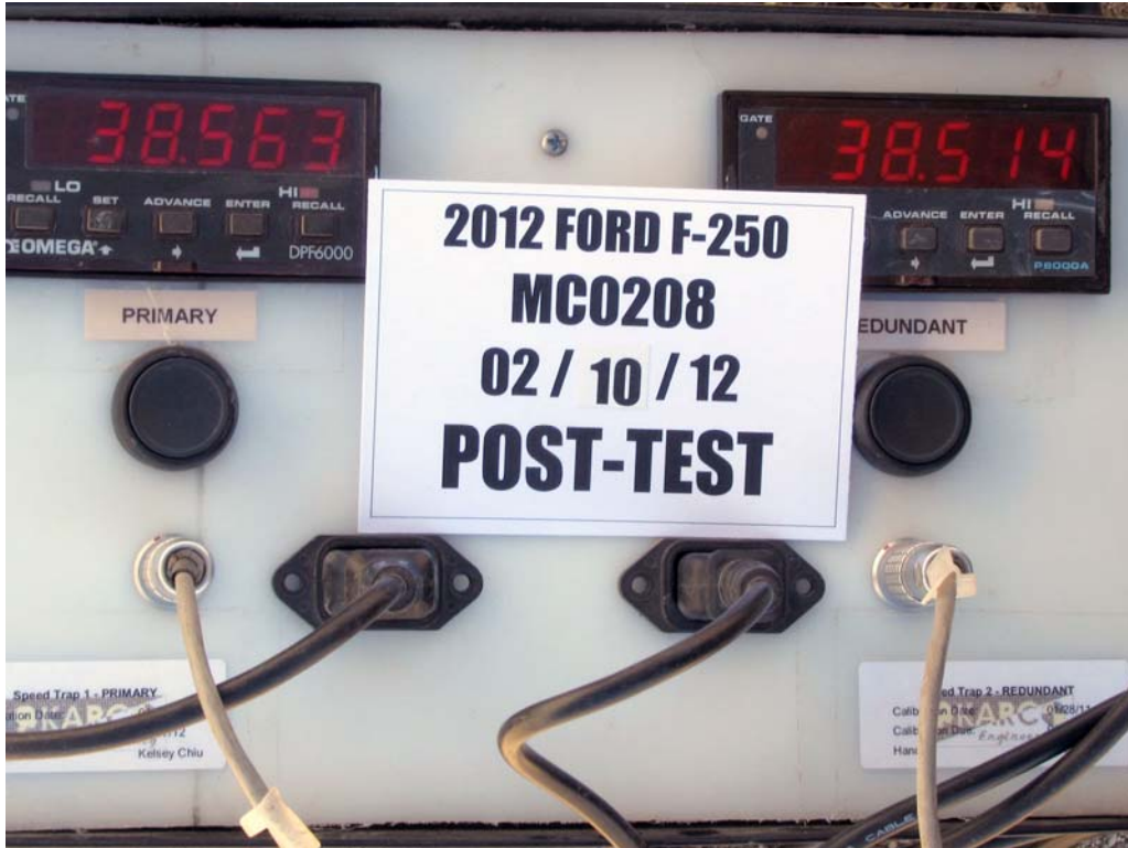
FIGURE 93. Post-Test Primary and Redundant Speed Trap Read-Out
