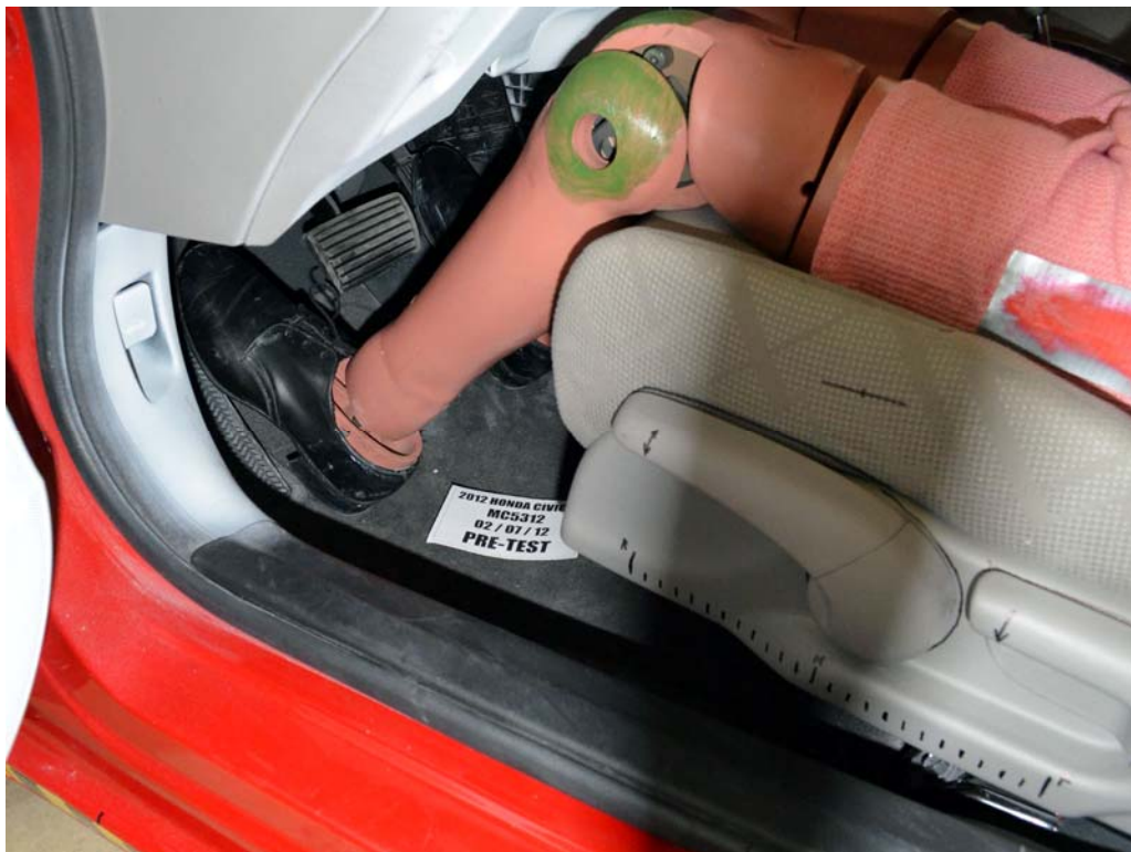
FIGURE 32. Pre-Test Placement of Dummy's Feet
