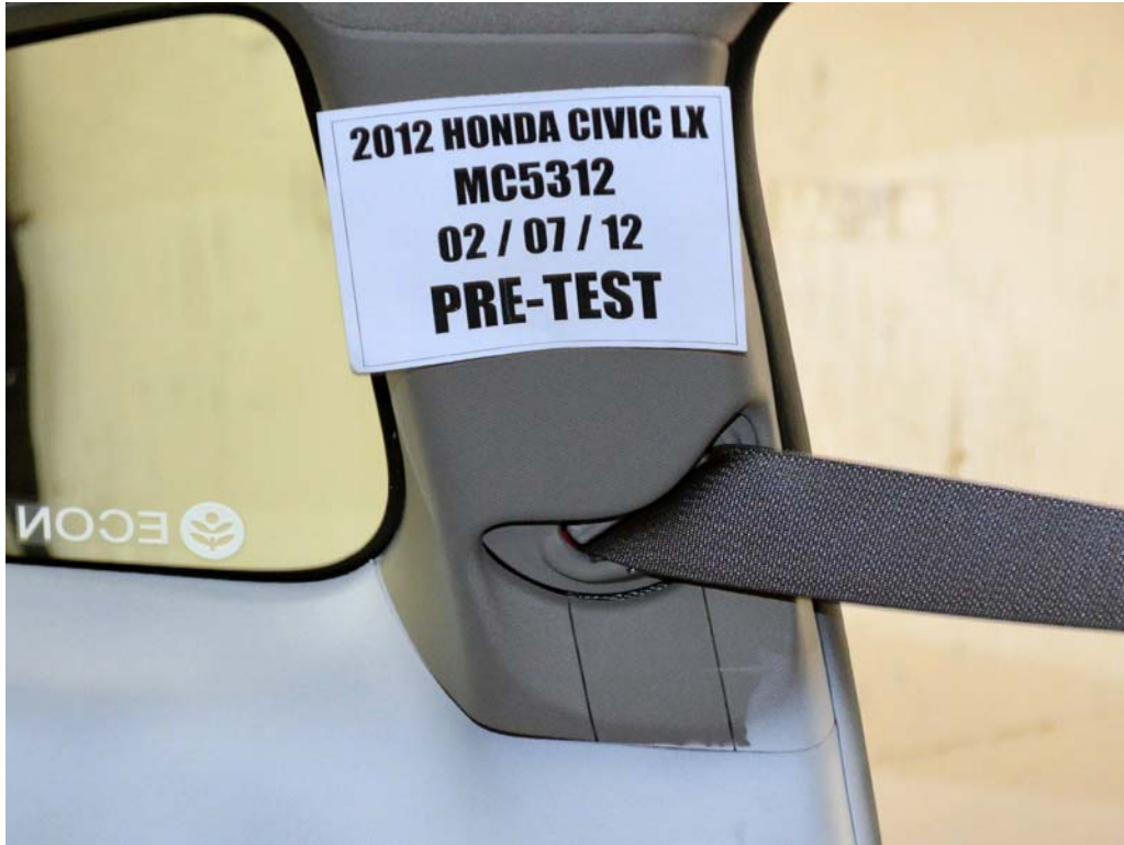
FIGURE 33. Pre-Test View of Belt Anchorage for Dummy
