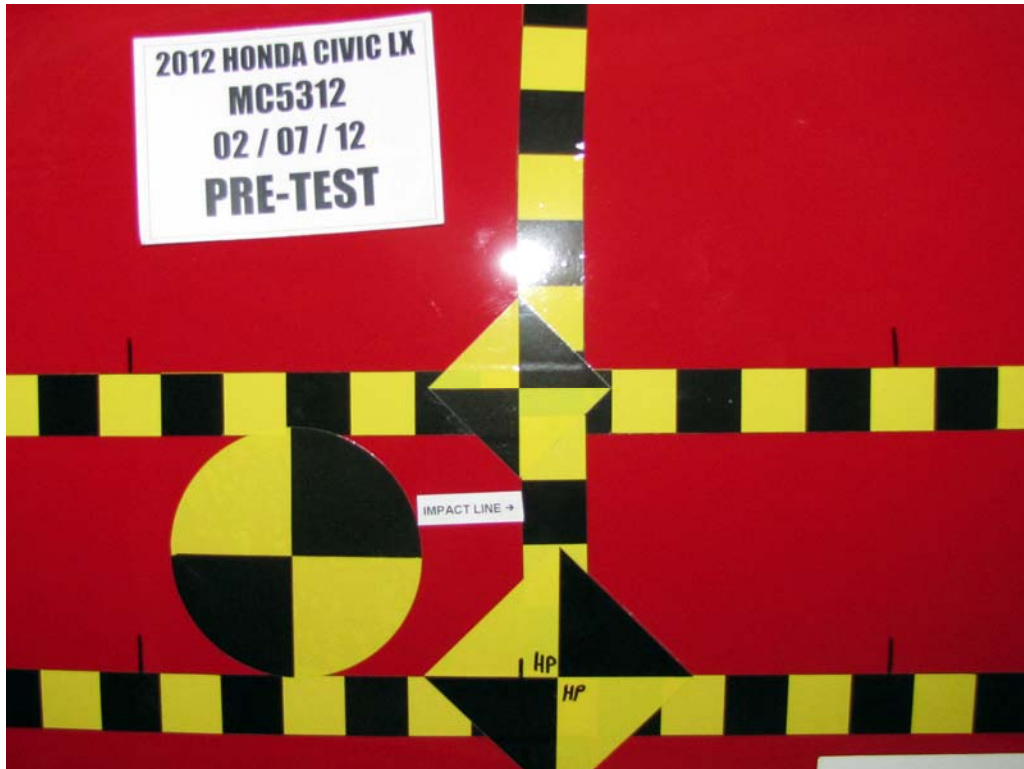
FIGURE 19. Pre-Test Close-Up View of Impact Point Target
