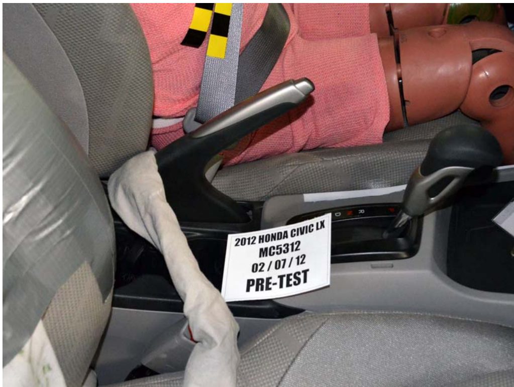
FIGURE 36. Pre-Test View of Parking Brake
