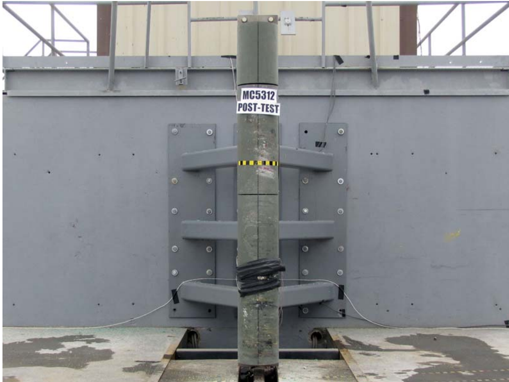
FIGURE 57. Post-Test Pole Barrier Front View
