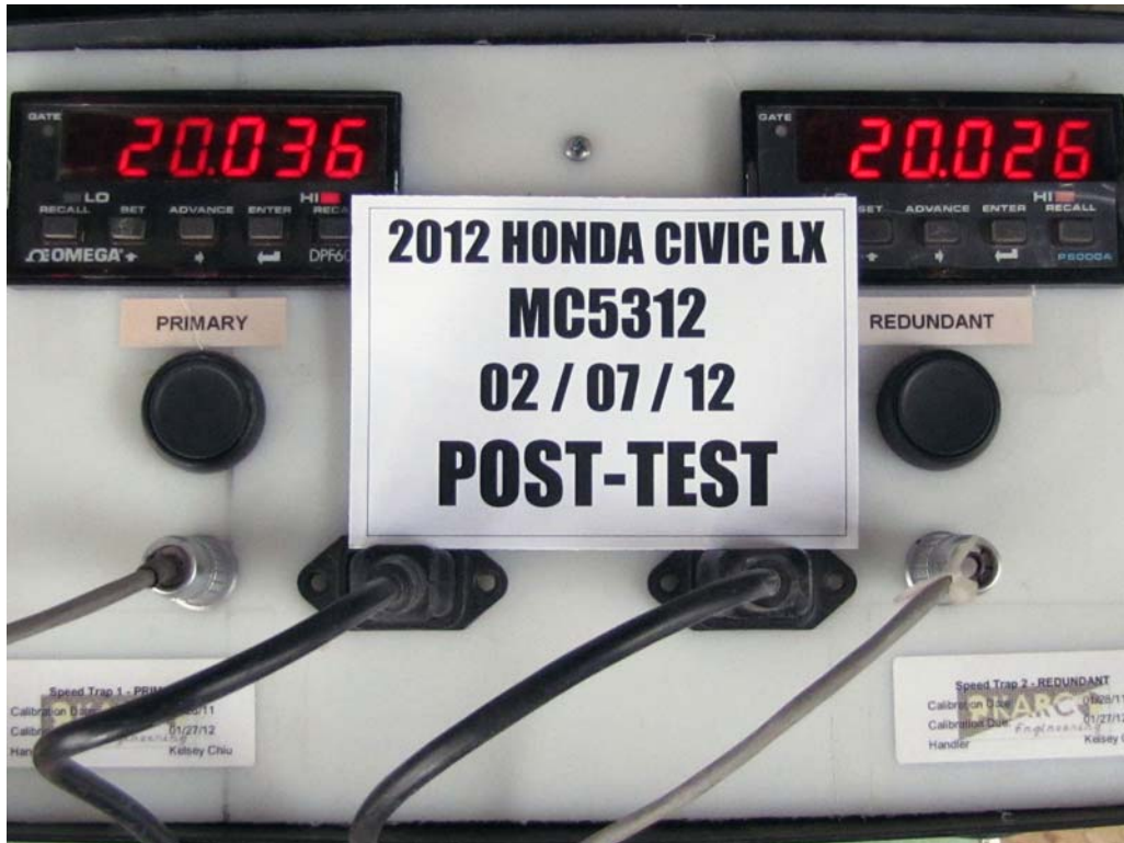
FIGURE 61. Post-Test Primary and Redundant Speed Trap Read-Out
