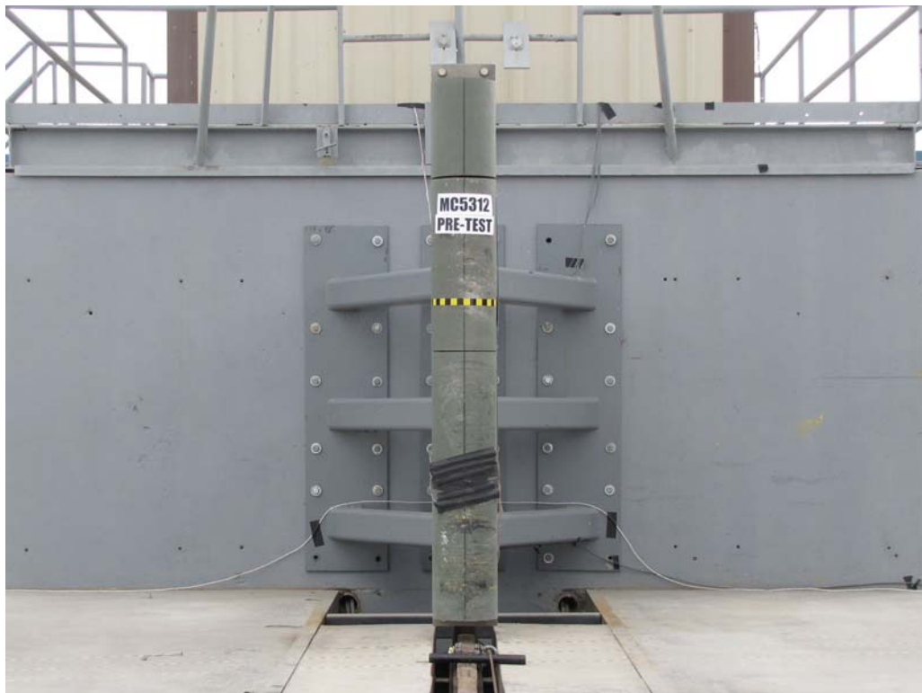
FIGURE 56. Pre-Test Pole Barrier Front View
