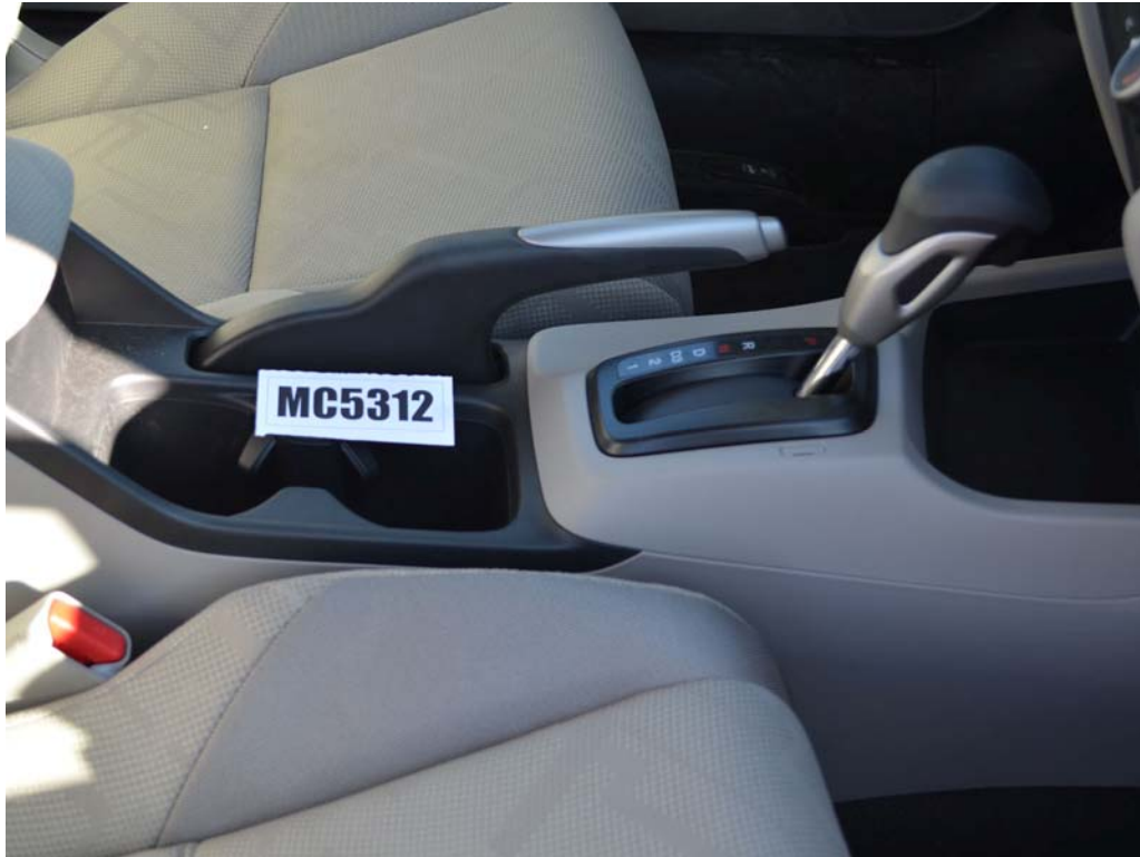
FIGURE 35. View of Disengaged Parking Brake
