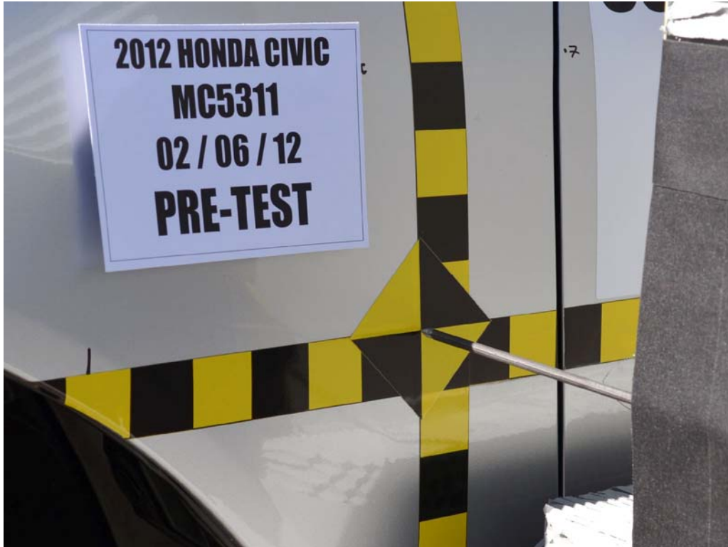
FIGURE 19. Pre-Test Close-Up View of Impact Point Target
