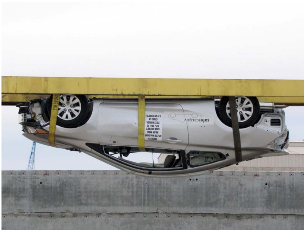
FIGURE 96. FMVSS No. 301 Static Rollover 180 Degrees
