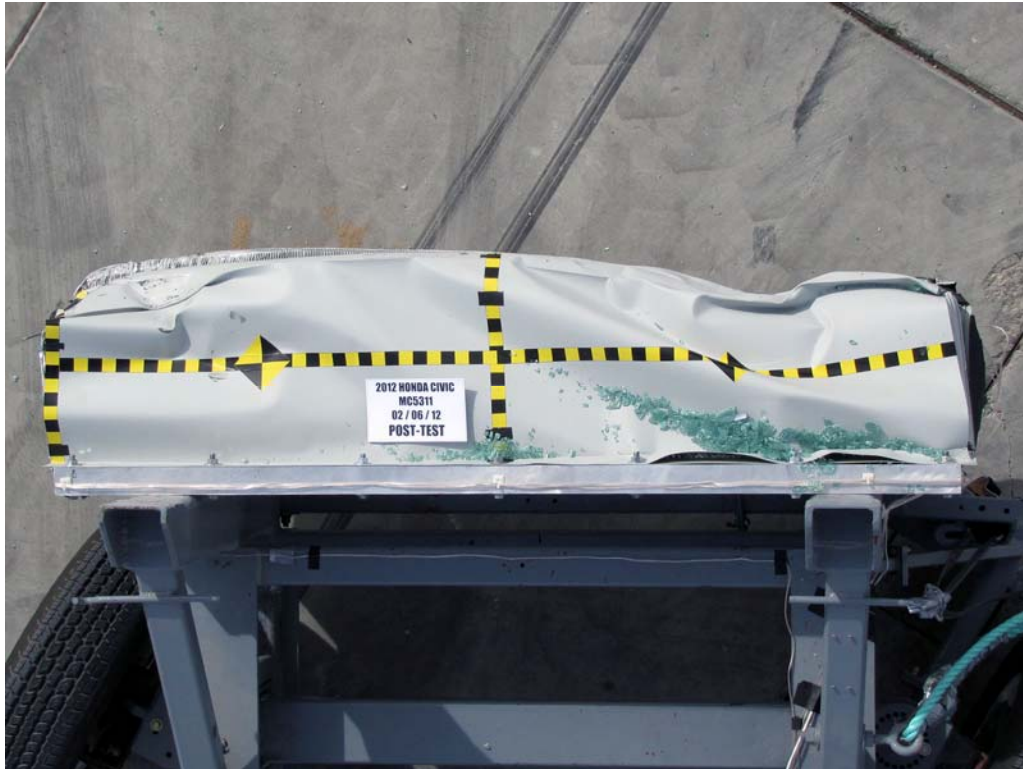
FIGURE 85. Post-Test Top View of MDB Impactor Face
