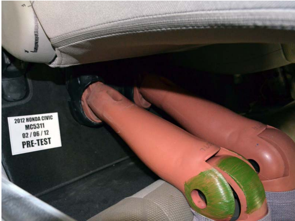
FIGURE 63. Pre-Test Placement of Rear Passenger Dummy's Feet
