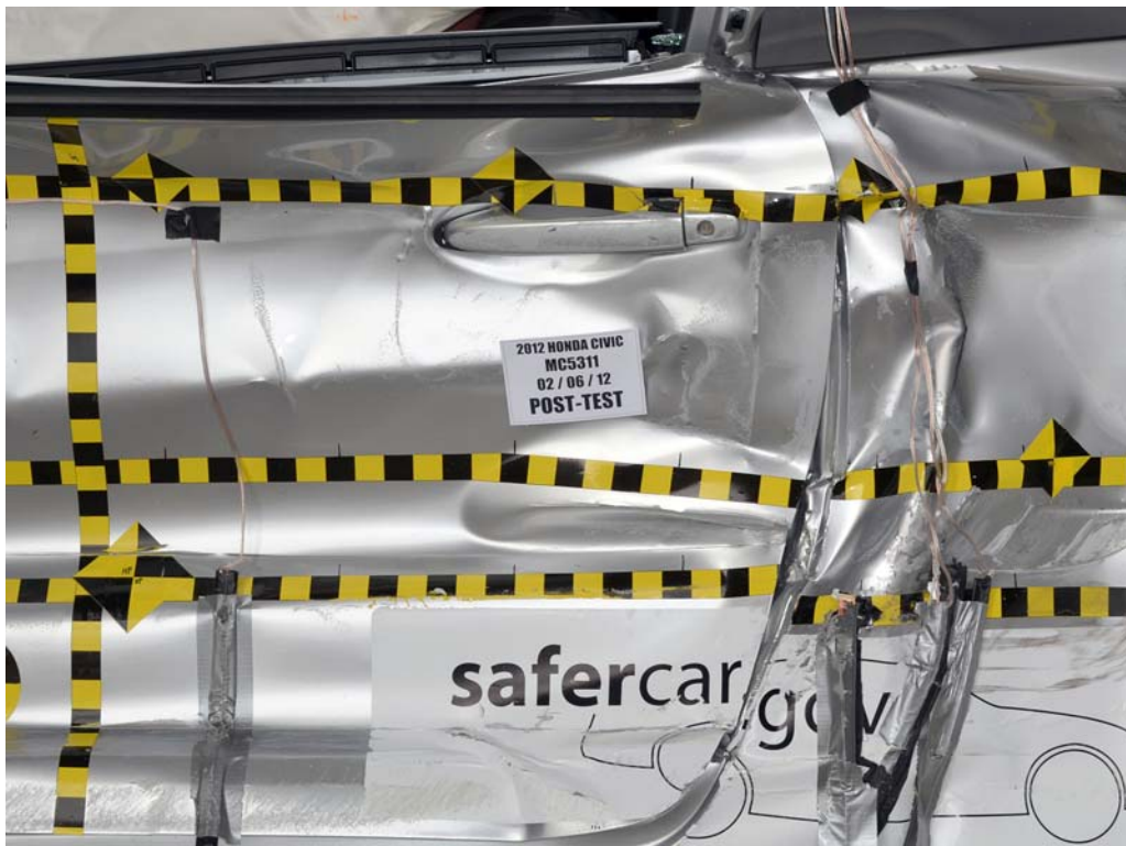
FIGURE 22. Post-Test Left Front Door Latch Close-Up
