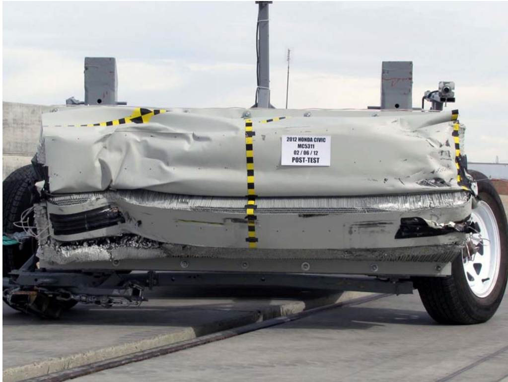
FIGURE 83. Post-Test Front View of MDB Impactor Face
