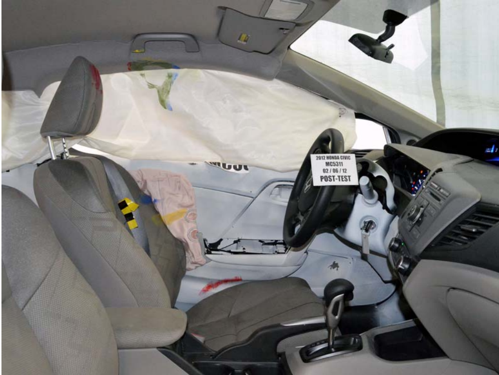
FIGURE 47. Post-Test Driver Inner Door Panel View
