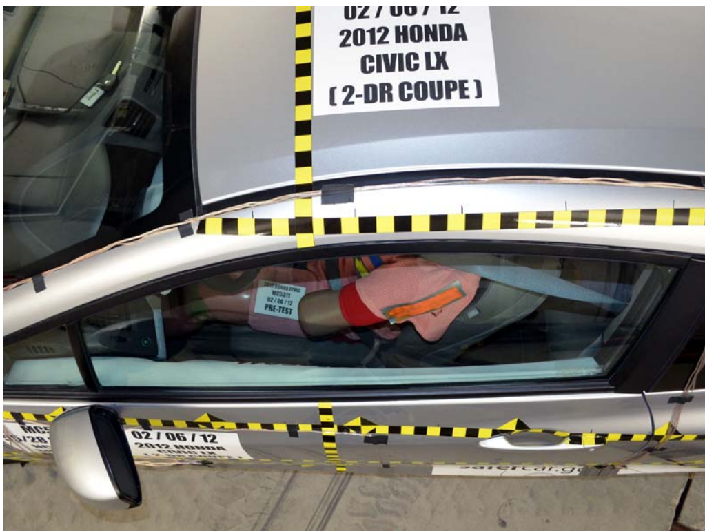
FIGURE 42. Pre-Test Driver Dummy and Door Clearance View
