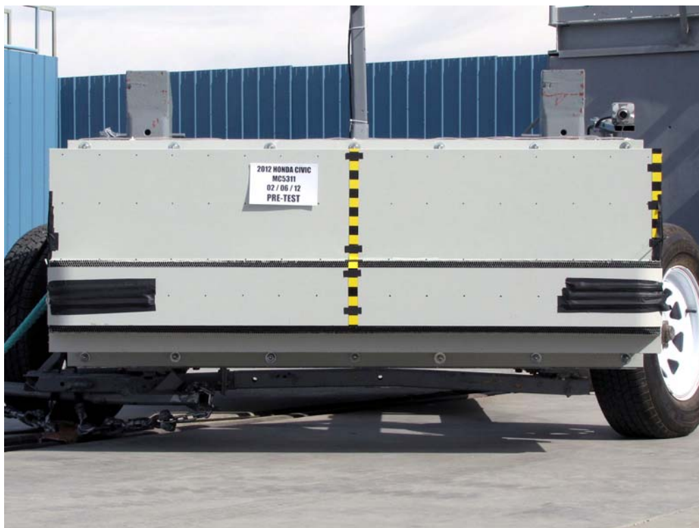
FIGURE 82. Pre-Test Front View of MDB Impactor Face
