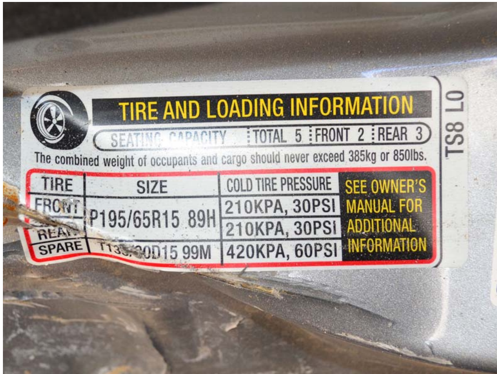
FIGURE 91. Close-Up View of Vehicle's Tire Information Placard
