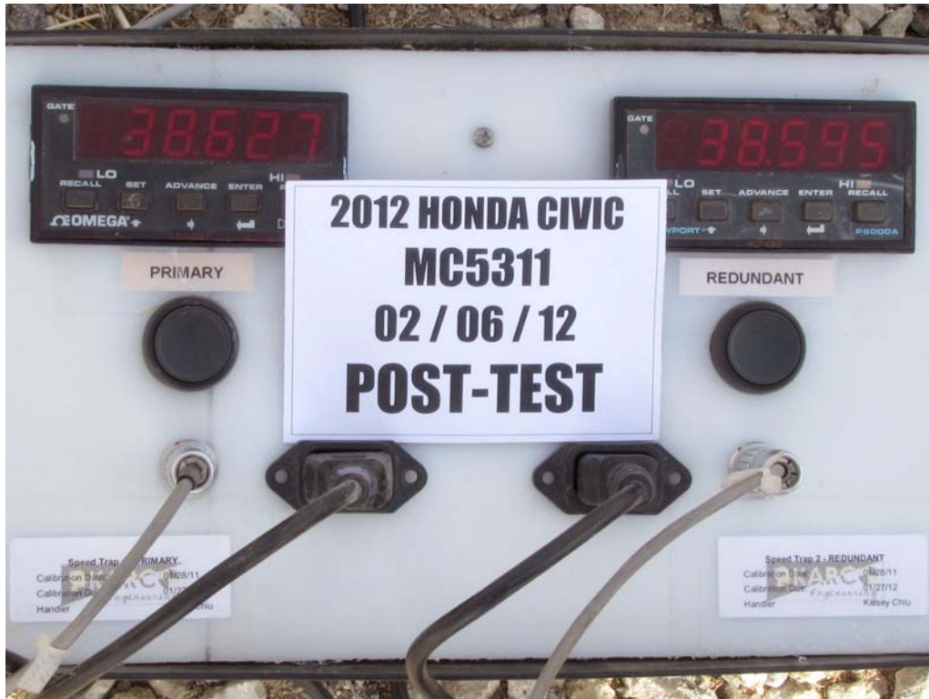
FIGURE 93. Post-Test Primary and Redundant Speed Trap Read-Out
