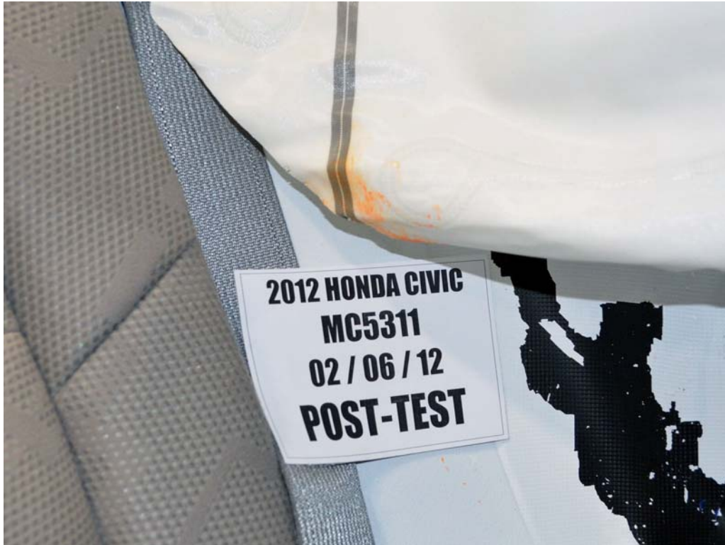
FIGURE 77. Post-Test Rear Passenger Dummy Close-Up Torso Contact with Side Airbag View
