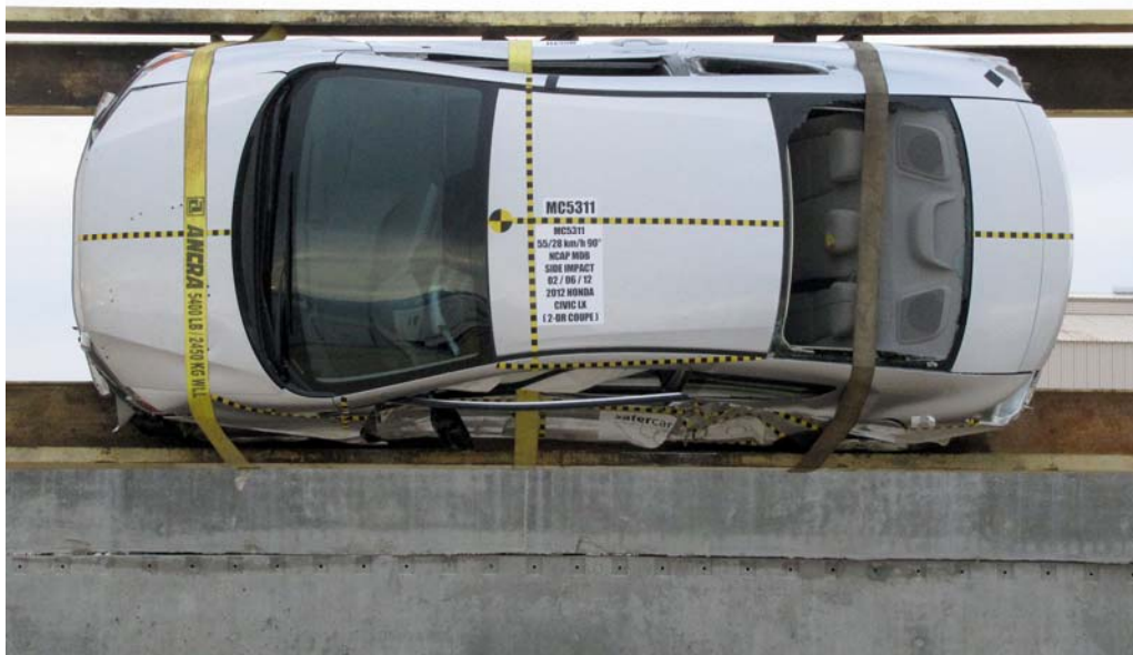
FIGURE 95. FMVSS No. 301 Static Rollover 90 Degrees
