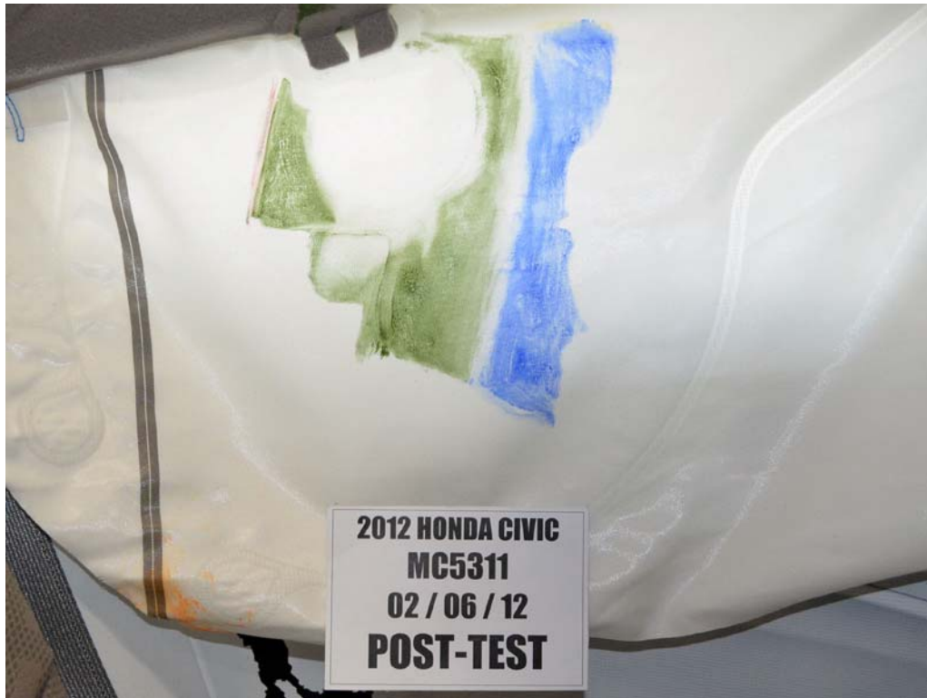
FIGURE 75. Post-Test Rear Passenger Dummy Close-Up Head Contact with Side Airbag View
