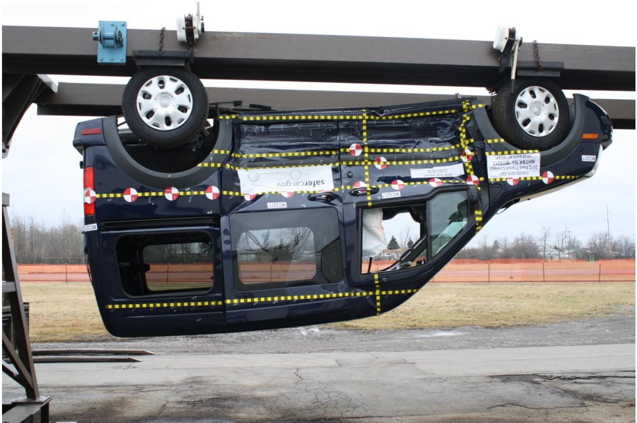
Figure A-96: FMVSS No. 301 Static Rollover 180 Degrees
