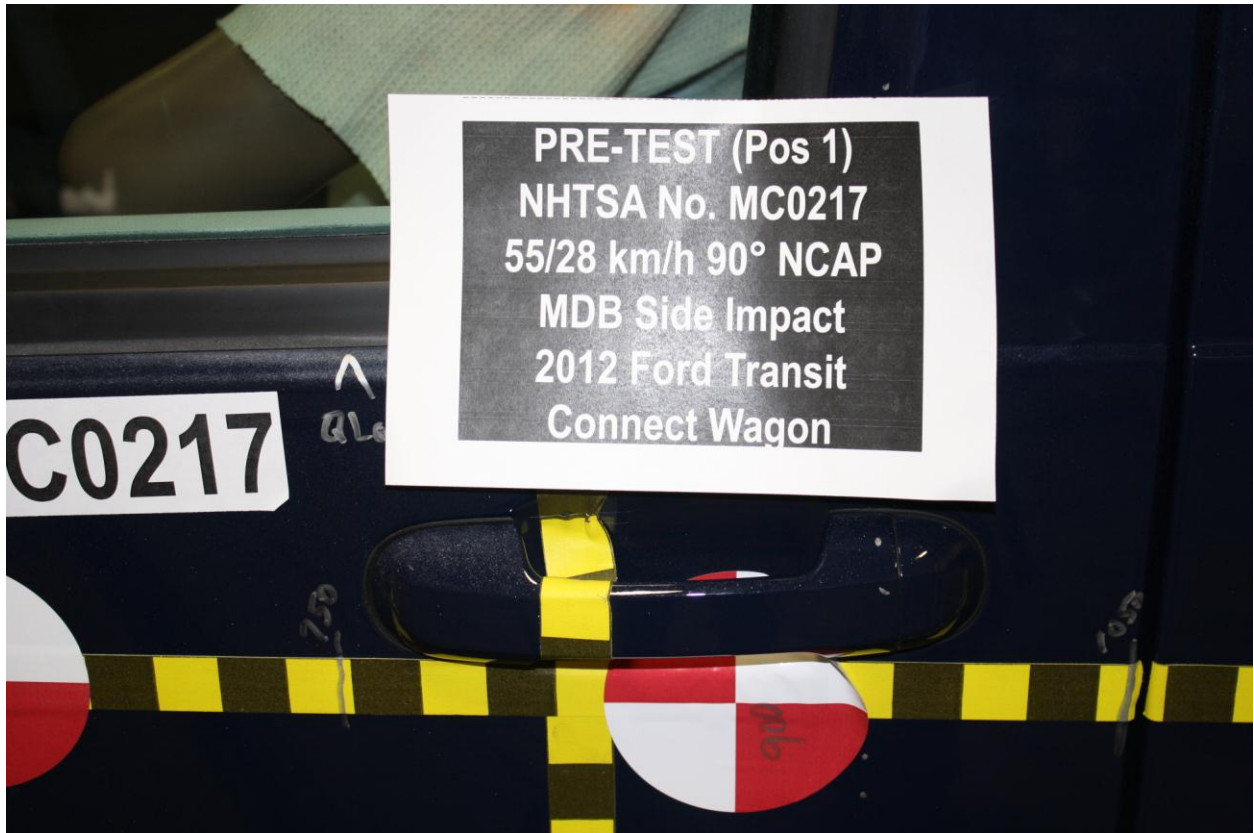
Figure A-21: Pre-Test Left Front Door Latch Close-Up
