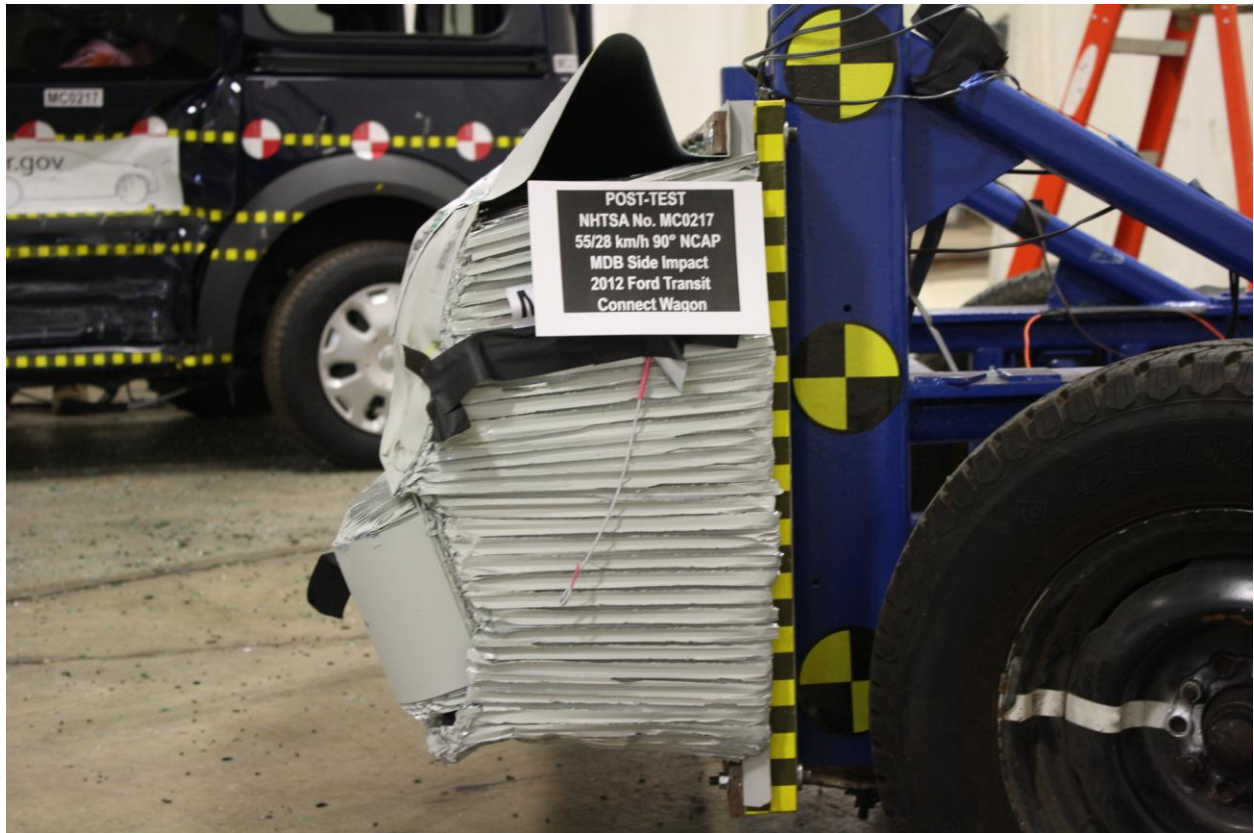
Figure A-87: Post-Test Left Side View of MDB Impactor Face
