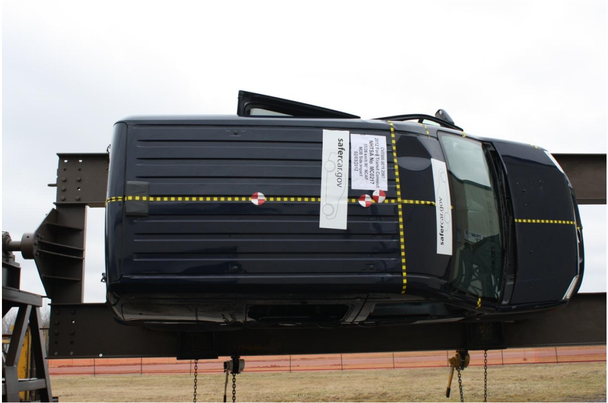
Figure A-95: FMVSS No. 301 Static Rollover 90 Degrees
