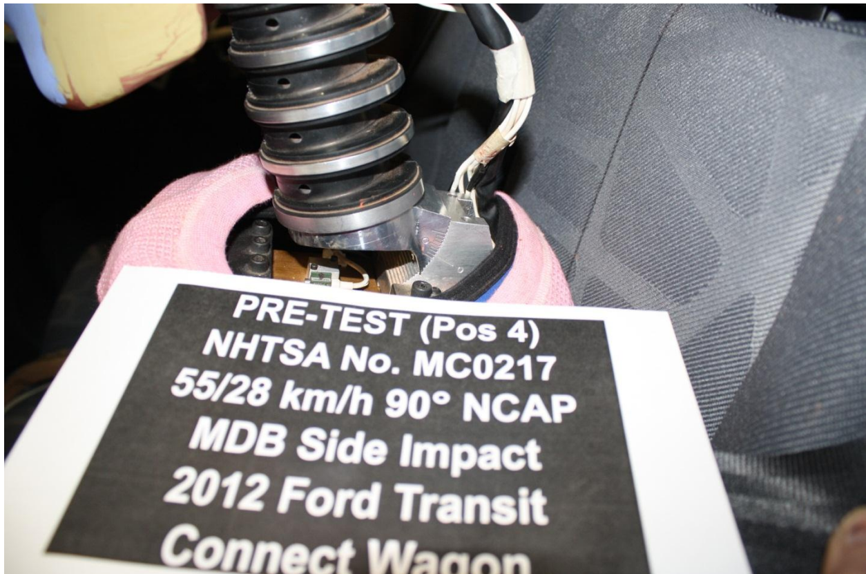
Figure A-61: Pre-Test View of Rear Passenger Dummy's Neck Showing Position of Adjustable Neck Bracket
