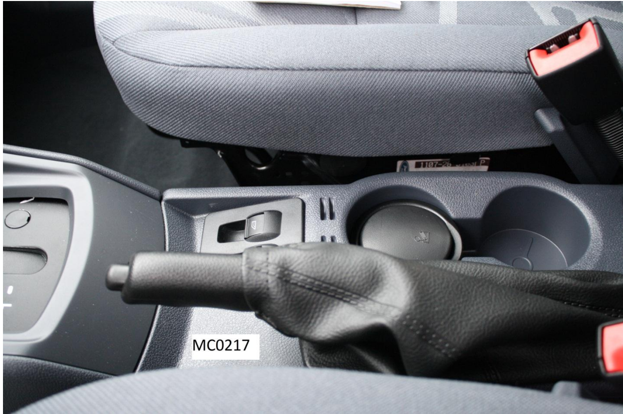
Figure A-37: View of Disengaged Parking Brake
