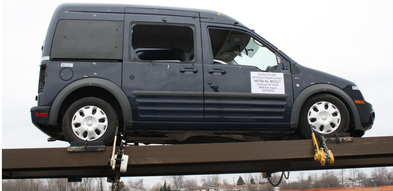
Figure A-98: FMVSS No. 301 Static Rollover 360 Degrees
