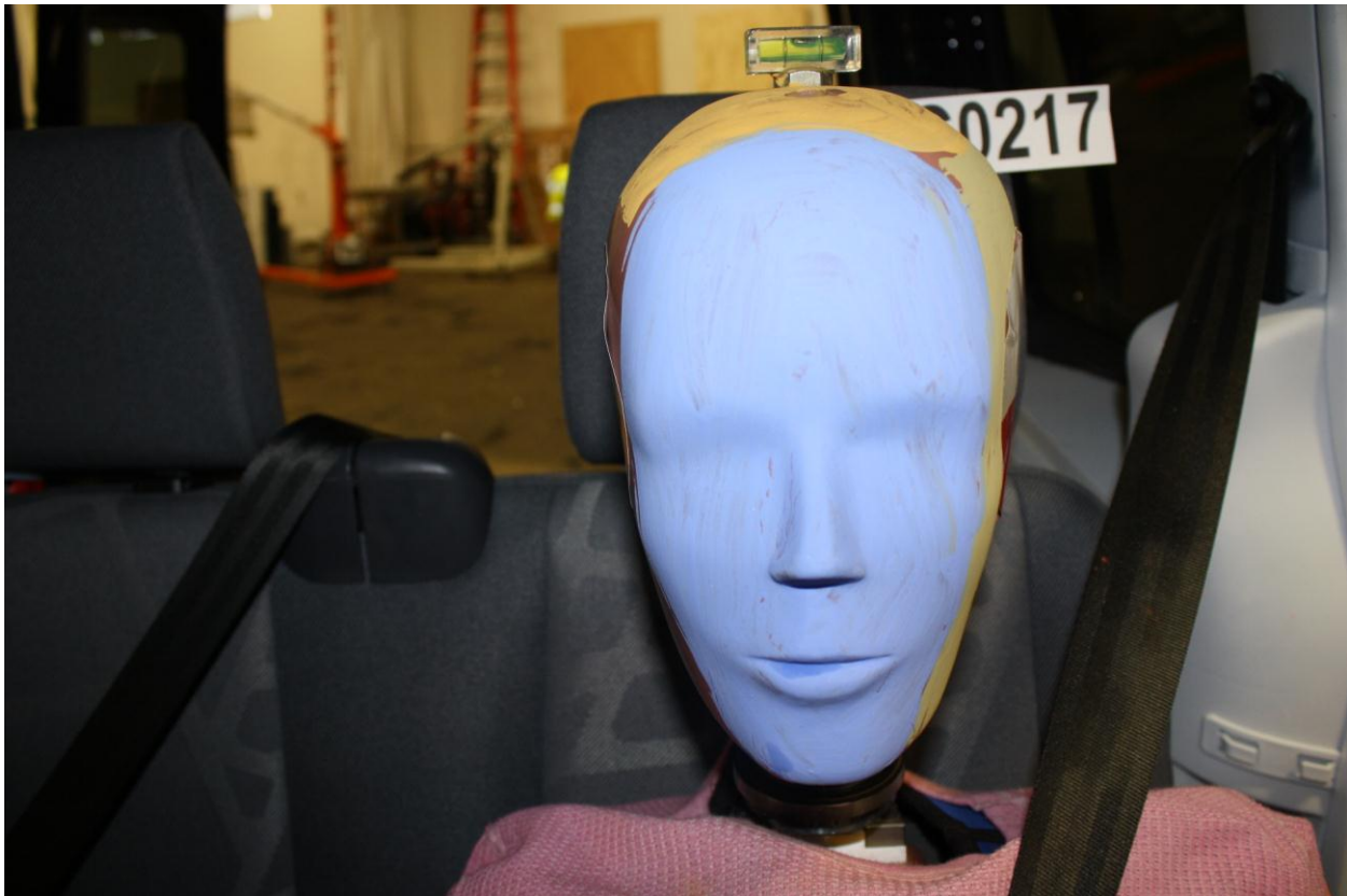
Figure A-58: Pre-Test Frontal View of Rear Passenger Dummy Head and Shoulders in Relation to Head Restraint
