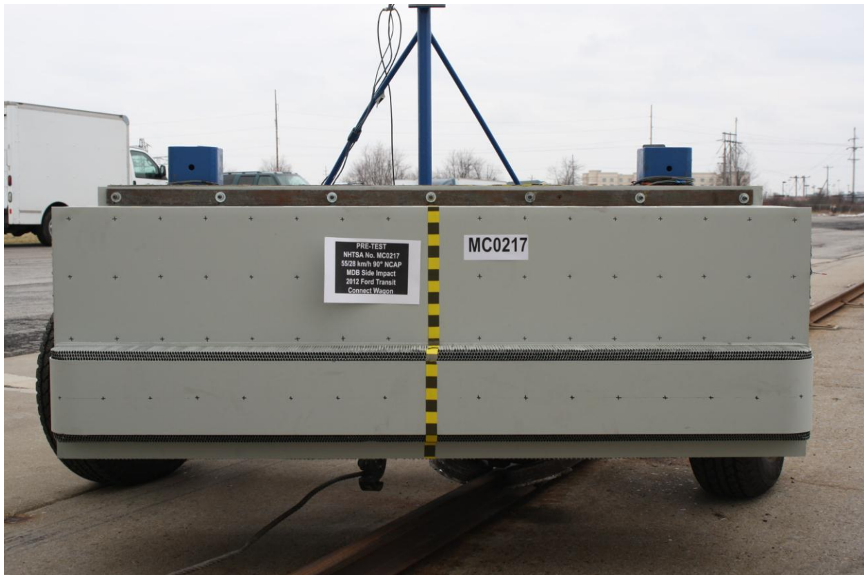
Figure A-82: Pre-Test Front View of MDB Impactor Face
