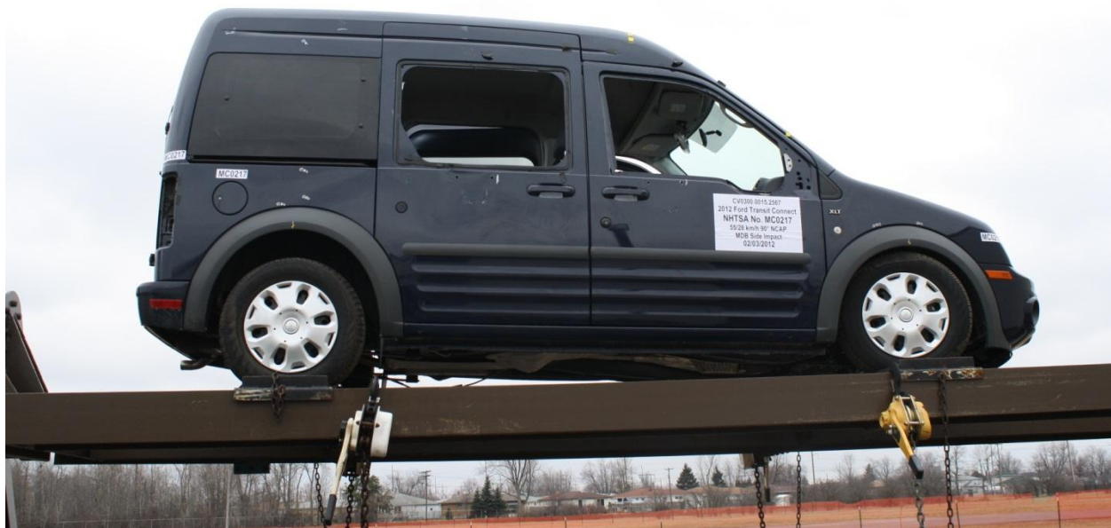
Figure A-94: FMVSS No. 301 Static Rollover 0 Degrees
