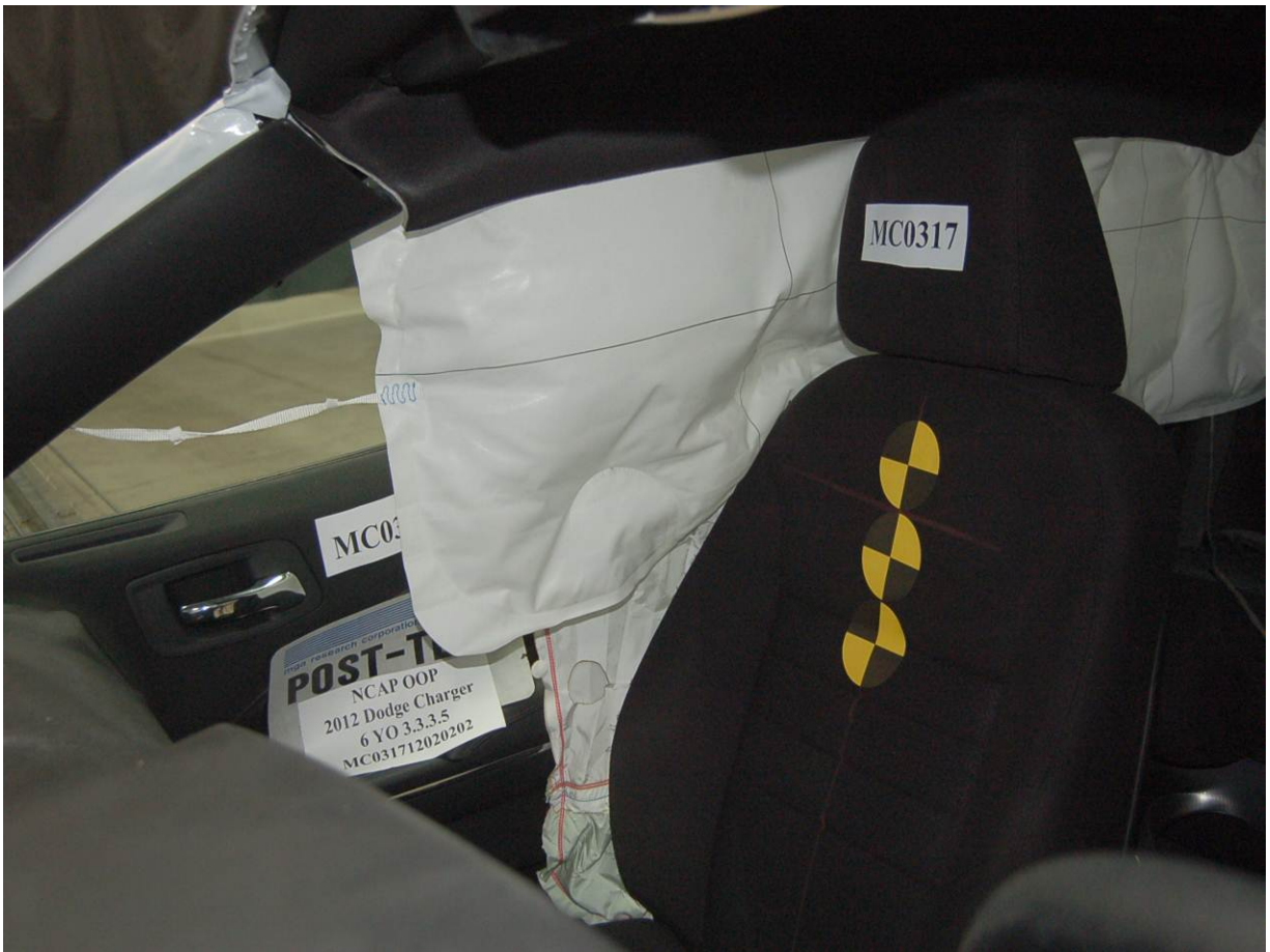
Post-Test Curtain Airbag Left 3/4 Front View
