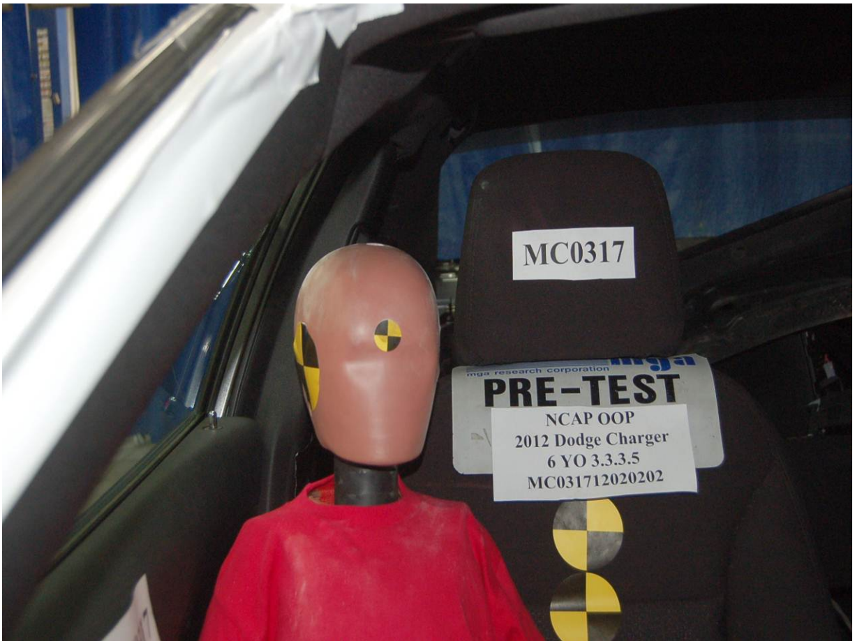
Pre-Test 6-Year-Old Child Dummy Front Closeup View
