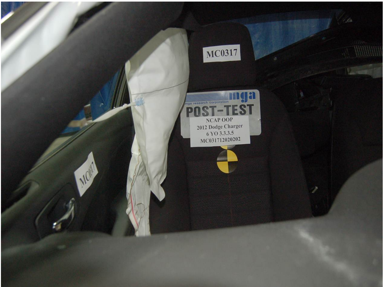
Post-Test Curtain Airbag Front View
