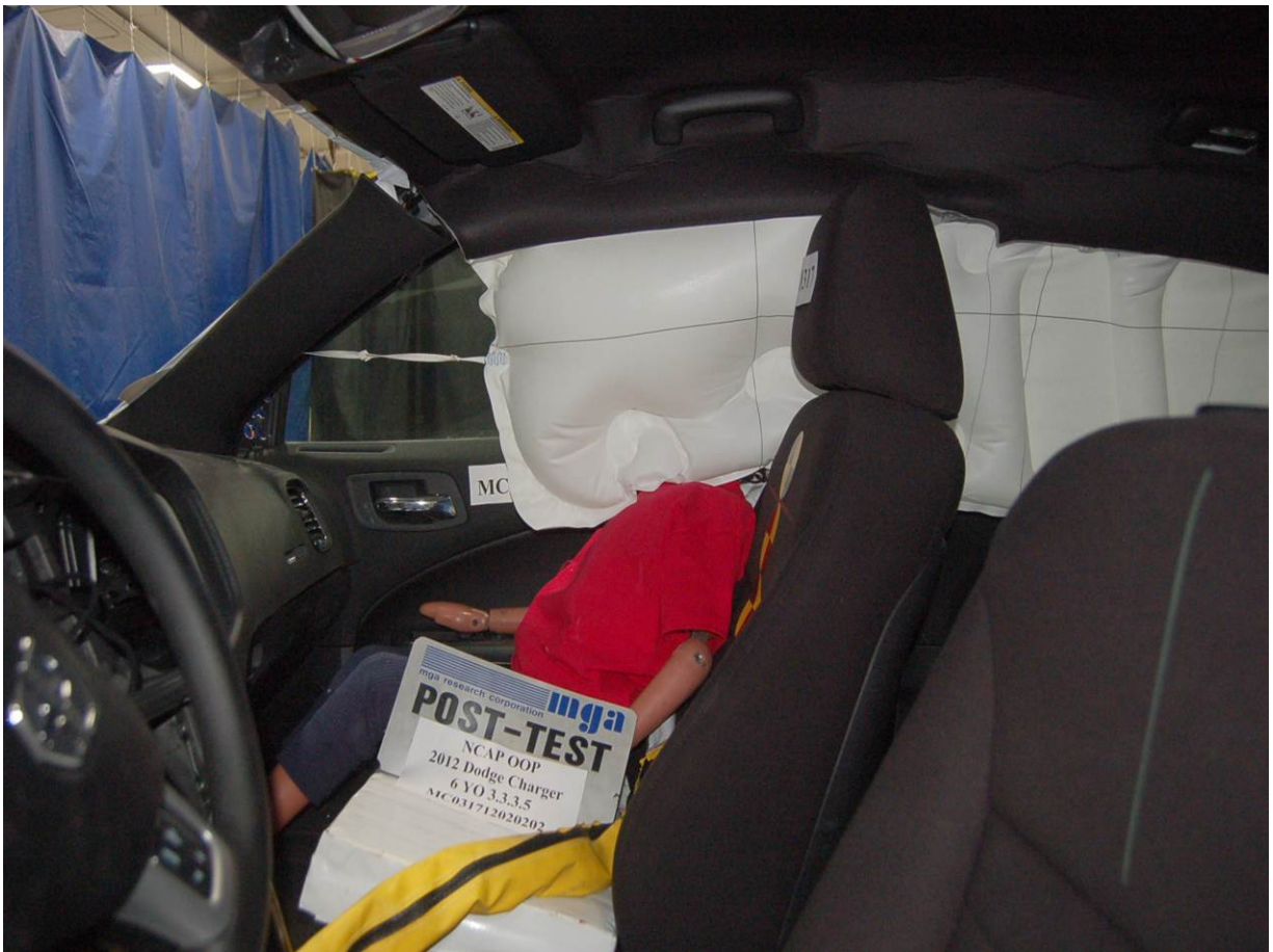
Post-Test 6-Year-Old Child Dummy Left Side View
