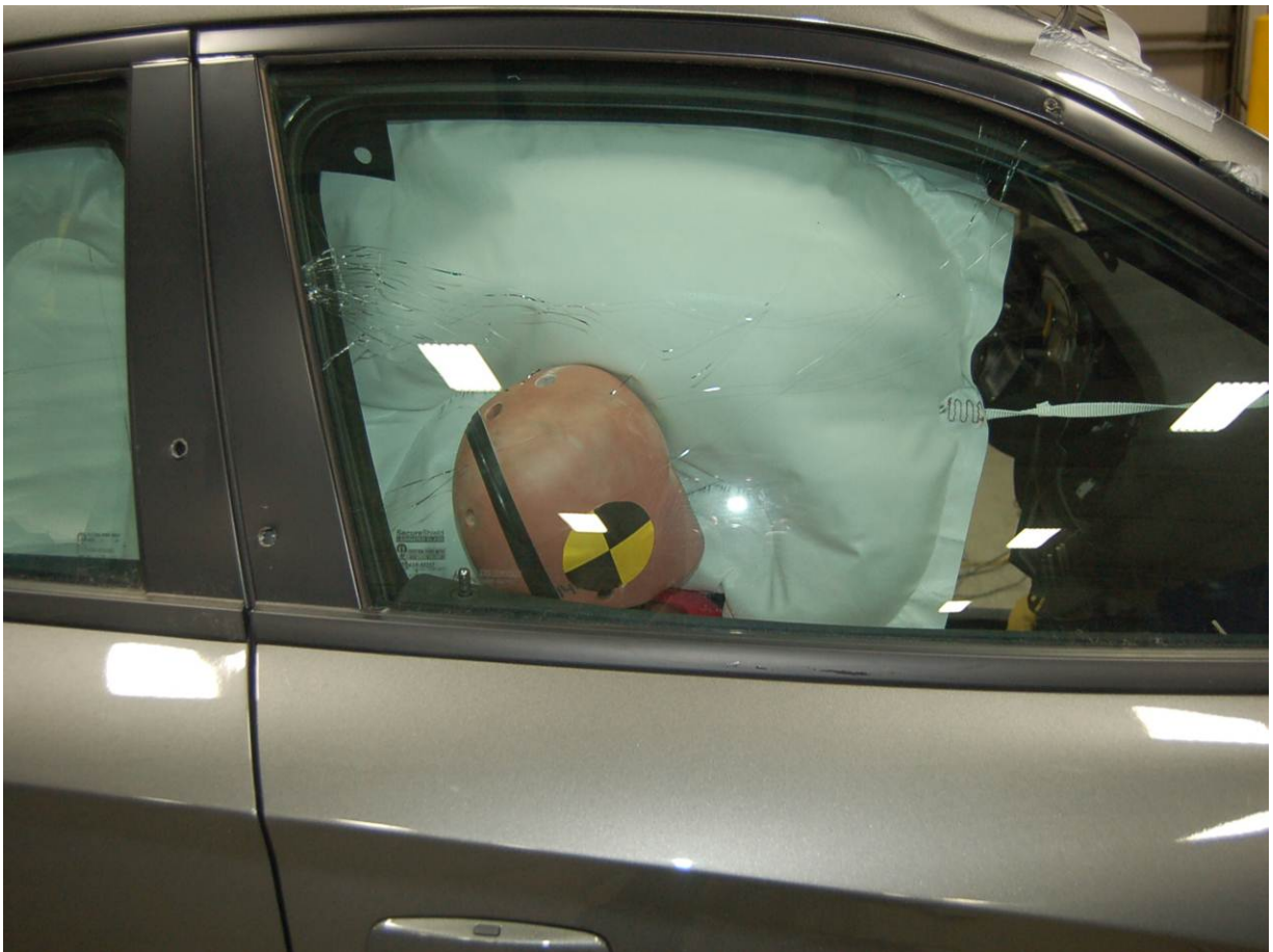
Post-Test 6-Year-Old Child Dummy Right Side View
