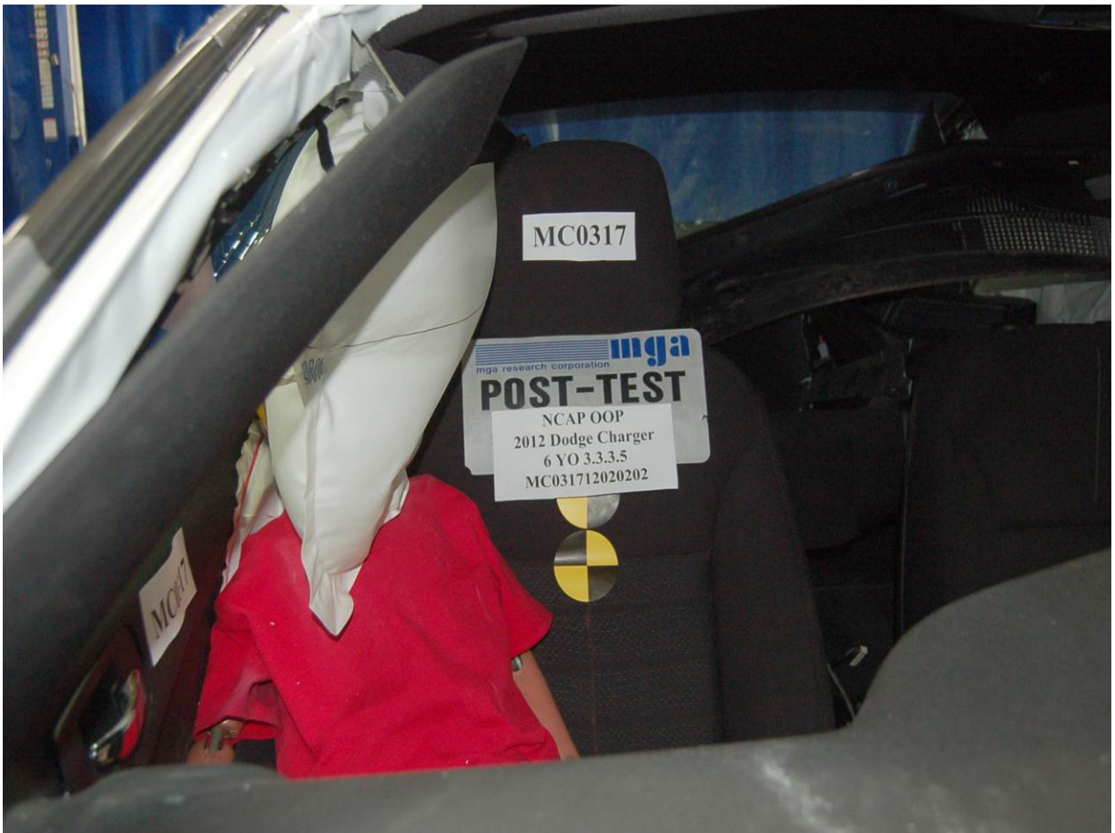
Post-Test 6-Year-Old Child Dummy Front View
