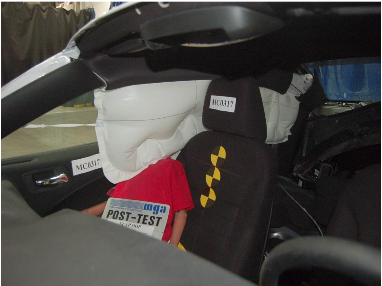
Post-Test 6-Year-Old Child Dummy Left 3/4 Front View
