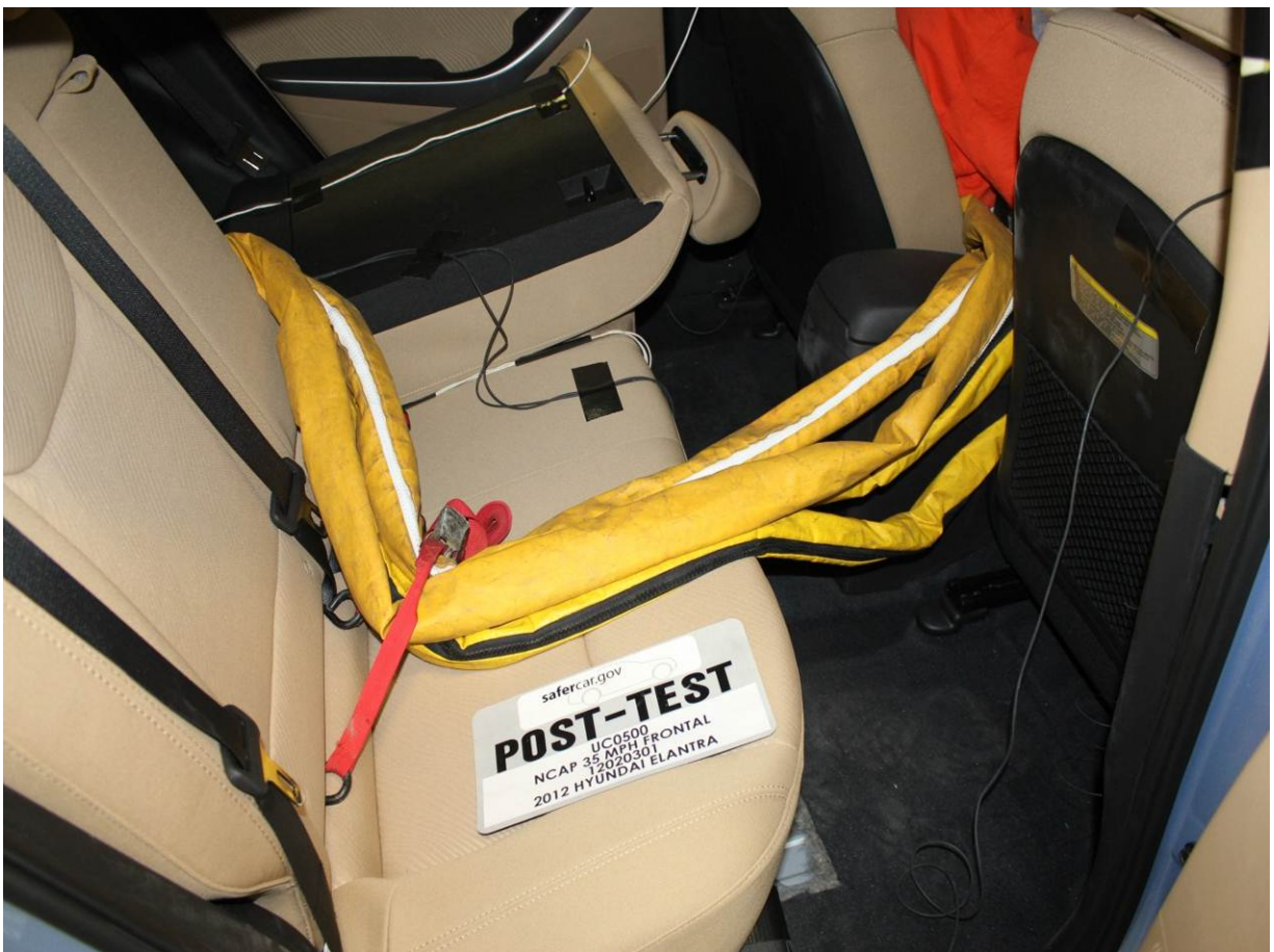
Post-Test Dummy Cable Routing
