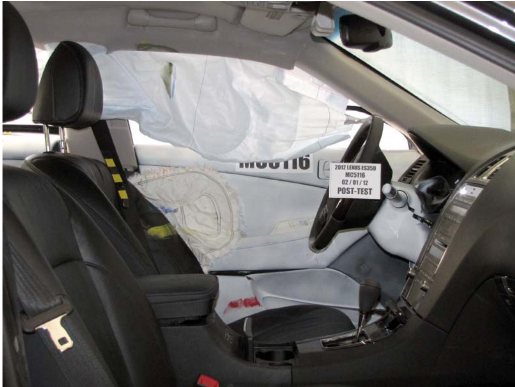
FIGURE 47. Post-Test Driver Inner Door Panel View
