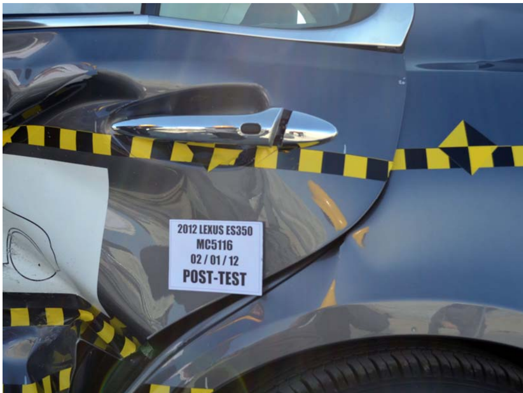
FIGURE 24. Post-Test Left Rear Door Latch Close-Up
