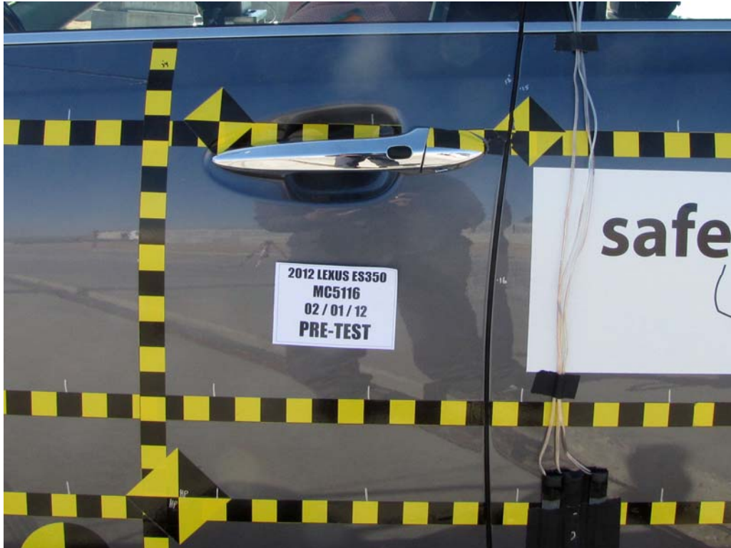
FIGURE 21. Pre-Test Left Front Door Latch Close-Up
