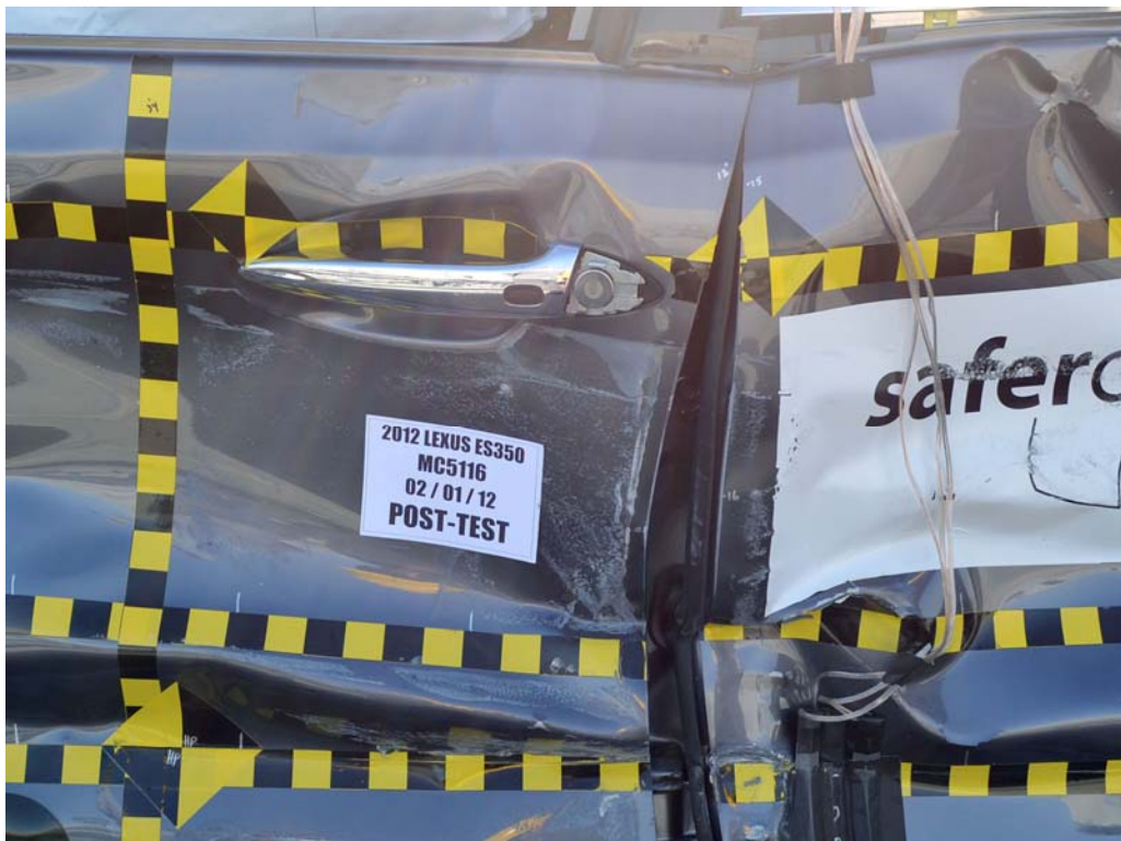
FIGURE 22. Post-Test Left Front Door Latch Close-Up
