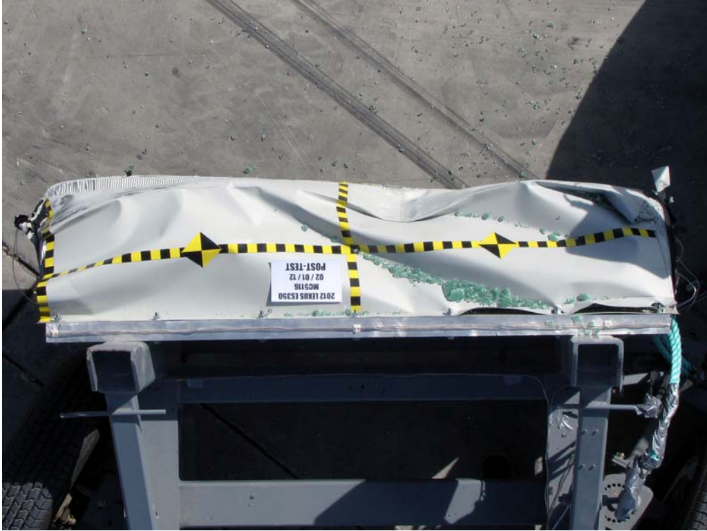
FIGURE 85. Post-Test Top View of MDB Impactor Face
