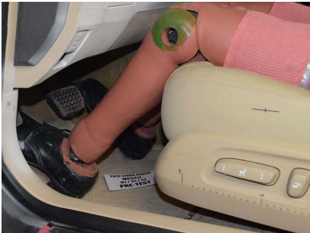
FIGURE 32. Pre-Test Placement of Dummy's Feet
