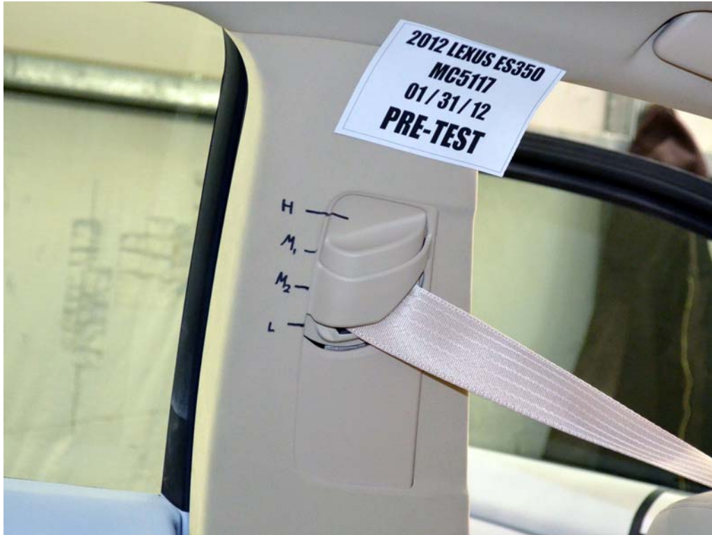
FIGURE 33. Pre-Test View of Belt Anchorage for Dummy
