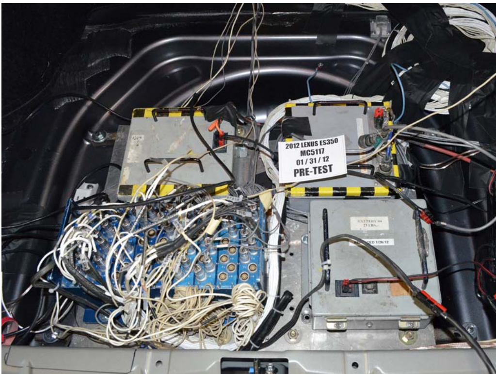
FIGURE 60. Pre-Test Ballast View
