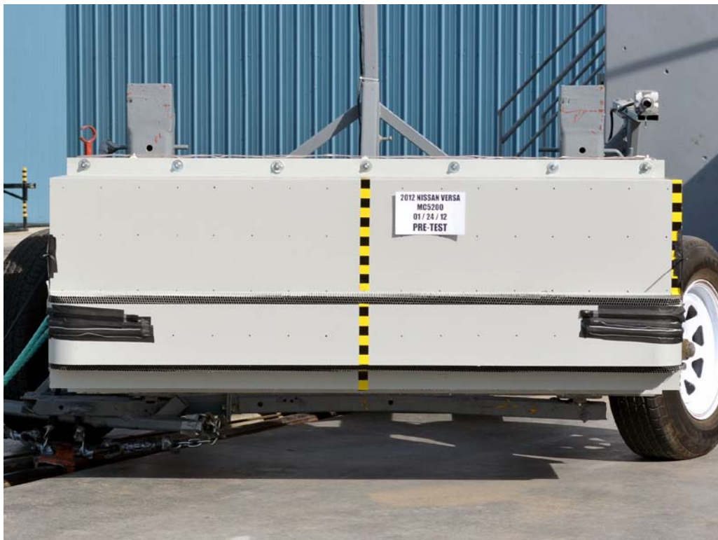
FIGURE 82. Pre-Test Front View of MDB Impactor Face
