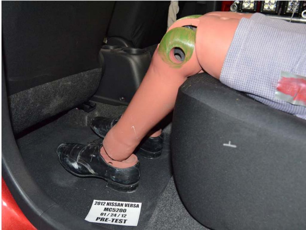
FIGURE 63. Pre-Test Placement of Rear Passenger Dummy's Feet
