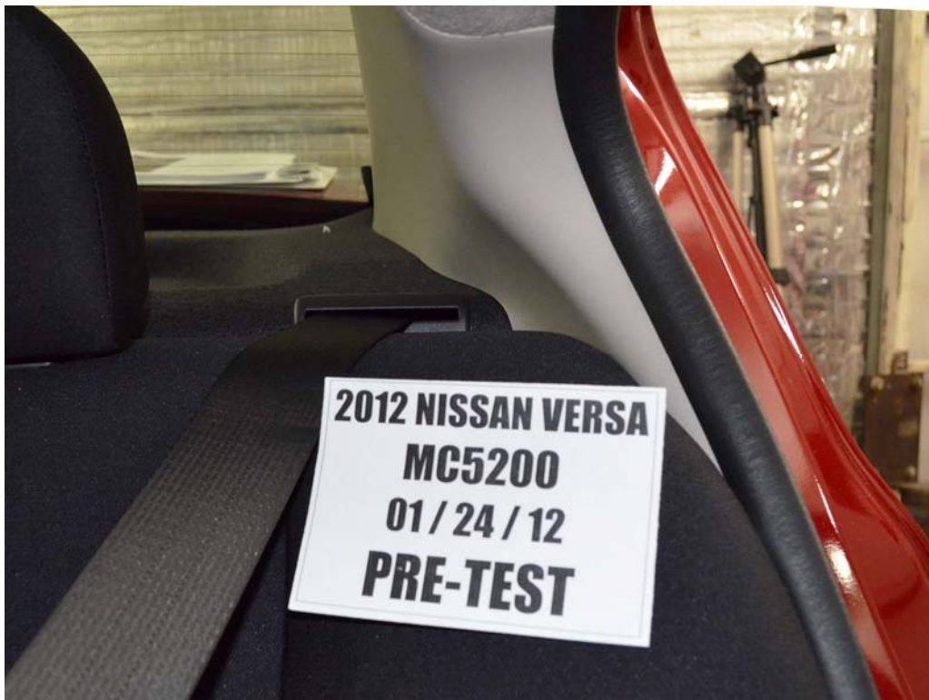
FIGURE 64. Pre-Test View of Belt Anchorage for Rear Passenger Dummy
