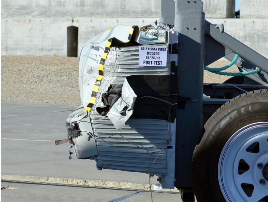
FIGURE 87. Post-Test Left Side View of MDB Impactor Face
