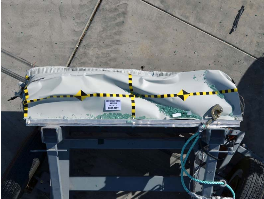
FIGURE 85. Post-Test Top View of MDB Impactor Face
