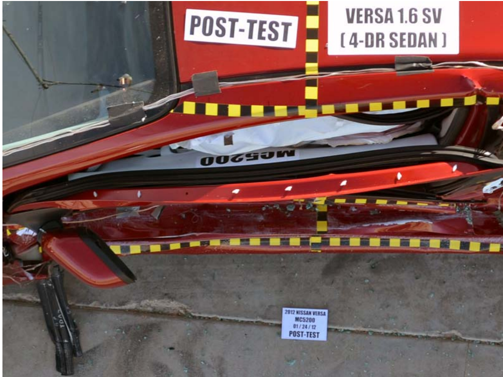
FIGURE 43. Post-Test Driver Dummy and Door Clearance View
