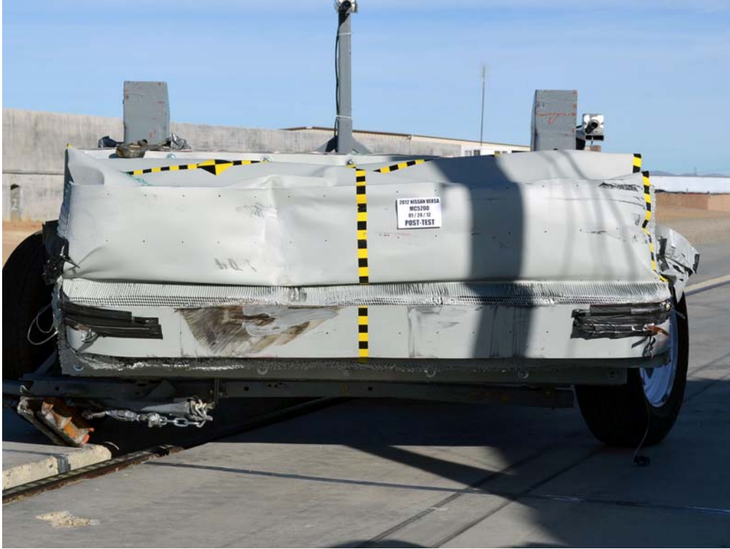
FIGURE 83. Post-Test Front View of MDB Impactor Face
