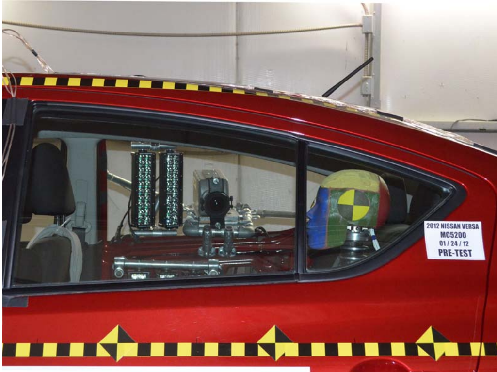
FIGURE 55. Pre-Test Left Side View of Rear Passenger Dummy Shoulder and Door Top View
