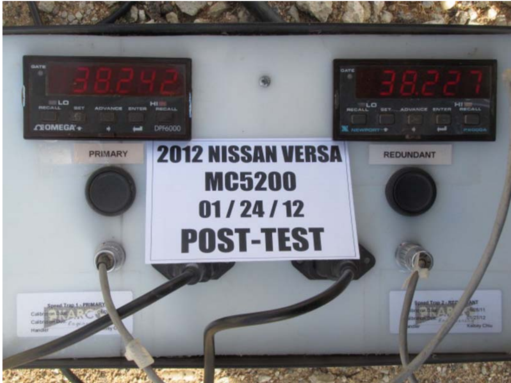
FIGURE 93. Post-Test Primary and Redundant Speed Trap Read-Out
