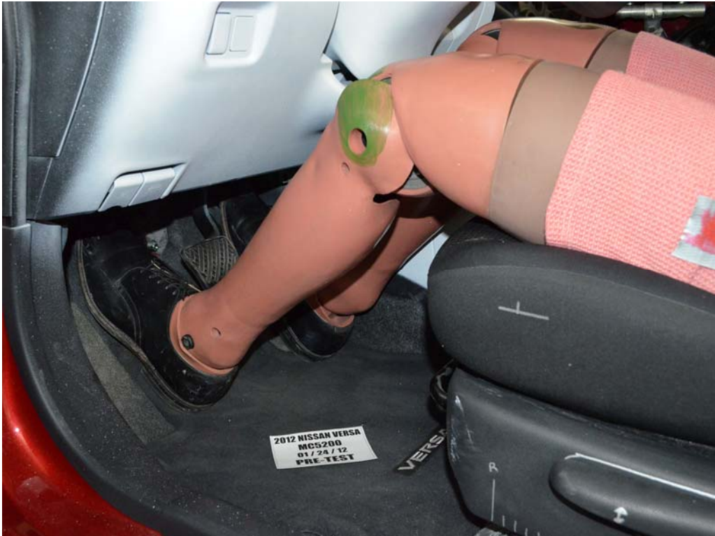
FIGURE 34. Pre-Test Placement of Driver Dummy's Feet
