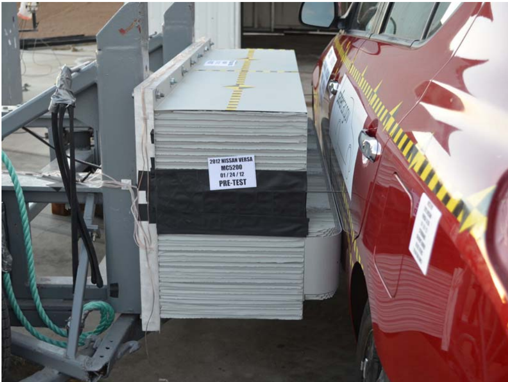
FIGURE 18. Pre-Test Right Side View of MDB Positioned Against Side of Test Vehicle
