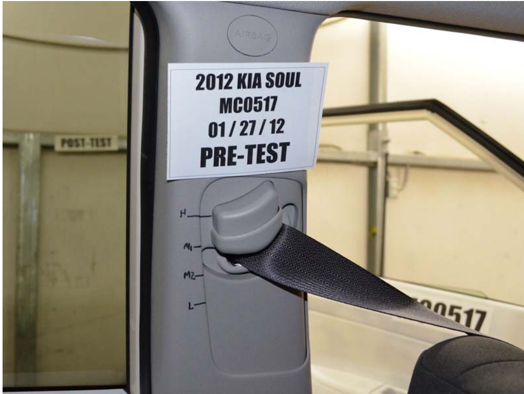
FIGURE 33. Pre-Test View of Belt Anchorage for Dummy
