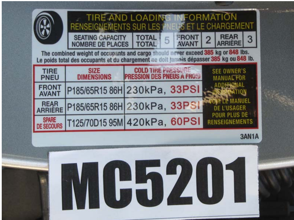
FIGURE 55. Close-Up View of Vehicle's Tire Information Placard
