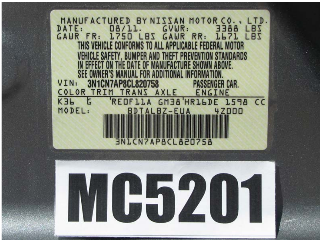
FIGURE 54. Close-Up View of Vehicle's Certification Label
