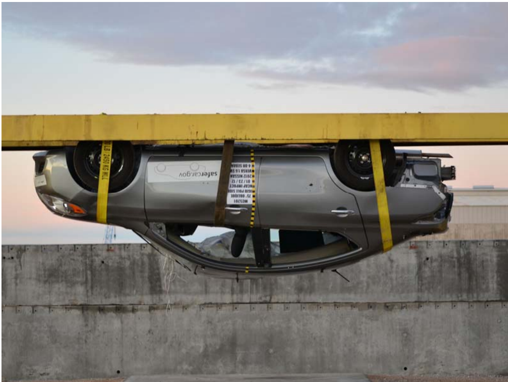
FIGURE 64. FMVSS No. 301-305 Rollover 180 Degrees
