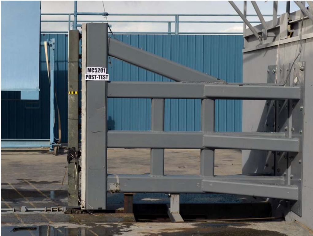
FIGURE 59. Post-Test Pole Barrier Side View
