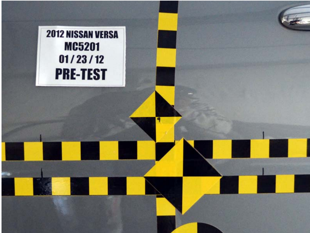
FIGURE 19. Pre-Test Close-Up View of Impact Point Target
