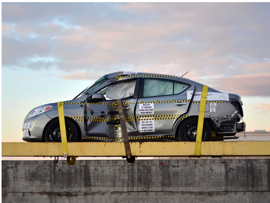
FIGURE 62. FMVSS No. 301-305 Rollover 0 Degrees
