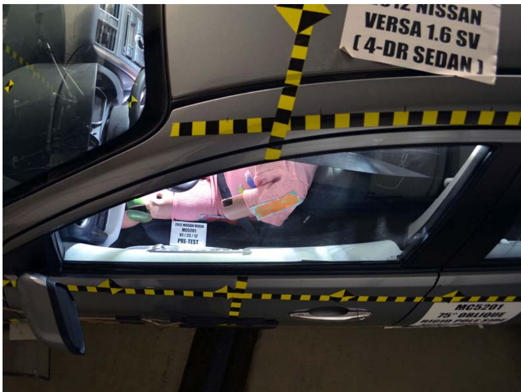
FIGURE 40. Pre-Test Driver Dummy and Door Clearance
