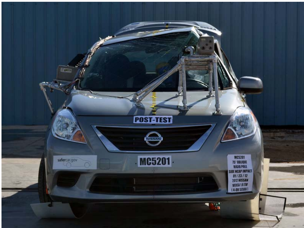
FIGURE 4. Post-Test Frontal View of Test Vehicle
