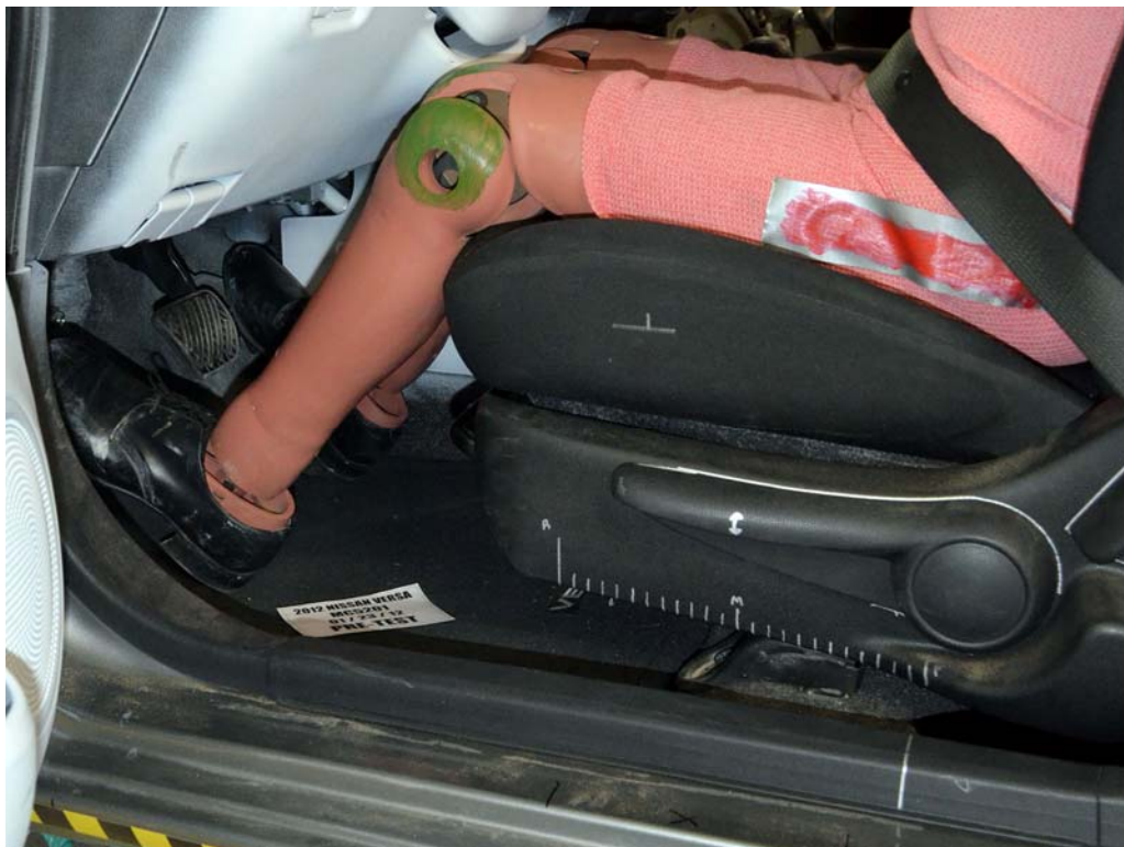
FIGURE 32. Pre-Test Placement of Dummy's Feet
