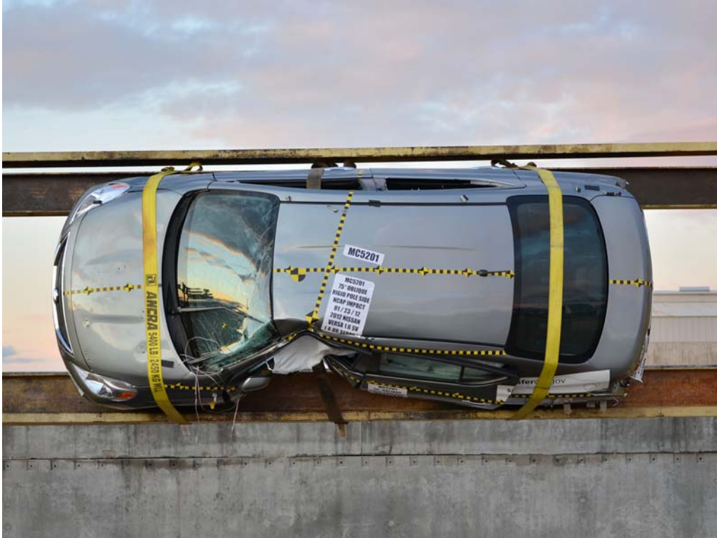
FIGURE 63. FMVSS No. 301-305 Rollover 90 Degrees
