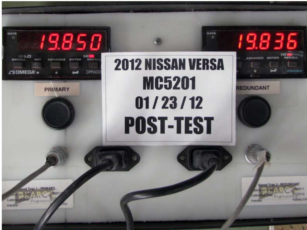
FIGURE 61. Post-Test Primary and Redundant Speed Trap Read-Out
