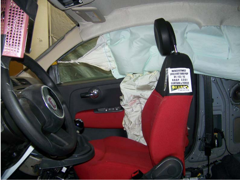
FIGURE 13. Post-Test Airbags, Left Side View
