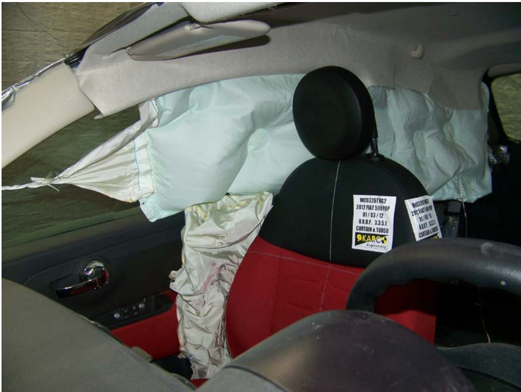
FIGURE 14. Post-Test Airbags, Left Front ¾ View
