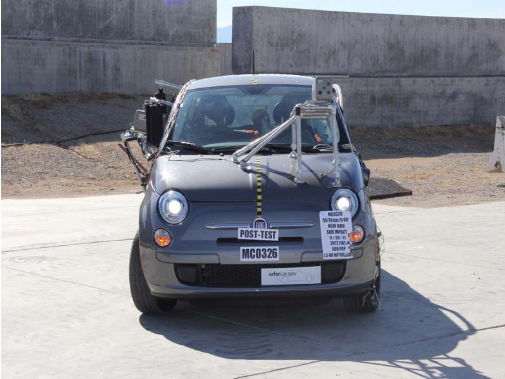
FIGURE 3. Post-Test Front View of NCAP Side Impact Test
