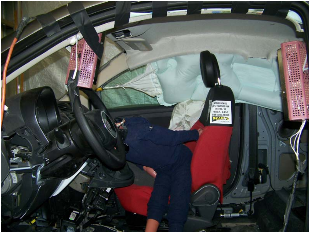
FIGURE 8. Post-Test Dummy Position, Left Side View
