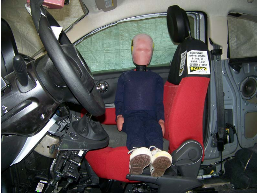
FIGURE 7. Pre-Test Dummy Position, Left Side View
