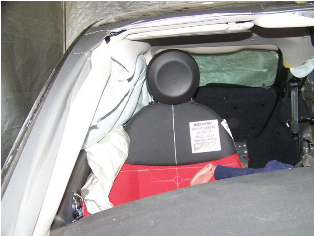
FIGURE 12. Post-Test Dummy Position, Front View
