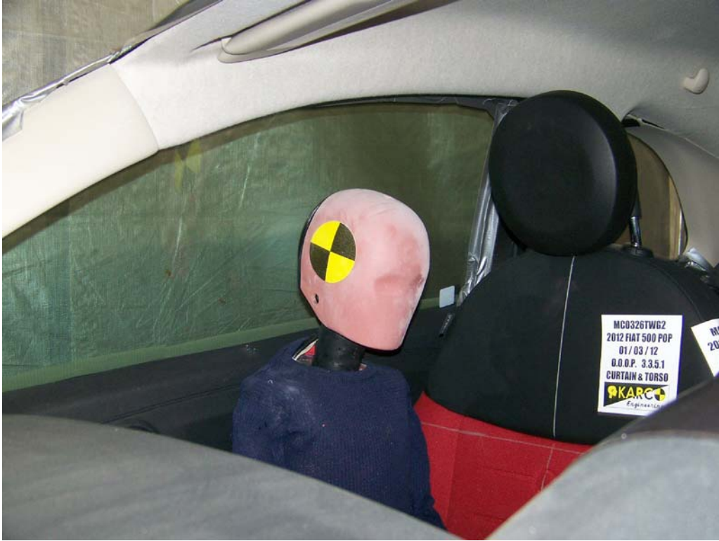
FIGURE 9. Pre-Test Dummy Position, \frac{3}{4} View
