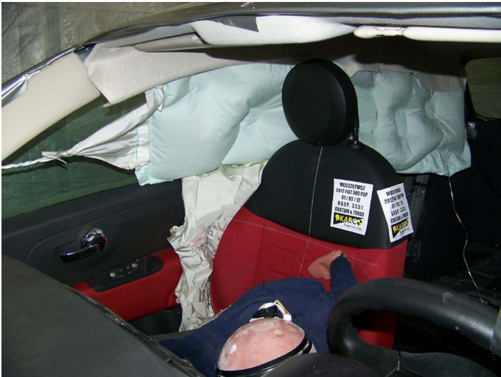
FIGURE 10. Post-Test Dummy Position, \frac{3}{4} View
