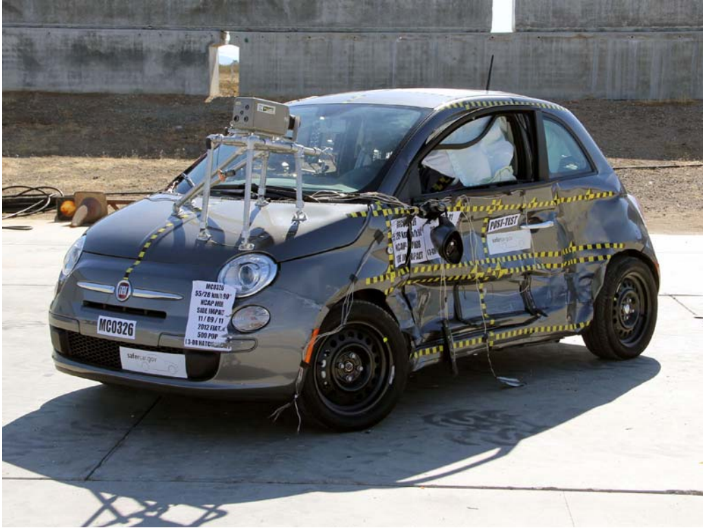
FIGURE 5. Post-Test Right Front 3/4 View of NCAP Side Impact Test
