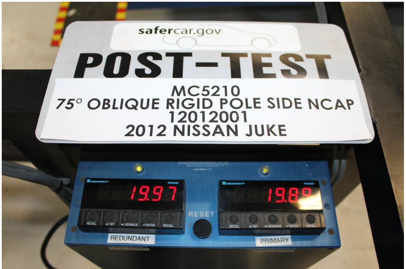
Post-Test Primary and Redundant Speed Trap Read-Out
