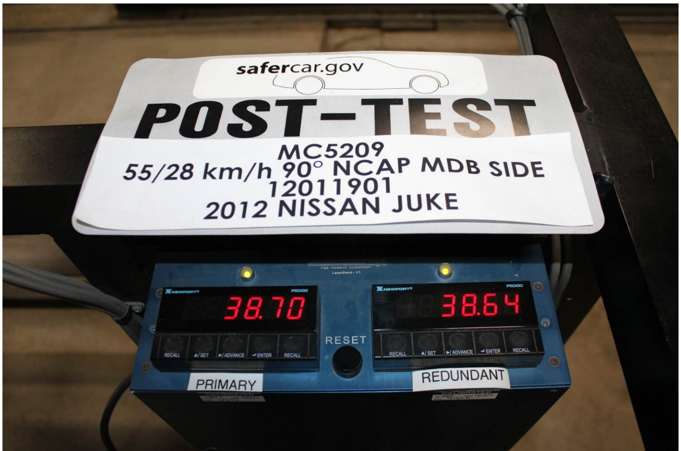
Post-Test Primary and Redundant Speed Trap Read-Out
