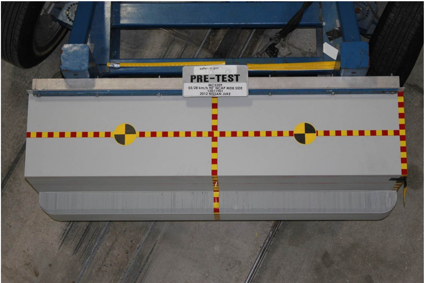
Pre-Test Top View of MDB Impactor Face
