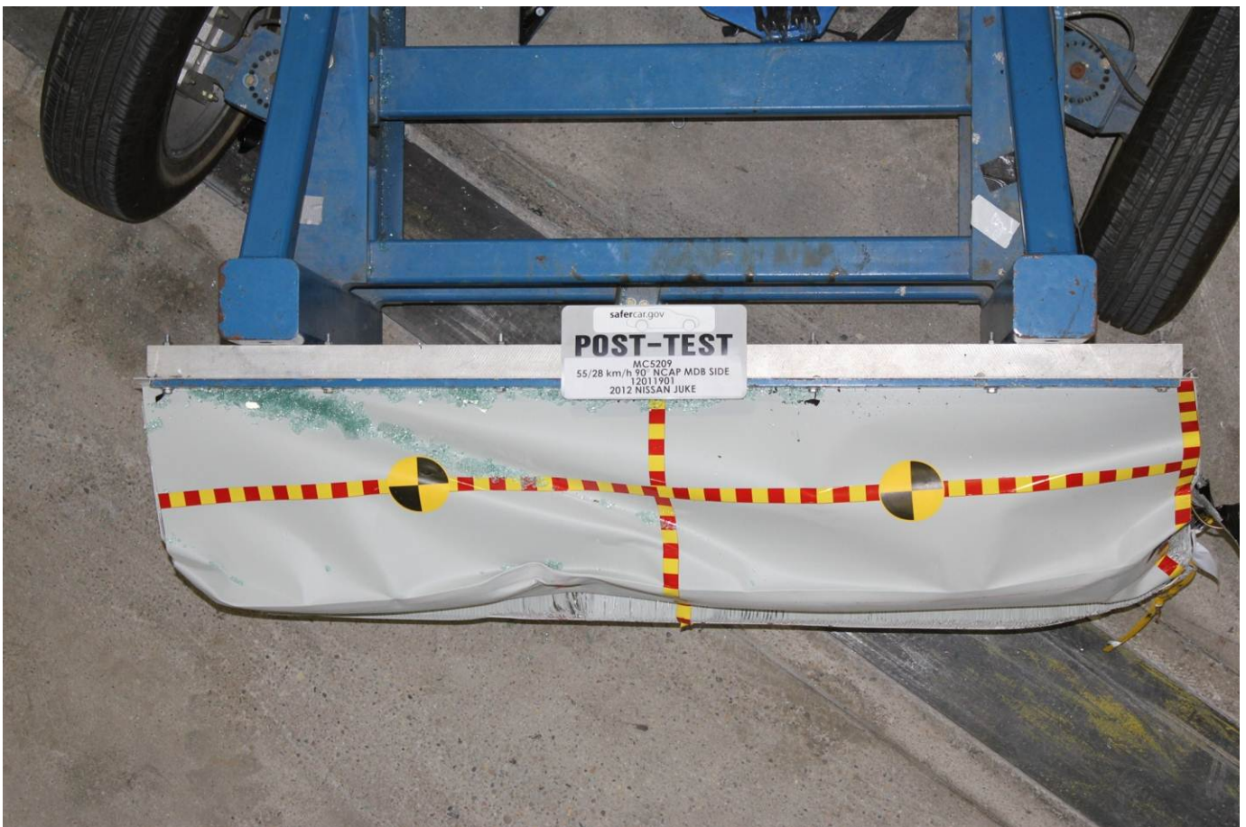
Post-Test Top View of MDB Impactor Face
