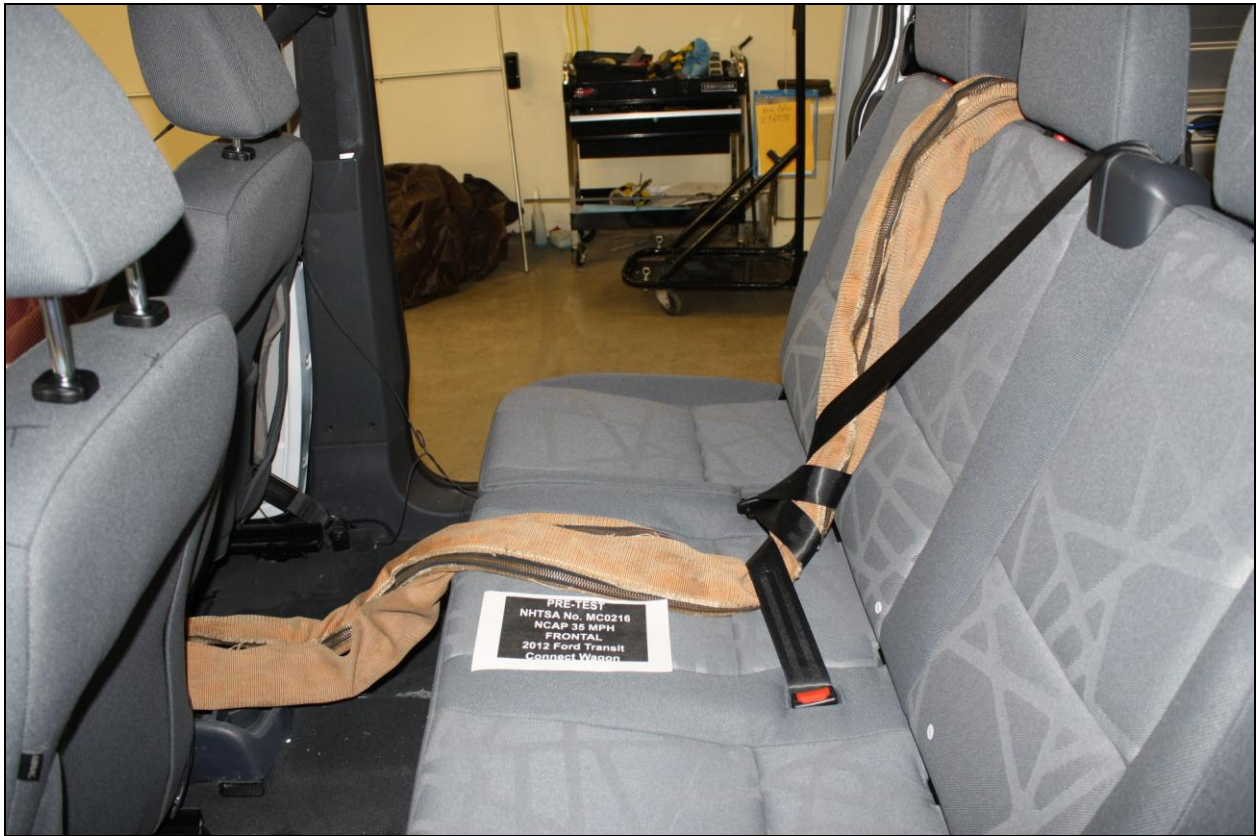
Figure A-27: Pre-Test Dummy Cable Routing
