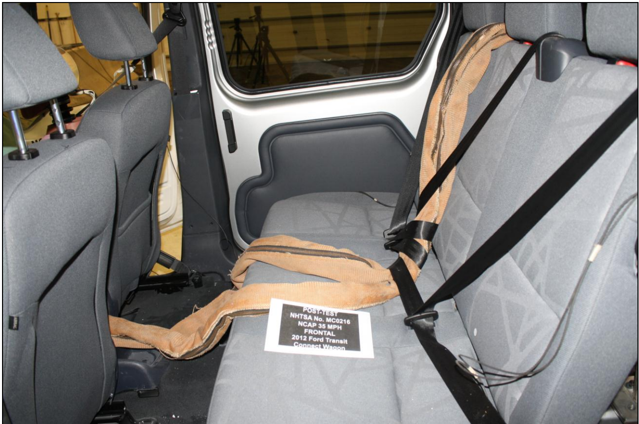
Figure A-28: Post-Test Dummy Cable Routing
