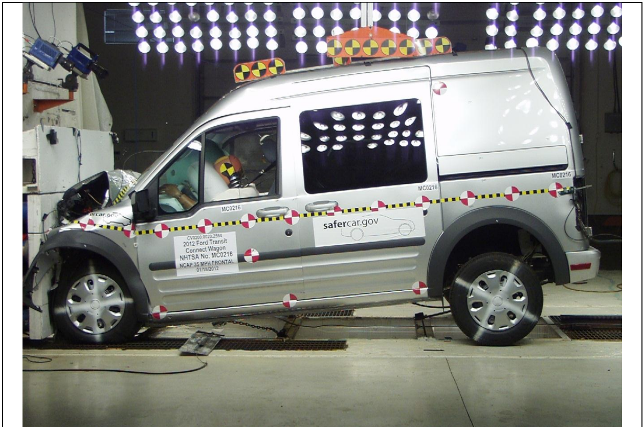
Figure A-71: 2012 Ford Transit Connect XLT Wagon Frontal Impact Event
