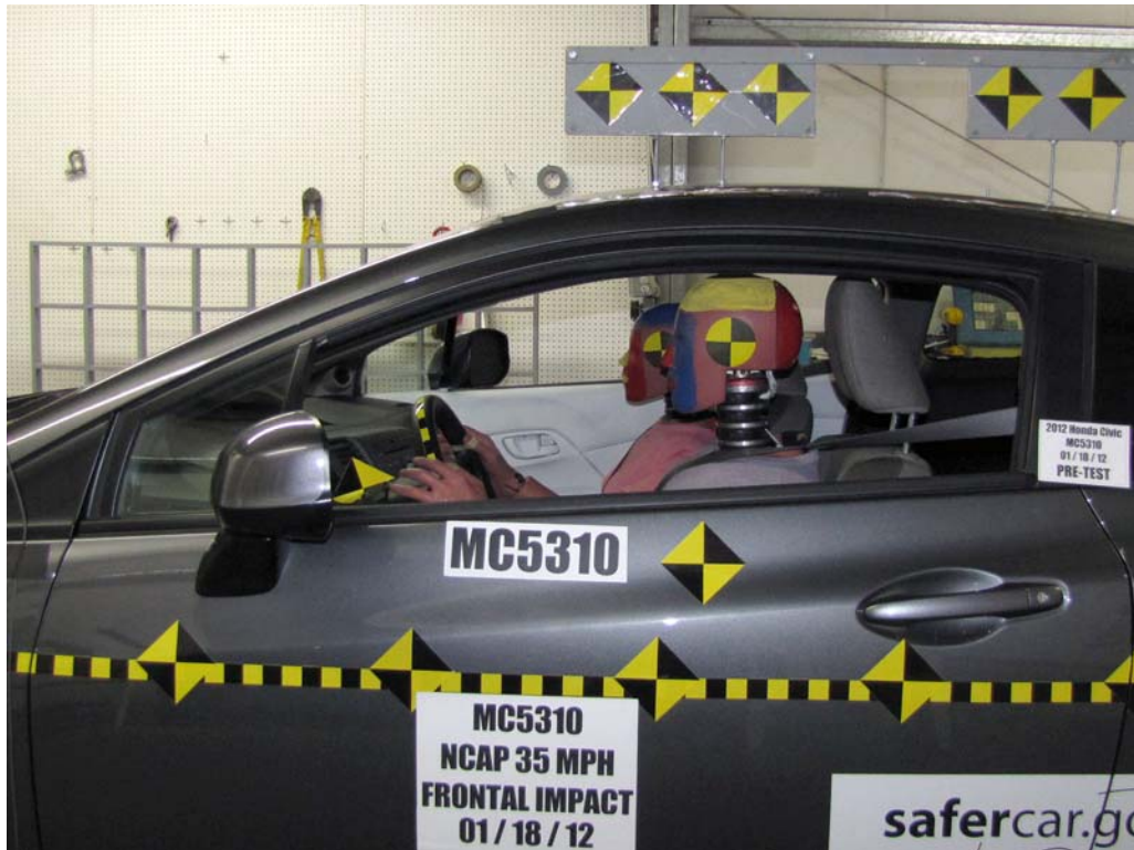
FIGURE 31. Pre-Test Driver Dummy Window View
