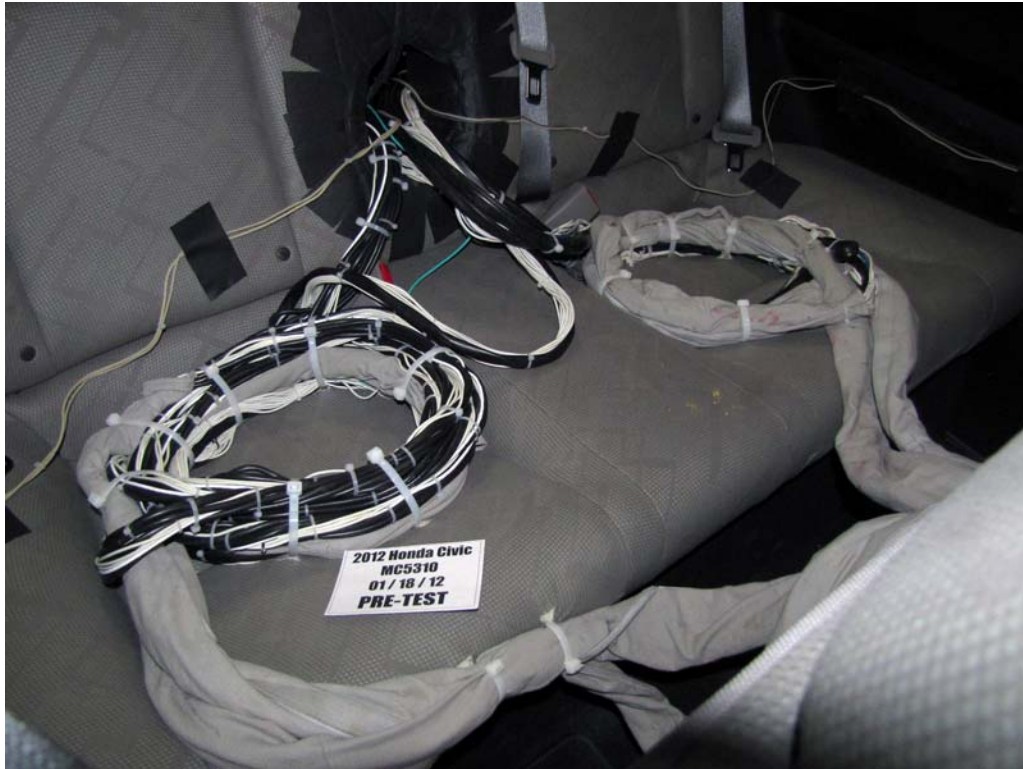
FIGURE 27. Pre-Test Dummy Cable Routing
