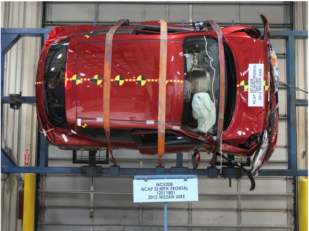
Vehicle at 90 Degrees on Static Rollover Device
