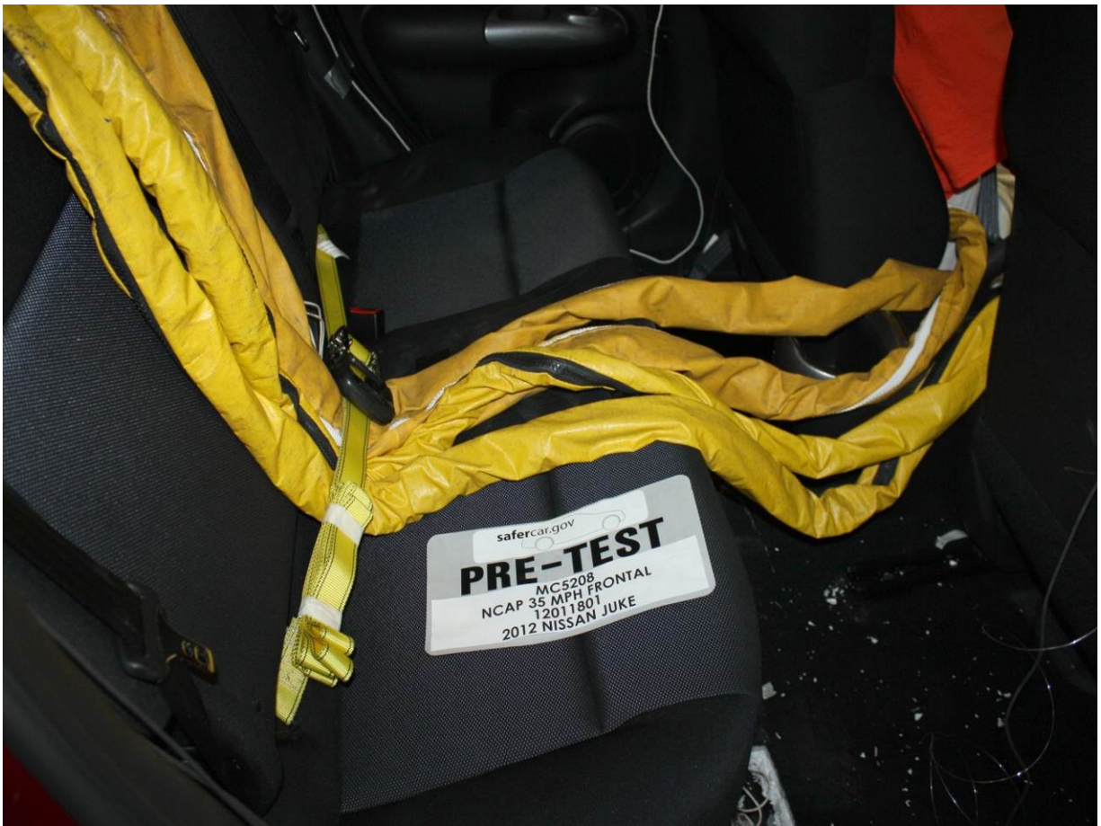
Pre-Test Dummy Cable Routing
