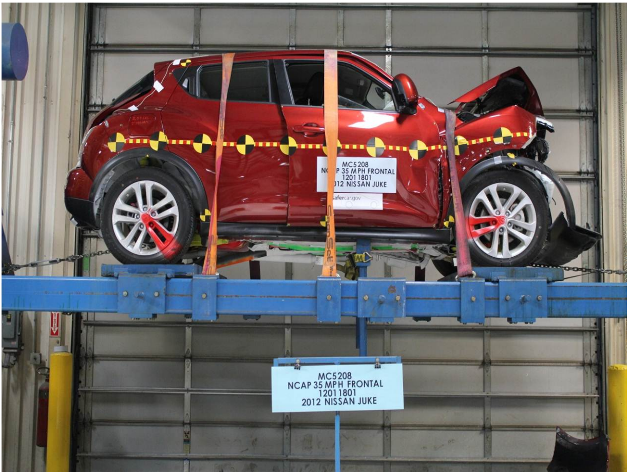
Vehicle at 360 Degrees on Static Rollover Device
