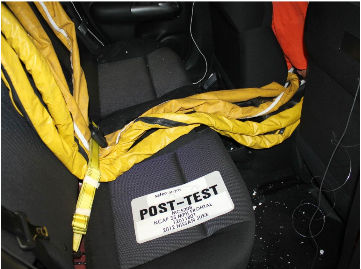
Post-Test Dummy Cable Routing
